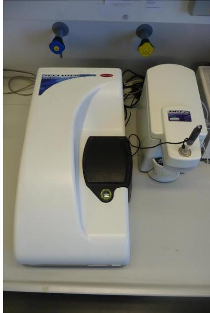
*Figure A.GRANULO.5 Zetasizer nano zs de Malvern Instruments*
