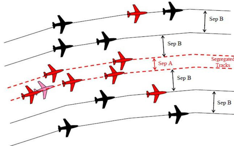
FIGURE 2.2: Creating of segregated tracks within the OTS with reduced lateral separation<sup>6</sup>
