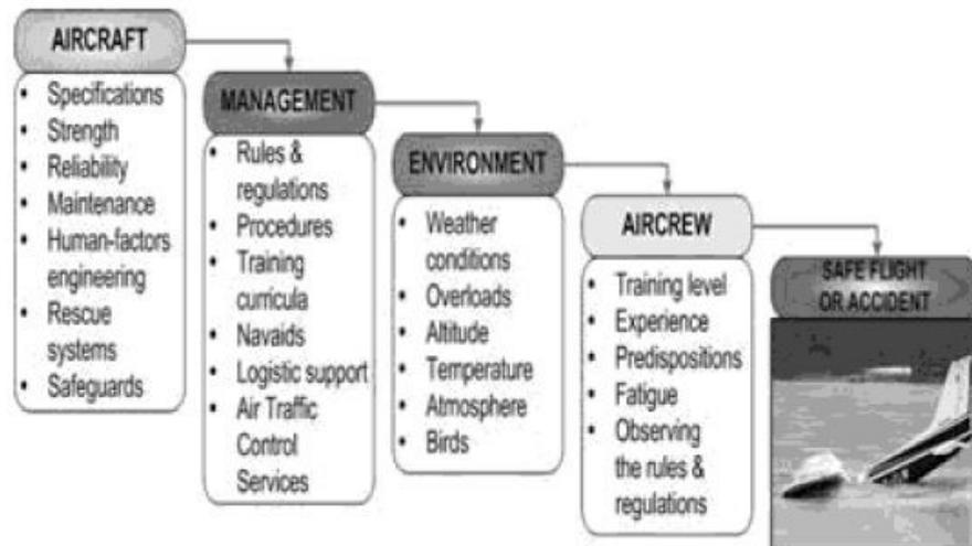
FIGURE U.2: A chain of safety for a flight<sup>2</sup>
