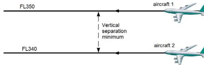
FIGURE 1.9: Vertical separation
