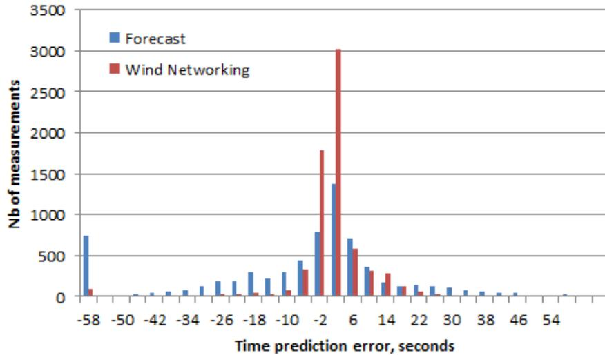
FIGURE 3.21: MF and WN prediction error distribution for 1,000 flights on the OTS
