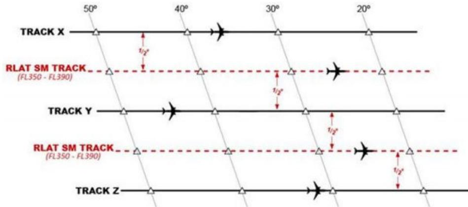
FIGURE 2.3: Creating of additional tracks within the OTS according to RLatSM<sup>8</sup>
