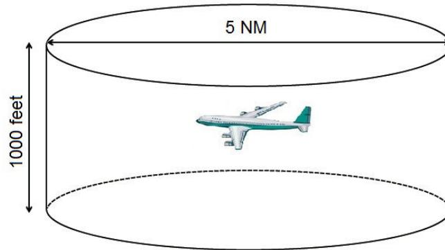
FIGURE 1.13: Aircraft reserved block within en-route radar separation
