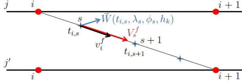
FIGURE 3.3: Simulation of flight between two waypoints
