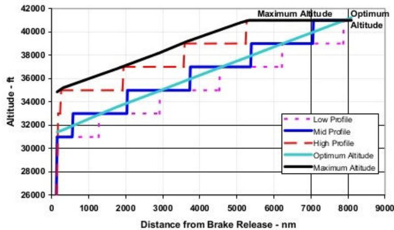
FIGURE 1.4: Continuous optimal flight altitude profile vs. step climbs<sup>12</sup>
