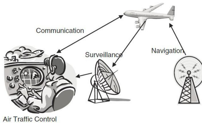
FIGURE 1.3: Generic systems of Air Traffic Control<sup>11</sup>
