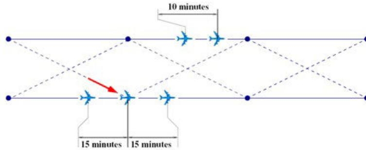
FIGURE 1.19: Current longitudinal separation standards in NAT (CSS)
