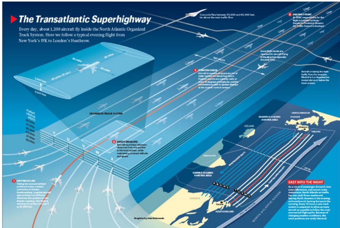
FIGURE 1.18: NAT traffic model with separation standards<sup>39</sup>
