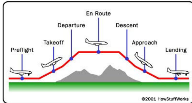
FIGURE 1.2: Typical flight phases<sup>8</sup>
