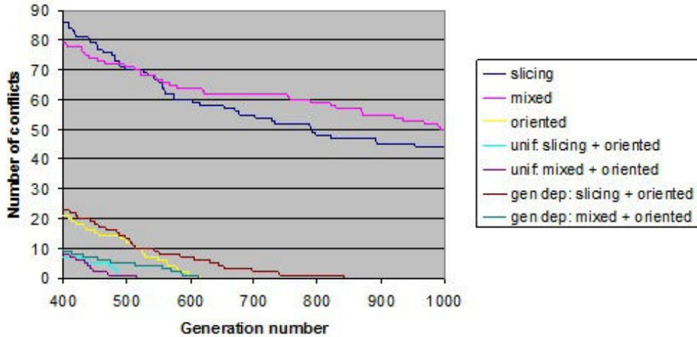
FIGURE Q.3: Convergence of GA with different crossover methods in logarithmic scale
