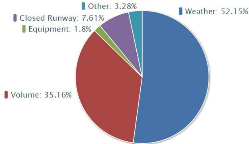
FIGURE 3.2: Distribution of causes of the U.S. National Aviation System Delays from December 2013 to December 2014<sup>2</sup>
