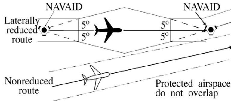
FIGURE 1.10: Lateral separation of aircraft on different routes<sup>20</sup>
