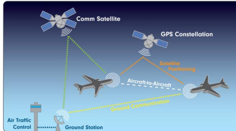
FIGURE 1.14: Automatic Dependent Surveillance-Broadcast technology<sup>31</sup>
