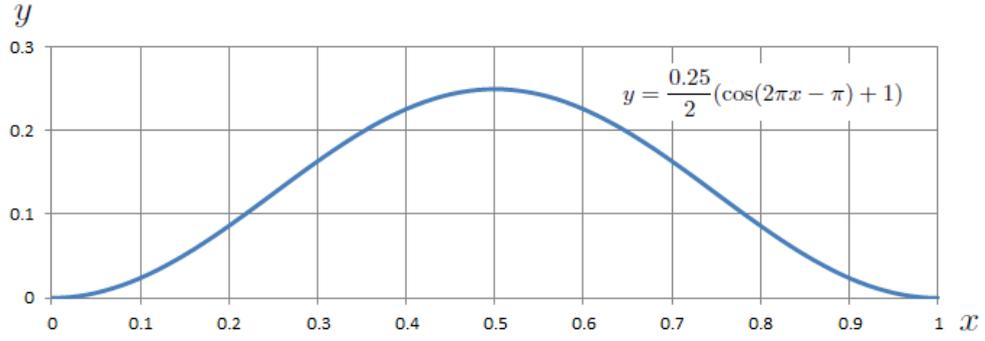
FIGURE 4.6: A cosine-like function used for trajectory transformation
