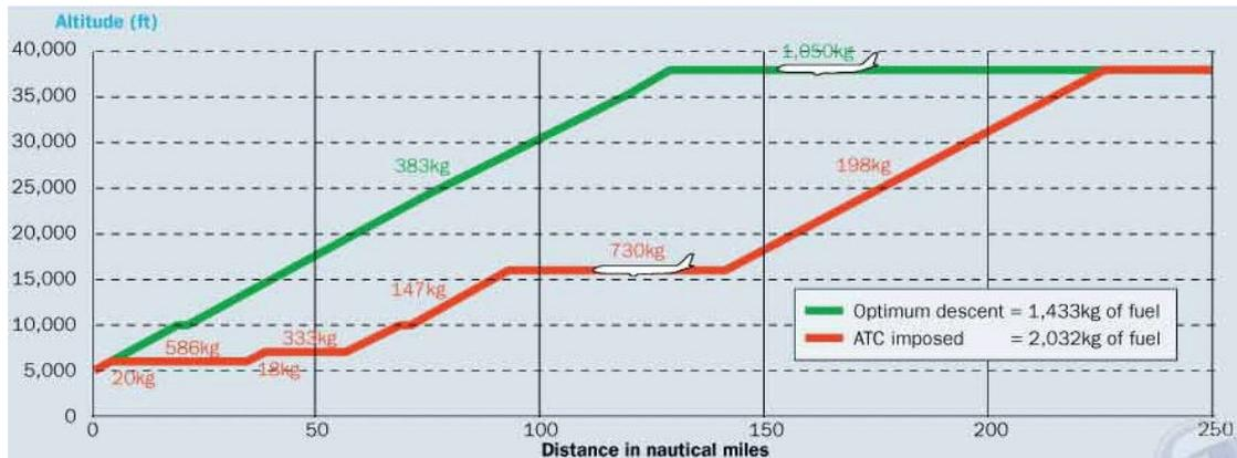
FIGURE E.1: Optimal vs. ATC imposed descent profiles for SAS flights into Newark using A330<sup>5</sup>
