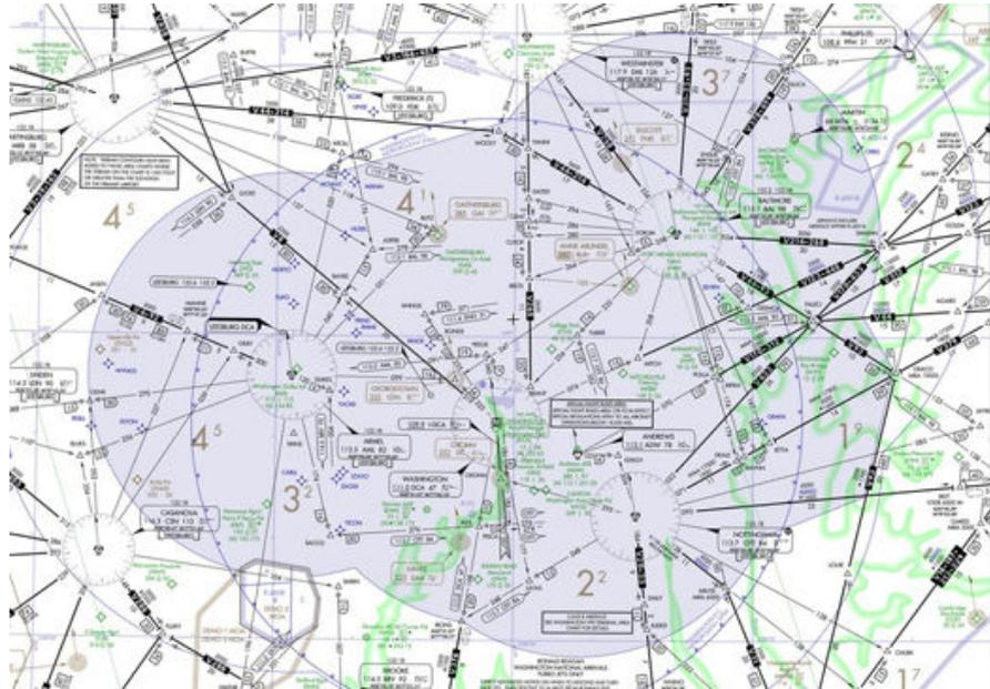
FIGURE H.2: Jet routes around Washington, DC, depicted on an aeronautical chart<sup>3</sup>
