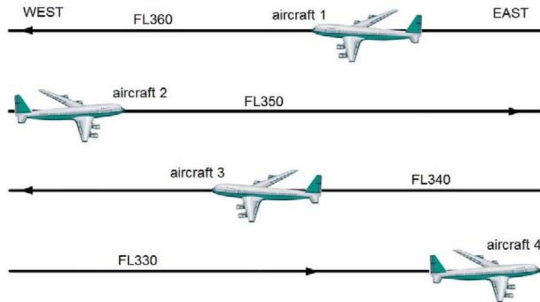
FIGURE 1.12: Vertical separation of aircraft by semi-circular rule
