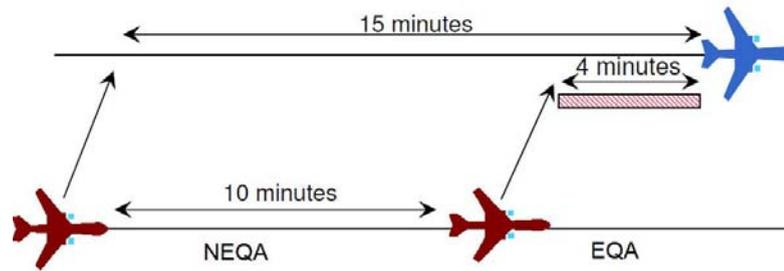
FIGURE 2.4: Separation standards for re-routing aircraft depending on their equipment<sup>11</sup>
