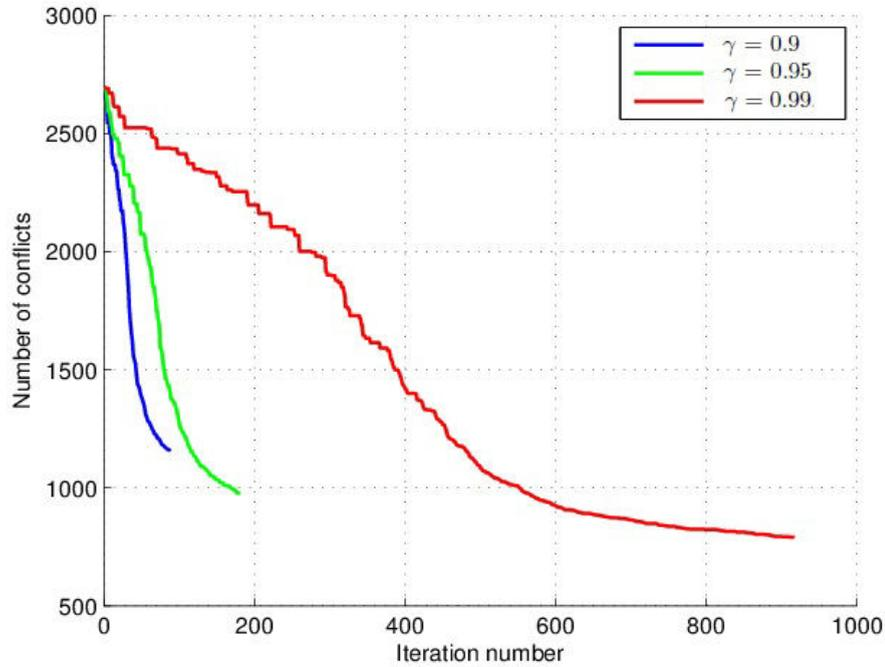
FIGURE 2.16: Simulated Annealing progress for a flight set with CSS
