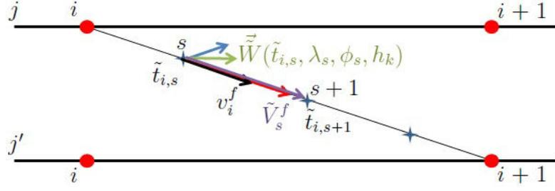
FIGURE 3.4: Estimation of flight between two waypoints
