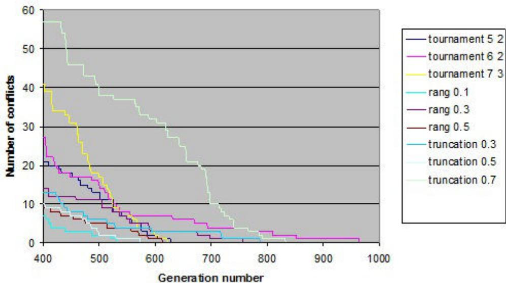
FIGURE Q.2: Convergence of GA with different selection methods in logarithmic scale
