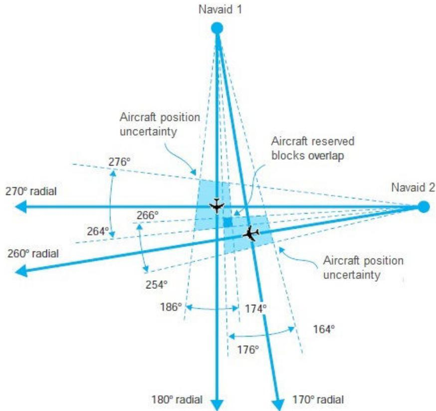
FIGURE 1.8: Separation of aircraft reserved blocks<sup>19</sup>
