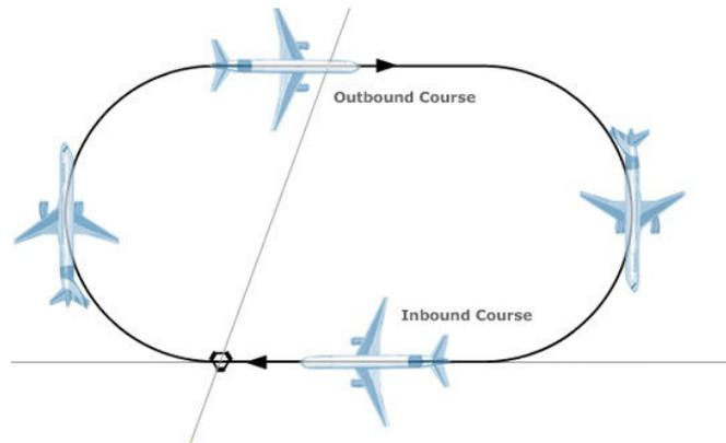
FIGURE K.3: A holding pattern<sup>3</sup>
