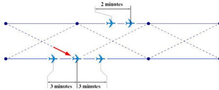
FIGURE 1.20: Reduced longitudinal separation standards in NAT (RSS)
