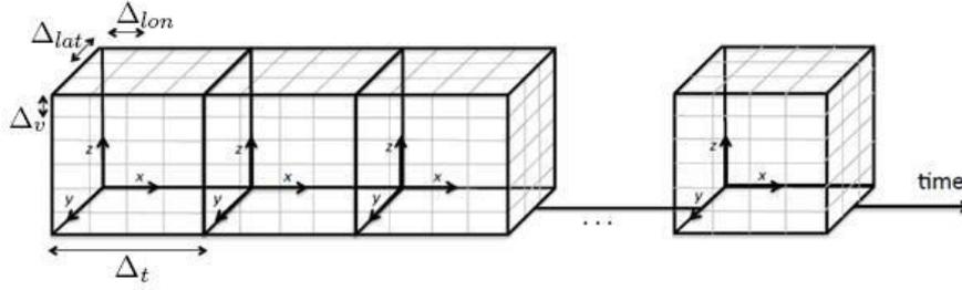
FIGURE 4.8: Four-dimensional grid for conflict detection <sup>3</sup>
