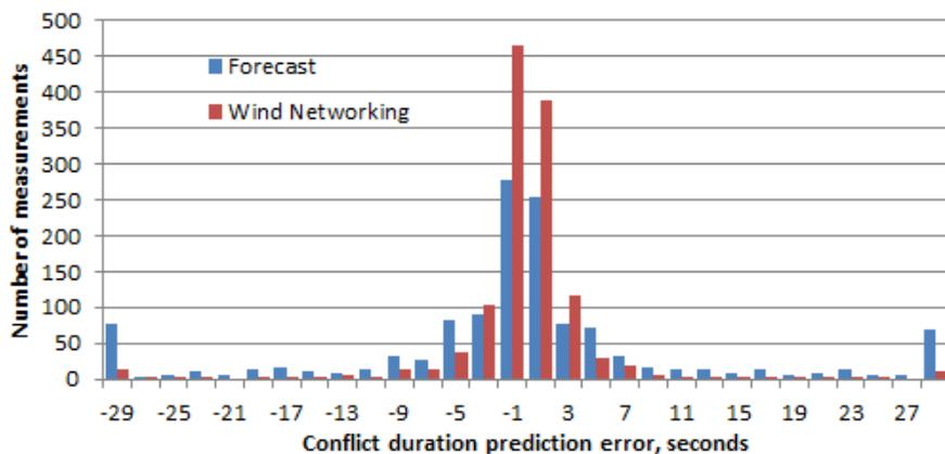
FIGURE 3.22: Distribution of the total conflict duration errors using MF and WN for 1,000 flights on the OTS
