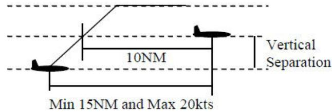
FIGURE 2.1: Longitudinal separation using ASAS ITC procedure<sup>2</sup>
