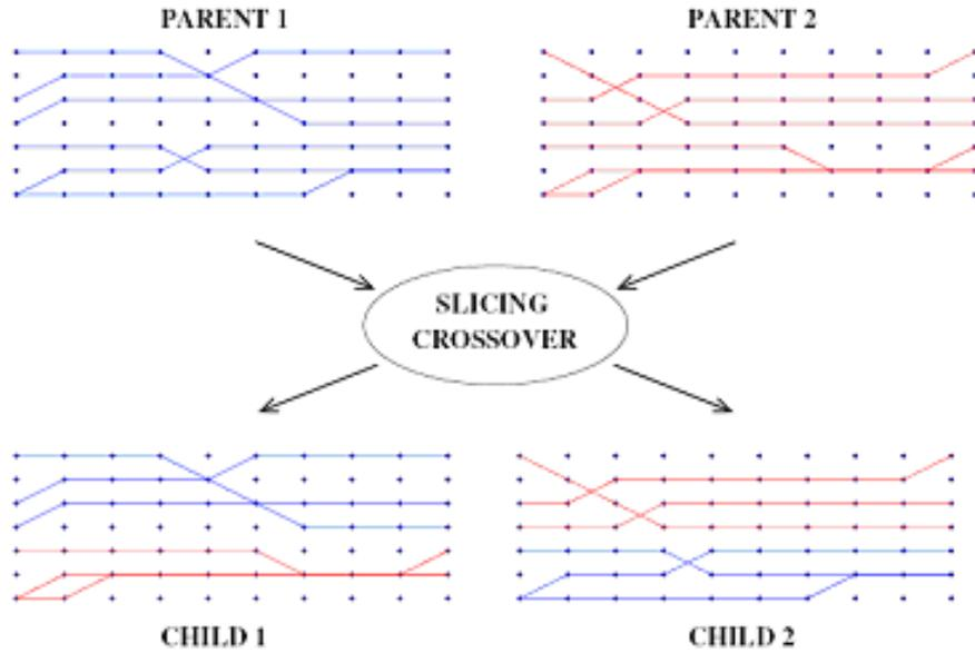
FIGURE 2.12: Crossover operator applied to two flight sets
