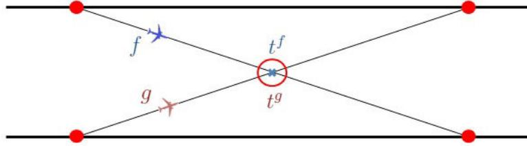
FIGURE 2.9: Conflict between two aircraft at a common node
