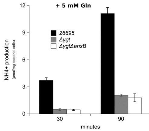
$\text{NH}_3$  production from 5 mM Gln by *H. pylori* 26695 parental strain or by isogenic mutants. Catalytic activity of  $\text{NH}_3$  production was measured after 30 and 90 minutes incubation at 37°C. Error bars represent the standard deviation obtained with at least three measurements.
