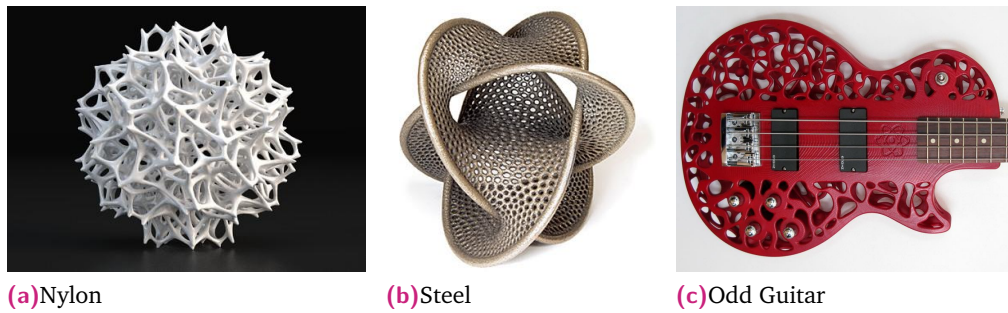
Fig. 4.1.: Some examples of 3Dprinted parts, which were until now impossible to produce. In addition, it can be done with a large range of material from wax to titanium.
