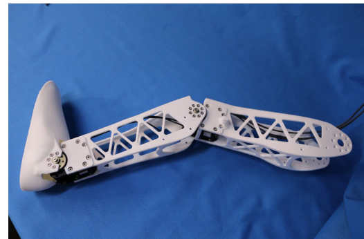
(b) Poppy's leg mechanical structure
