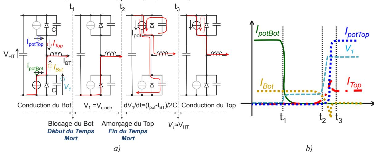
Figure 4.22 – Amorçage commandé
