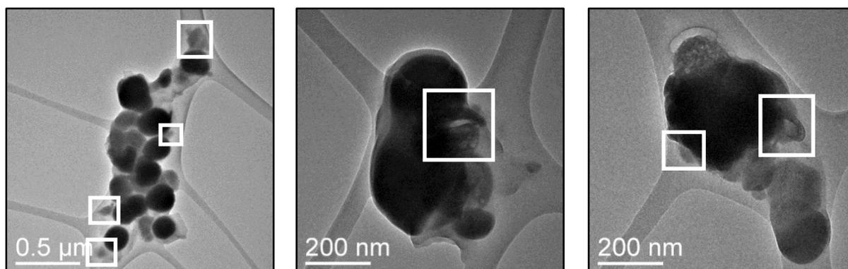
**Figure 4.13.** Damaged nanoparticles collected on the wear scar after HFRR testing in the presence of dispersants and S – Fe bonding to occur between the MoS<sub>2</sub> and the iron oxide of the surfaces.
