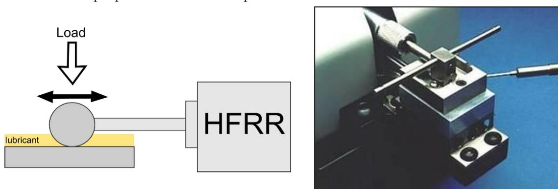
**Figure 2.2.** Schematic (left) and picture (right, *source PCS Instruments*) of the HFRR
