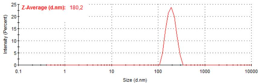
**Figure 4.15.** Nanoparticle agglomerate size distribution for the lubricant containing 0.05wt% of dispersants
