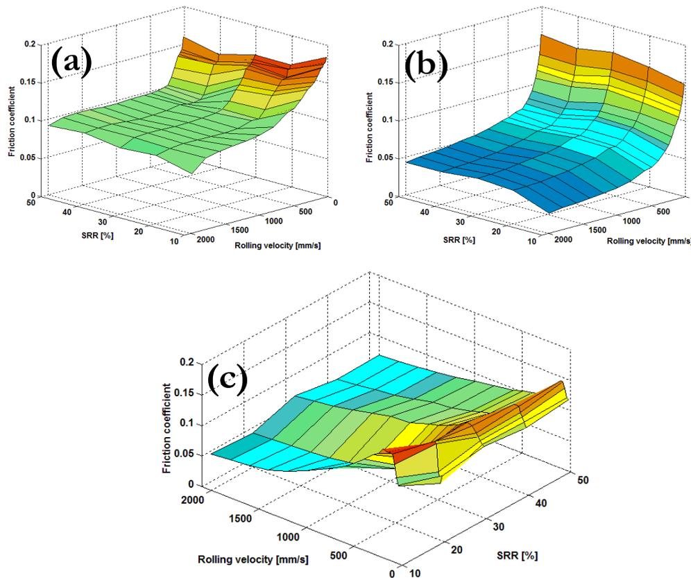
**Figure 5.13.** Mapping of the Stribeck curves depicting the influence of IF-MoS<sub>2</sub> in the presence of rough surfaces (a) PAO alone before running-in; (b) PAO alone after running-in; (c) PAO + IF-MoS<sub>2</sub> after running-in
