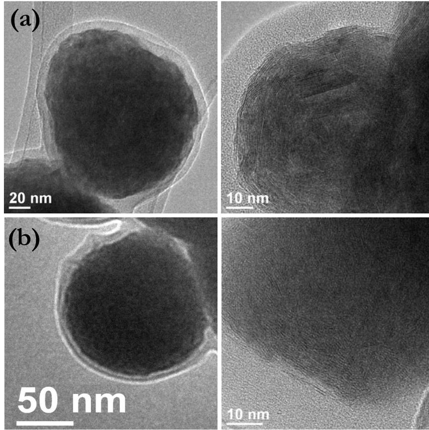
Figure 3.3. HR-TEM images of SC (a) and SpC (b) IF-MoS<sub>2</sub> nanoparticles
