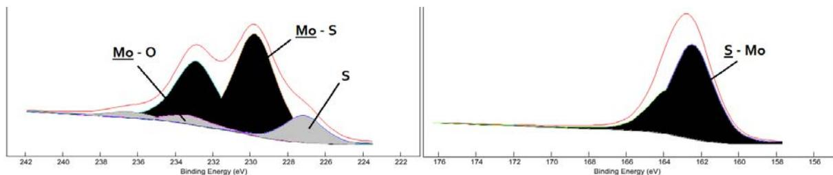
**Figure 3.31.** XPS spectra of molybdenum (right) and sulfur (left) of the bulk MoS<sub>2</sub> particles
