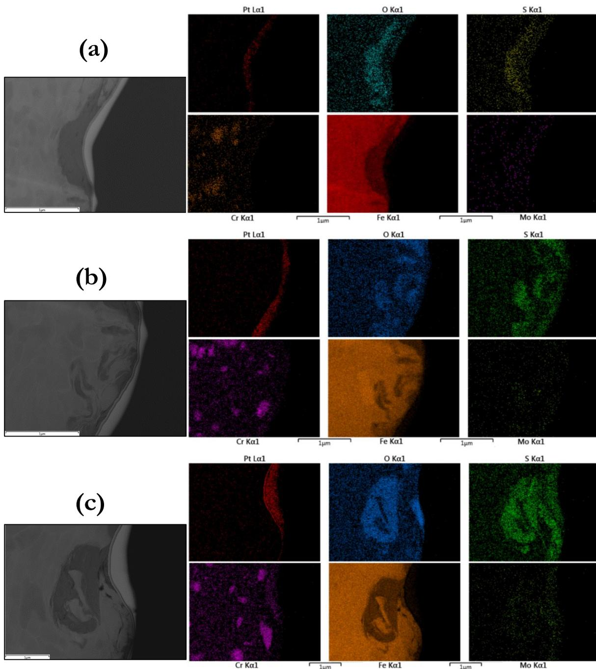
**Figure 3.29.** EDX maps of the main elements present on the FIB cross-section of the wear scar for the LC IF-MoS<sub>2</sub>
