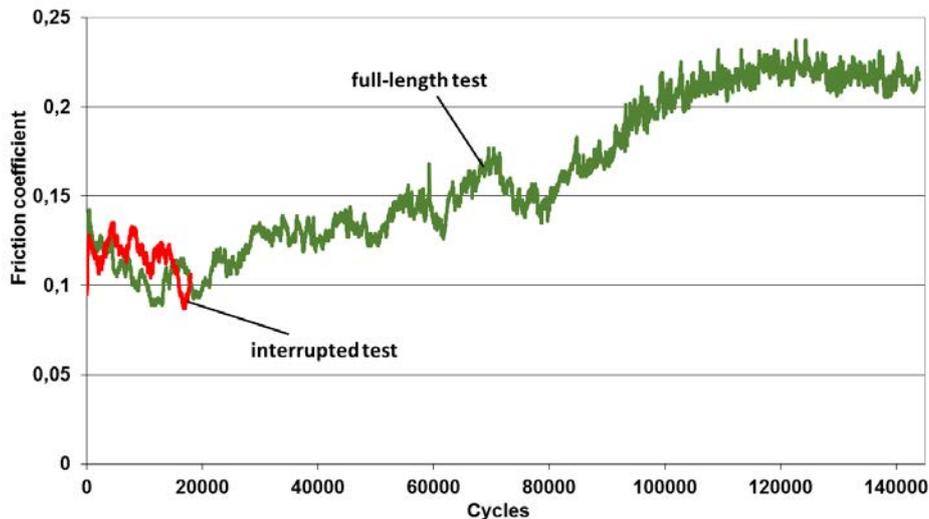
Figure 3.34. Full-length and interrupted test using 1wt% h-MoS<sub>2</sub> particles in order to compare the surfaces during and after testing
