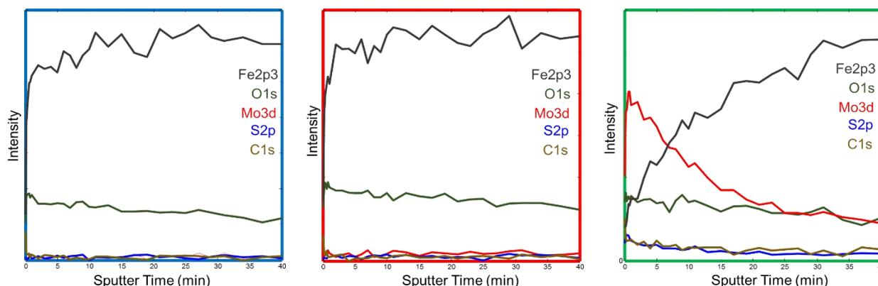
Figure 4.10. Ion etching profiles by XPS of the wear surfaces resulting from the test on Figure 4.7 PAO + dispersant (blue), PAO + dispersant + IF-MoS<sub>2</sub> (red), PAO + IF-MoS<sub>2</sub> (green)
