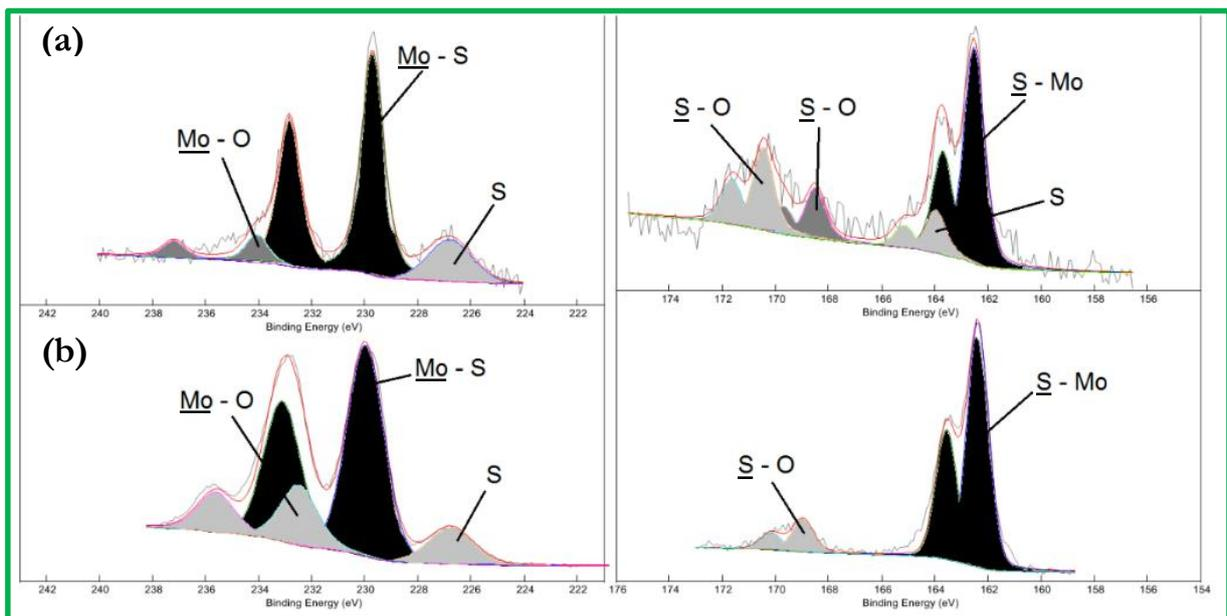
**Figure 3.19.** XPS spectra of molybdenum (left) and sulfur (right) for the SpC IF-MoS<sub>2</sub>
