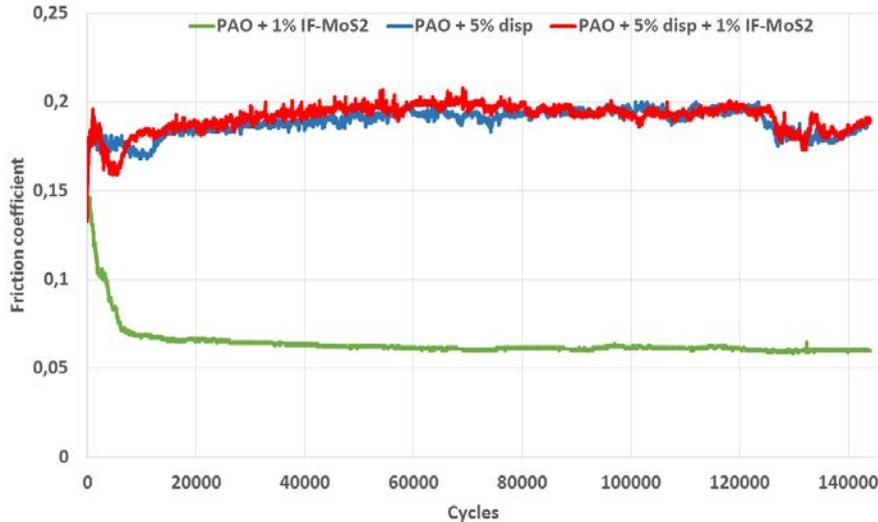
Figure 4.7. HFRR testing of the base oil containing IF-MoS<sub>2</sub> and/or dispersants
