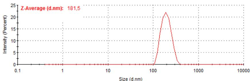
Figure 4.18. Nanoparticle agglomerate size distribution at the end of the tribological test (PAO base oil containing 1wt% IF-MoS<sub>2</sub> and 5wt% dispersants)
