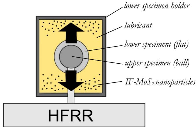
Figure 3.11. Top view of the HFRR set-up
