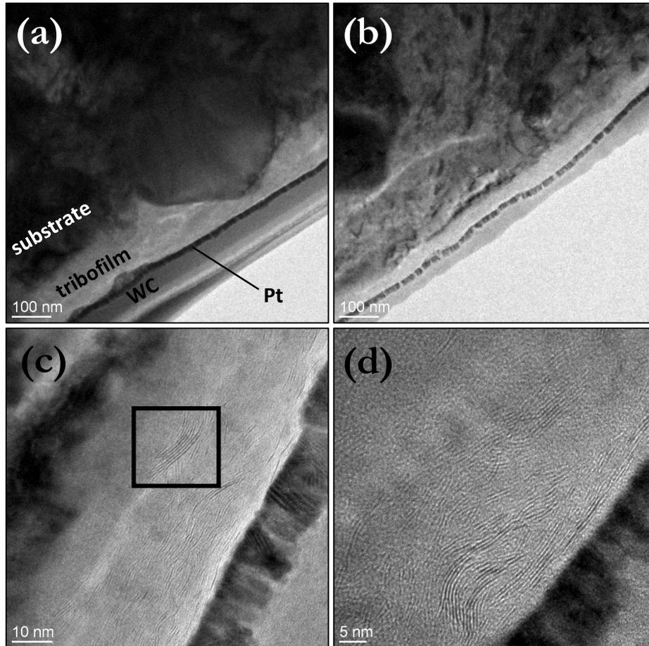
**Figure 3.25.** FIB cross-section of the wear scar at the end of the HFRR test for the PAO+1% SpC IF-MoS<sub>2</sub> blend
