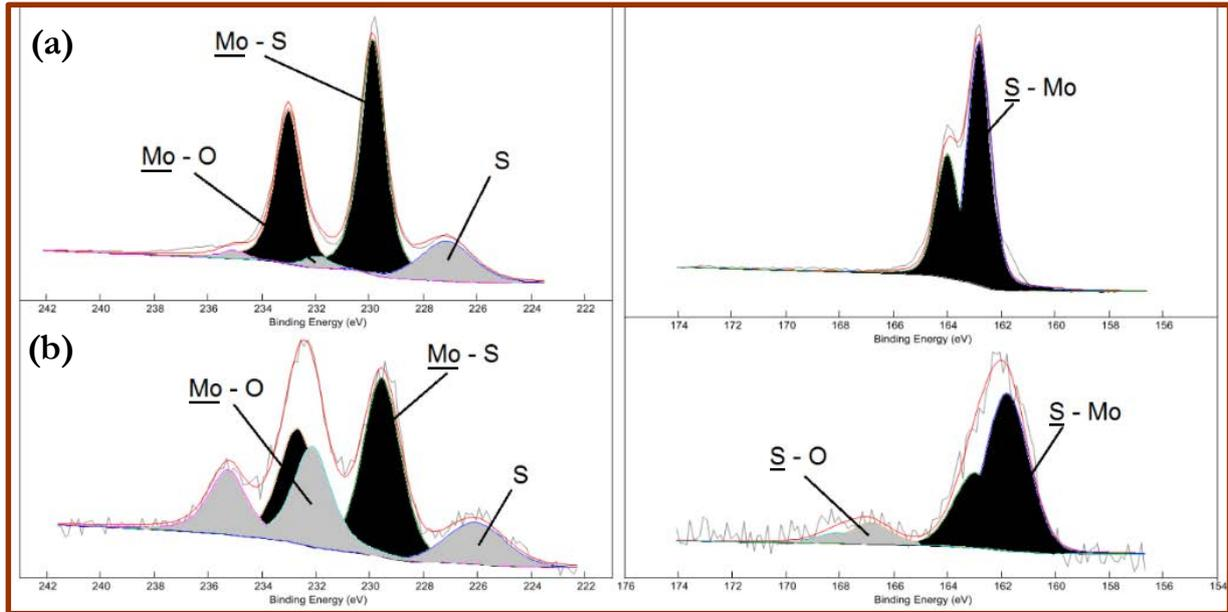
Figure 3.21. XPS spectra of molybdenum (left) and sulfur (right) for the SC IF-MoS<sub>2</sub>
