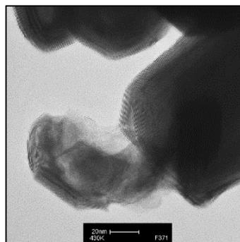
Figure 1.17. TEM observation of an IF-WS<sub>2</sub> nanoparticle after high-load tribological testing
