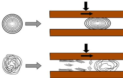
Figure 3.12. Facilitated exfoliation of poorly crystalline IF-MoS<sub>2</sub> under a given load and shear stress
