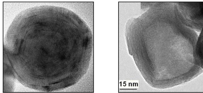
Figure 1.15. IF-TiS<sub>2</sub> synthesized by Margolin et al (left) and IF-WS<sub>2</sub> produced by Yang et al (right)
