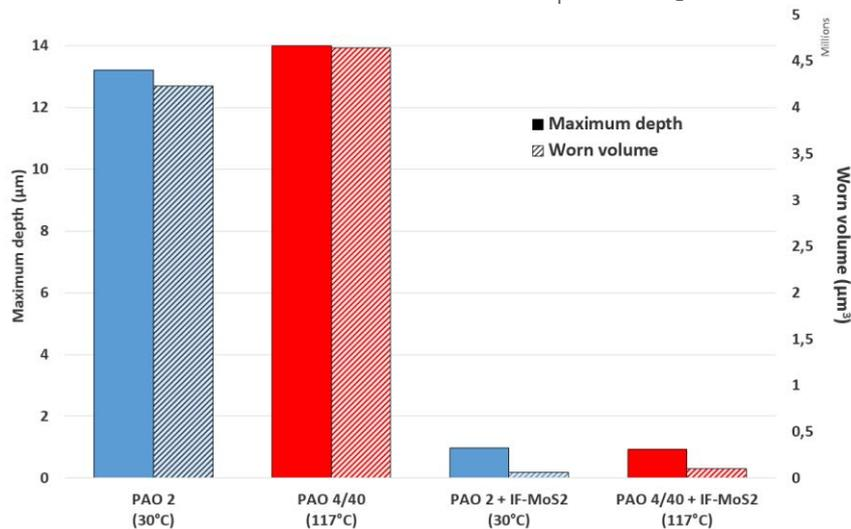
Figure 5.6. Maximum depth and worn volume of the wear scars after the HFRR tests shown on **Figure 5.5**
