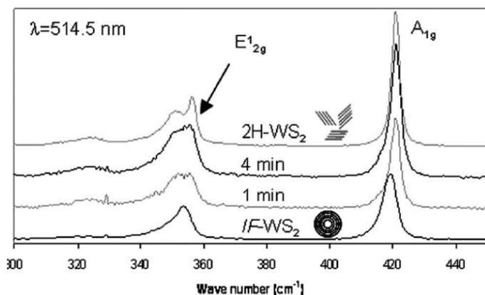
**Figure 1.21.** Progressive formation of 2H-WS<sub>2</sub> platelets from the exfoliation of IF-WS<sub>2</sub> nanoparticles observed using *in-situ* Raman analysis
