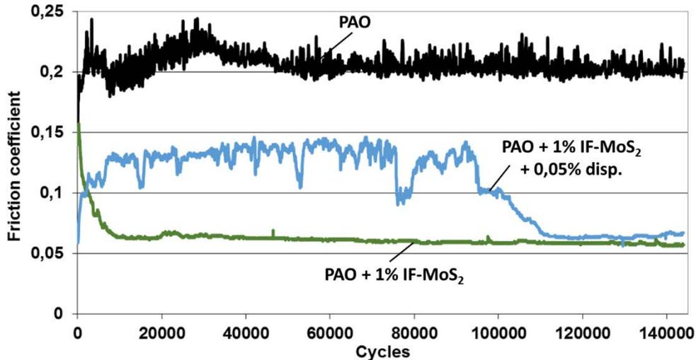
Figure 4.16. Tribological performance of the IF-MoS<sub>2</sub>-doped base oil containing 0.05 wt% of dispersants
