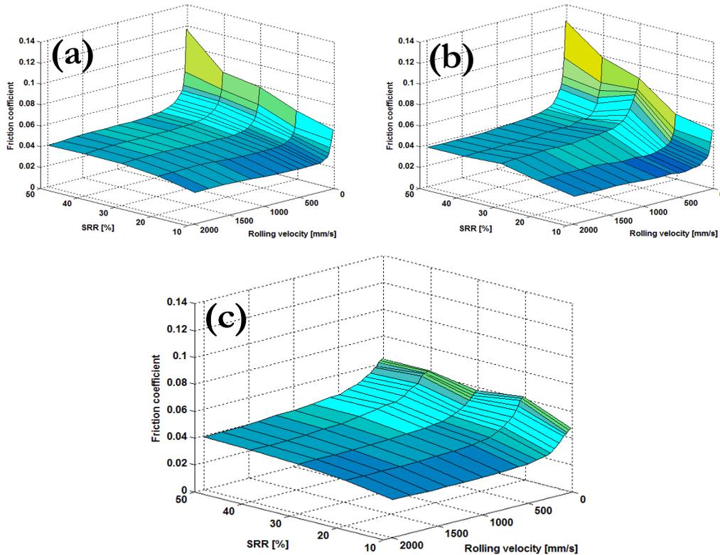
**Figure 5.8.** Mapping of the Stribeck curves depicting the influence of IF-MoS<sub>2</sub> on friction in mixed lubrication
