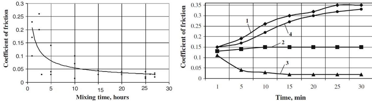
**Figure 1.22.** Influence of oil agitation before testing (left) and mechanical excitation of the contact (right) - 1. base oil with no excitation; 2. doped oil with no excitation; 3. doped oil with excitation and 4. base oil with excitation
