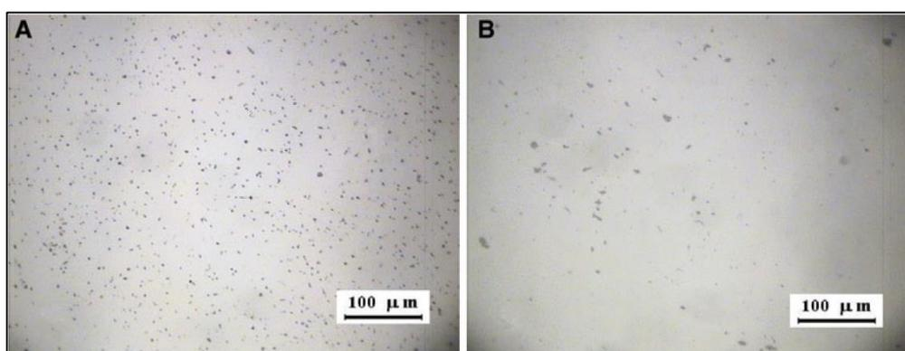
**Figure 1.27.** Sedimentation tests and resulting agglomeration state for rhenium doped IF-(Re)MoS<sub>2</sub> (left) and common IF-MoS<sub>2</sub> (right)
