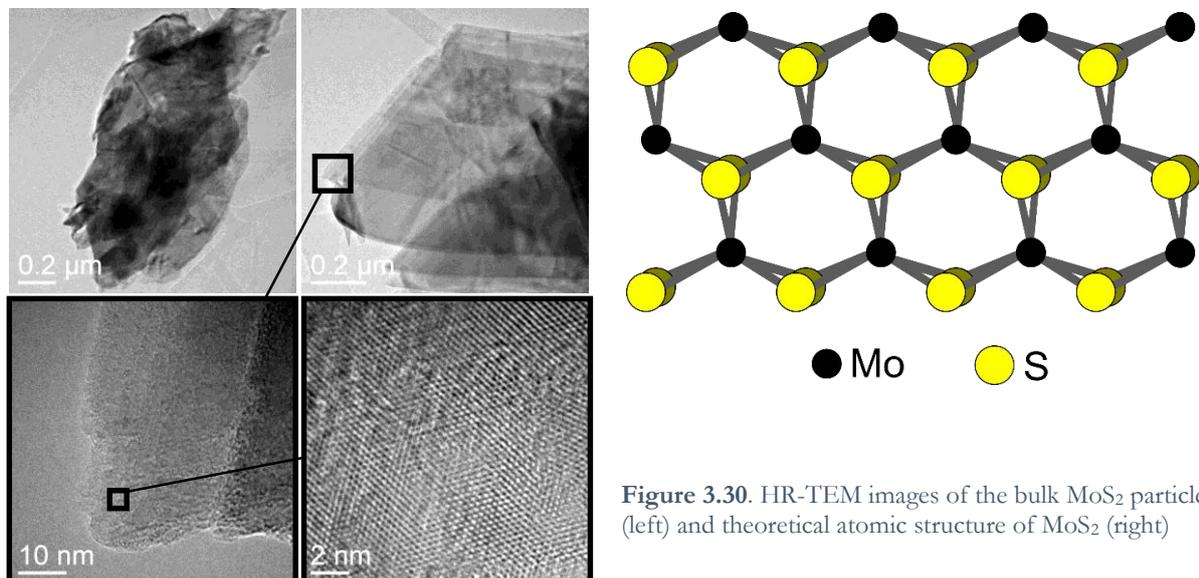
**Figure 3.30.** HR-TEM images of the bulk MoS<sub>2</sub> particles (left) and theoretical atomic structure of MoS<sub>2</sub> (right)
