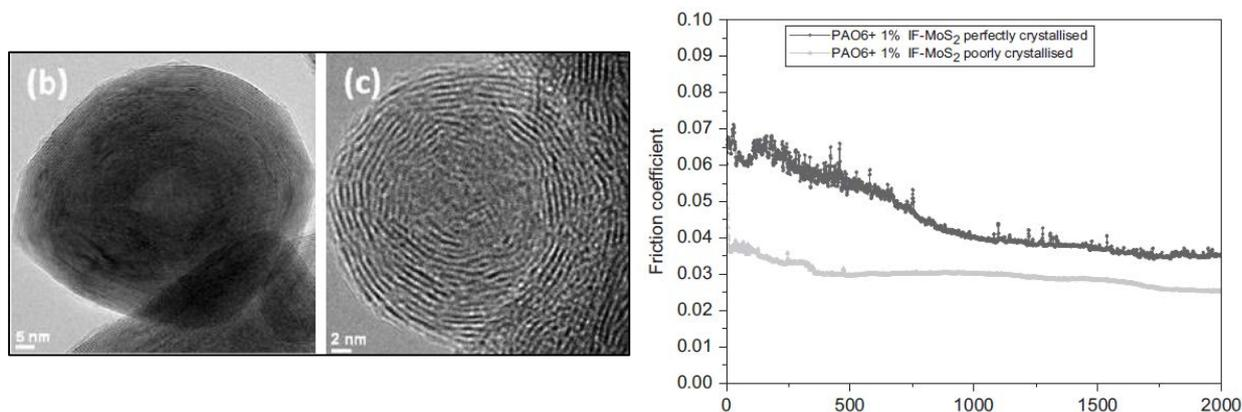
**Figure 1.26.** Crystalline (left) and poorly crystalline (center) IF-MoS<sub>2</sub> and associated tribological performances (right)
