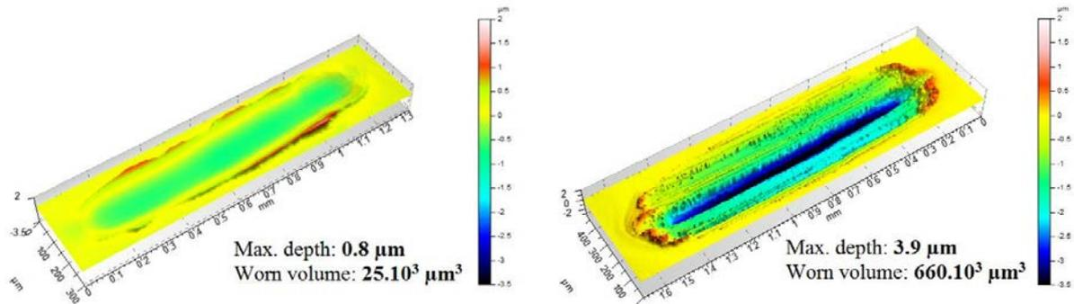
Figure 3.15. Wear scars corresponding to the 20 Hz HFRR test with 1wt% LC IF-MoS<sub>2</sub> after 17 minutes (left) and 4 hours (right)
