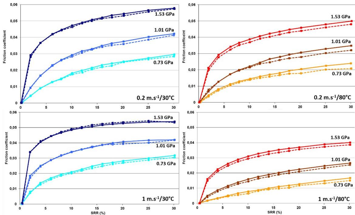
Figure 5.10. Traction curves in full-film lubrication conditions: PAO base oil (dotted lines) and PAO + IF-MoS<sub>2</sub> (full lines), tests at 30°C (blue, left) and 80°C (yellow/red, right), 0.2 m.s<sup>-1</sup> (top) and 2 m.s<sup>-1</sup> (bottom)
