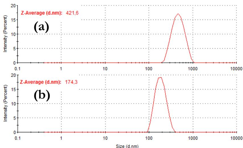
**Figure 4.6.** Nanoparticle agglomerate size distributions for the oils containing 1% IF-MoS<sub>2</sub> with (a) no dispersant and (b) with 5% dispersant
