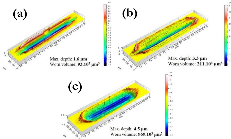
Figure 3.33. Wear scars after the HFRR testing of (a) LpC IF-MoS<sub>2</sub>, (b) LC IF-MoS<sub>2</sub> and (c) h-MoS<sub>2</sub>
