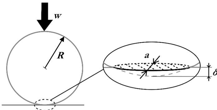
**Figure A.1.** Hertzian contact between a sphere and a flat surface
