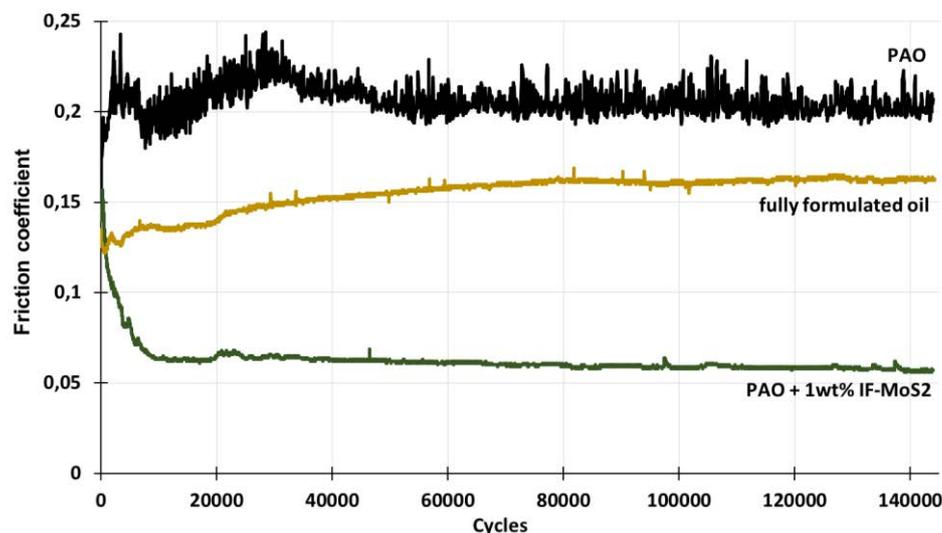
**Figure 4.3.** Compared performances of a PAO base oil with and without IF-MoS<sub>2</sub> and a fully formulated oil (test conditions given in **Table 3.3**)
