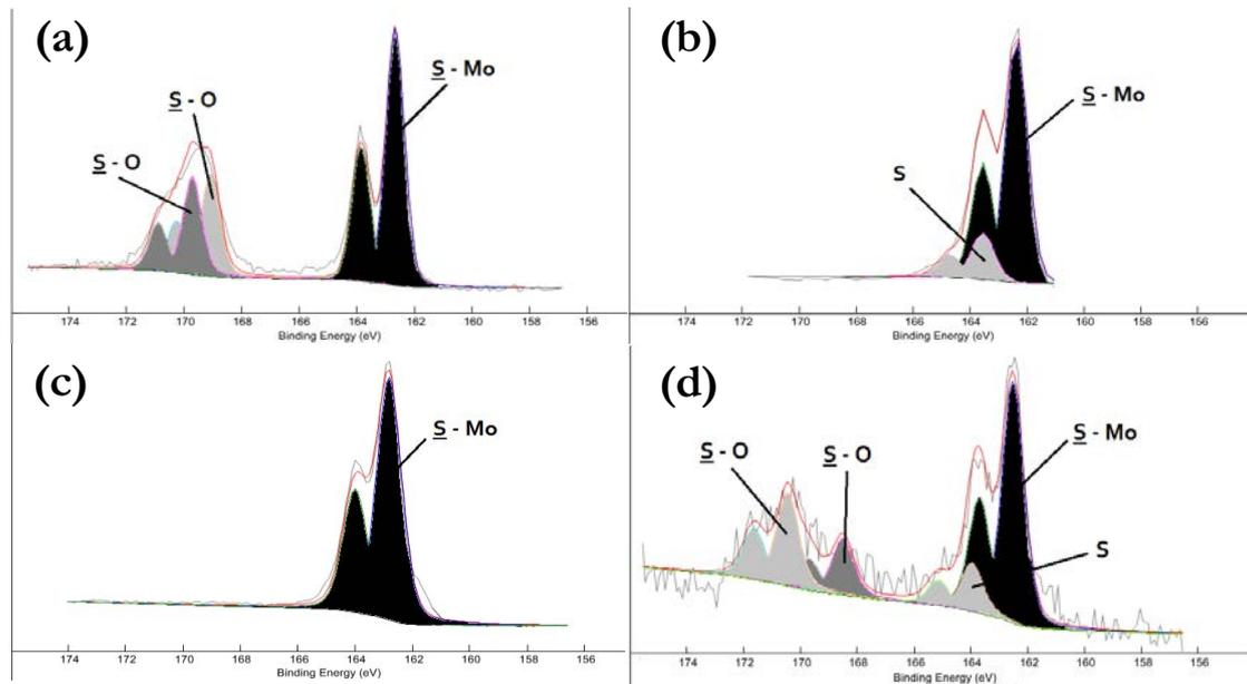
**Figure 3.5.** Sulfur 2p spectra measured by XPS for the (a) LC, (b) LpC, (c) SC and (d) SpC IF-MoS<sub>2</sub>
