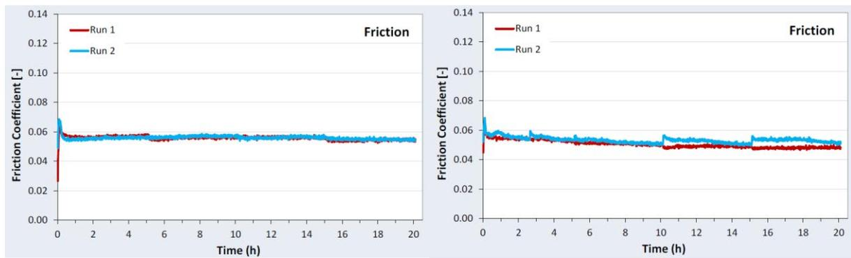
Figure C. 5. Repeatability of the friction measurements during the MPR tests for the PAO alone (left) and the PAO + 1wt% IF-MoS<sub>2</sub> (right)
