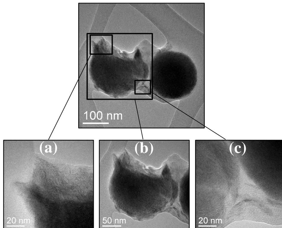
**Figure 4.12.** Nanoparticles collected after tribological testing in the presence of dispersants – damaged (left) and intact (right) IF-MoS<sub>2</sub>
