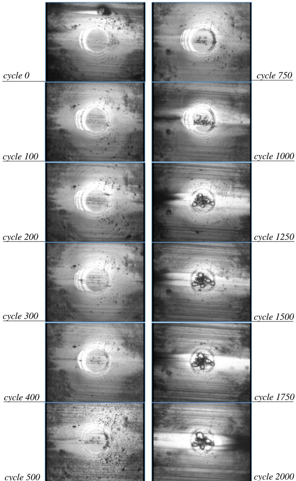
**Figure 4.17.** Nanovisus test for the PAO base oil containing 1wt% IF-MoS<sub>2</sub> and 0.05wt% dispersants
