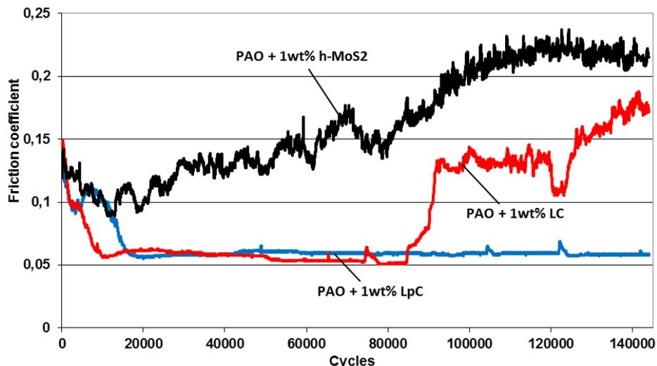
**Figure 3.32.** Comparison of the friction reducing properties of h-MoS<sub>2</sub> particles and IF-MoS<sub>2</sub> nanoparticles
