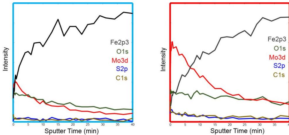
**Figure 5.4.** Ion etching profiles by XPS of the wear surfaces resulting from the testing of the PAO + 1wt% SpC IF-MoS<sub>2</sub> at 30°C (left) and 80°C (right)
