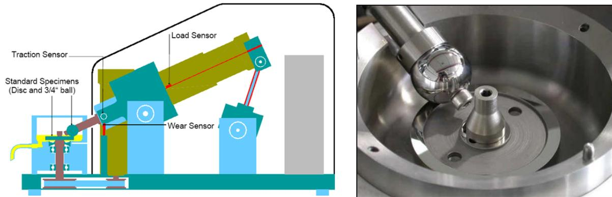
Figure 2.3. Schematic (left) and picture (right) of the MTM (source: PCS Instruments)
