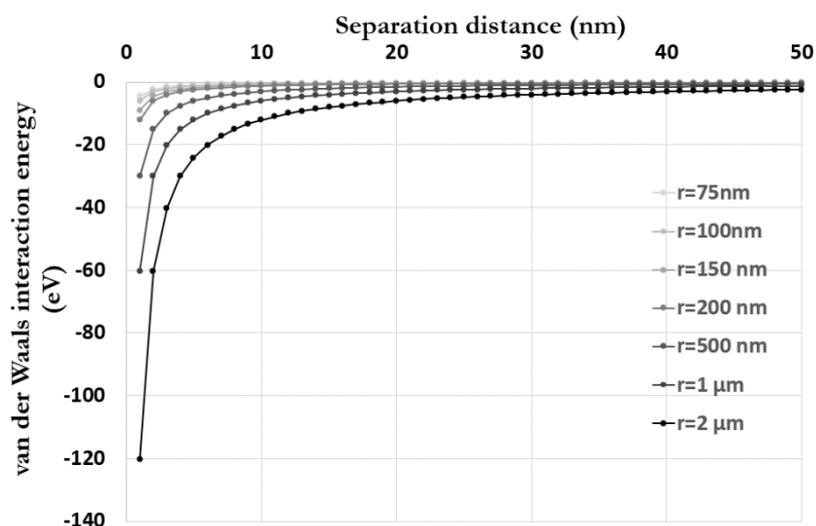
Figure 4.2. Van der Waals interaction energies for IF-MoS<sub>2</sub> of different sizes
