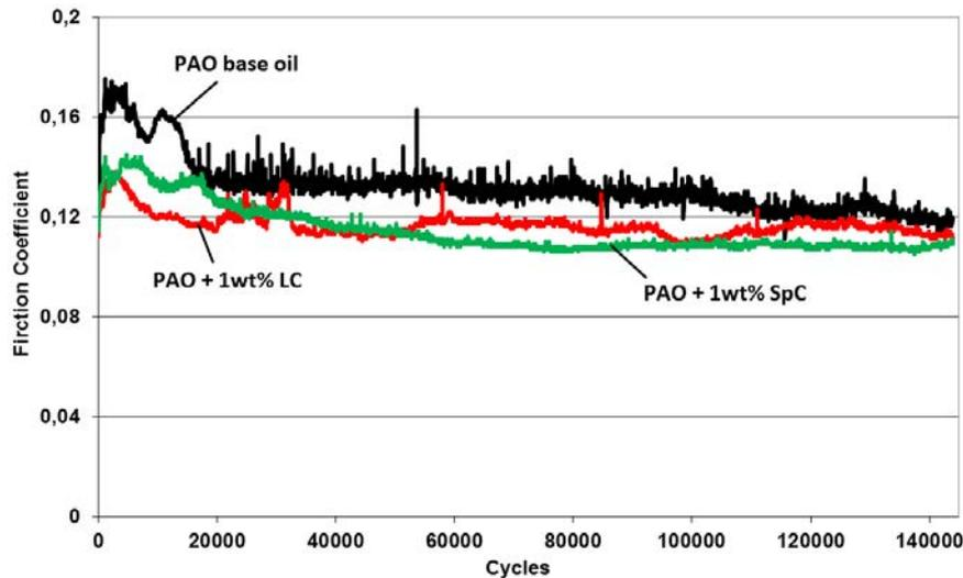
Figure 5.1. HFRR testing of the LC and SpC IF-MoS<sub>2</sub> under ambient temperature
