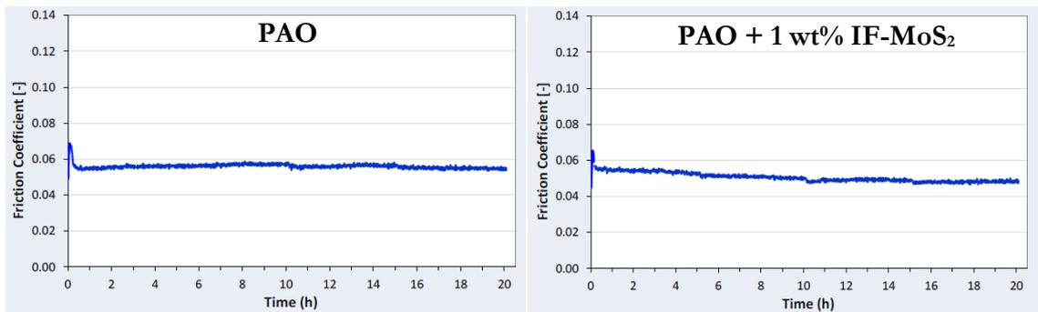
**Figure 5.16.** Evolution of the friction coefficients during the MPR testing of the PAO base oil alone (left) and the PAO containing 1 wt% IF-MoS<sub>2</sub> (right)
