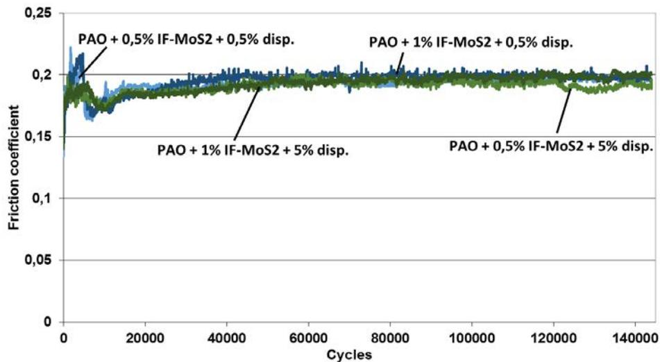
Figure 4.5. Tribological testing of a PAO base oil containing various concentrations of IF-MoS<sub>2</sub> and dispersants
