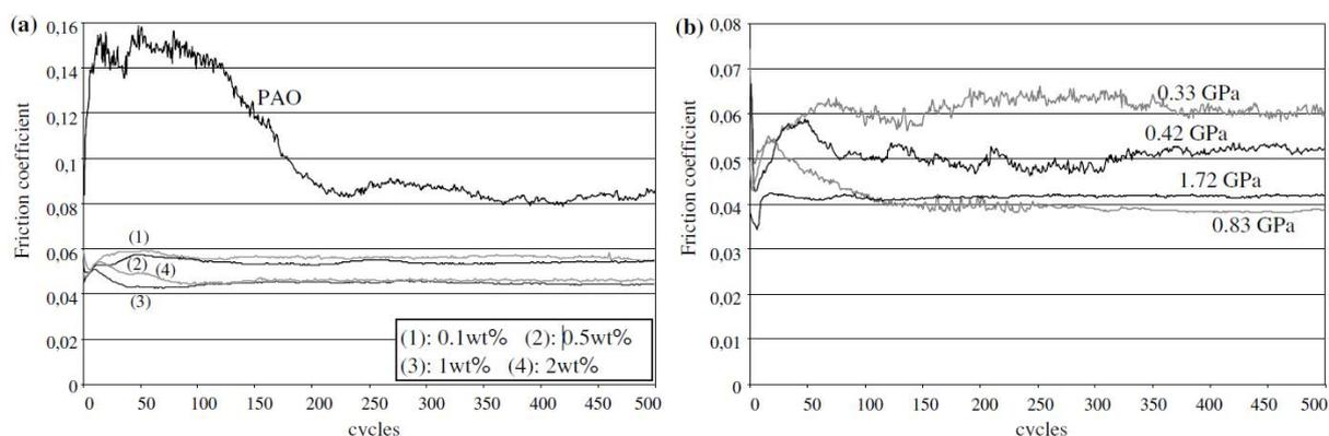
**Figure 1.18.** Friction reduction for different IF-WS<sub>2</sub> concentrations (left, 1.12 GPa) and contact pressures (right, 1wt%)
