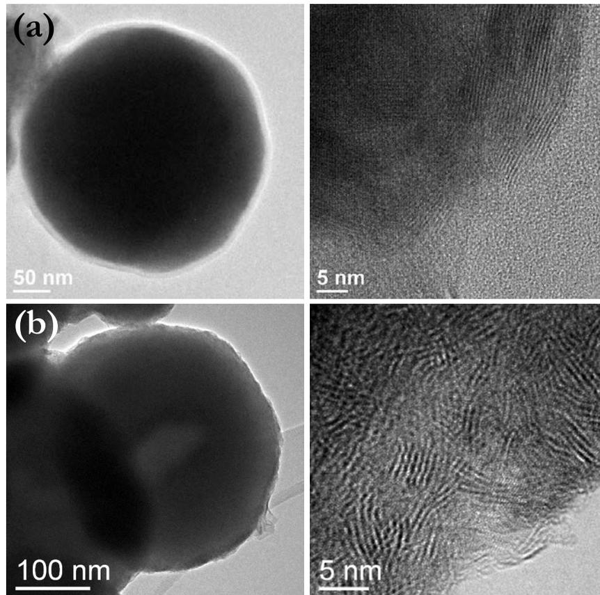
**Figure 3.2.** HR-TEM images of LC (a) and LpC (b) IF-MoS<sub>2</sub> nanoparticles
