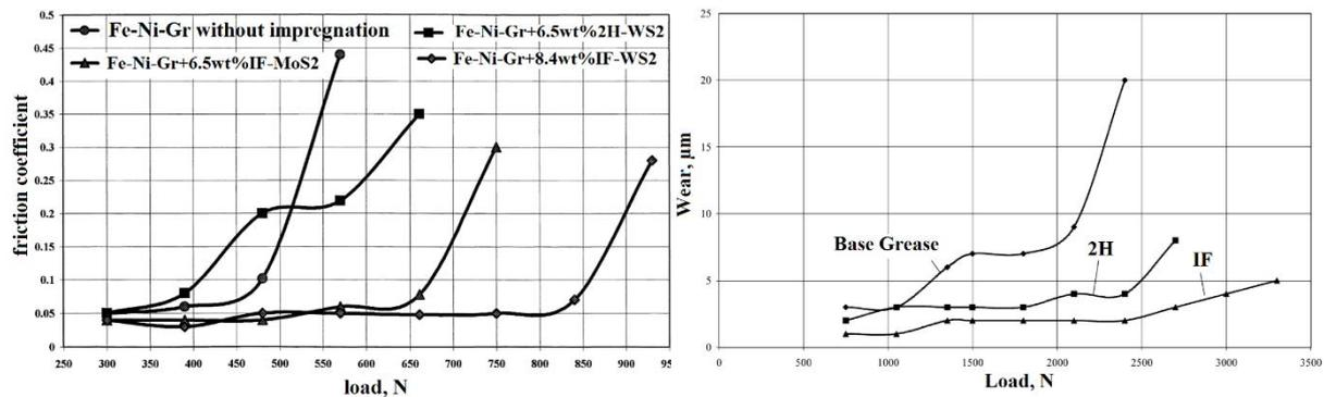
Figure 1.16. Friction and wear reductions observed for the contact between two porous materials in the case of "classical" (2H-WS<sub>2</sub>) and nanoparticle (IF-WS<sub>2</sub>) lubrication
