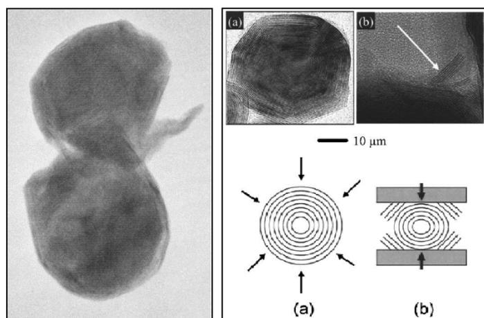
**Figure 1.19.** IF-WS<sub>2</sub> exfoliation as observed by Leshchinsky et al (left) and Joly-Pottuz et al (top right), and schematized behavior of fullerene-like nanoparticles under hydrostatic (a) and uni-axial (b) pressures
