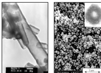
**Figure 1.11.** Hollow nanotubes and nanospheres synthesized in [30] and [31]
