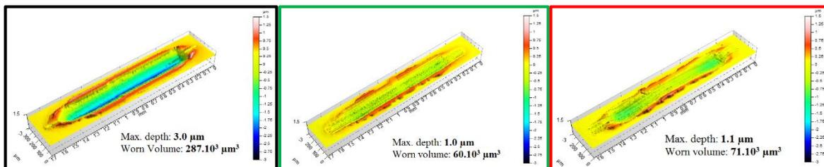
Figure 5.2. Comparison of the wear scars obtained for the PAO base oil alone (left), the PAO+1wt% SpC IF-MoS<sub>2</sub> (center) and the PAO+1wt% LC IF-MoS<sub>2</sub> (right)
