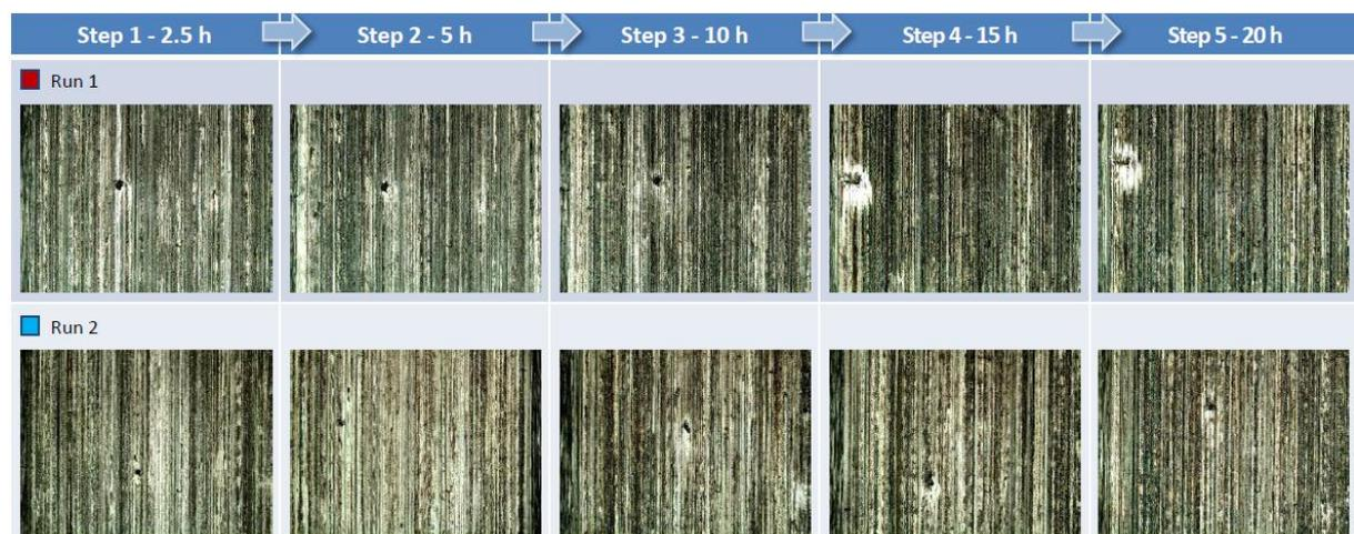
Figure C. 7. Evolution of the contact surface during both MPR runs on the PAO + 1wt% IF-MoS<sub>2</sub>
