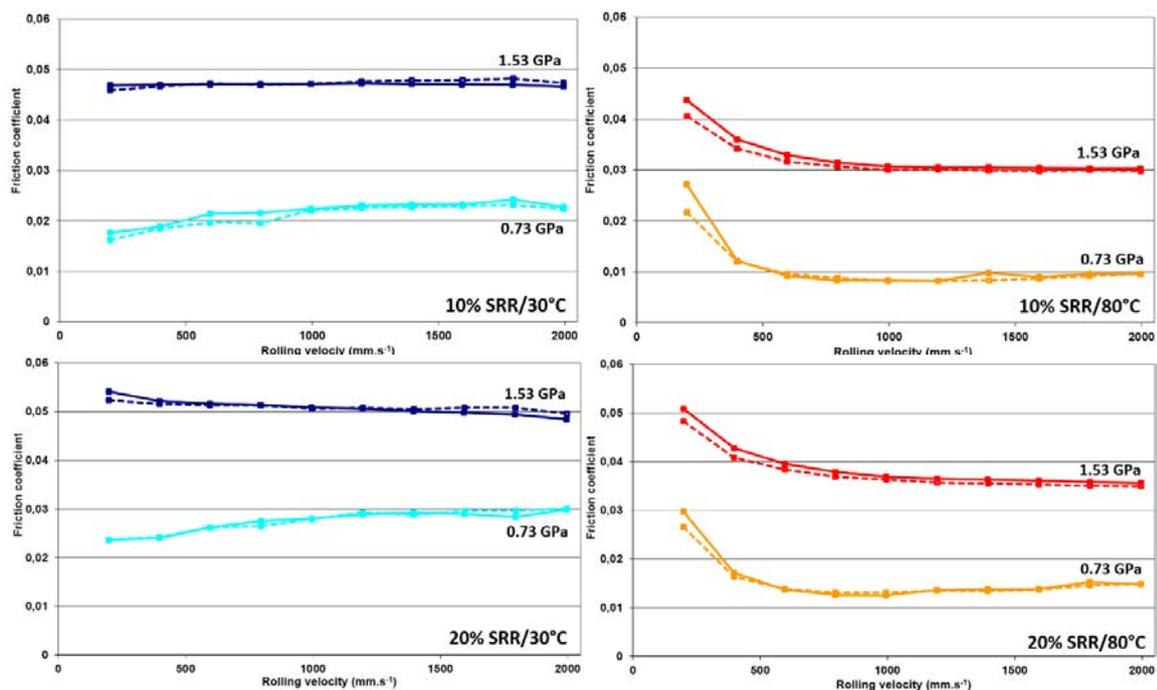
Figure 5.11. Stribeck curves in full-film lubrication conditions: PAO base oil (dotted lines) and PAO + IF-MoS<sub>2</sub> (full lines), tests at 30°C (blue, left) and 80°C (yellow/red, right), 10% SRR (top) and 20% SRR (bottom)
