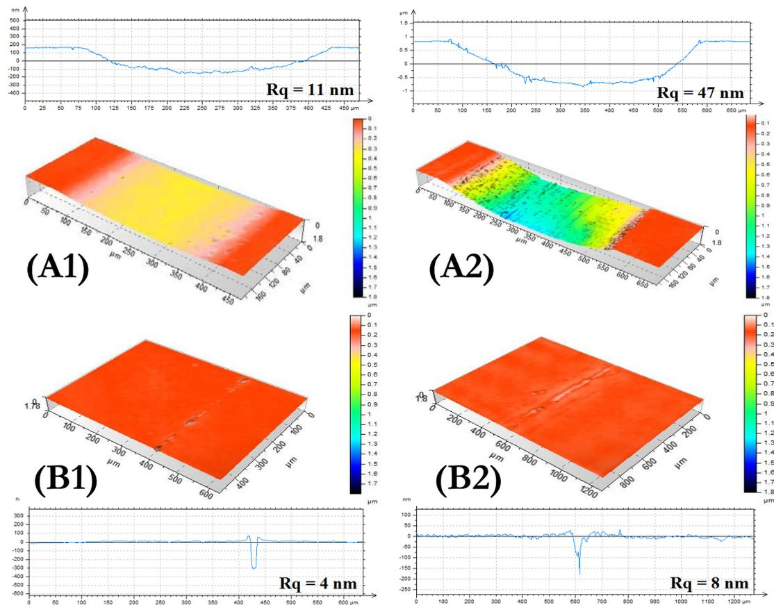
Figure 5.9. Typical surface topographies and profiles obtained at 10% (1) and 50% (2) SRR for the PAO alone (A) and the PAO + IF-MoS<sub>2</sub> (B). Rq values were determined taking into account only the wear scar.
