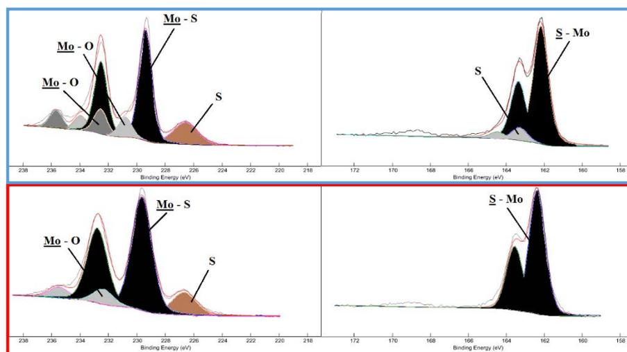
**Figure 5.7.** Mo 3d (left) and S 2p (right) spectra measured on the wear scars of the PAO2+IF-MoS<sub>2</sub> test carried out at 30°C (top) and the PAO4/40+IF-MoS<sub>2</sub> test carried out at 117°C (bottom)
