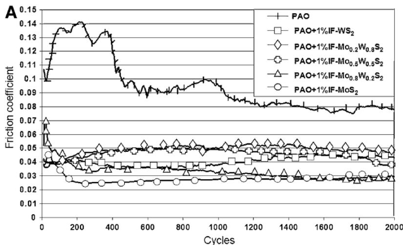
**Figure 1.23.** Friction coefficients for IF-Mo<sub>x</sub>W<sub>(1-x)</sub>S<sub>2</sub> nanoparticles of varying stoichiometry (contact pressure of 1.12 GPa)
