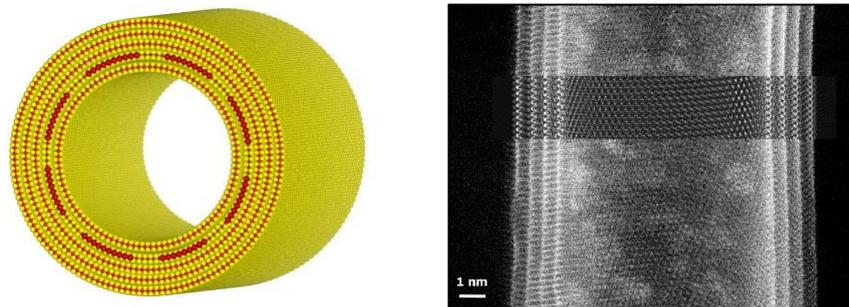
**Figure 1.24.** Numerical model (left) and HR-TEM observation (right) of a multi-wall WS<sub>2</sub> nanotube
