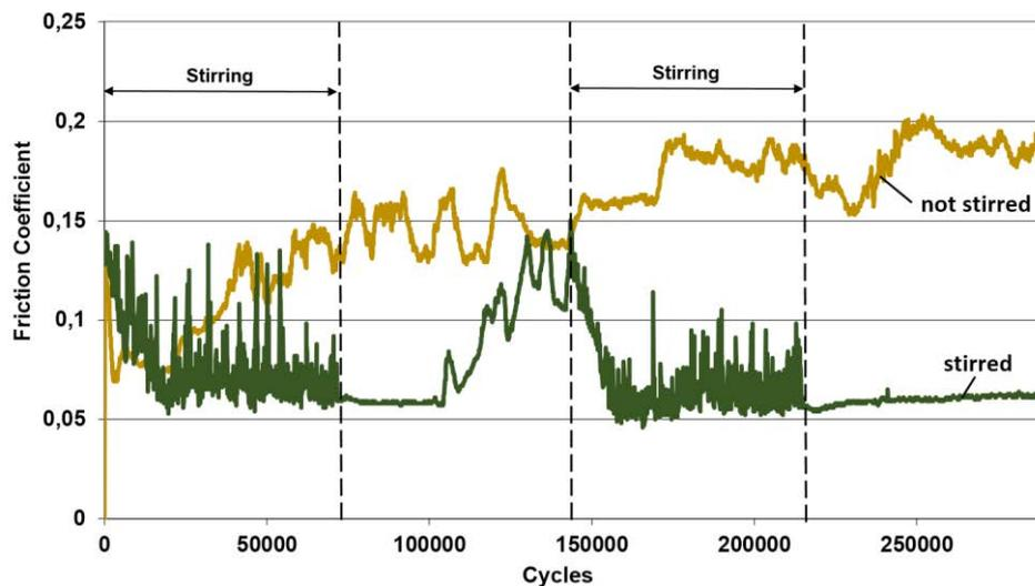
Figure 3.17. Performance of LC-type IF-MoS<sub>2</sub> enhanced by modifying the oil flow around the contact
