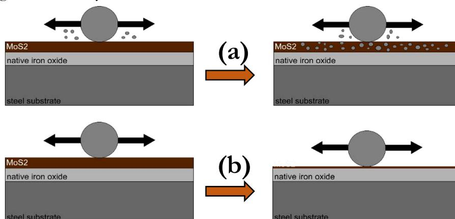
**Figure 3.23.** Possible scenarios for the loss of tribological performance of the more crystalline IF-MoS<sub>2</sub> and the presence of higher quantities of iron sulfides at the surface of the corresponding wear scars
