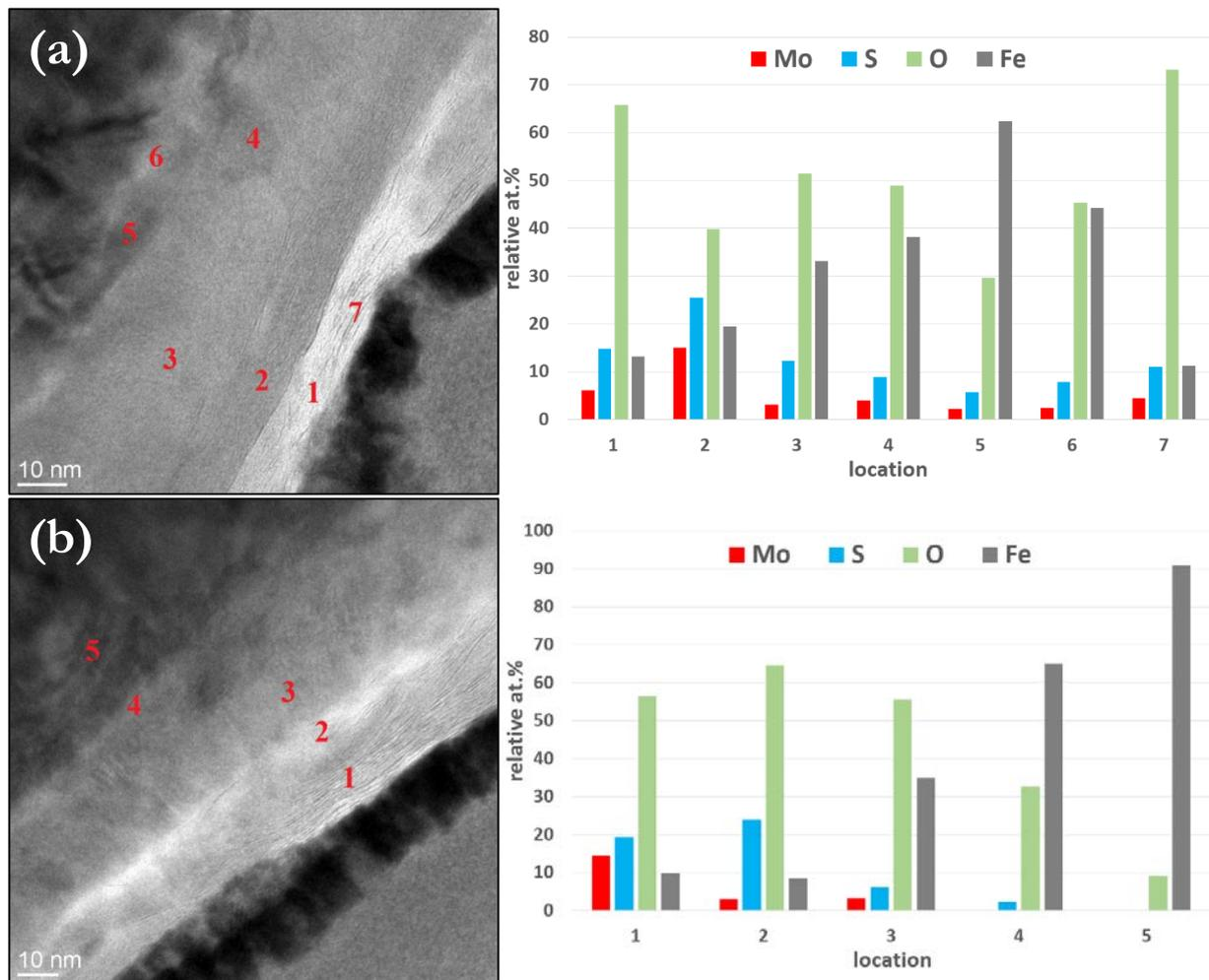
Figure 3.26. EDX analyses at different locations of the wear surface for the SpC IF-MoS<sub>2</sub>
