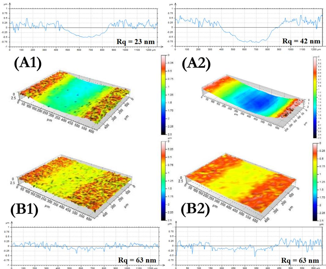
**Figure 5.14.** Typical surface topographies and profiles obtained at 10% (1) and 50% (2) SRR for the PAO alone (A) and the PAO + IF-MoS<sub>2</sub> (B).  $R_q$  values were determined taking into account only the wear scar.
