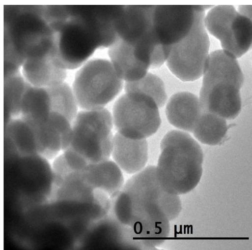
**Figure 3.1.** Typical size distribution of the nanoparticles (SC IF-MoS<sub>2</sub> shown here)
