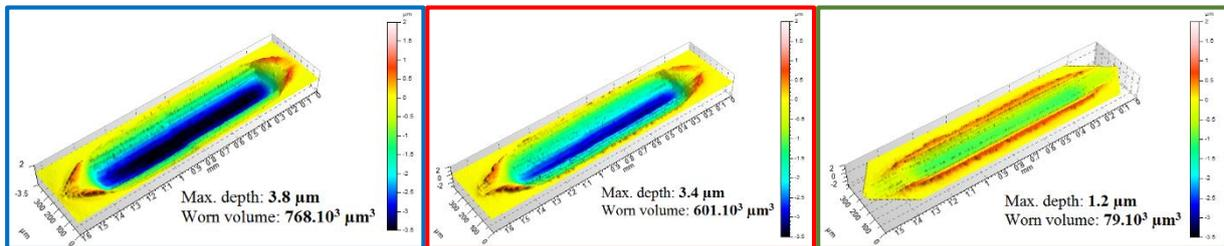
Figure 4.8. Wear scars for the HFRR tests showed on Figure 4.7: PAO + 5% disp. (left), PAO + 5% disp. + 1% IF-MoS<sub>2</sub> (center) and PAO + 1% IF-MoS<sub>2</sub> (right)
