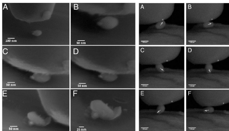
**Figure 1.20.** Exfoliation (left) and rolling/sliding (right) of an IF-WS<sub>2</sub> nanoparticle in a HR SEM
