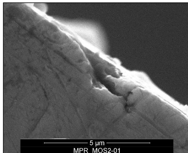
Figure 5.20. Cross-section of the roller tested with the PAO + 1 wt% IF-MoS<sub>2</sub>
