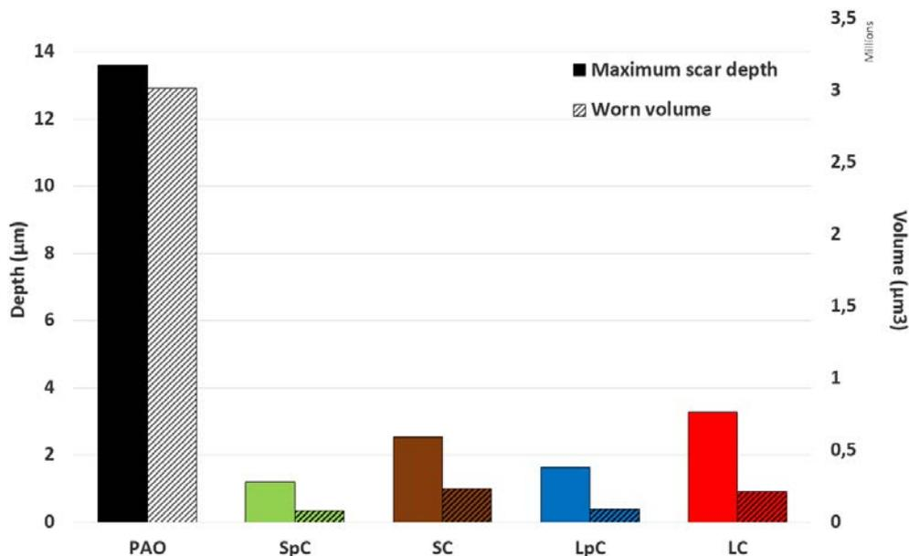
Figure 3.10. Maximum depths and wear volumes of the scars obtained for the different types of IF-MoS<sub>2</sub>
