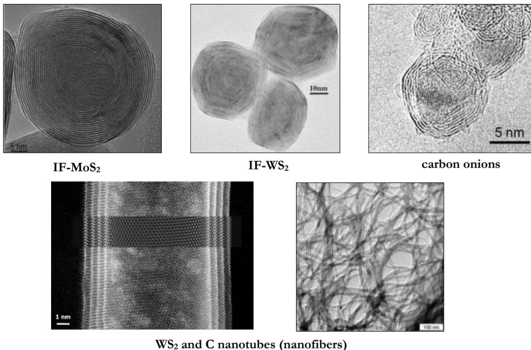
**Figure 1.7.** Examples of existing types of nanoparticles [10,23,51,56,64]
