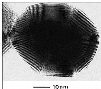
**Figure 1.14.** IF-WS<sub>2</sub> studied in [35]: closed nanoparticles with many concentric layers
