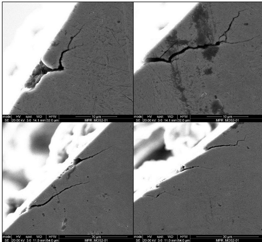
Figure 5.21. Cross-sections of the roller tested with the PAO base oil
