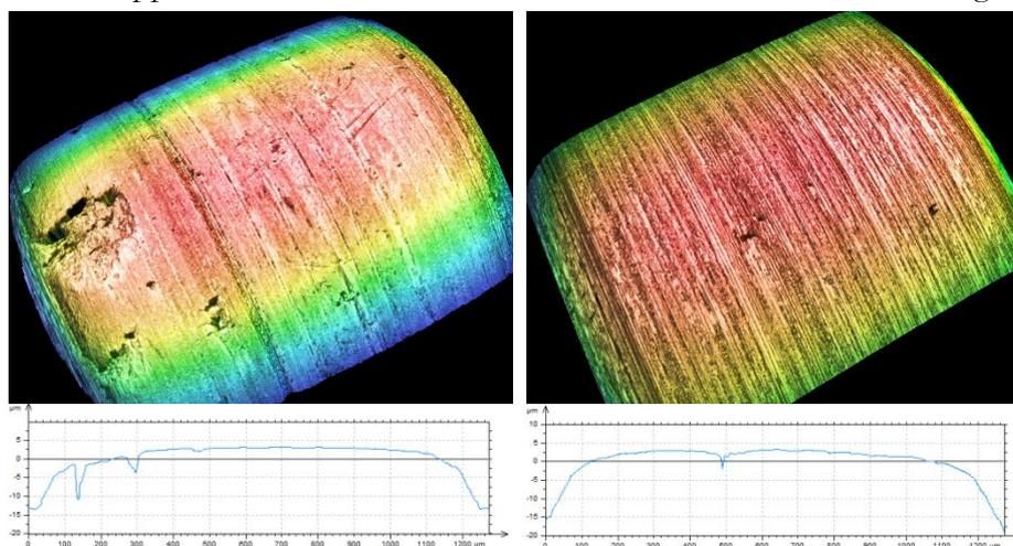
**Figure 5.17.** 3D topographies and profiles of the surfaces resulting from the MPR testing of the PAO (left) and PAO + 1 wt% IF-MoS<sub>2</sub> (right)
