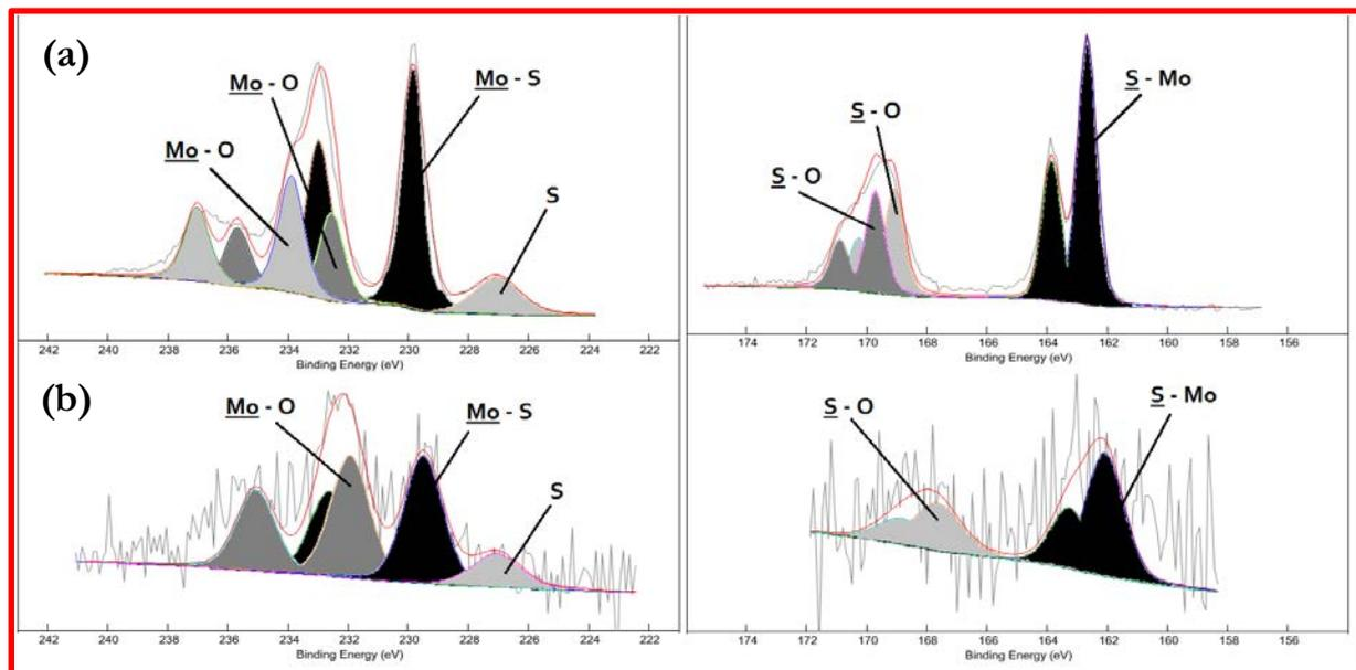
Figure 3.22. XPS spectra of molybdenum (left) and sulfur (right) for the LC IF-MoS<sub>2</sub>
