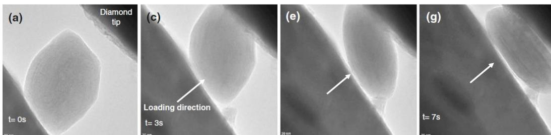
**Figure 1.29.** Compression of an individual IF-MoS<sub>2</sub> during *in-situ* HR-TEM experiments
