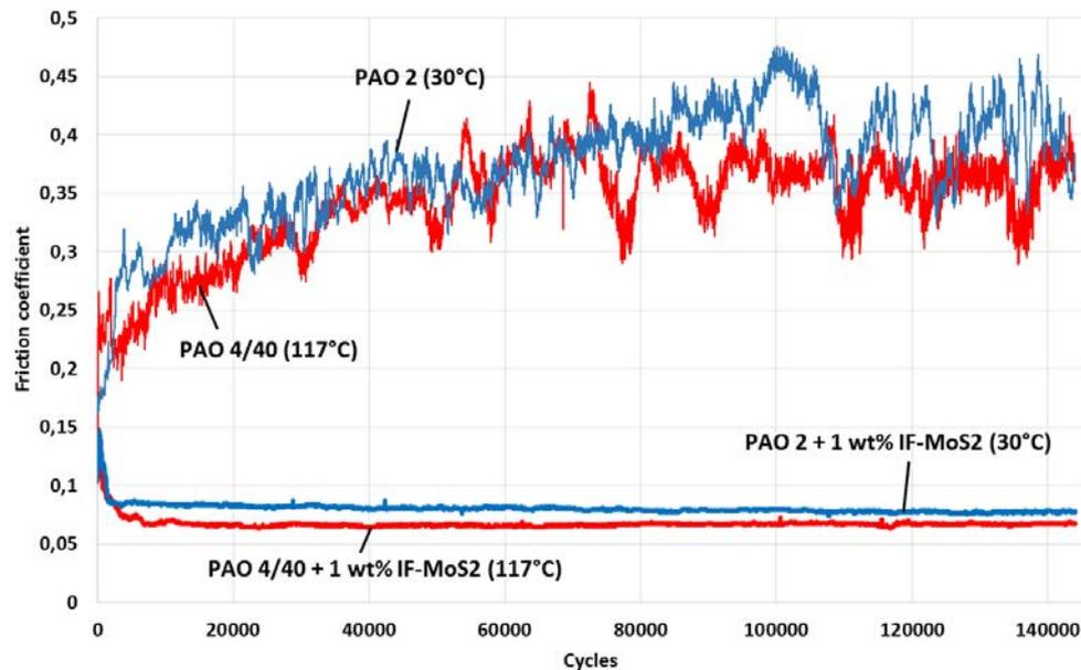
Figure 5.5. HFRR testing of PAO 2 at 30°C (blue) and PAO 4/40 at 117°C (red) with and without 1 wt% SpC IF-MoS<sub>2</sub>
