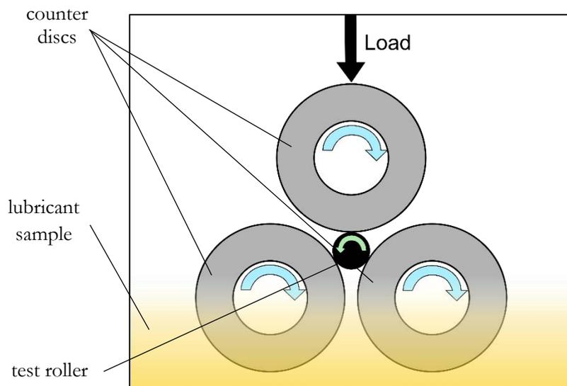
Figure 2.5. Schematic of the MPR
