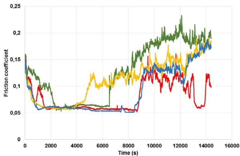
**Figure C. 3.** Repeatability of the test results for the PAO + 1wt% LC IF-MoS<sub>2</sub>
