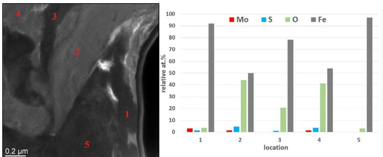
**Figure 3.28.** EDX analyses at different locations of the wear surface for the LC IF-MoS<sub>2</sub>
