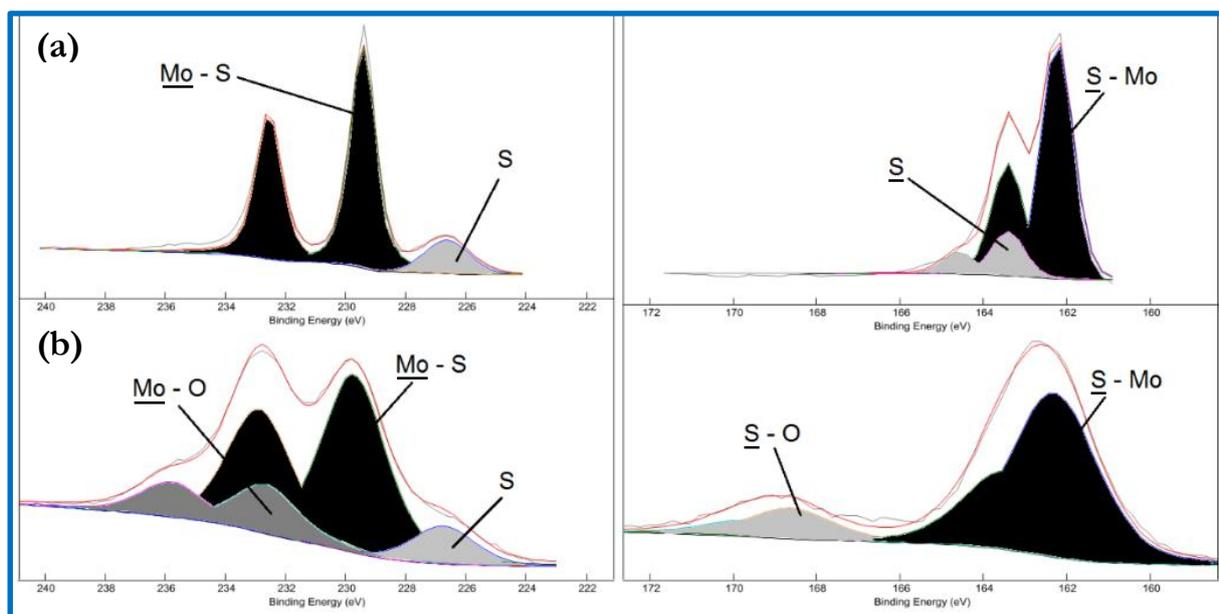
Figure 3.20. XPS spectra of molybdenum (left) and sulfur (right) for the LpC IF-MoS<sub>2</sub> (a) Powder and (b) Tribofilm after 144 000 cycles
