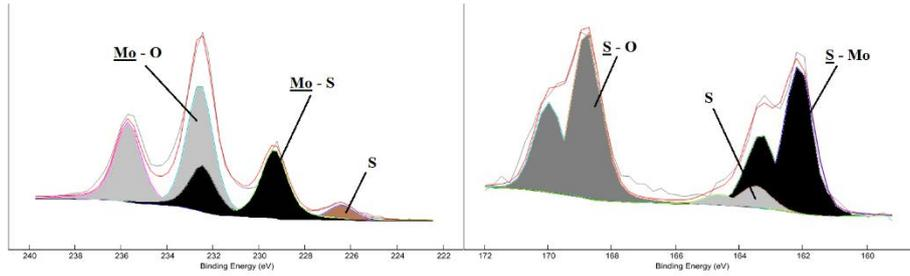
**Figure 5.3.** Mo 3d (left) and S 2p (right) energy peaks found after XPS analysis on the wear scar after HFRR testing for the PAO+1wt% SpC IF-MoS<sub>2</sub> blend at ambient temperature
