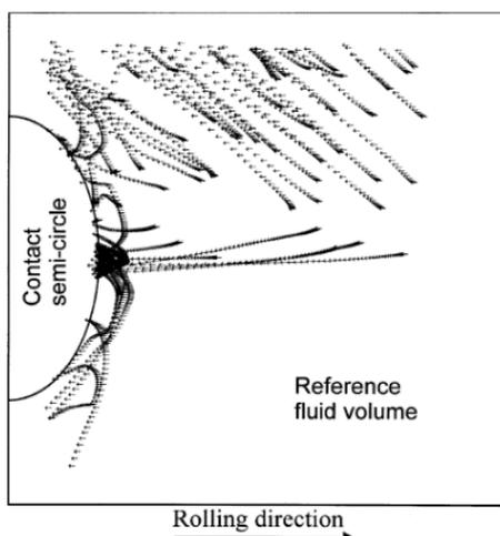
Figure 1.33. Prediction of the trajectory of a 20  $\mu\text{m}$  particle when it is randomly placed before an EHD contact ( $h_c=0.3 \mu\text{m}$ )
