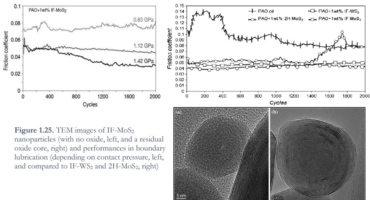
**Figure 1.25.** TEM images of IF-MoS<sub>2</sub> nanoparticles (with no oxide, left, and a residual oxide core, right) and performances in boundary lubrication (depending on contact pressure, left, and compared to IF-WS<sub>2</sub> and 2H-MoS<sub>2</sub>, right)
