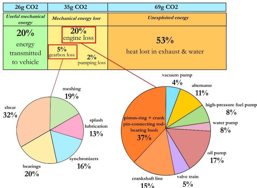
**Figure 1.3.** Estimation of the main sources of energy loss and corresponding CO<sub>2</sub> emissions for a typical Diesel 1.6L engine and gearbox (values extracted from internal PSA Peugeot Citroën data)
