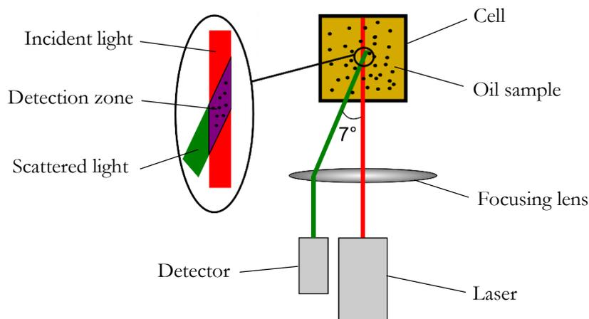
Figure 2.7. Schematic representation of granulometry measurement by DLS
