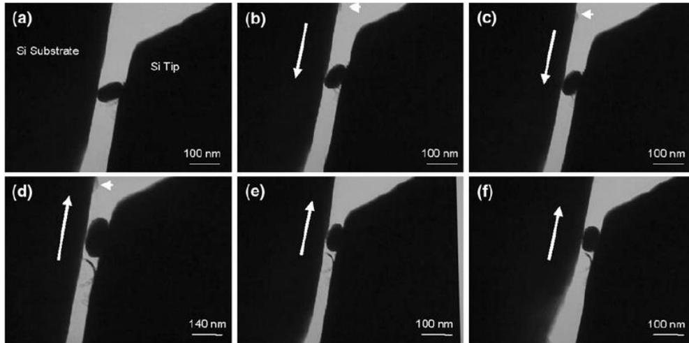
**Figure 1.28.** Rolling/sliding of an individual IF-MoS<sub>2</sub> and partial exfoliation during an *in-situ* HR TEM experiment
