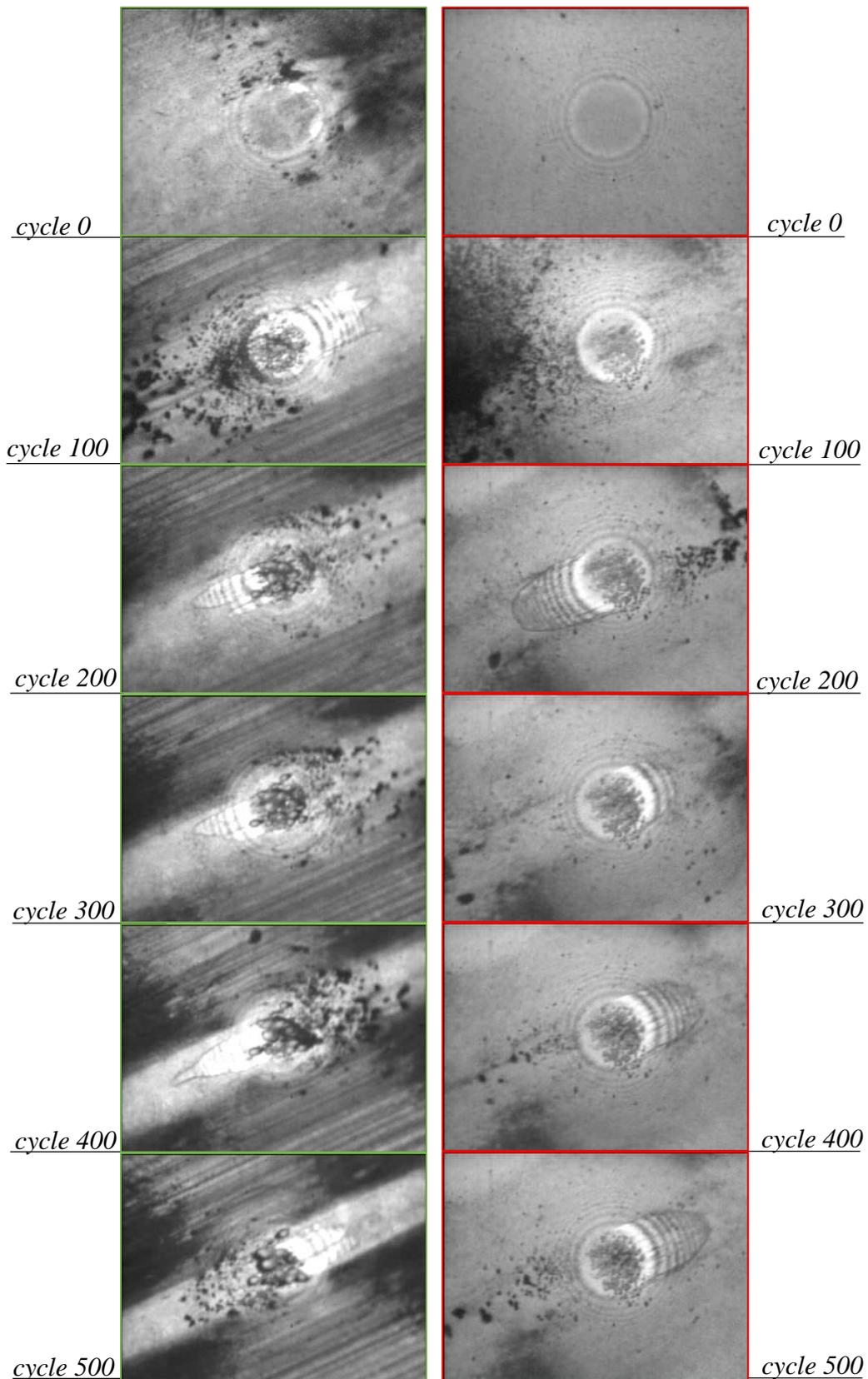
**Figure 4.11.** Nanovisus tests for the nanoparticle-doped base oil (1 wt%) with (right) and without (left) dispersants (5%)
