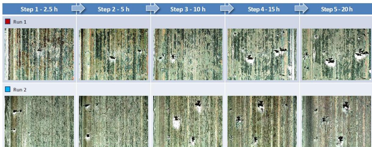
Figure C. 6. Evolution of the contact surface during both MPR runs on the PAO base oil alone
