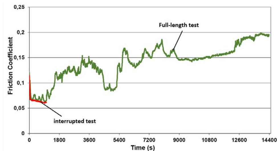
**Figure 3.14.** Full-length and interrupted test using 1wt% LC IF-MoS<sub>2</sub> in order to compare the surfaces during and after testing
