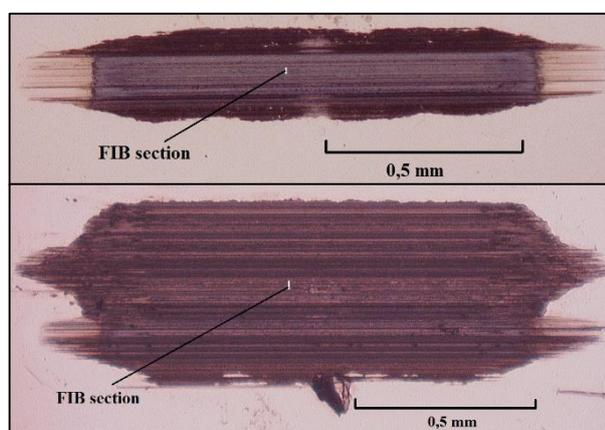
**Figure 3.24.** Positioning of the FIB cross-sections for the SpC (top) and LC (bottom) IF-MoS<sub>2</sub> wear scars (sections not to scale)
