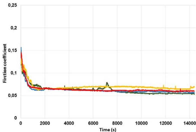
Figure C. 2. Repeatability of the test results for the PAO + 1wt% SpC IF-MoS<sub>2</sub>
