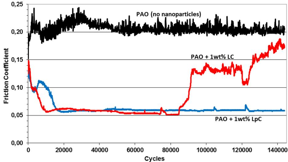
**Figure 3.6.** Friction coefficients of the LC and LpC nanoparticles during the HFRR test
