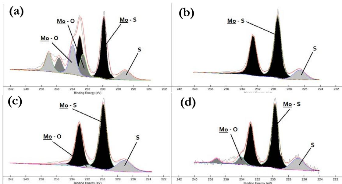
Figure 3.4. Molybdenum 3d spectra measured by XPS for the (a) LC, (b) LpC, (c) SC and (d) SpC IF-MoS<sub>2</sub>
