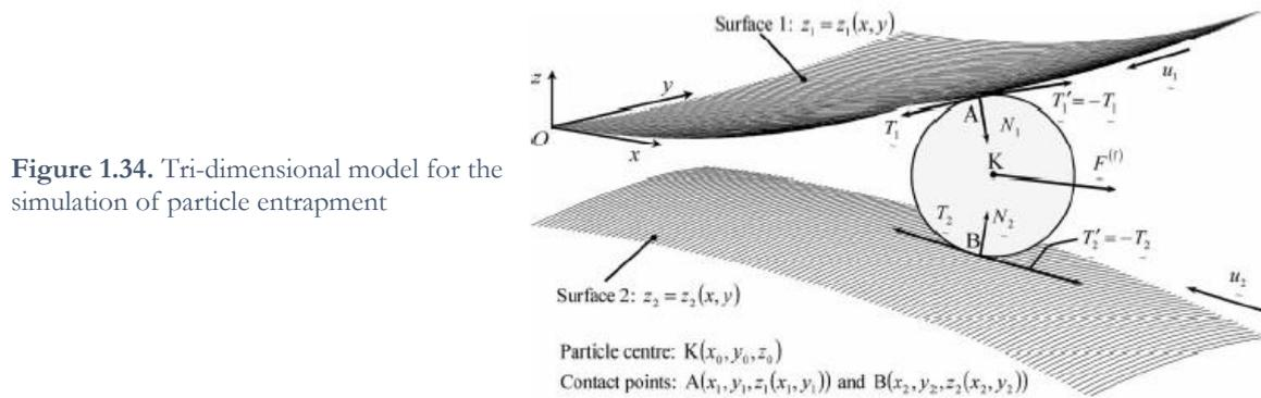
**Figure 1.34.** Tri-dimensional model for the simulation of particle entrapment
