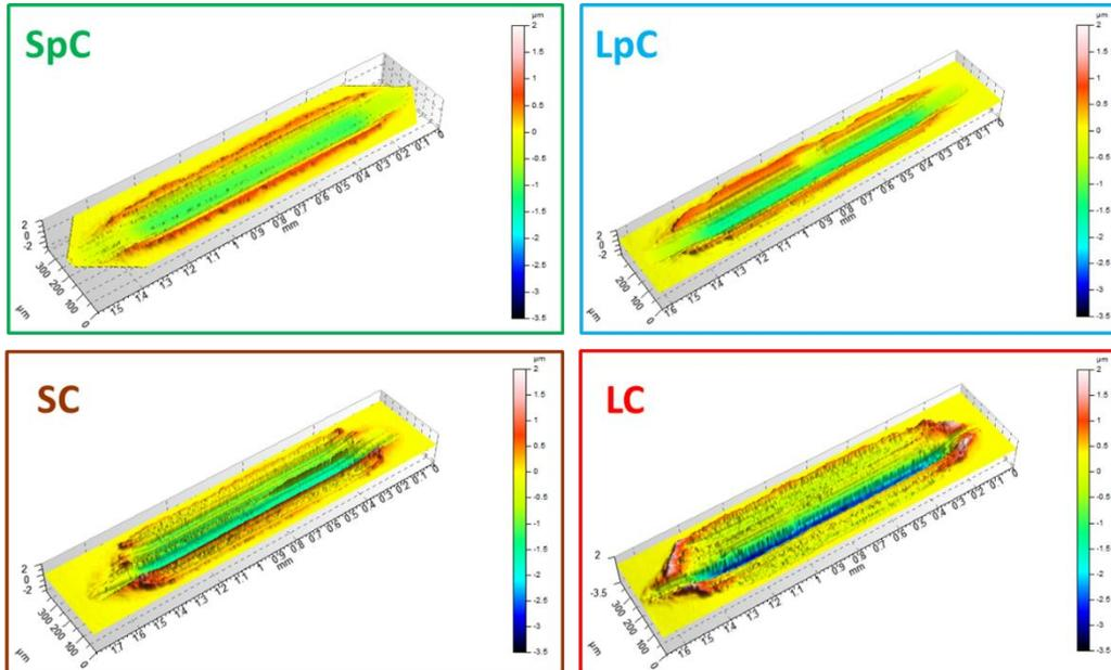
Figure 3.9. 3D measurements of the wear scars obtained for the four different types of IF-MoS<sub>2</sub> nanoparticles
