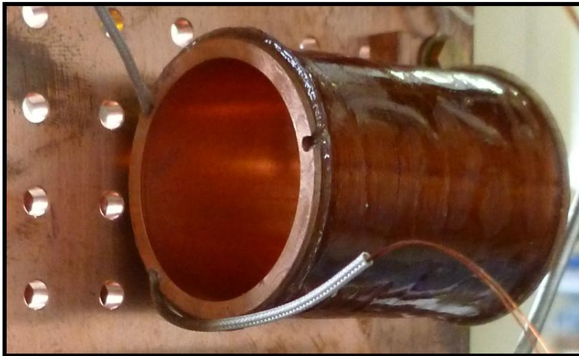
*Figure (2.17): Superconducting coil screwed on the mixing chamber cold plate.*
