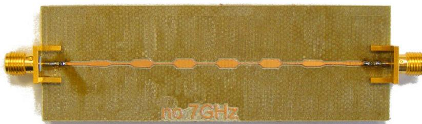
Figure (2.13): Photography of the microwave 7 GHz band-rejection filter.
