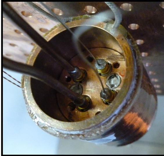
*Figure (2.19): Photograph of the sample holder inside the magnetic coil. Two BeCu/BeCu coax cable are connected to the sample holder via SMP connectors. Two microcoax SS-SS cables are also connected to the sample holder via SMP connectors.*
