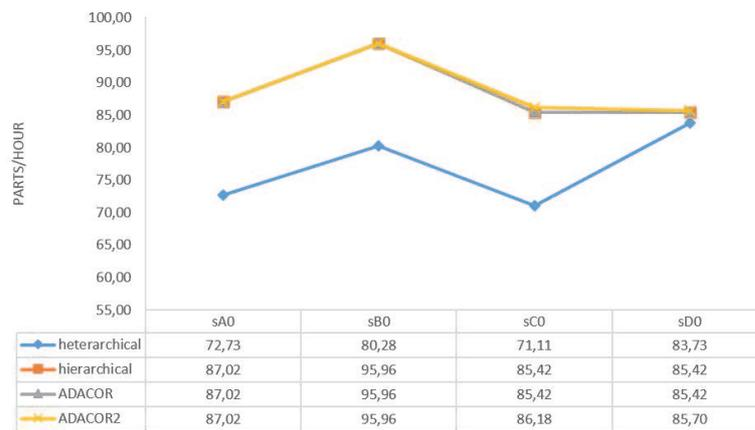
Figure 6.15 – Throughput for the Structural Self-Organization
