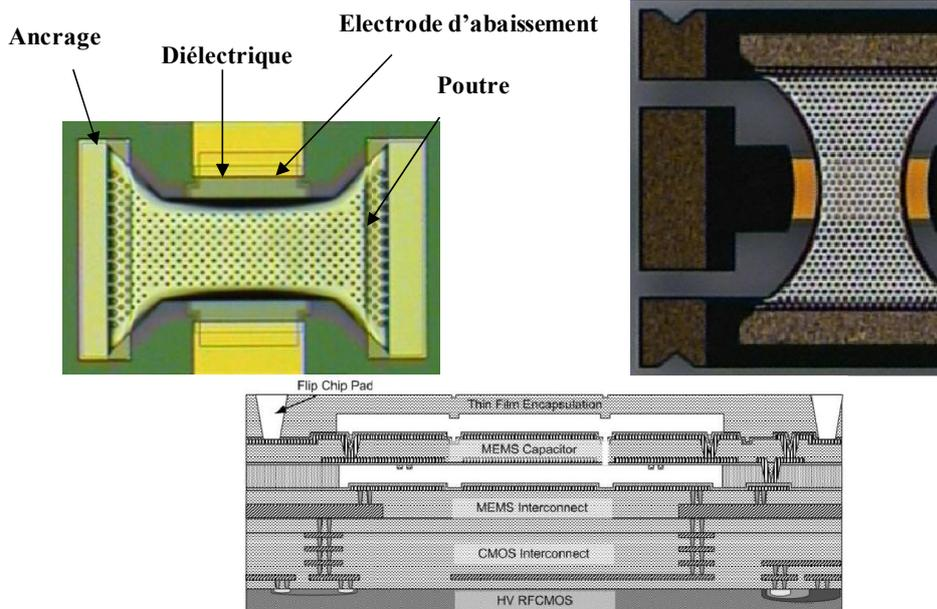
Figure IV-7 : MEMS-RF capacitif Raytheon [25], Memstronic [26], Wispry [27]
