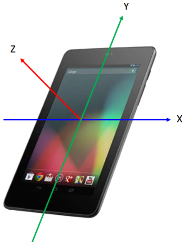
Figure 5.1 – Coordinate definition of the Google Nexus 7 tablet
