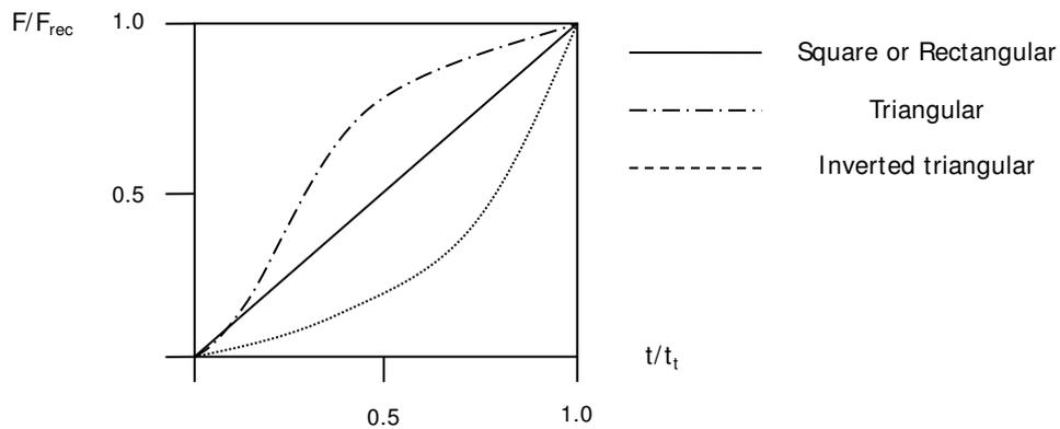
Fig. 2.7 Time and area curve in typical urban catchment
