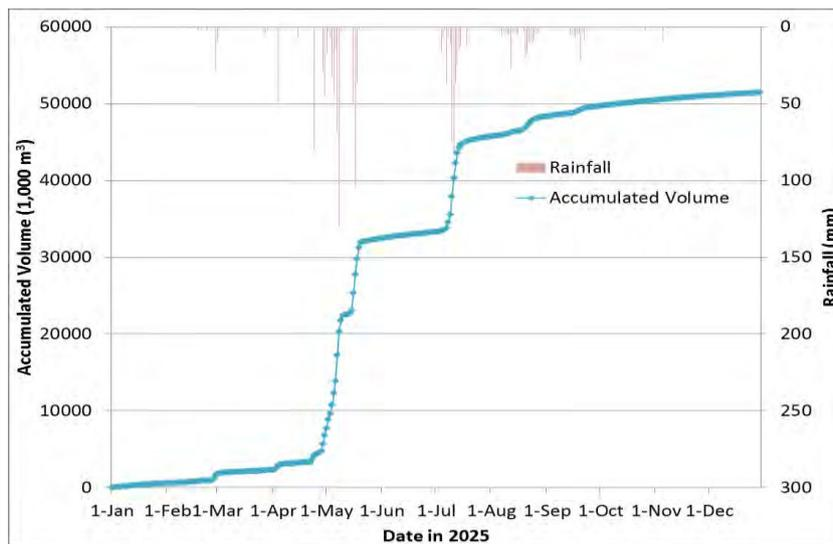
Fig. 5.15 Accumulated water volume of South retention pond
