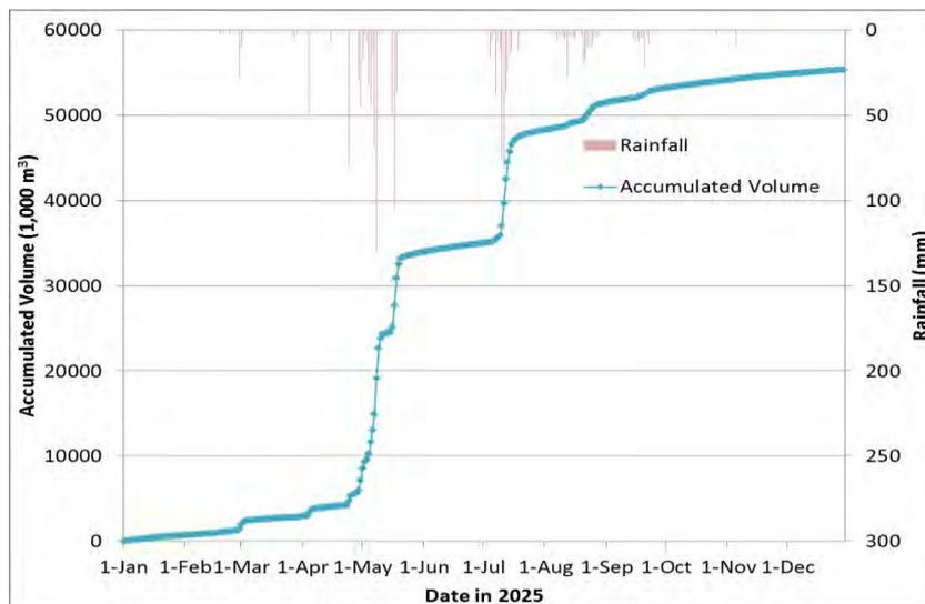
Fig. 5.13 Accumulated water volume of North retention pond
