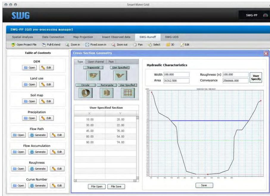
Fig. 3.11 Description of open channel flow modeling
