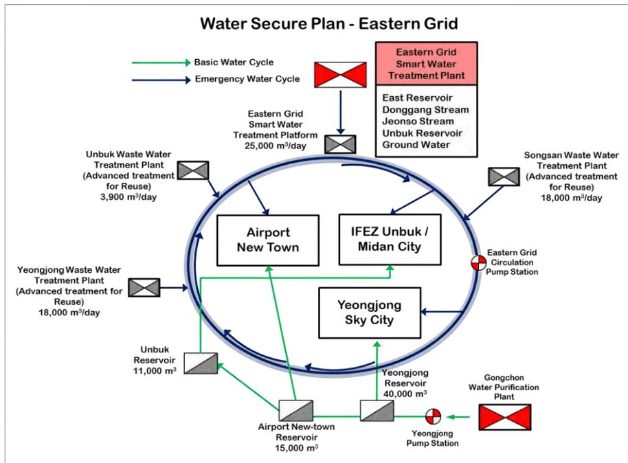
Fig. 5.19 Water secure plan for emergency state (eastern grid)
