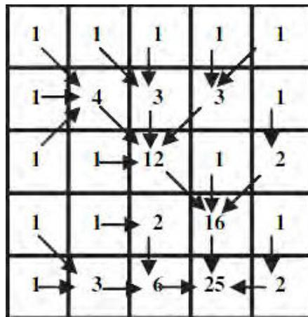
Fig. 2.1 Concept of D-8 Flow grid [79-affdef 논문]
