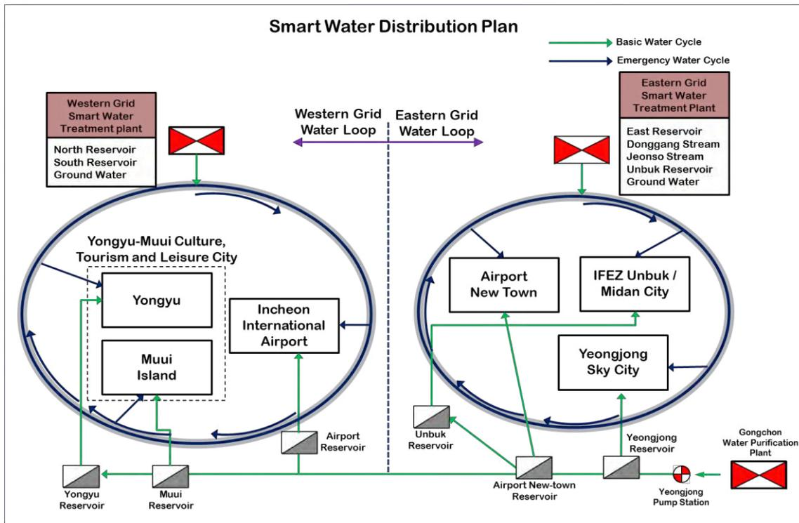
Fig. 5.18 Suggestion of smart water distribution plan
