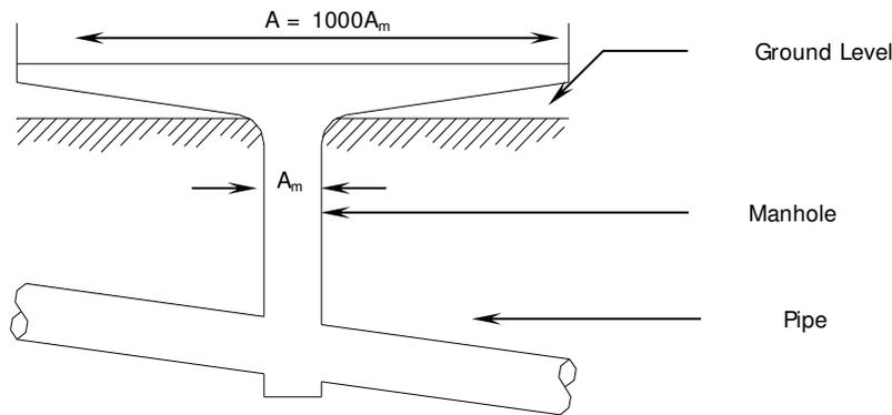
Fig. 2.8 Scenario A Simulation of Surface Flooding [106]
