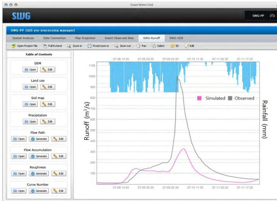
Fig. 3.10 The instant result window after the first simulation
