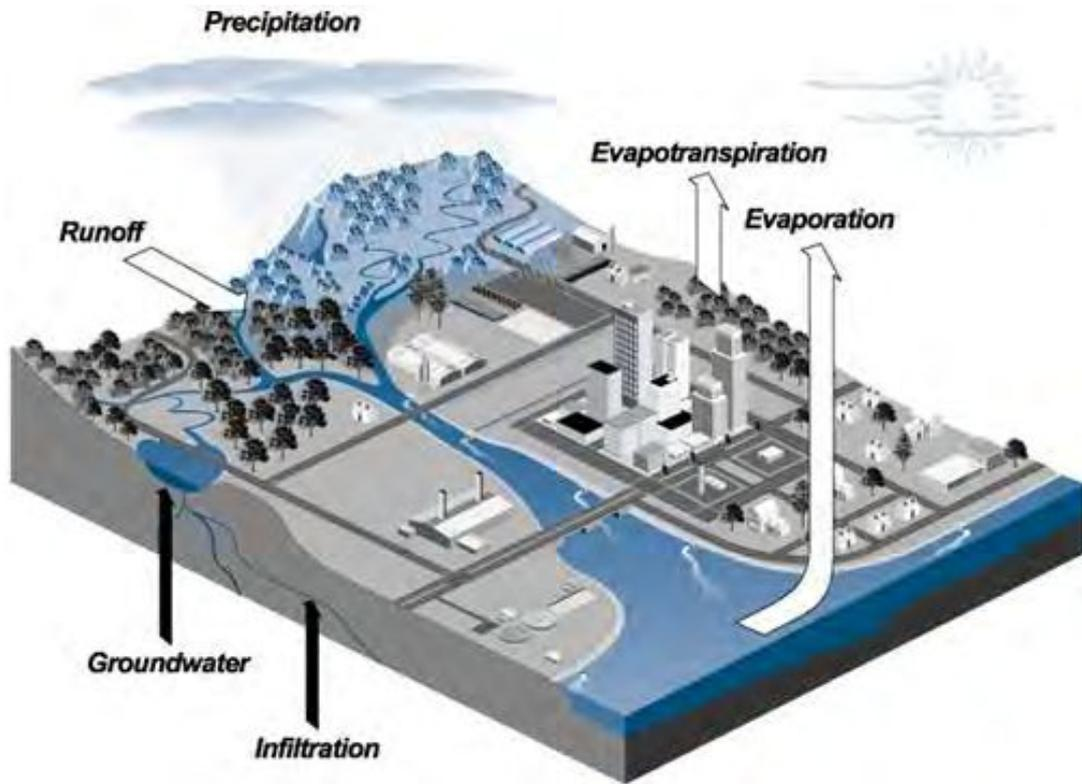
Fig. 1.1 Common view of hydrologic cycle (Gourbesville, 2014)
