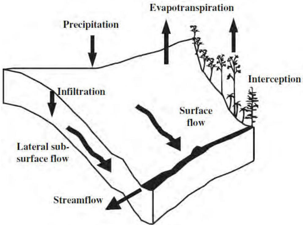
Fig. 2.3 The schematic diagram describing hill slope hydrology (Moretti, 2007)
