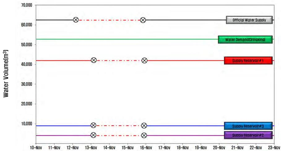
Fig. 5.25 Broken water balance due to the accident at western grid
