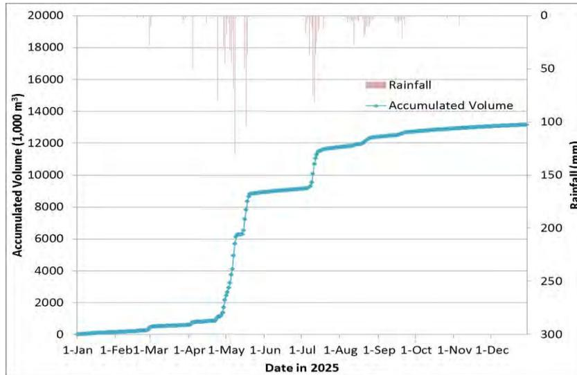
Fig. 5.5 Accumulated water volume of Donggang Stream
