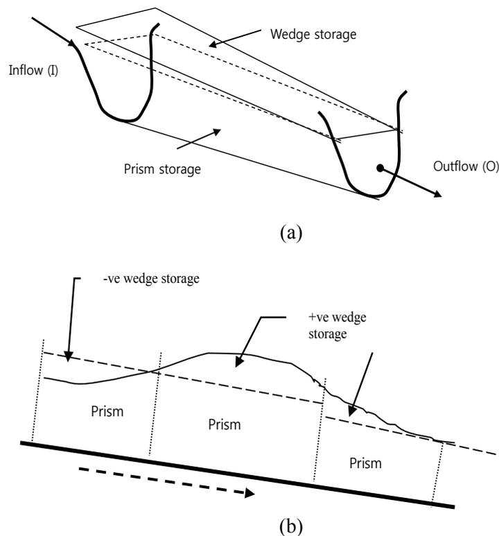
Fig. 2.11 Prism and wedge storage in a river channel during flood flow
