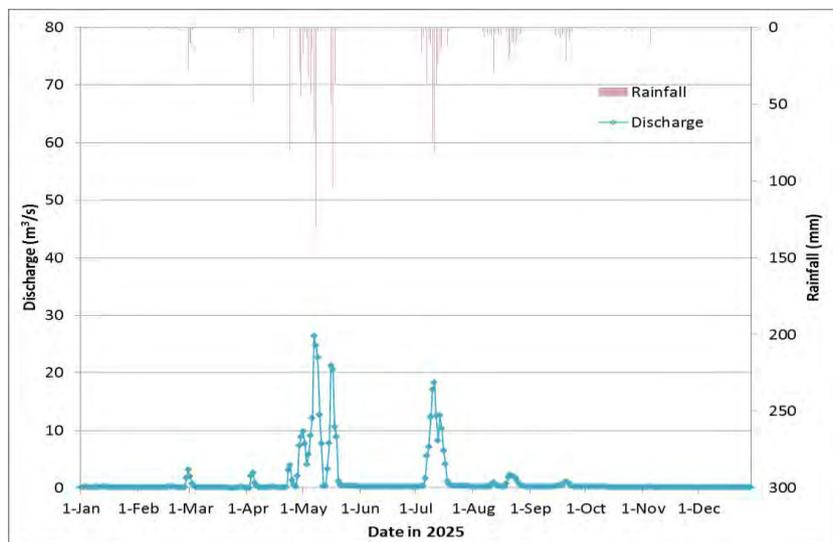
Fig. 5.10 Daily flow discharge of the East retention pond
