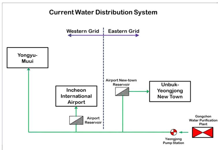
Fig. 5.16 Current water distribution system of study area
