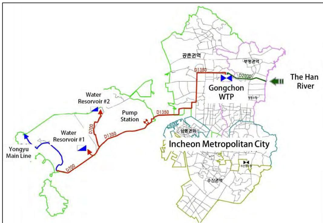
Fig. 4.8 Main pipe line of official water distribution system
