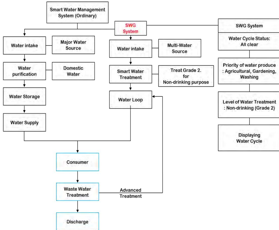
Fig. 3.16 Ordinary water distribution with smart water technologies
