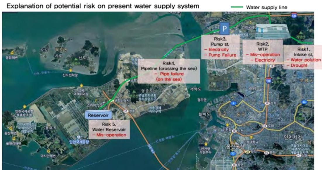
Fig. 4.3 Potential risks on present water supply system of the Yeongjongdo Island
