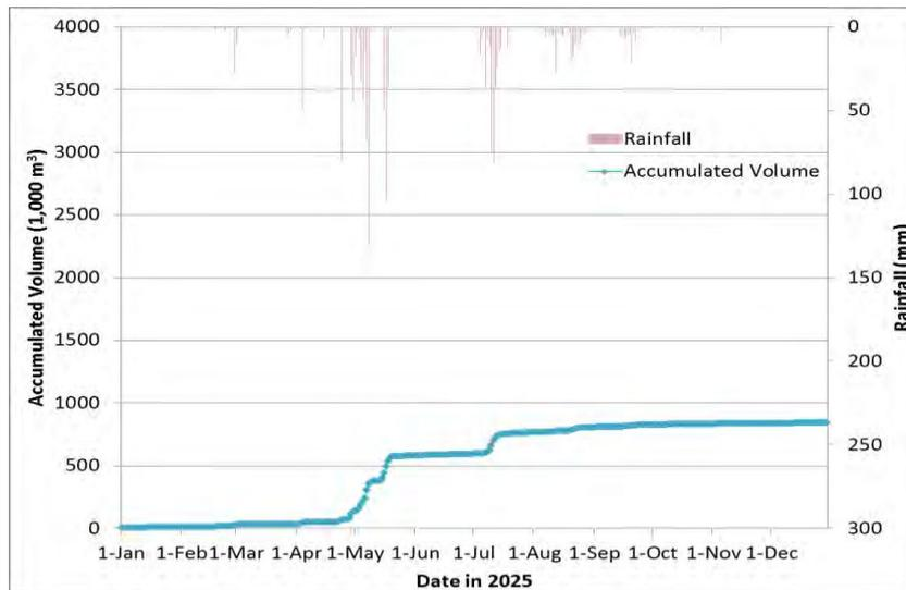
Fig. 5.9 Accumulated water volume of Unbuk reservoir
