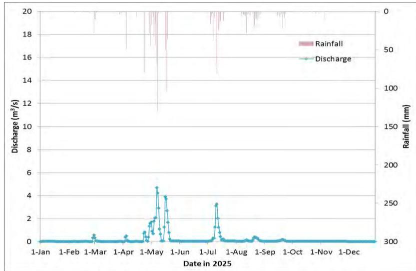
Fig. 5.14 Daily flow discharge of the South retention pond
