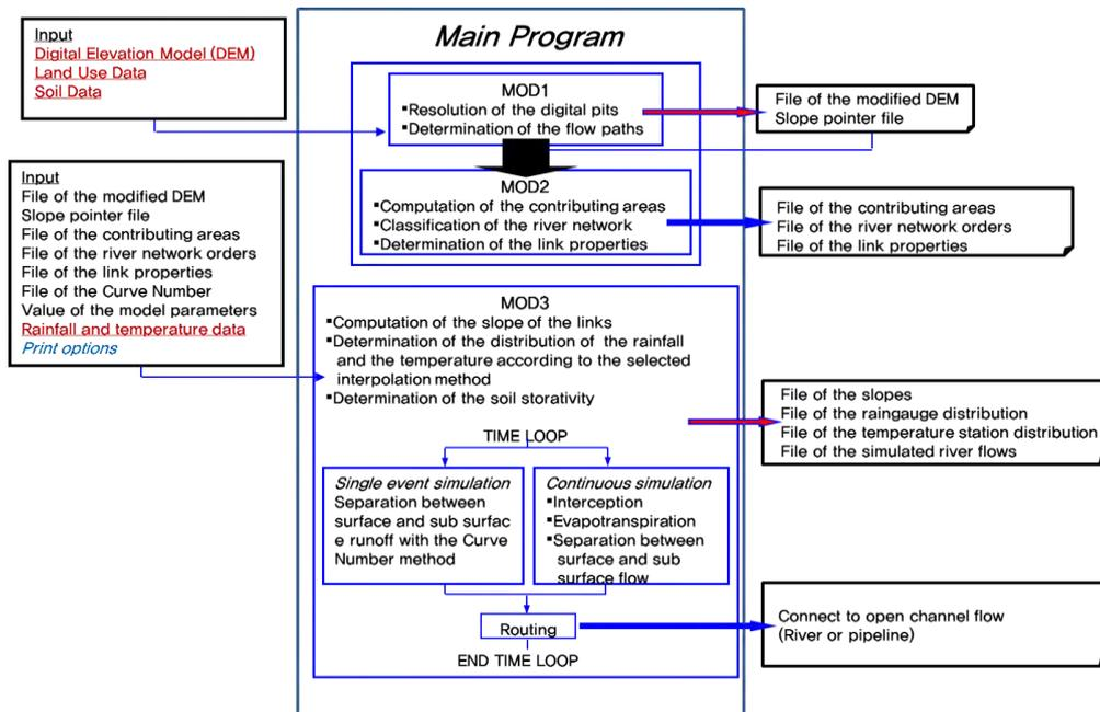
Fig. 3.8 General framework of data flow and simulation
