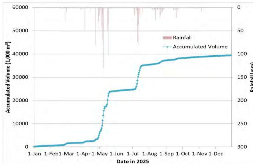
Fig. 5.11 Accumulated water volume of East retention pond
