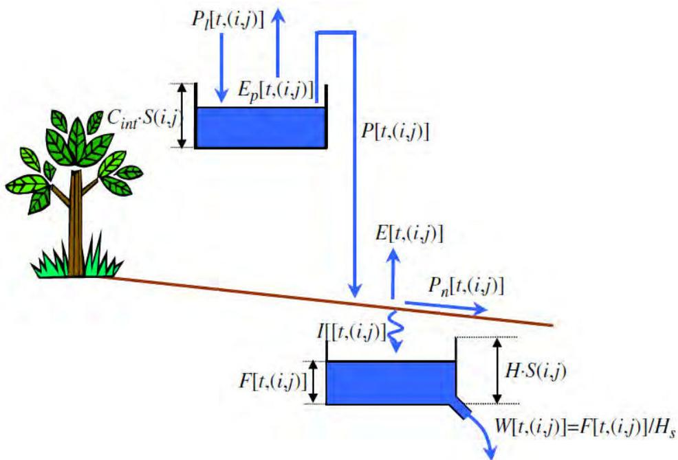
Fig. 2.4 The schematic diagram of soil interaction of water (Moretti, 2007)
