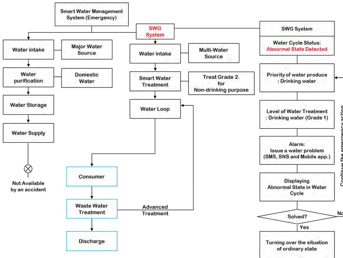
Fig. 3.18 Emergency water distribution with smart water technologies
