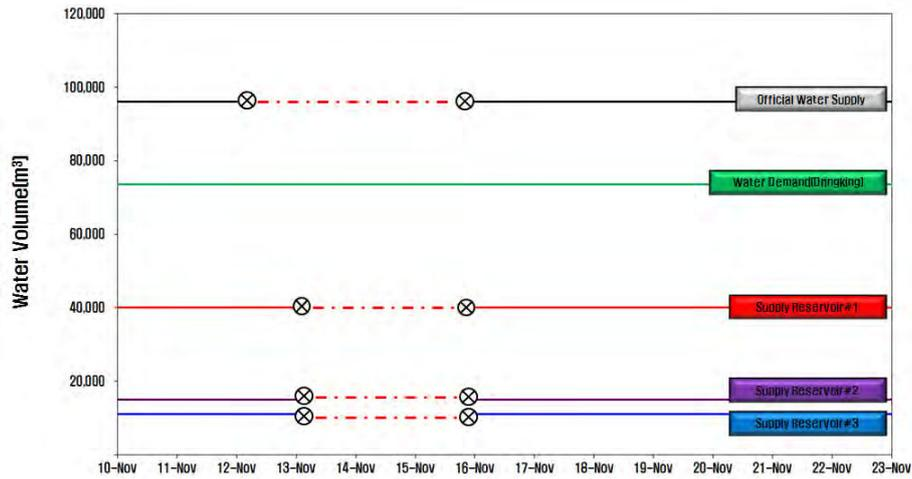
Fig. 5.21 Broken water balance due to the accident at eastern grid
