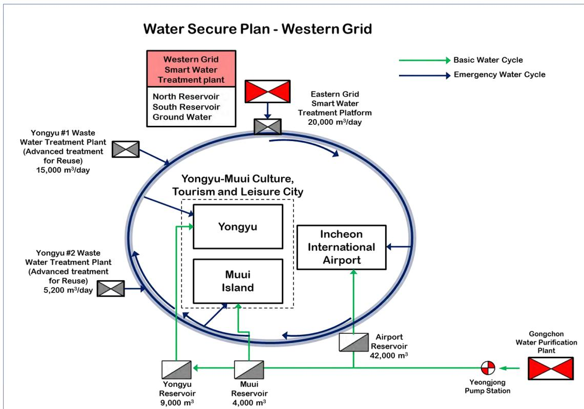
Fig. 5.23 Water secure plan for emergency state (western grid)
