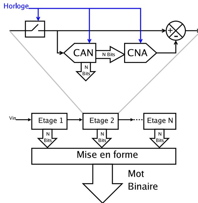
FIGURE 2.8 – Structure Pipeline
