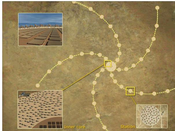
FIGURE 2 – Structure du Square Kilometer Array
