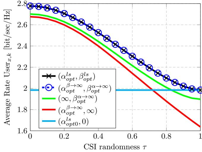
Figure 4.4: Average user rate vs. CSI quality for adaptive precoder weights ( $N = 160$ ,  $K = 40$ ,  $\varepsilon = 0.7$ ,  $P = 10\text{dB}$ ).
