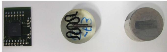
**Figure 3.13: Different steps of the sample preparation: single package (left), embedded package prepared for optical microscopy (middle), and for SEM+EDS (right)**
