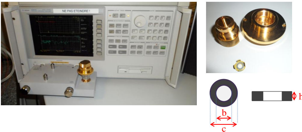
Figure 3-4: Complex permeability measurement set-up; b and c : respectively internal and external diameter of the tore; h : thickness of the tore
