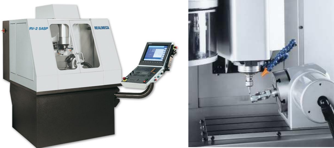
Figure A2-3: Micro-milling machine Réalmecca RV2 SP (left) and 200 µm end mill (right)
