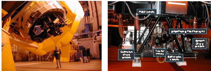
Figure 1: OHANA injection module mounted under the Adaptive Optics PUEO at Canada-France-Hawaii Telescope.
