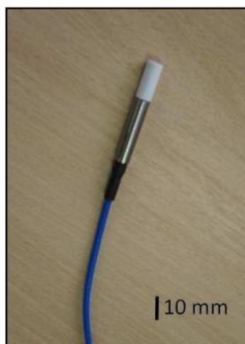
Figure IV-6 : Diode E de PTW (PTW Freiburg, Freiburg, Germany), modèle T60012.
