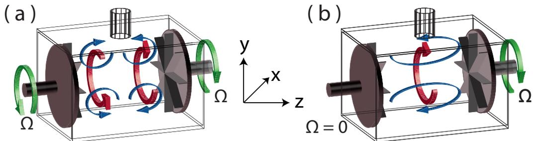
Figure VI.1: Drawing of the mean flow in a square section von Kármán apparatus. (a): two counter-rotating discs product two azimuthal counter-rotating cells (red arrows) and meridional recirculations (blue arrows). (b): one disc products a strong azimuthal rotation (red arrow) and a meridional recirculation (blue arrows).
