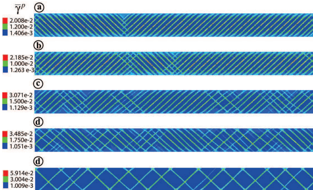
Figure 7 The \bar{\gamma}^p patterns in layer 2 in four models run to the same total horizontal shortening of 2.8 \times 10^{-2} m. (a) E = 5E_2 . (b) E = E_2 . (c) E = 0.5E_2 . (d) E = 0.3E_2 . (e) E = 0.05E_2 . Other model parameters are indicated in the caption of Fig. 5.
