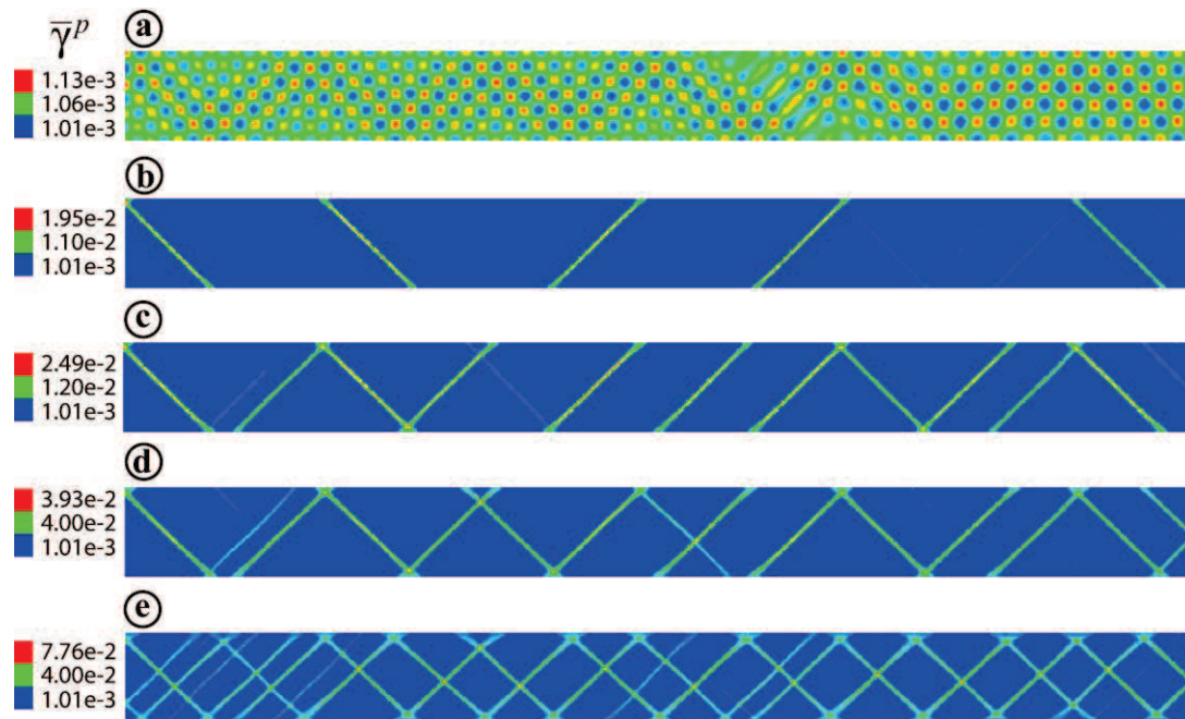
Figure 8 Several stages of the evolution of the \bar{\gamma}^p pattern in layer 2 at E = 0.05E_2 . Other model parameters are indicated in the caption of Fig. 5.
