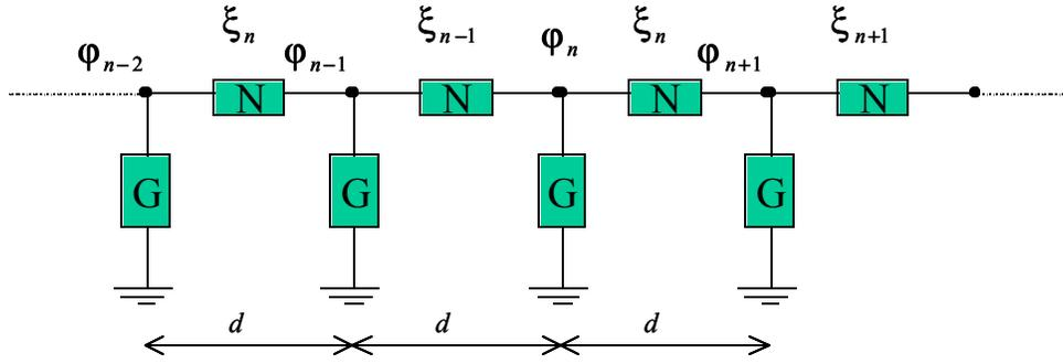
Figure 3-6: Generalized lumped transmission line
