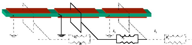
Figure 6-3: Transmission Line with Line Resistance and Inductance (*TL-R<sub>l</sub>-L<sub>l</sub>*): Basic Cell
