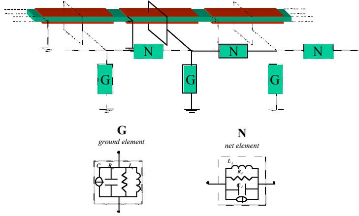
Figure 5-1: Basic cell of the periodic PEM structure
