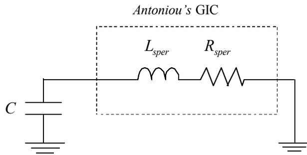
Figure 7-9:  $RLC$  resonant circuit for experimental testing of the Antoniu's  $GIC$  by frequency response measurements.
