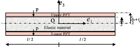
Figure 4-1: Laminated PiezoElectroMechanical (*PEM*) beam: lateral view
