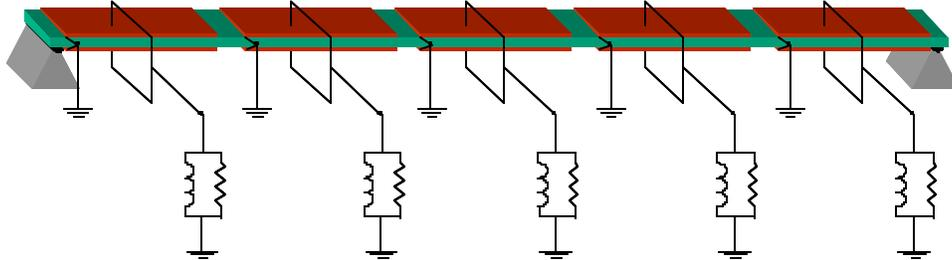
2. a beam<sup>7</sup> coupled with the lumped version of an electric transmission line with line resistances and inductances
