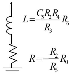
Figure 7-7: Synthetic Inductor: ideal equivalent impedance
