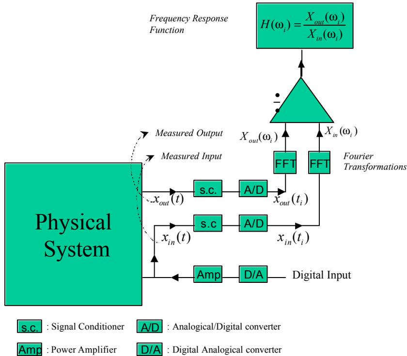
Figure 7-12: Logical scheme for Frequency Response measurements
