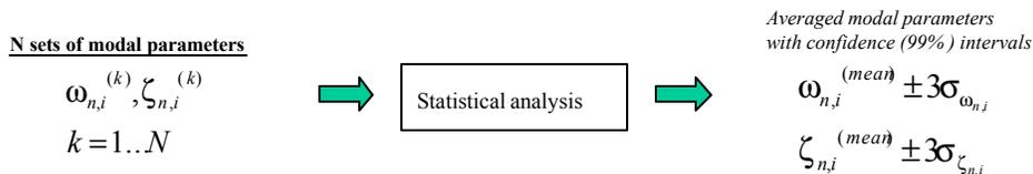
Figure 7-15: Identification procedure
