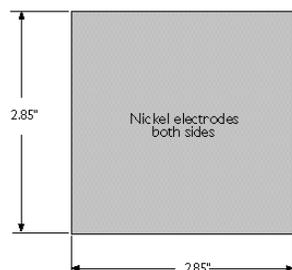
Figure 7-3: Single sheet piezoelectric transducer
