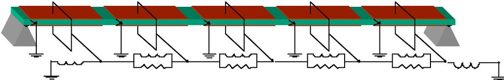
3. a beam coupled with the lumped version of an electric transmission line with line inductances and ground resistances
