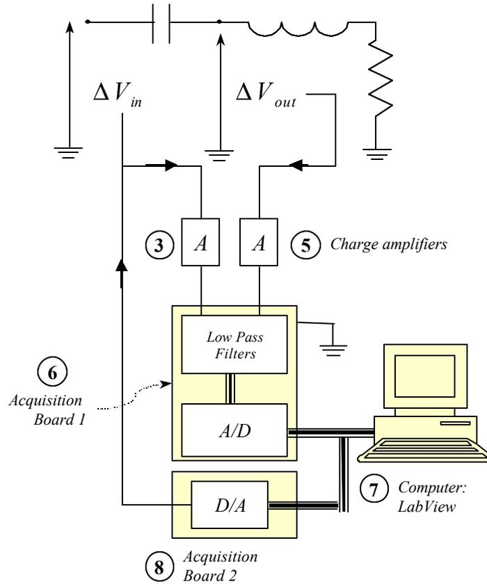
Figure 7-14: Experimental set up for electrical FRF measurements
