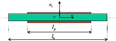
Figure 4-9: Bimorph PZT transducer on a elastic beam: lateral view
