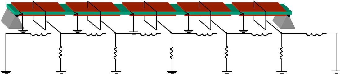
Their performances in the suppression of mechanical vibrations must be investigated as a function of the values of the electrical parameters to validate the theoretical and numerical results obtained in the previous chapters. To this aim the mechanical forced response can be found with the experimental setup in figure 7-13.
