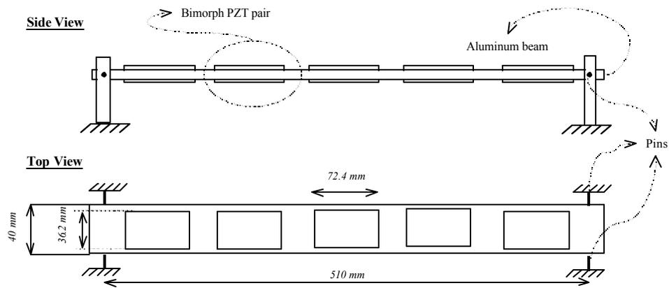
Figure 7-1: Pinned-pinned beam with five bimorph PZT pairs
