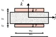
Figure 4-2: Laminated PiezoElectroMechanical (*PEM*) beam: cross section
