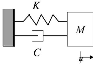
Figure 3-2: Spring-mass-damper system
