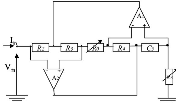
Figure 7-6: Synthetic inductor: an alternative modification of Antoniou's GIC
