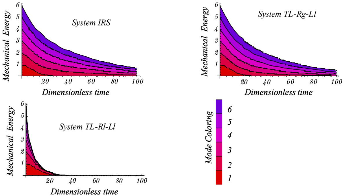
Figure 6-8: Modal mechanical energies as a function of time for a simply supported  $PEM$  beam with different network topologies optimized for the first bending mode.
