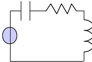
Figure 3-3: RLC series circuit
