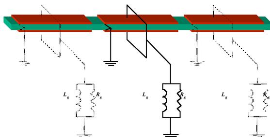
Figure 6-2: Isolated Resonant Shunts (*IRS*): Basic Cell
