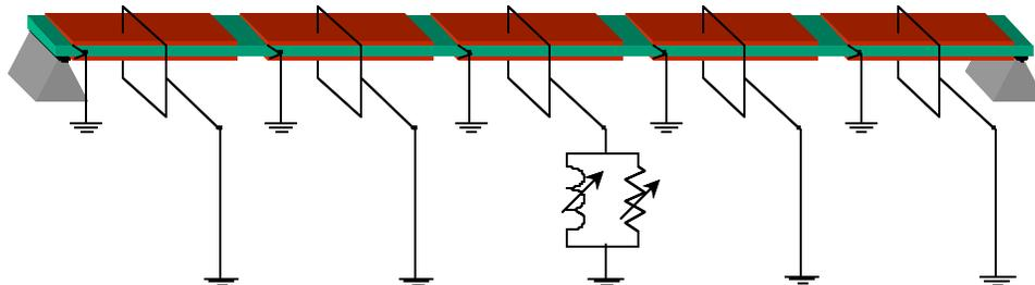
Figure 7-20: Configuration for the resonant shunted PZT experiment
