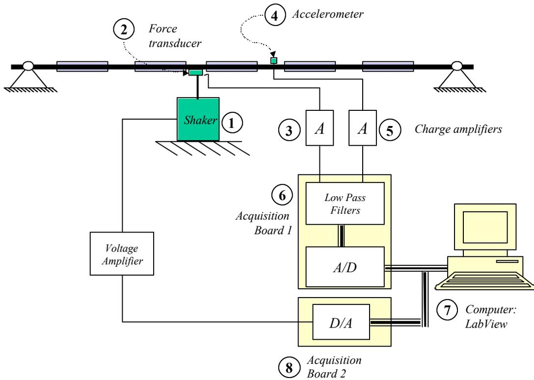
Figure 7-13: Experimental set up for mechanical FRF measurements
