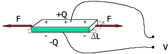
Figure 2-2: *PZT* sheet working by 3 – 1 effect.
