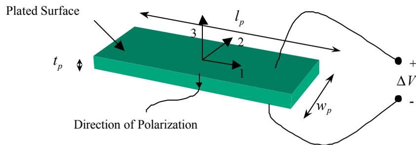
Figure 2-1: PZT sheet working by 3 – 1 effect
