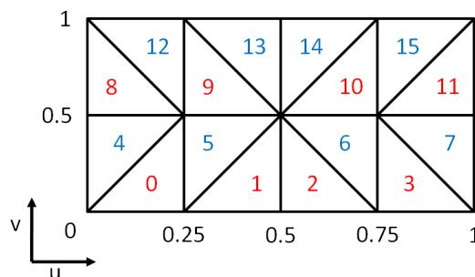
Figure 4.9: A quadrilateral patch is tessellated into  $i \times j$  quadrilaterals with  $i = 4$  and  $j = 2$ , each of which being subdivided into 2 triangles. We index the triangles depending on their barycentric tessellation coordinates  $u, v$  following the algorithm 2. Red indices correspond to triangle being the lower part of the quadrilateral, while blue indices are upper parts.
