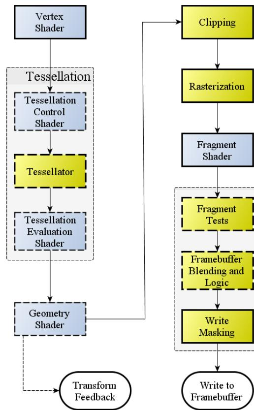
Figure 2.12: OpenGL 4.0 Pipeline.
