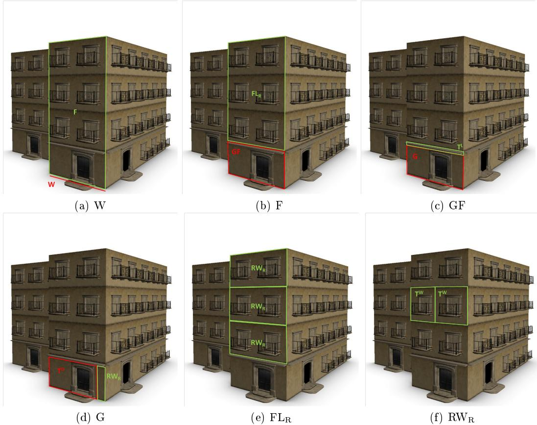
Figure 4.12: Non terminal rules of the above grammar are explained on example. The axiom **W** is shown in a red line, while successors are blue and green quadrilaterals, respectively for the first and second successors.
