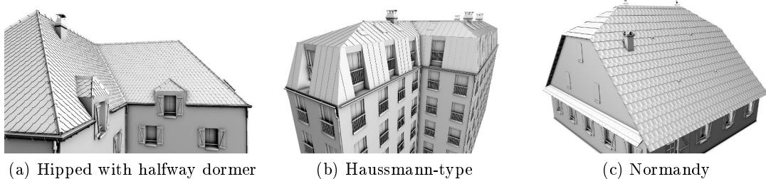
Figure 5.1: We extend the GPU shape grammars pipeline to reconstruct structured data. Our solution allows for efficient modeling of complex roof structures starting from independent 1D atoms. Note that gutters, chimneys, ridge tiles and overhangs are also generated by the system.
