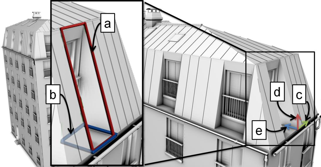
Figure 5.8: Illustration of the *Project* rule. The blue quadrilateral *b*) is the projection of the red quadrilateral *a*). The projection axes are the local tangent *c*) and the cross product *e*) between the local tangent and the global normal *d*).
