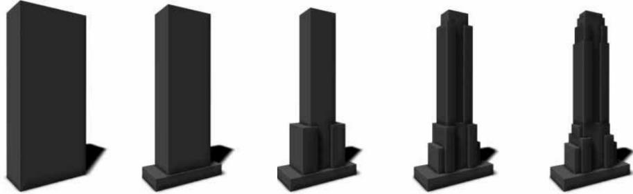
Figure 3.7: L-System for building. Five consecutive steps of the generation of a building, allowing easy LOD generation. Image from [PM01].
