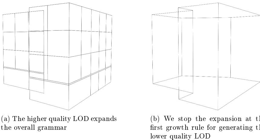
Figure 7.4: We define two grammar-based LODs for architecture modeling.
