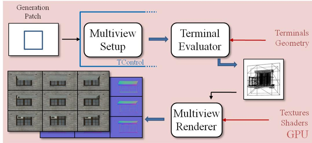
Figure 7.5: We generate impostors on the fly. For each terminal shape, we generate it using the same principle as for the terminal evaluation described in Chapter 4 (*i.e.*, with the hardware tessellator of the GPU). By specifying a multi setup, we are able to render the same geometry from various view angles in a single render pass. We store both photometric and normal information for later use at run-time.
