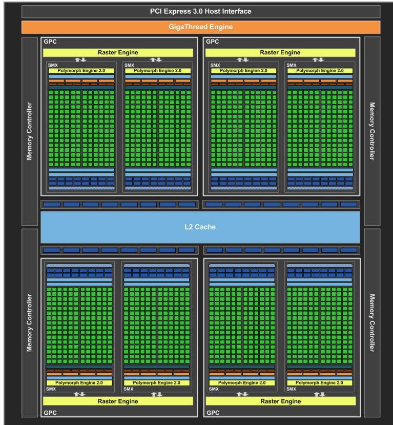
Figure 2.9: GeForce 680 GTX - GK104 Kepler Architecture.
