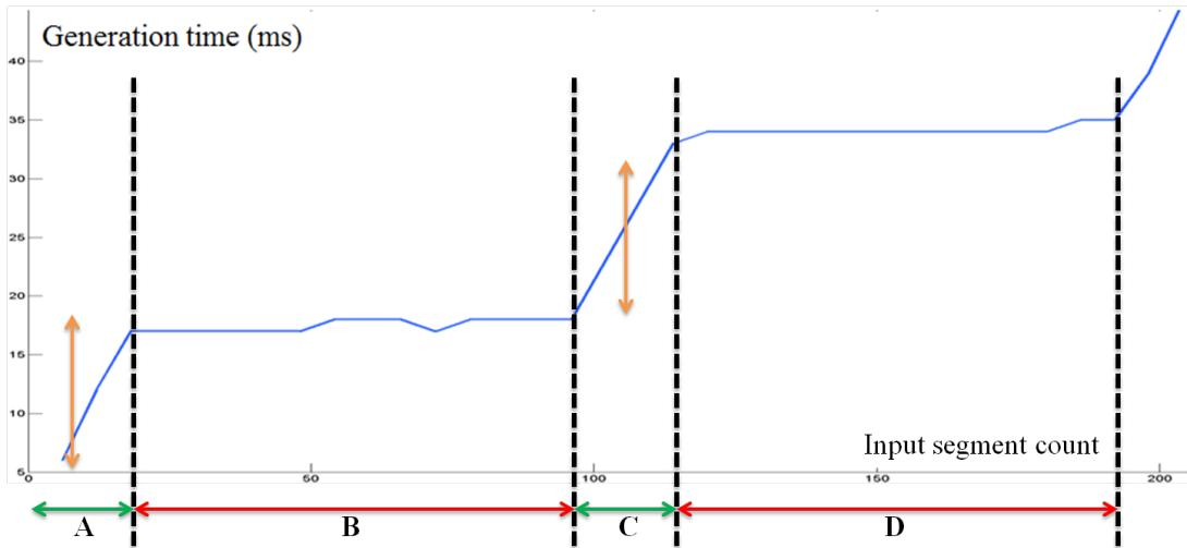
Figure 4.17: Sublinear complexities are observed when the GPU shape grammars is filled with many input segments. Around 100 input segments are processed in parallel at each computation round. The orange arrows show the preparation time of one computing grid. For a given round of computation (*e.g.*, A+B, C+D sections), the first linear slope is due to the first grid preparation. Then, other grids preparation are performed in parallel to the first one.
