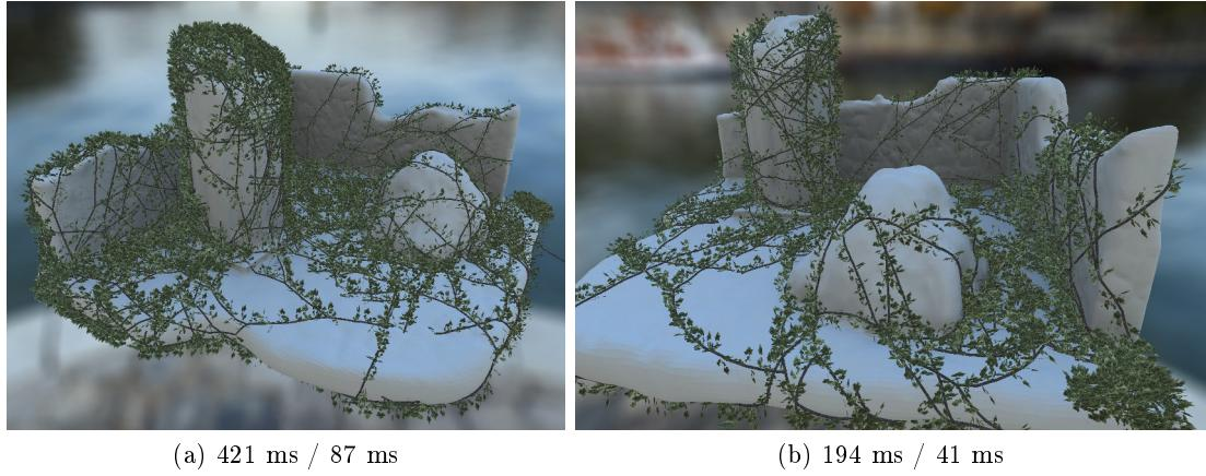
Figure 6.15: The ruins model is covered by 18 (a) and 24 (b) ivy plants, with grammar parameters  $stepNumber = 34/48(a/b)$ ,  $stepSize = 10/13$ ,  $stepBranch = 6/14$  and  $numberOfLeaves = 2/2$ . Respectively 5.17M and 2.27M polygons are generated. Timings are indicated as rule expander / terminal evaluation and rendering.
