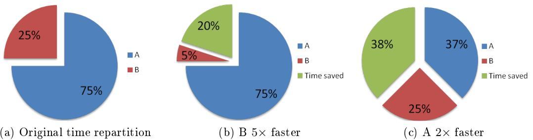
Figure 2.2: Focusing efforts on parallelizing larger parts of an algorithm is more profitable than working hard to achieve a better speedup onto the smaller parts. Here a speedup of  $\times 2$  for the computation of the part A gives a better total speed computation improvement (c) than a speedup of  $\times 5$  for the part B (b).
