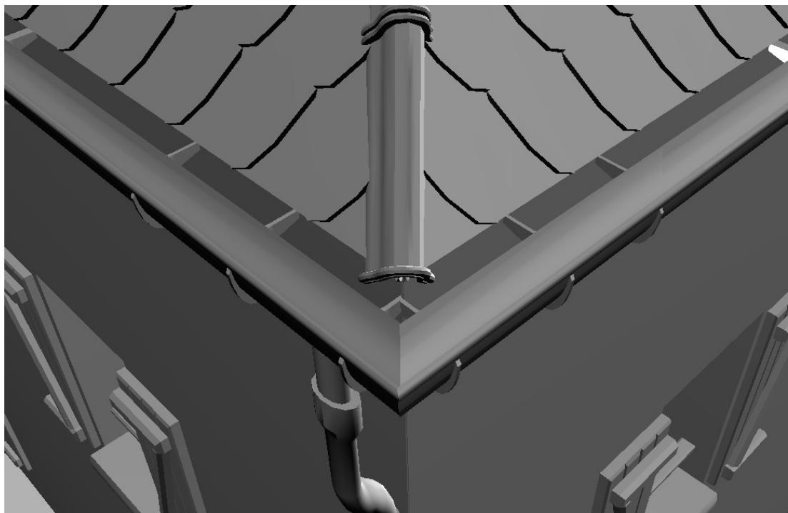
Figure 5.10: Gutters are consistent models which use the same local context information as for roof construction. We benefit from seamless geometry mapping between adjacent gutters using the *Join* and the automatically generated clipping planes.
