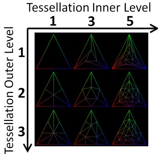
Figure 2.13: Triangle refinement according to the inner and outer tessellation factors.
