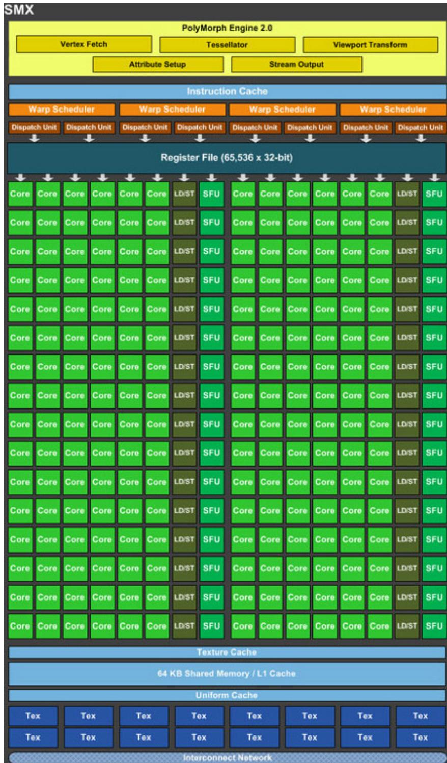
Figure 2.11: GeForce 680 GTX - SMX Diagram.
