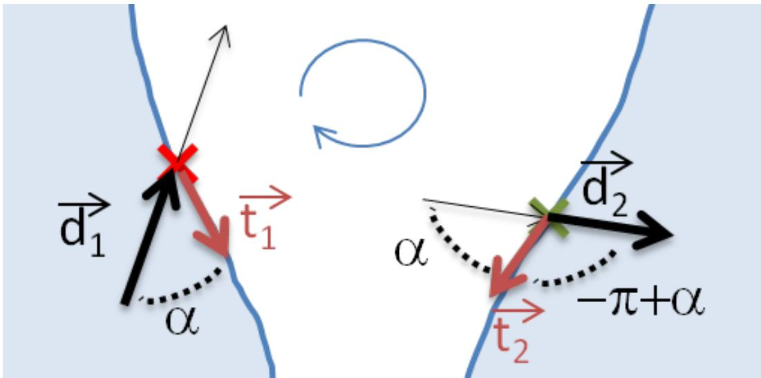
Figure 6.9: Marching direction is oriented according to the source and destination 2D tangent vectors. Let  $\alpha$  be the angle between  $\vec{t}_1$  and  $-\vec{d}_1$ , the destination marching direction  $d_2$  is the rotation of  $t_2$  of  $-\pi + \alpha$ .
