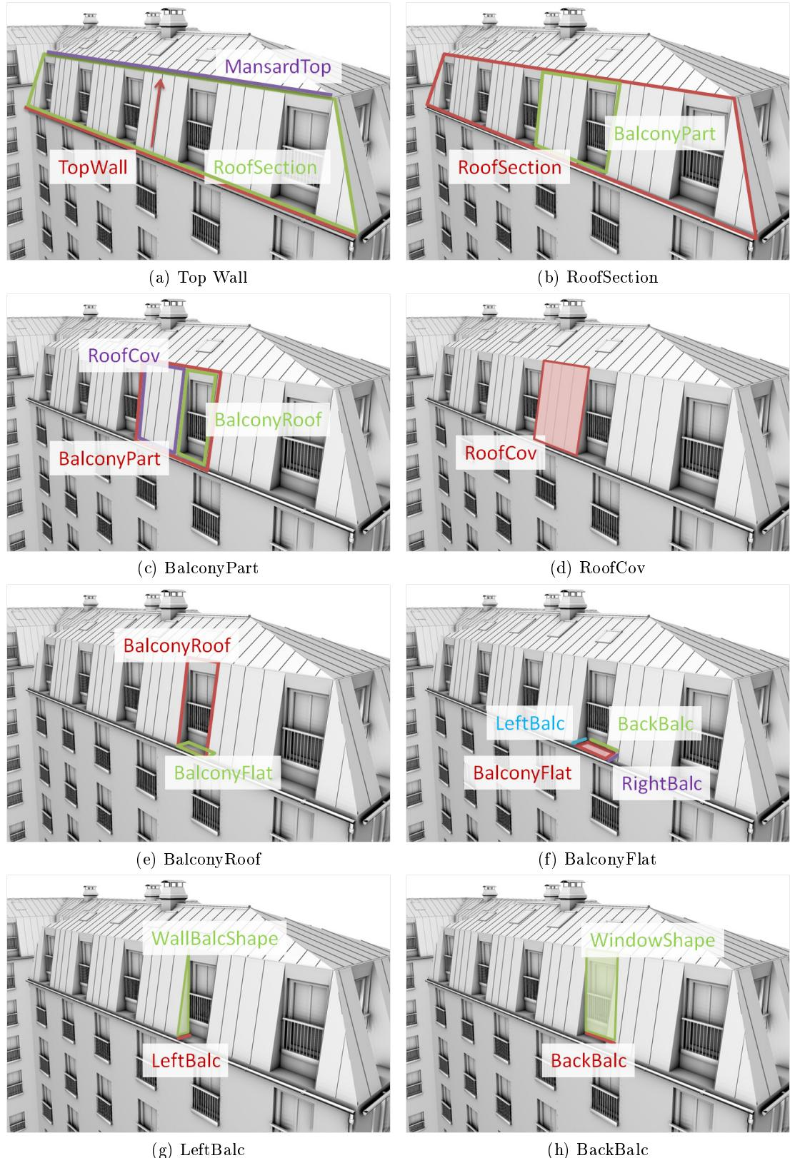
Figure 5.9: The roof grammar presented in this chapter is described rule by rule. Predecessor is indicated in red, while successors are either in green, blue or purple. *RightBalc* rule is similar to the *LeftBalc*. Terminal shapes are applied on color filled quadrilaterals.
