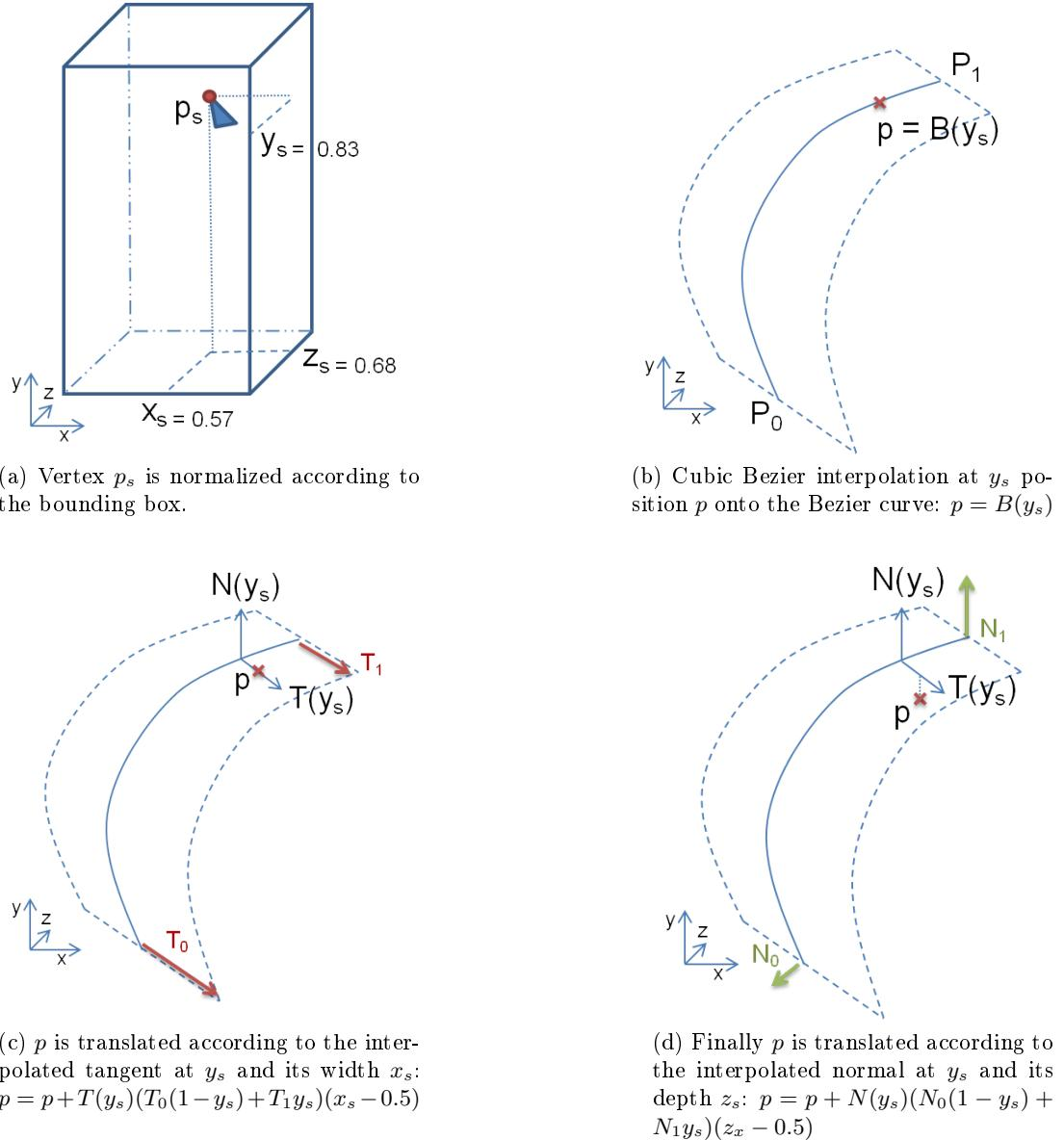
Figure 6.13: Incremental computation of the position  $p$  according to the Bezier curve.
