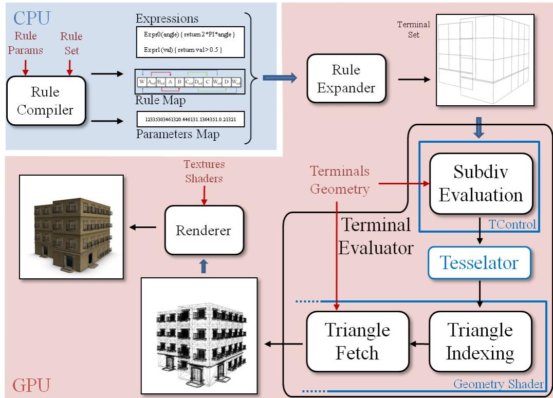
Figure 4.10: The detailed geometry of the terminal symbols is substituted to the terminal set using hardware tessellation and on the fly geometry evaluation, providing a fully detailed model ready for rendering.
