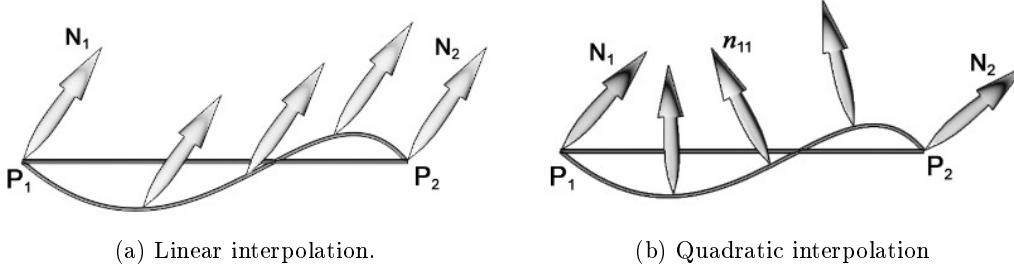
Figure 6.12: Linear interpolation of the normal endpoints (a) does not preserve the inflection of the surface, while quadratic interpolation does. Figures courtesy of [VPBM01].
