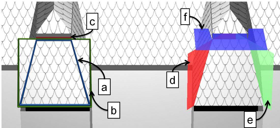
Figure 5.6: The *Join* rule has three successors : a) a joined face, b) an extruded rectangular quadrilateral including the joined face, and c) the top segment defined by  $v1$  and  $v2$  at  $heightExtrusion$  added to starting height. Clipping planes are defined around the joined face and applied on the extruded quadrilateral. The left d), right e) and top f) clipping planes are oriented according to the bissector angles.
