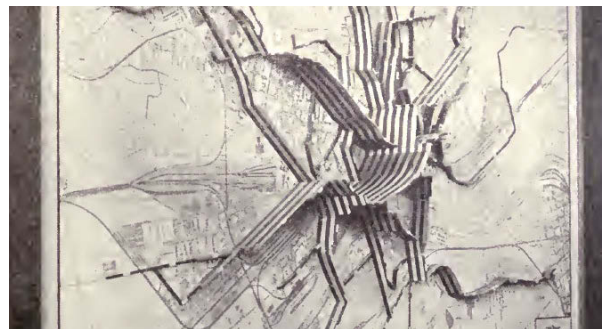
Figure 2.6: A map of the load of the street car network in Frankfurt a. M. from 1913.
