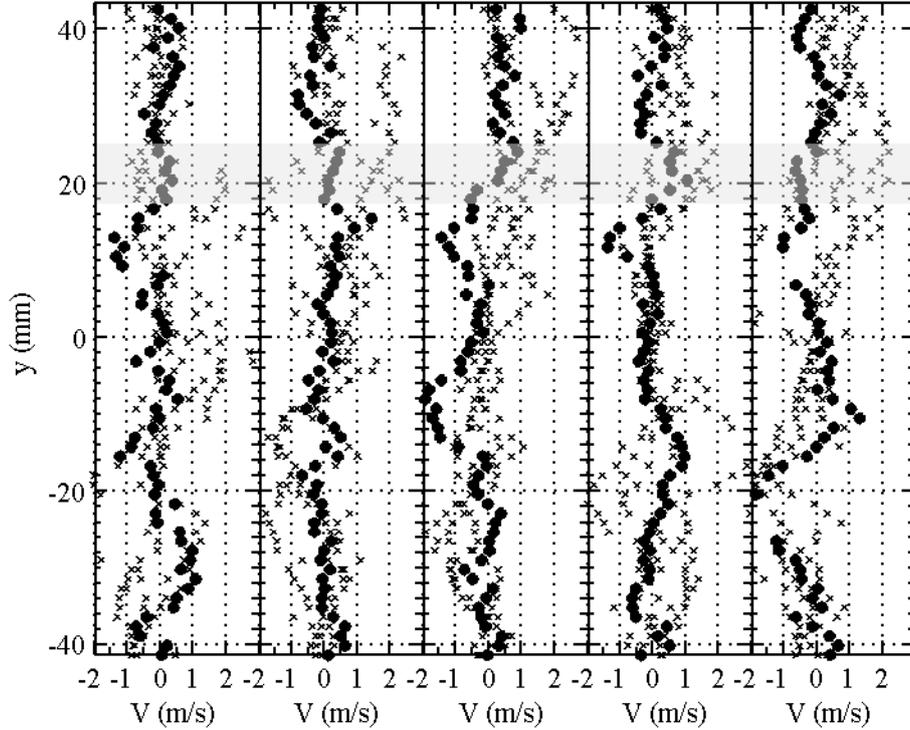
**Figure 6.12:** Mean (over 40 velocity fields  $\bar{I}$  PVC cycle) of vertical velocity components at the axial location of the spark before spark energy deposition;  $\times$  corresponds to non-igniting sparks and  $\bullet$  corresponds to successfully igniting spark; from left to right: test 1-5.
