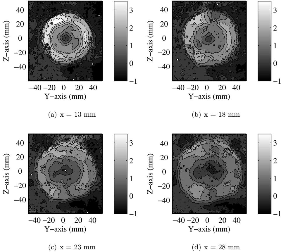
**Figure 5.16:** Radial velocity fields (m/s) for droplet flow at different axial locations inside the burner.
