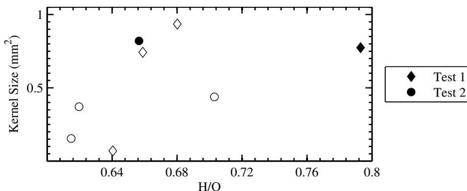
**Figure 9.27:** Size of the initial flame kernel as a function of mean H/O inside the kernel for sparks created at location ‘f’. Filled markers represent successful sparks and blank markers represent unsuccessful sparks.
