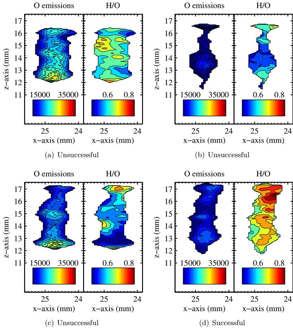
**Figure D.23:** Location *e*; Test#6, Analysis of 2D-LIPS experiments for (a) Spark#1, (b) Spark#2, and (c) Spark#3 which failed to ignite, and (d) Spark#4 which successfully ignited.
