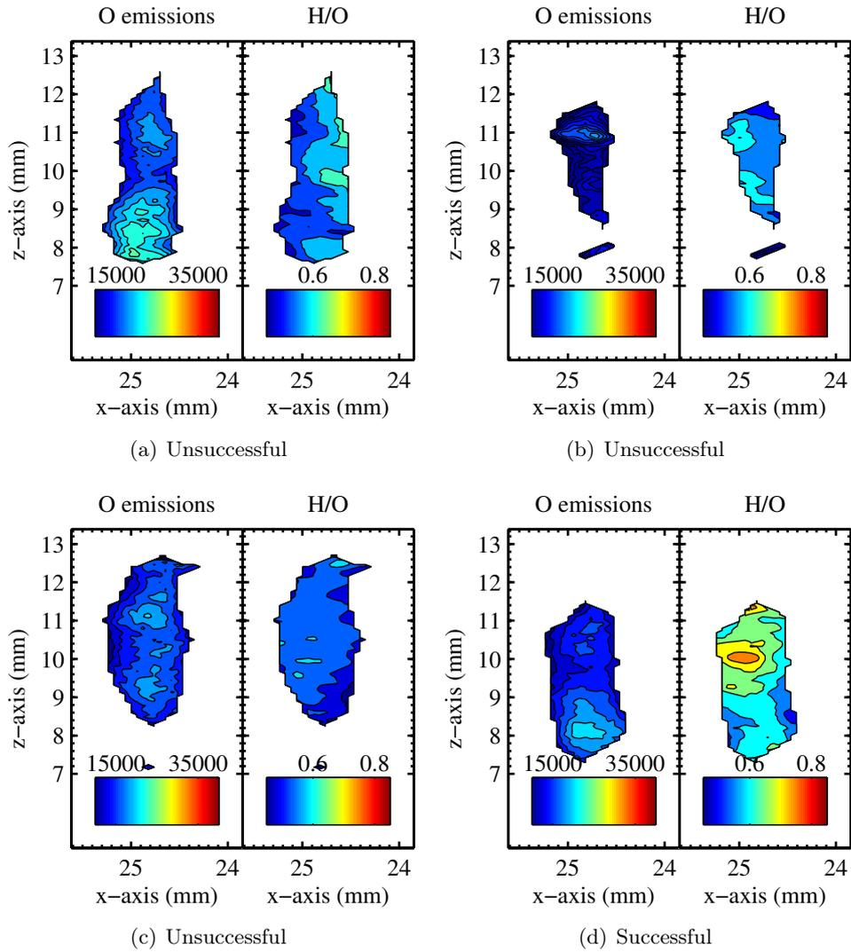
**Figure D.7:** Location b; Test#5, Analysis of 2D-LIPS experiments for (a) Spark#1, (b) Spark#2, and (c) Spark#3 which failed to ignite, and (d) Spark#4 which successfully ignited.
