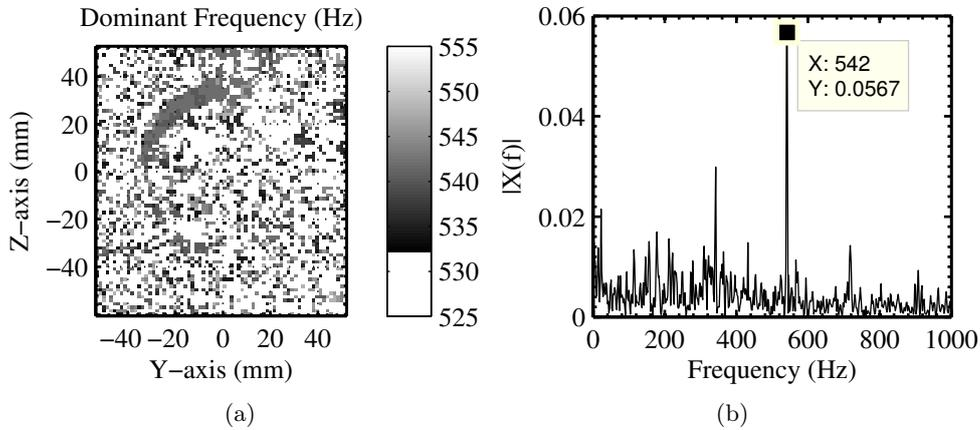
**Figure 5.21:** (a) Dominant frequencies inside the burner calculated using FFT of vertical velocity components; (b) Power spectral density as a function of wavelength at  $z = 28$  mm,  $y = -20$  mm, and an axial distance of 13 mm.
