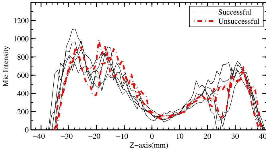
**Figure 9.17:** Radial profiles of mean Mie-scattering intensity (over 10 ms, before sparks) at axial location of the sparks created at location 'a'; Five successful and two unsuccessful sparks compared.
