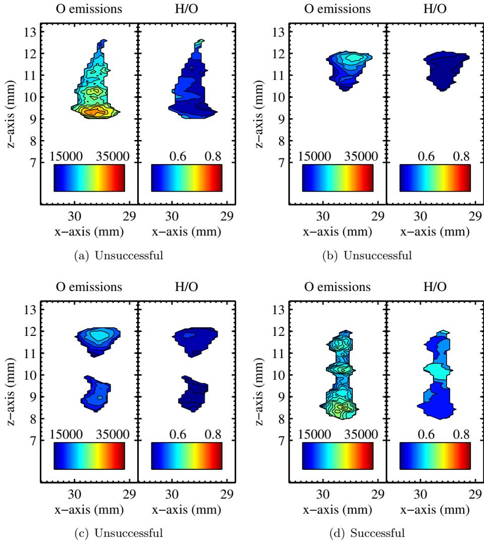
**Figure D.9:** Location c; Test#1, Analysis of 2D-LIPS experiments for (a) Spark#1, (b) Spark#2, and (c) Spark#3 which failed to ignite, and (d) Spark#4 which successfully ignited.
