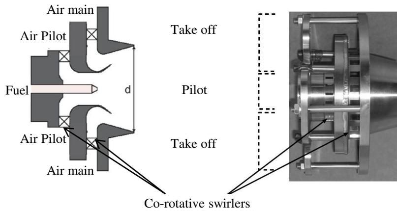
**Figure 3.4:** Schematic and image of the injector.
