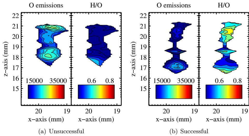
**Figure D.35:** Location *g*; Test#7, Analysis of 2D-LIPS experiments for (a) Spark#1 which failed to ignite, and (b) Spark#2 which successfully ignited.
