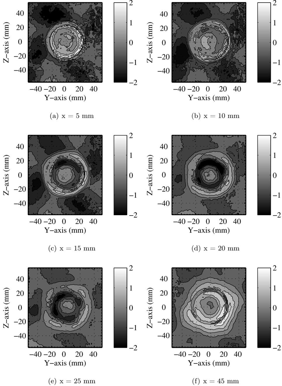
**Figure 5.7:** Radial velocity fields for different axial locations inside the burner.
