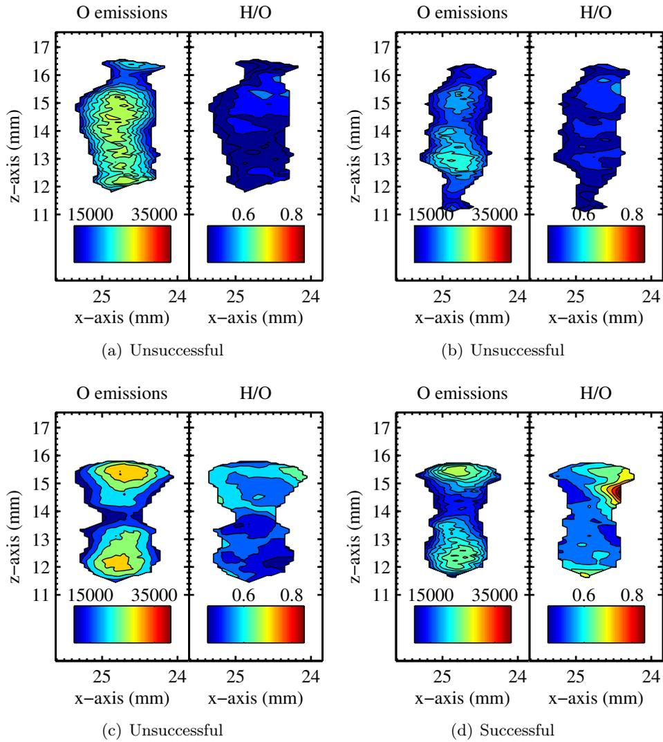
**Figure D.19:** Location *e*; Test#2, Analysis of 2D-LIPS experiments for (a) Spark#1, (b) Spark#2, and (c) Spark#3 which failed to ignite, and (d) Spark#4 which successfully ignited.
