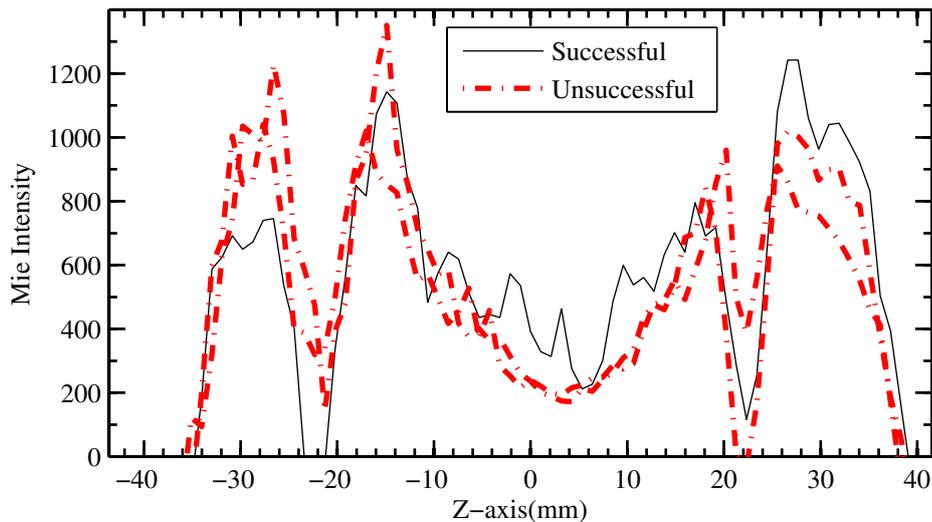
**Figure 9.31:** Radial profiles of mean Mie-scattering intensity (over 10 ms, before sparks) at axial location of the sparks created during Test#6 at location 'g'; Two unsuccessful and one successful sparks compared.
