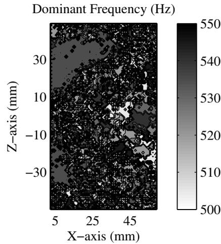
**Figure 5.23:** Dominant frequencies inside the burner calculated using FFT of vertical velocity components in the axial plane
