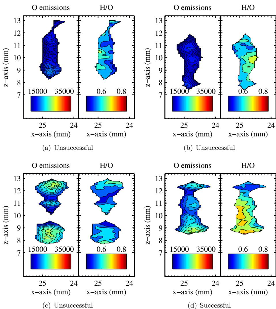
**Figure 9.4:** (a) Location b; Test#3, Analysis of 2D-LIPS experiments for Spark#1 which failed to ignite, (b) Location b; Test#3, Analysis of 2D-LIPS experiments for Spark#2 which failed to ignite, (c) Location b; Test#3, Analysis of 2D-LIPS experiments for Spark#3 which failed to ignite, (d) Location b; Test#3, Analysis of 2D-LIPS experiments for Spark#4 which successfully ignited.
