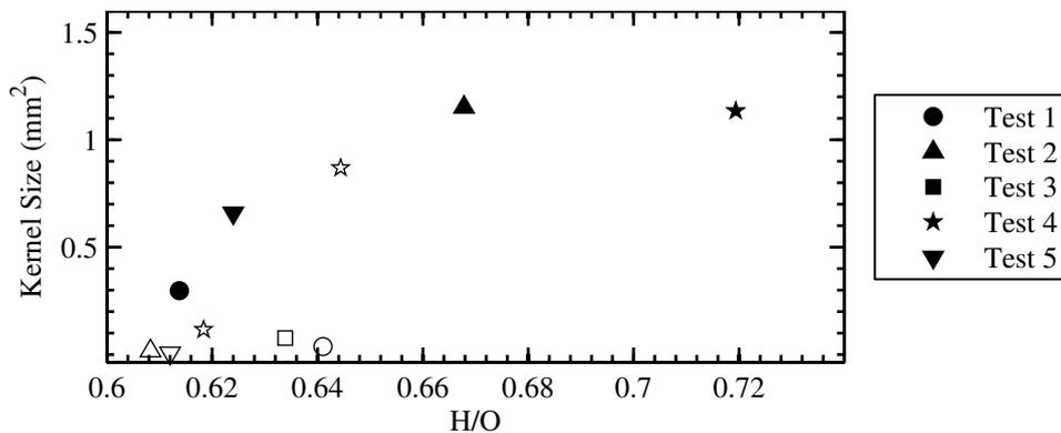
**Figure 9.19:** Size of the initial flame kernel as a function of mean  $H/O$  inside the kernel for sparks created at location ‘c’. Filled markers represent successful sparks and blank markers represent unsuccessful sparks.
