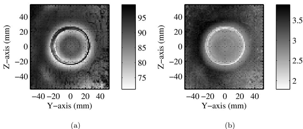
**Figure 5.9:** (a) Percentage of validated vectors for velocity field measurements in a transverse plane at an axial location of 25 mm.; (b) Mean of peak ratios during velocity field calculations for the transverse plane
