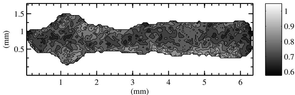
**Figure 7.15:** Typical intensity ratio ( $O/H$ ) obtained using bounding box approach; Images acquired with oxygen and hydrogen filters on ICCD cameras, laser-induced spark of energy 110.4 mJ created in a constant flow of methane-air mixture with equivalence ratio of 0.9.
