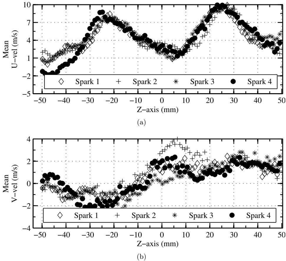
**Figure 9.11:** Location b; Test#3, Analysis of PIV measurements for four consecutive sparks. Spark#1, Spark#2 and Spark#3 failed to ignited while Spark#4 successfully ignited. Velocity profiles at the location of spark have been plotted as a function of radial distance; spark located at 8-13 mm. Profiles plotted using mean velocity fields (over 100 instantaneous fields equivalent to 10 ms) before the deposition of spark energy.
