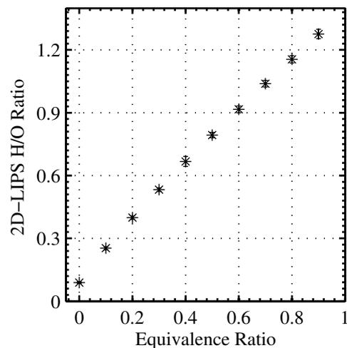
**Figure 8.11:** Variation of Hydrogen-Oxygen ratio obtained by 2D-LIPS as a function of equivalence ratio.
