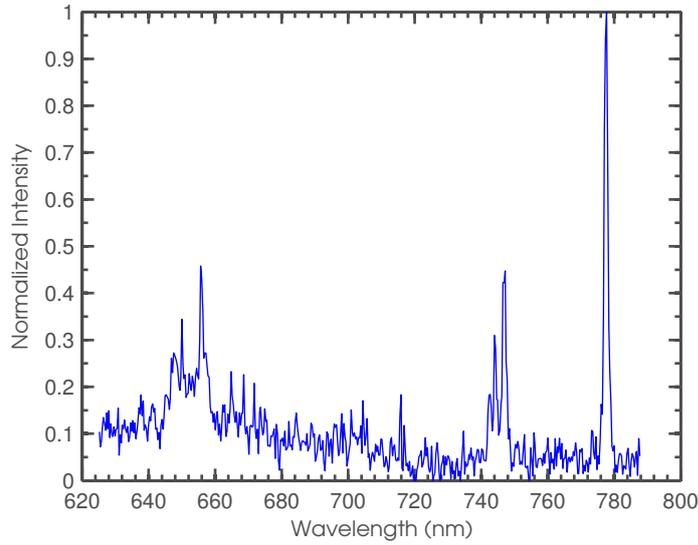
**Figure A.1:** *Spectral emission of a plasma created in air*
