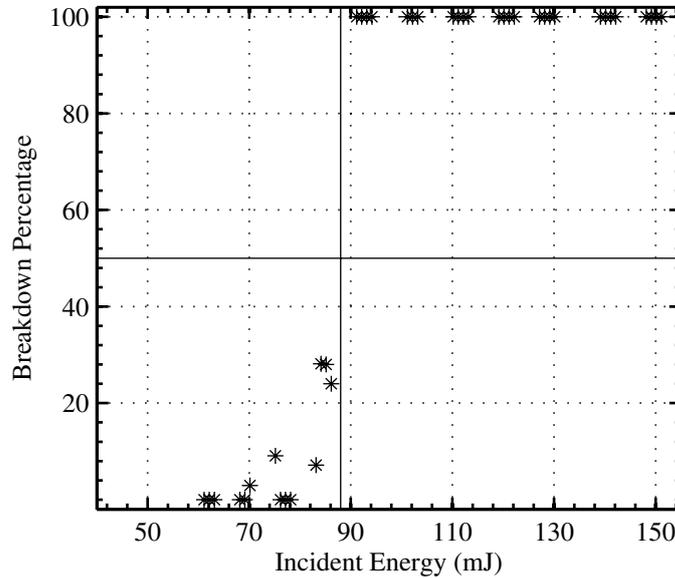
**Figure 7.2:** Probability of breakdown as a function of incident laser energy.
