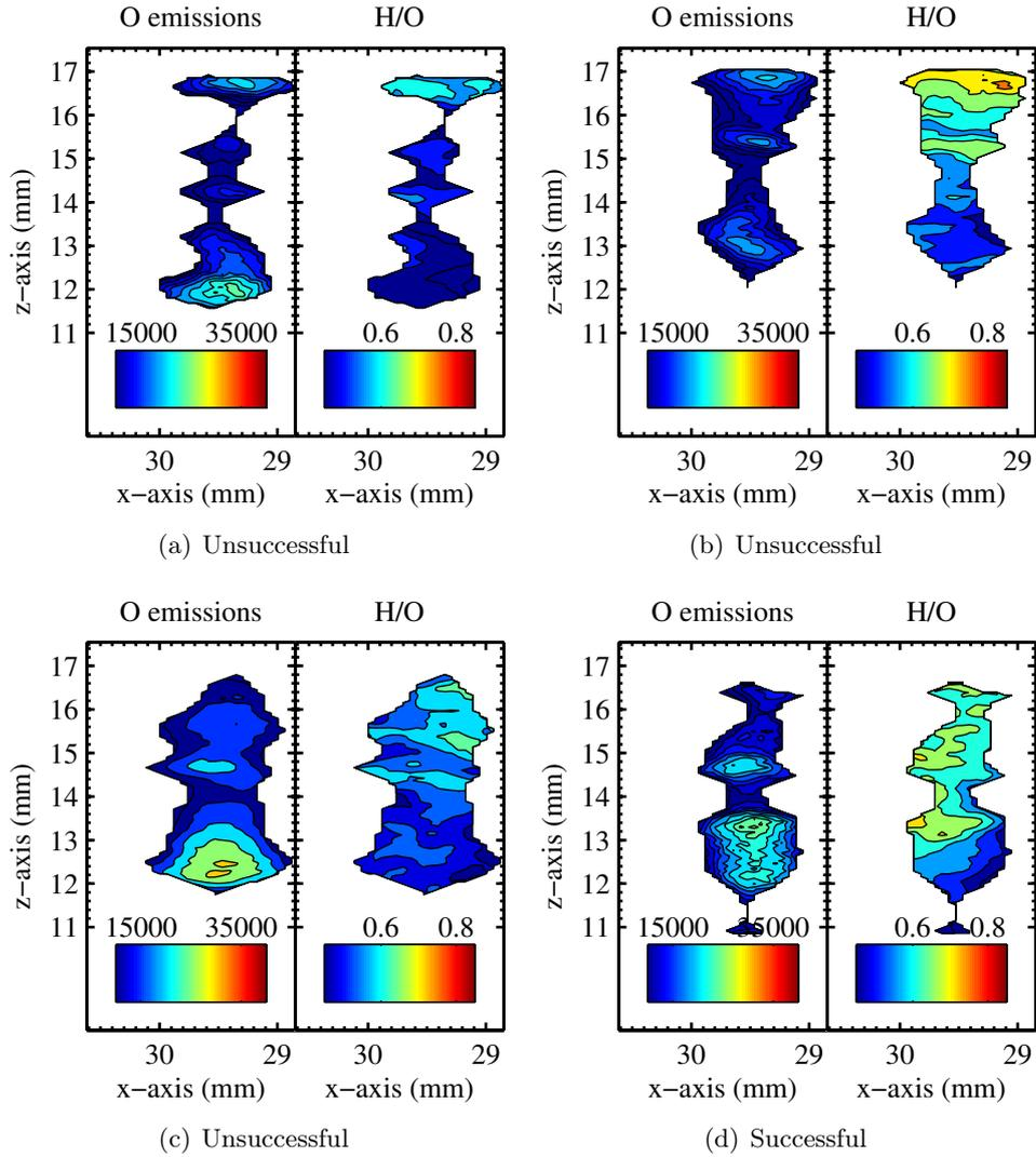
**Figure D.28:** Location *f*; Test#2, Analysis of 2D-LIPS experiments for (a) Spark#1, (b) Spark#2, and (c) Spark#3 which failed to ignite, and (d) Spark#4 which successfully ignited.
