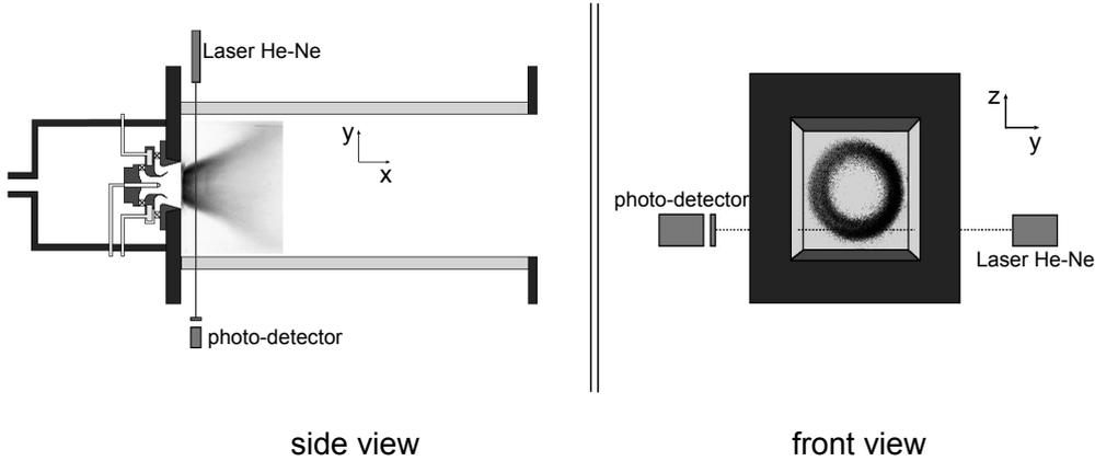
**Figure 2.1:** Position of the He-Ne laser with respect to spray in the combustion chamber.
