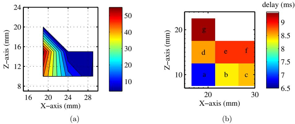
**Figure 9.1:** (a) Ignition probability (percentage) at few locations inside the chamber, (b) Locations of the laser-induced spark chosen for ignition experiments together with typical ignition delay.
