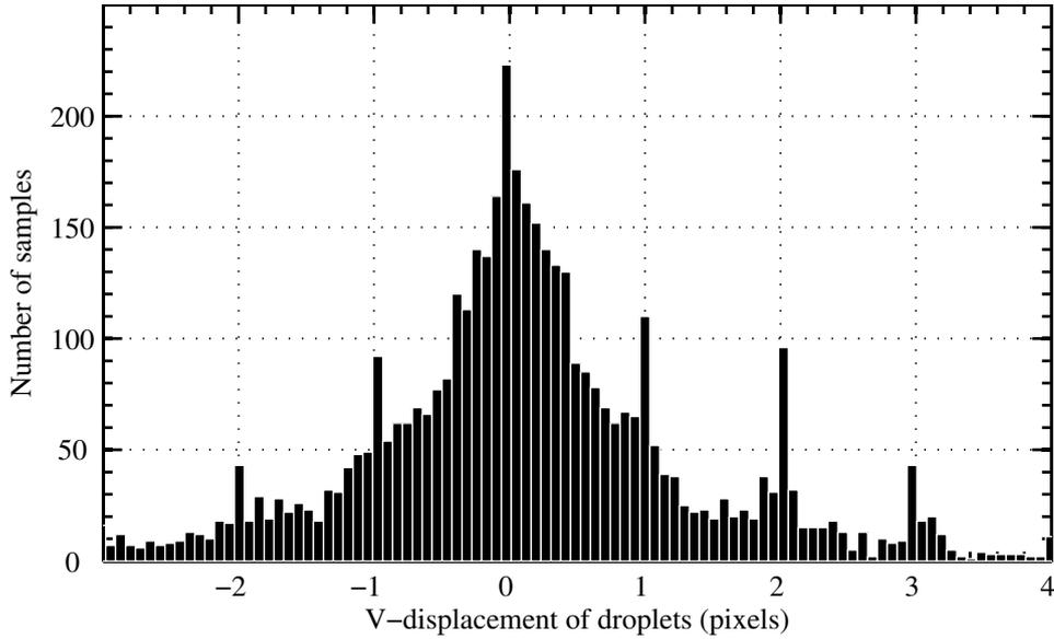
**Figure 5.20:** Histogram of vertical velocity component (displacement in pixels) at  $y = 0$  mm and  $z = 48$  mm for a transverse plane at an axial distance of 13 mm.
