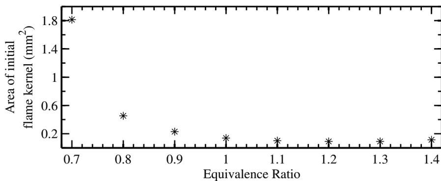
**Figure C.4:** Size of critical initial flame kernel as a function of equivalence ratio at the location of the spark.
