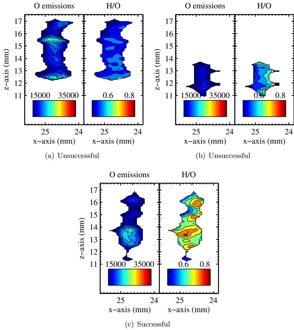
**Figure D.21:** Location e; Test#4, Analysis of 2D-LIPS experiments for (a) Spark#1, and (b) Spark#2 which failed to ignite, and (c) Spark#3 which successfully ignited.
