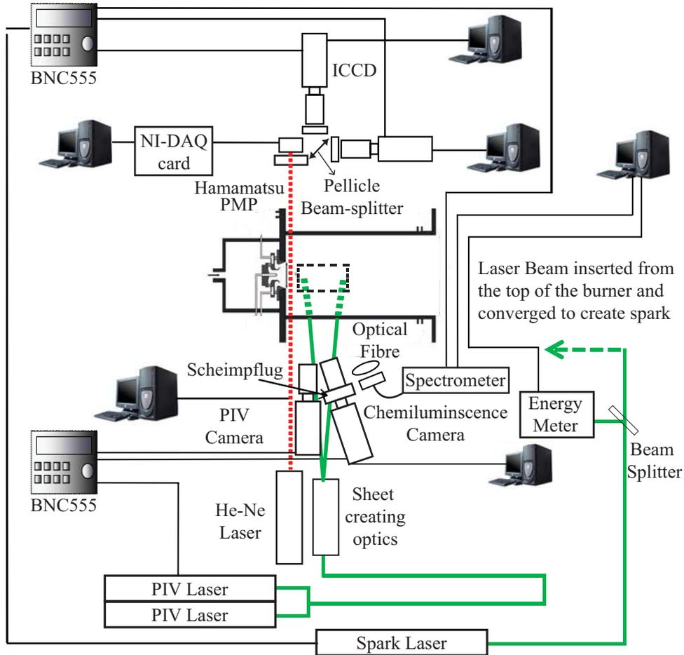
**Figure 3.7:** *Experimental setup for ignition experiments in two-phase, turbulent conditions.*
