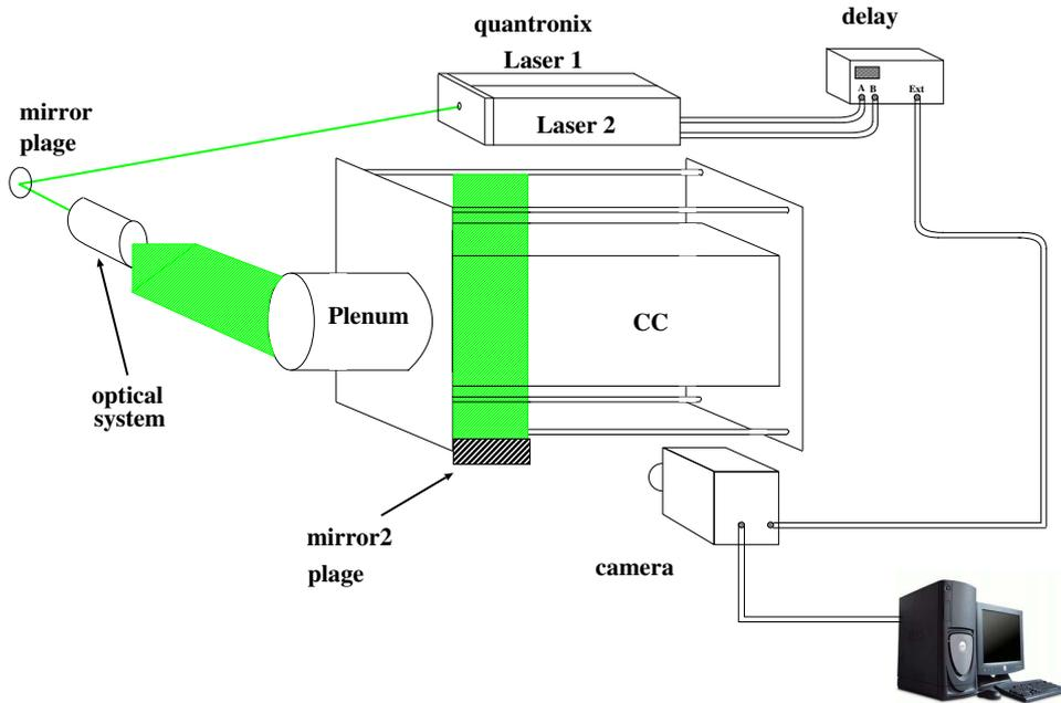
Figure 3.8: Schematic of HSPIV setup.
