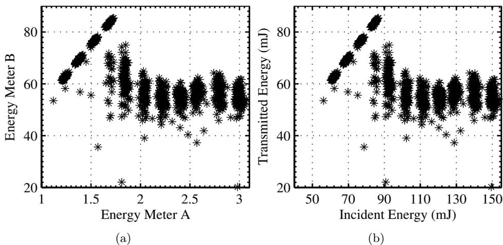
**Figure 7.1:** Laser Energy Measurements: (a) Variation of readings in the two energy meters; (b) Transmitted energy of the laser beam as a function of incident energy.
