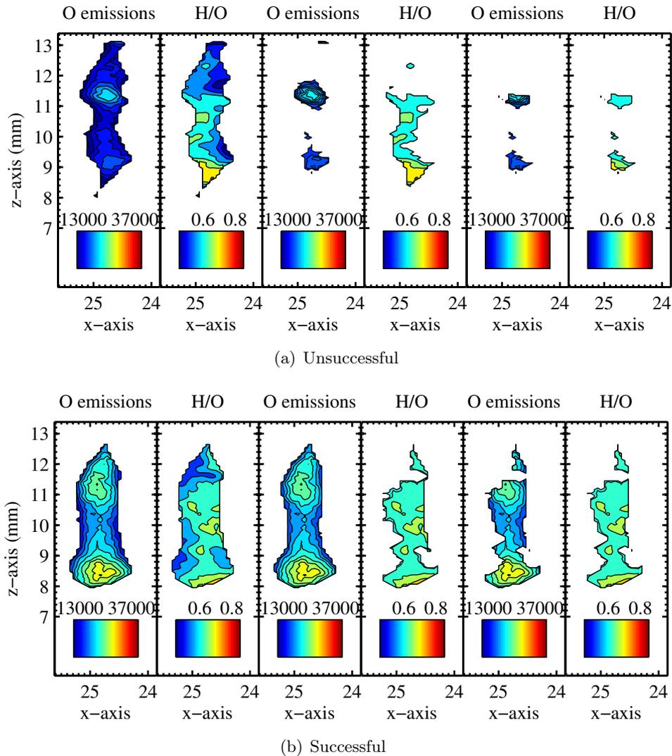
**Figure 9.7:** Location b; Test#1, Calculation of initial flame kernel size for (a) unsuccessful and (b) successful sparks, From left to right: Oxygen intensity and H/O ratio as obtained by 2D-LIPS, regions above thresholds separately applied to H/O and oxygen image intensity, and regions above both the thresholds.
