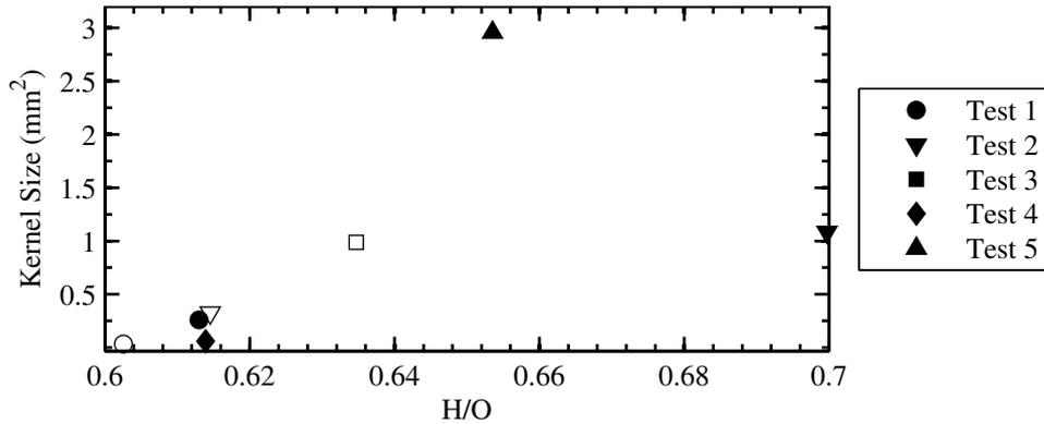
**Figure 9.15:** Size of the initial flame kernel as a function of mean H/O inside the kernel for sparks created at location ‘a’. Filled markers represent successful sparks and blank markers represent unsuccessful sparks.
