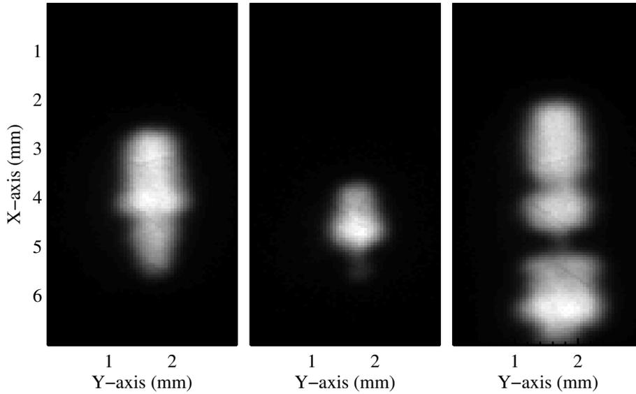
**Figure 7.6:** Typical images of laser-induced plasmas generated in presence of droplets. Images acquired through oxygen filter ( $\lambda = 780 \pm 10 \text{ nm}$ ), 1500 ns after the deposition of spark energy with a 90 ns exposure.
