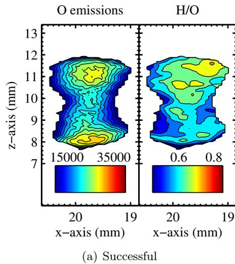
**Figure D.5:** Location a; Test#5, Analysis of 2D-LIPS experiments for (a) Spark#1 which successfully ignited.
