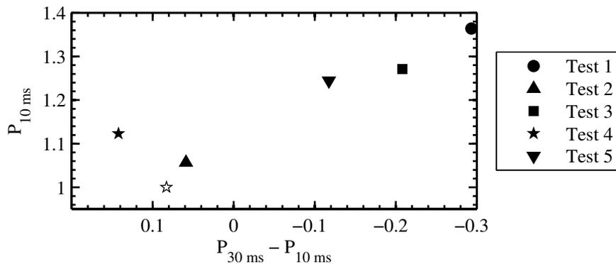
**Figure 9.21:** Strength of the PVC 10 ms before the spark as a function of decrease in the strength of PVC, for sparks created at location 'c'
