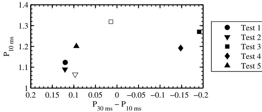
**Figure 9.18:** Strength of the PVC 10 ms before the spark as a function of decrease in the strength of PVC, for sparks created at location ‘a’
