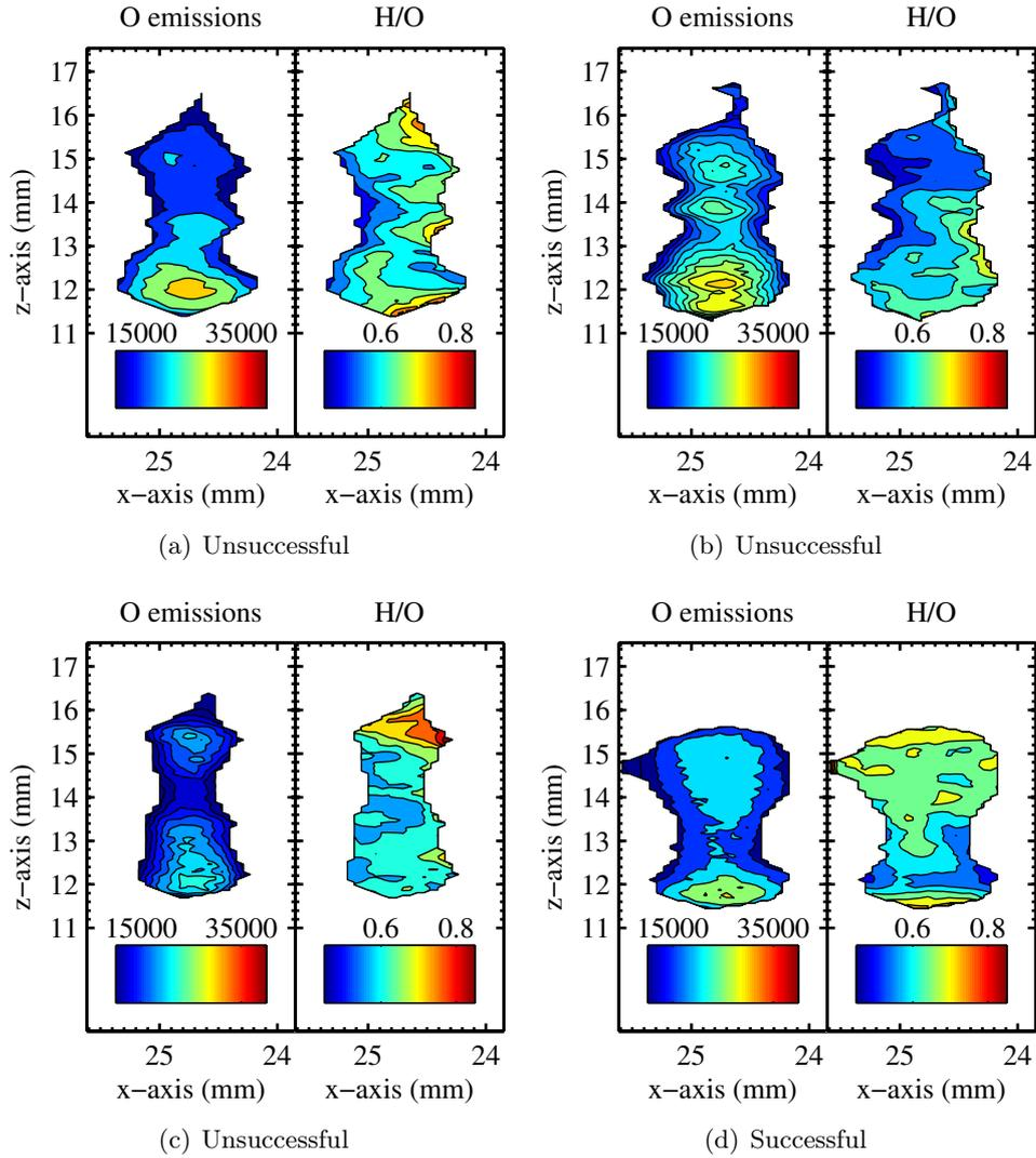
**Figure D.24:** Location *e*; Test#7, Analysis of 2D-LIPS experiments for (a) Spark#1, (b) Spark#2, and (c) Spark#3 which failed to ignite, and (d) Spark#4 which successfully ignited.
