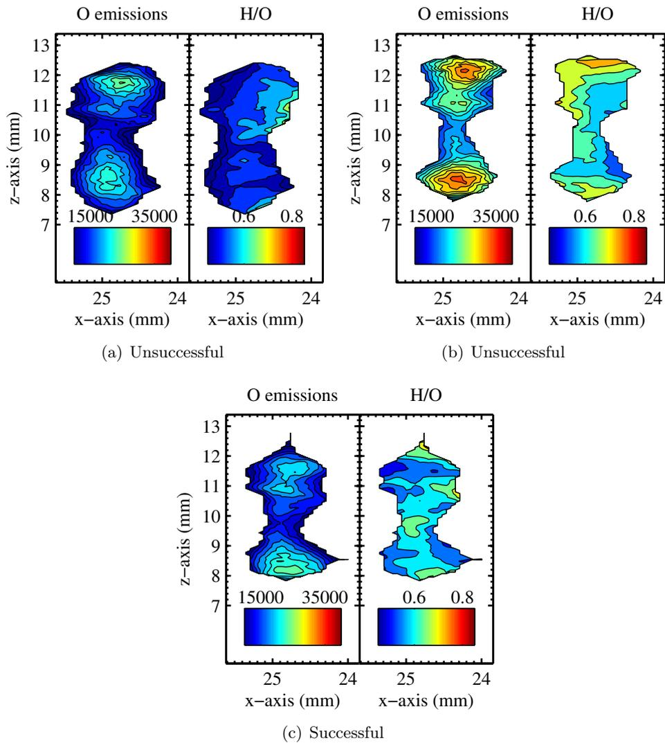
**Figure 9.6:** (a) Location b; Test#2, Analysis of 2D-LIPS experiments for Spark#1 which failed to ignite, (b) Location b; Test#2, Analysis of 2D-LIPS experiments for Spark#2 which failed to ignite, (c) Location b; Test#2, Analysis of 2D-LIPS experiments for Spark#3 which successfully ignited.
