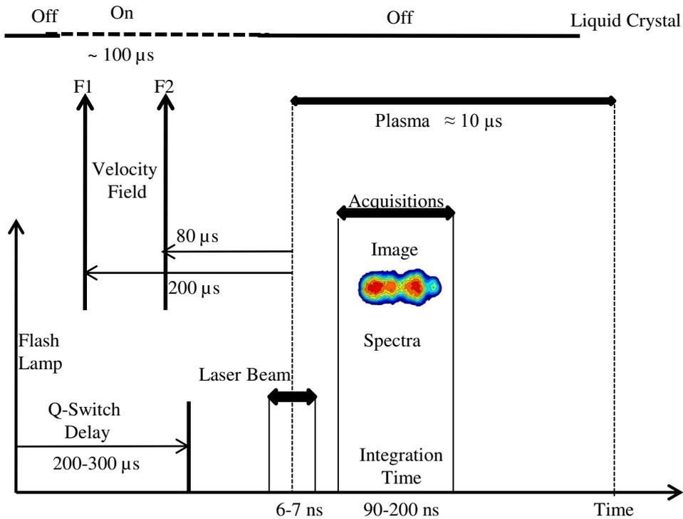
**Figure 3.3:** Chronology of the PIV measurements simultaneously with spectral and 2D-LIPS measurements
