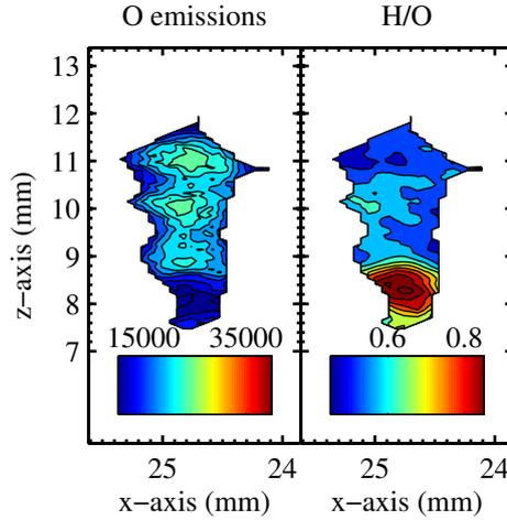
**Figure 9.5:** Location b; Test#7, Analysis of 2D-LIPS experiment where single shot ignition occurred.
