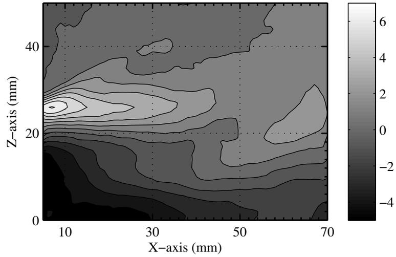
**Figure 5.25:** *Difference between aerodynamic and droplets' velocity fields in an axial plane.*
