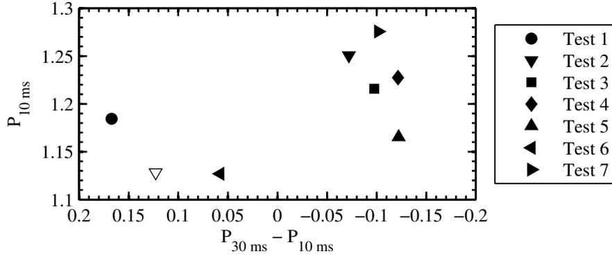
**Figure 9.14:** Strength of the PVC 10 ms before the spark as a function of decrease in the strength of PVC, for sparks created at location ‘b’
