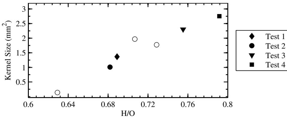
**Figure 9.22:** Size of the initial flame kernel as a function of mean  $H/O$  inside the kernel for sparks created at location 'd'. Filled markers represent successful sparks and blank markers represent unsuccessful sparks.
