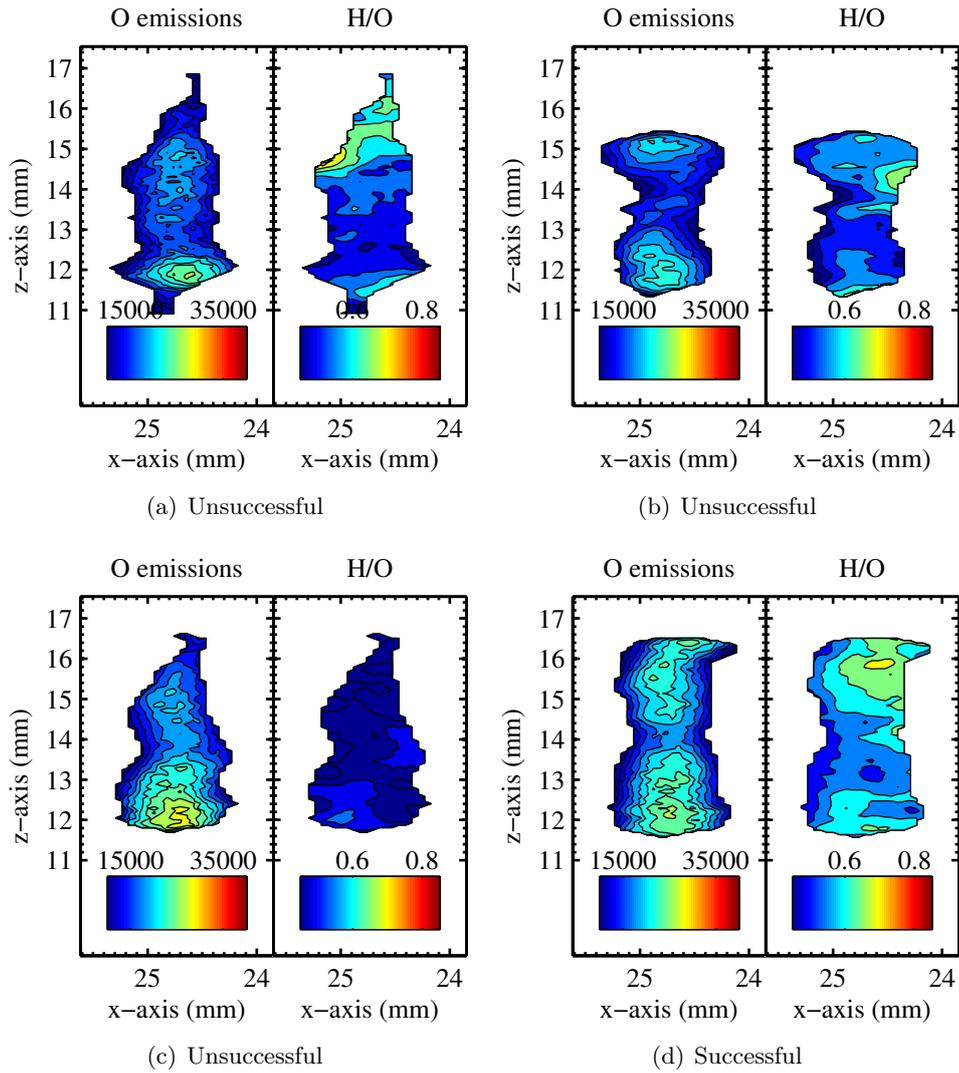
**Figure D.25:** Location *e*; Test#8, Analysis of 2D-LIPS experiments for (a) Spark#1, (b) Spark#2, and (c) Spark#3 which failed to ignite, and (d) Spark#4 which successfully ignited.
