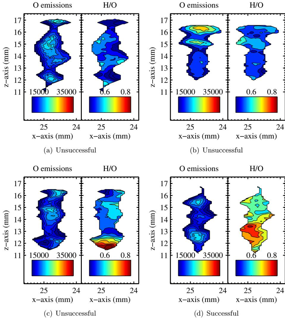
**Figure D.18:** Location e; Test#1, Analysis of 2D-LIPS experiments for (a) Spark#1, (b) Spark#2, and (c) Spark#3 which failed to ignite, and (d) Spark#4 which successfully ignited.
