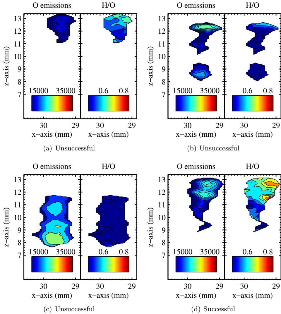
**Figure D.10:** Location *c*; Test#2, Analysis of 2D-LIPS experiments for (a) Spark#1, (b) Spark#2, and (c) Spark#3 which failed to ignite, and (d) Spark#4 which successfully ignited.
