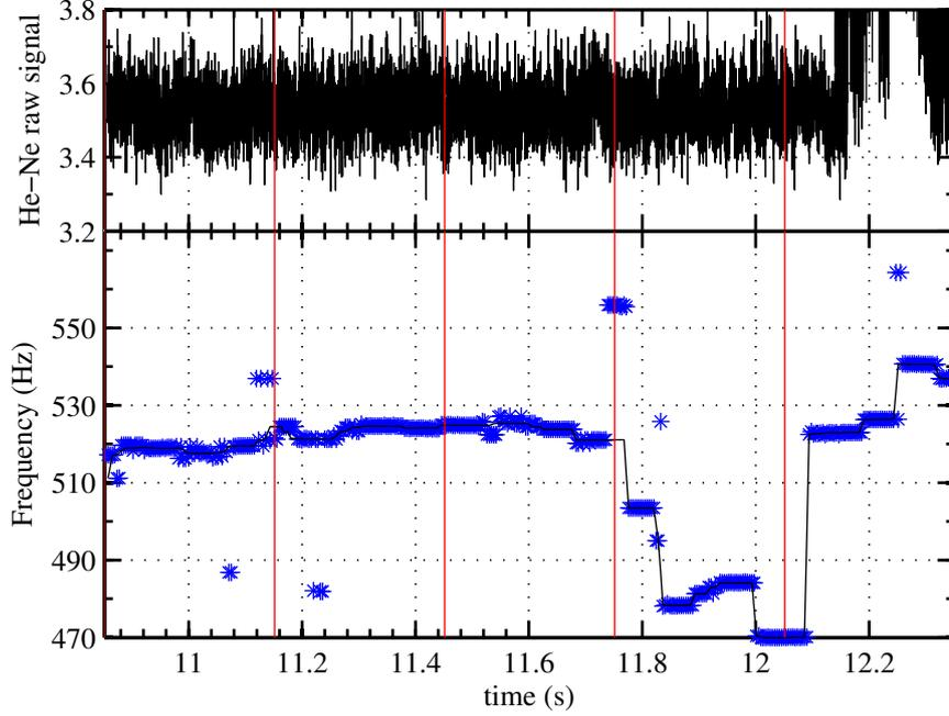
**Figure 6.6:** Temporal variation of PVC frequency (blue-bottom) and variation of He-Ne transmitted energy signal (black-top); red lines indicate locations of sparks, last spark corresponding to igniting spark.
