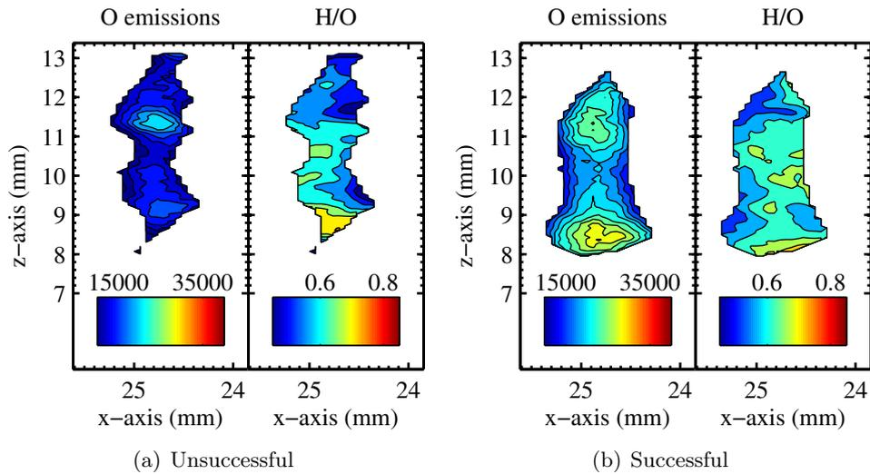
**Figure 9.3:** (a) Location b; Test#1, Analysis of 2D-LIPS experiments for Spark#1 which failed to ignite, (b) Location b; Test#1, Analysis of 2D-LIPS experiments for Spark#2 which successfully ignited.
