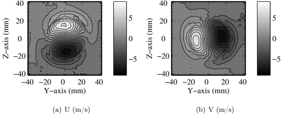
**Figure 5.6:** Mean  $U$  (axial) and  $V$  (vertical) components in transverse planes at an axial distance of 25 mm, Mean calculated over 10000 velocity fields (0.5 s).
