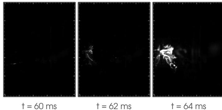
**Figure 6.17:** Chemiluminescence images acquired at 10 kHz, at respectively 60, 62, and 64 ms after the igniting spark.
