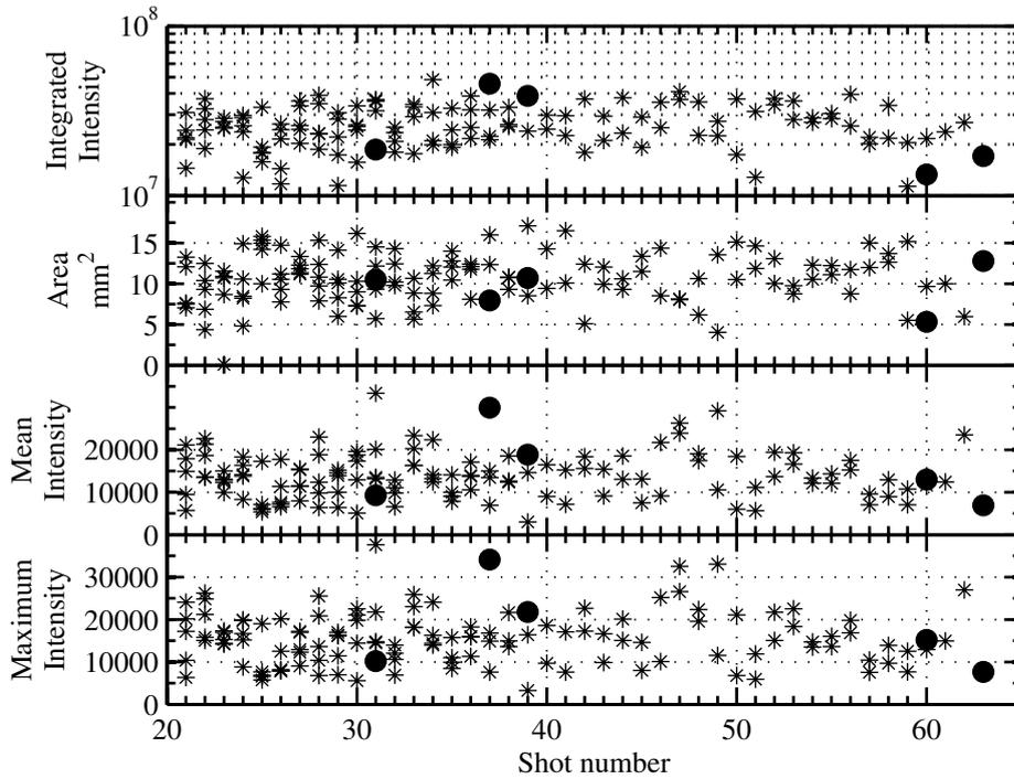
**Figure 6.3:** From top to bottom: Integrated spark intensity, Area of the laser induced spark, Mean intensity of the laser induced spark, Maximum intensity of the laser induced spark; Circles correspond to successful ignition and stars correspond to unsuccessful ignition attempts.
