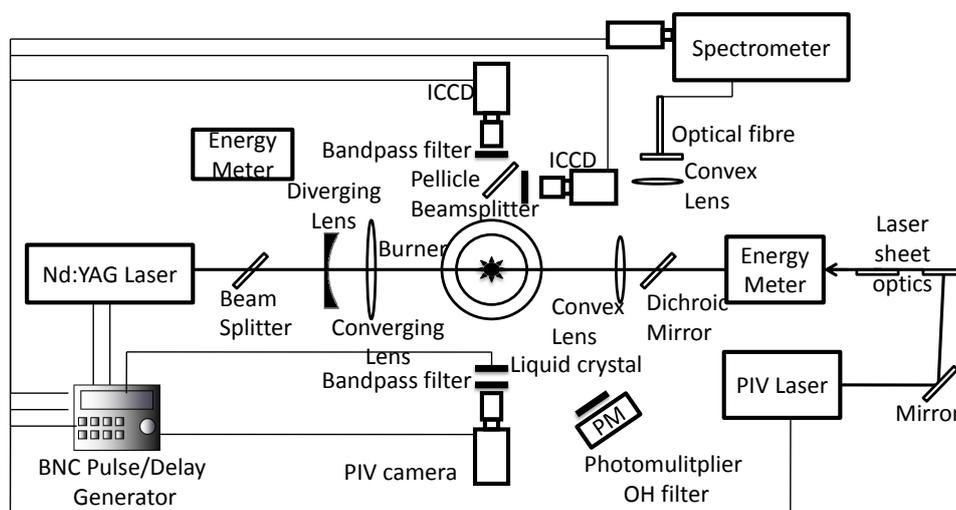
**Figure 3.2:** *Experimental setup for simultaneous 2D-LIPS and PIV measurements*
