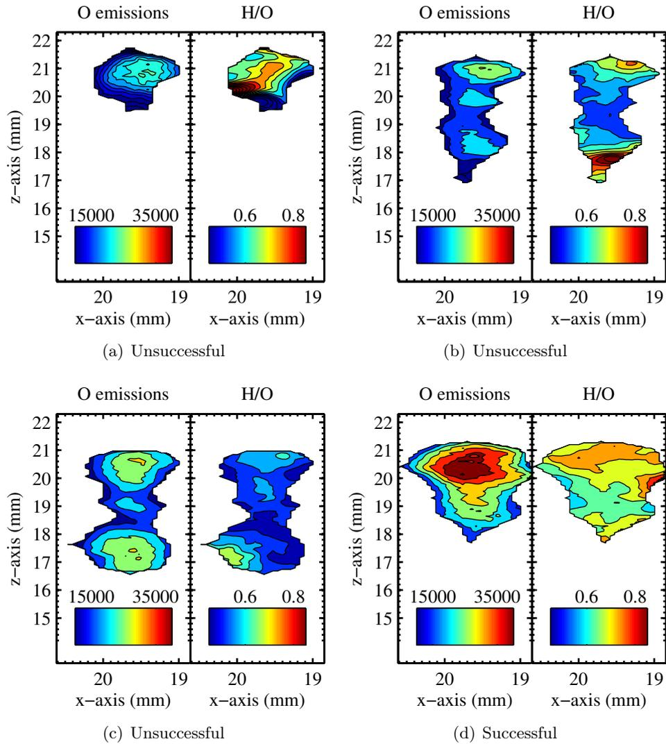
**Figure D.29:** Location g; Test#1, Analysis of 2D-LIPS experiments for (a) Spark#1, (b) Spark#2, and (c) Spark#3 which failed to ignite, and (d) Spark#4 which successfully ignited.
