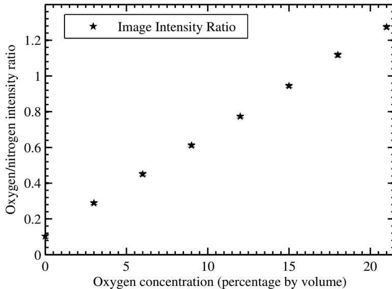
**Figure 8.2:** Evolution of the image intensity ratio of oxygen over nitrogen emissions as a function of the oxygen concentration.
