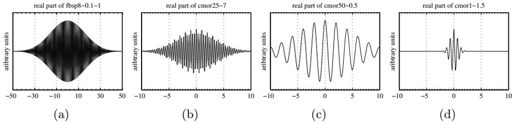
**Figure 4.2:** Typical mother wavelet for Frequency-B Spline (a), Complex Morlet 1-1.5 (b), Complex Morlet 50-0.5 (c) and Complex Morlet 25-7 (d).
