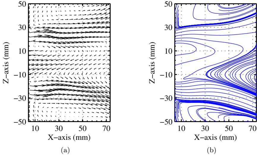
**Figure 5.3:** Velocity vectors (a) and streamlines (b), representing the mean aerodynamic flow inside the burner, mean calculated over 10000 velocity fields (1 s).
