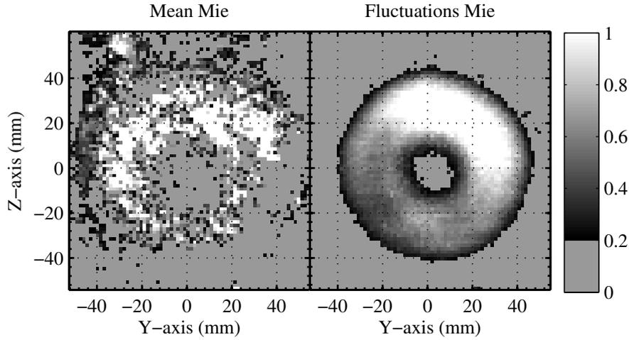
**Figure 5.15:** Mean and fluctuations (over 1 s) of Mie-scattering from fuel droplets in a transverse plane at an axial distance of 23 mm.
