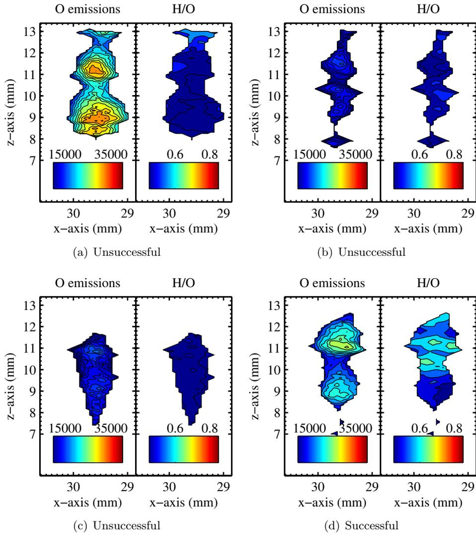
**Figure D.13:** Location c; Test#5, Analysis of 2D-LIPS experiments for (a) Spark#1, (b) Spark#2, and (c) Spark#3 which failed to ignite, and (d) Spark#4 which successfully ignited.
