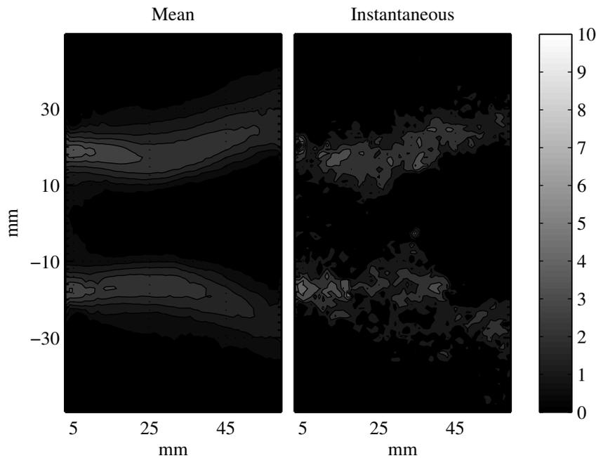
**Figure 6.11:** Mean (over 100 ms) and instantaneous axial velocity fields calculated using the Mie-scattering images of the droplets
