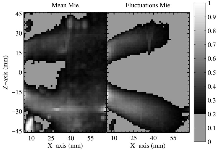
**Figure 5.13:** Mean and fluctuations of Mie-scattering intensity in an axial plane, averaged over 1 s.
