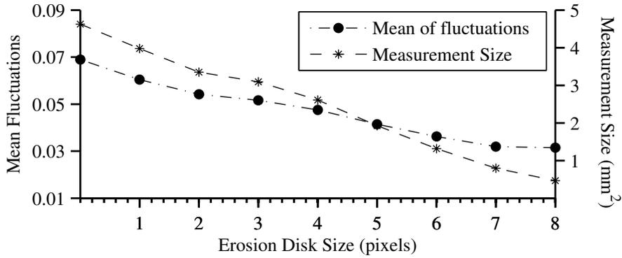
**Figure 7.19:** Variation of standard deviation in calculations of intensity ratio and the number of points/pixels where information is available with size of erosion disk for a fixed filter size of 4 and an intensity threshold of 33%.
