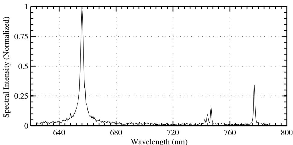
**Figure 7.7:** Example of single shot spectral emission obtained in methane-air mixture with an equivalence ratio of 0.6, for an integration time of 90 ns at a delay of 1500 ns from plasma formation.
