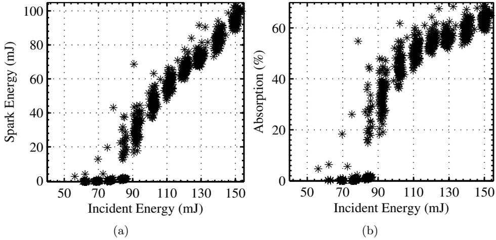
**Figure 7.3:** *Laser Energy Measurements: (a) Spark Energy as a function of incident energy, and (b) absorption percentage of the laser beam energy as a function of incident energy.*
