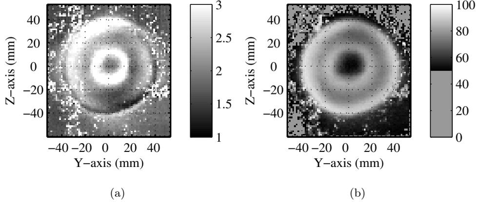
**Figure 5.18:** (a) Mean of peak ratios during correlation of images for velocity field calculations; mean calculated using only the validated vectors; (b) Percentage of validated vectors at each location inside the burner.
