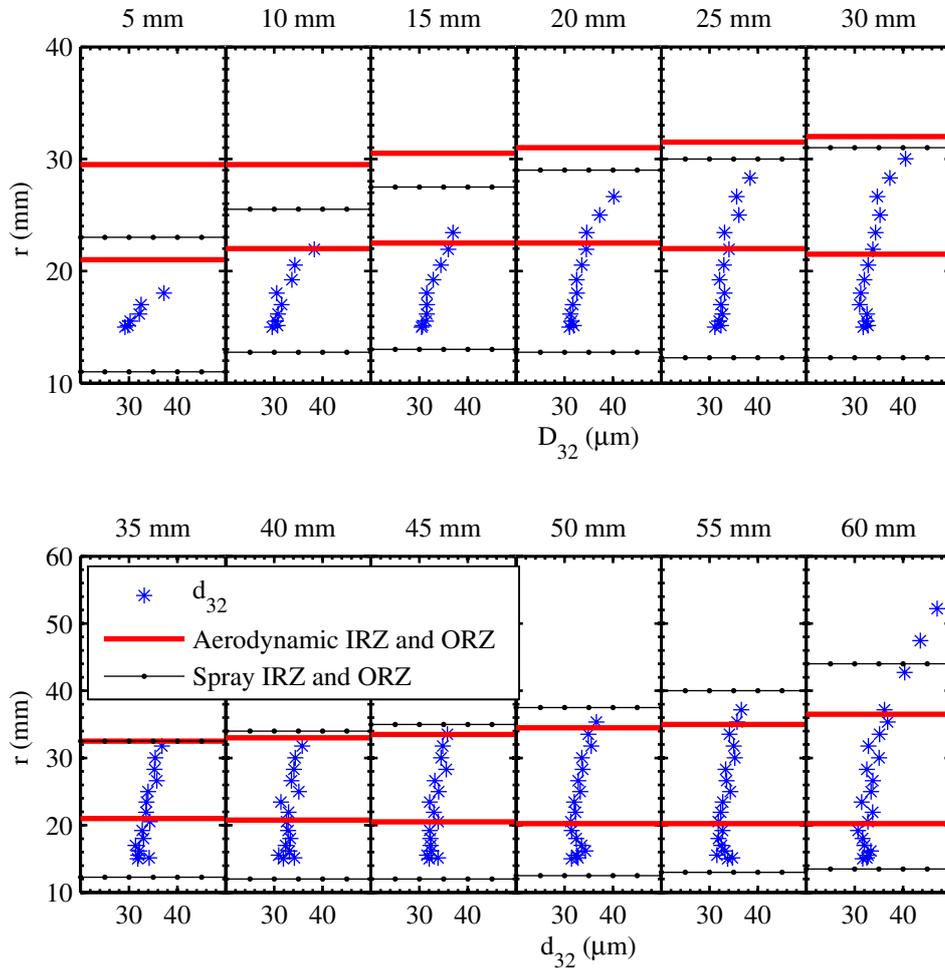
**Figure 5.12:** Sauter Mean diameter of droplets coming out of injector at various axial locations as a function of radial location, Aerodynamic and spray recirculation zone also simultaneously plotted.
