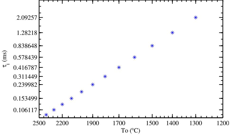
**Figure C.1:** Ignition delay,  $\tau_i$  (ms) as a function of initial temperature,  $T_o$  ( $^{\circ}$ C) for methane-air mixture.
