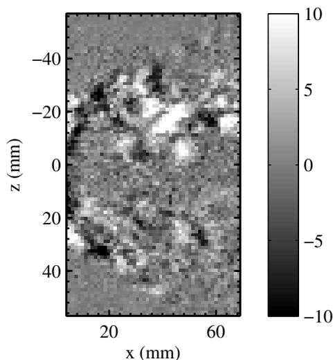
**Figure 6.14:** Typical magnitude of the eigenvalues corresponding to the PVC mode as obtained from DMD.
