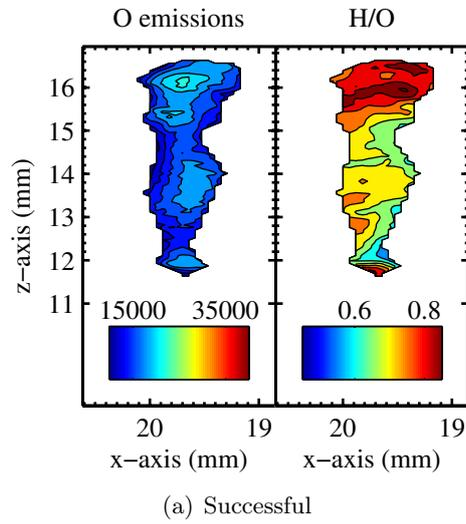
**Figure D.16:** Location *d*; Test#3, Analysis of 2D-LIPS experiments for (a) Spark#1 which successfully ignited.
