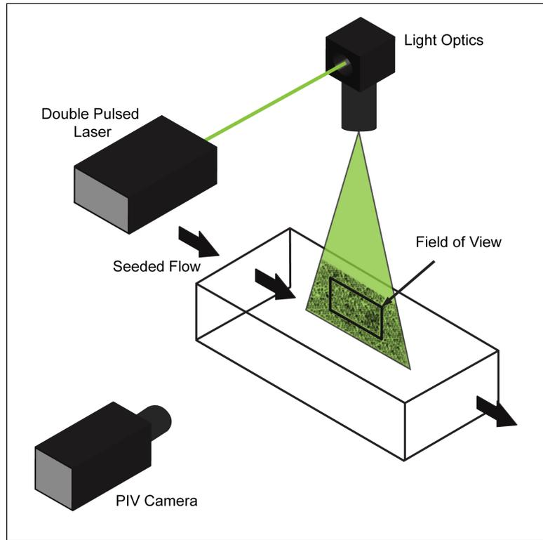
**Figure 2.3:** *Typical setup for PIV measurements.*
