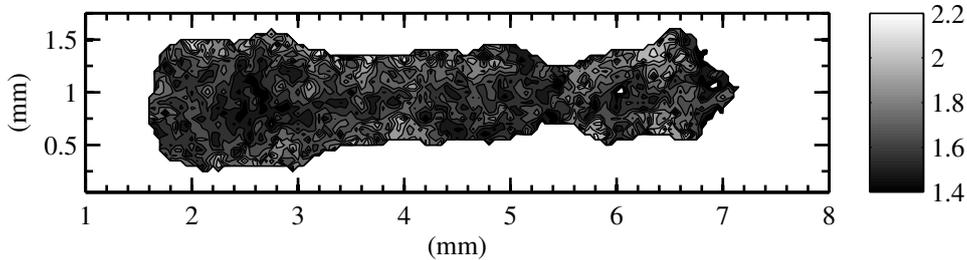
**Figure 7.12:** Intensity ratio of images obtained after image correlation using PIV measurements; Images acquired with nitrogen filters on both cameras, laser-induced spark of energy 94.8 mJ created in a constant flow of air.
