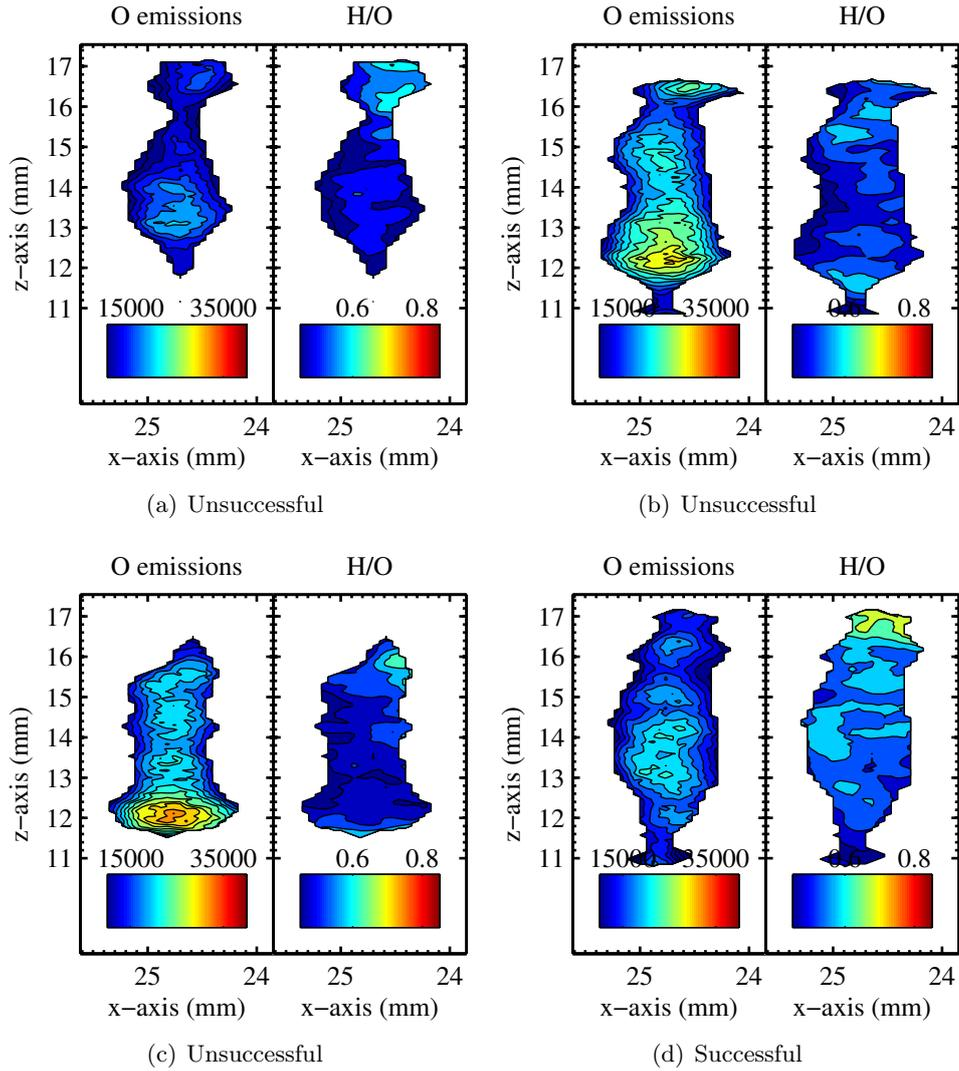
**Figure D.26:** Location *e*; Test#9, Analysis of 2D-LIPS experiments for (a) Spark#1, (b) Spark#2, and (c) Spark#3 which failed to ignite, and (d) Spark#4 which successfully ignited.
