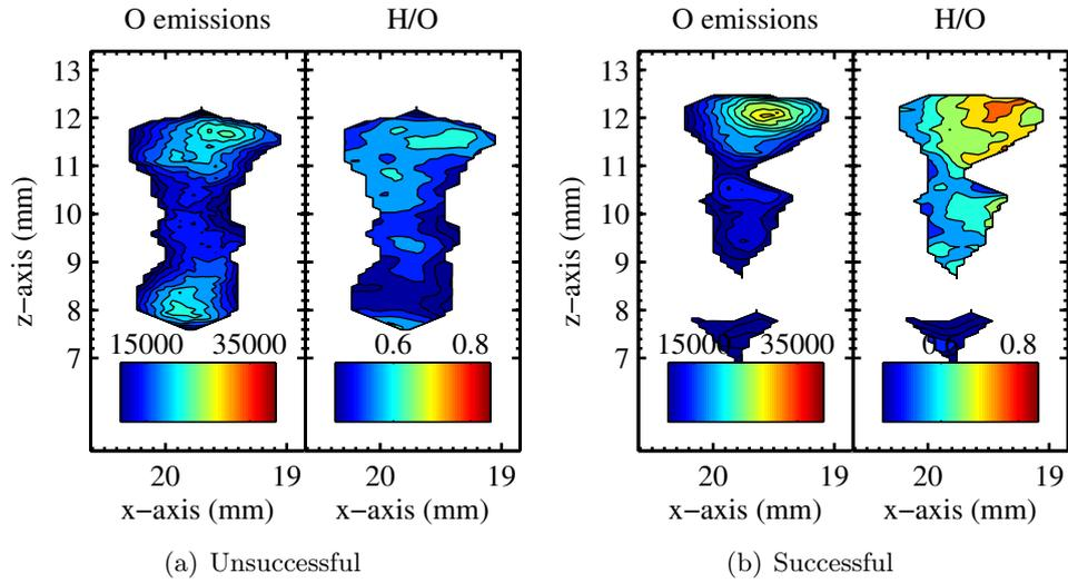
Figure D.2: Location a; Test#2, Analysis of 2D-LIPS experiments for (a) Spark#1 which failed to ignite, and (b) Spark#2 which successfully ignited.
