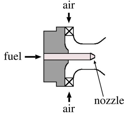
**Figure 3.5:** Schematic of Pilot stage of injector system
