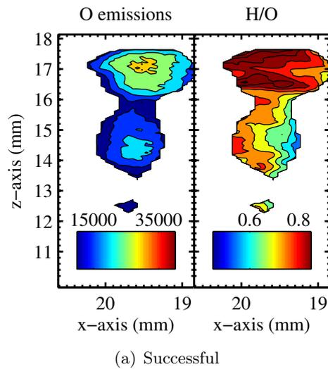
**Figure D.17:** Location *d*; Test#4, Analysis of 2D-LIPS experiments for (a) Spark#1 which successfully ignited.
