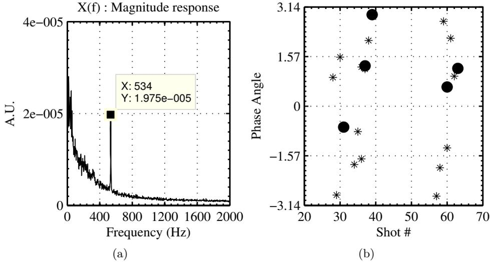
**Figure 6.5:** (a) Fast fourier transform of the helium neon laser transmitted energy measurements.; and, (b) Variation of phase of PVC at the times of spark, obtained from Helium Neon measurements; Circles correspond to successful ignition and stars correspond to unsuccessful ignition attempts.
