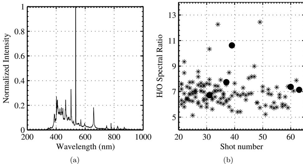
**Figure 6.4:** (a) Typical Spectral measurements from a laser induced spark; and, (b) Hydrogen to oxygen spectral ratio; Circles correspond to successful ignition and stars correspond to unsuccessful ignition attempts.
