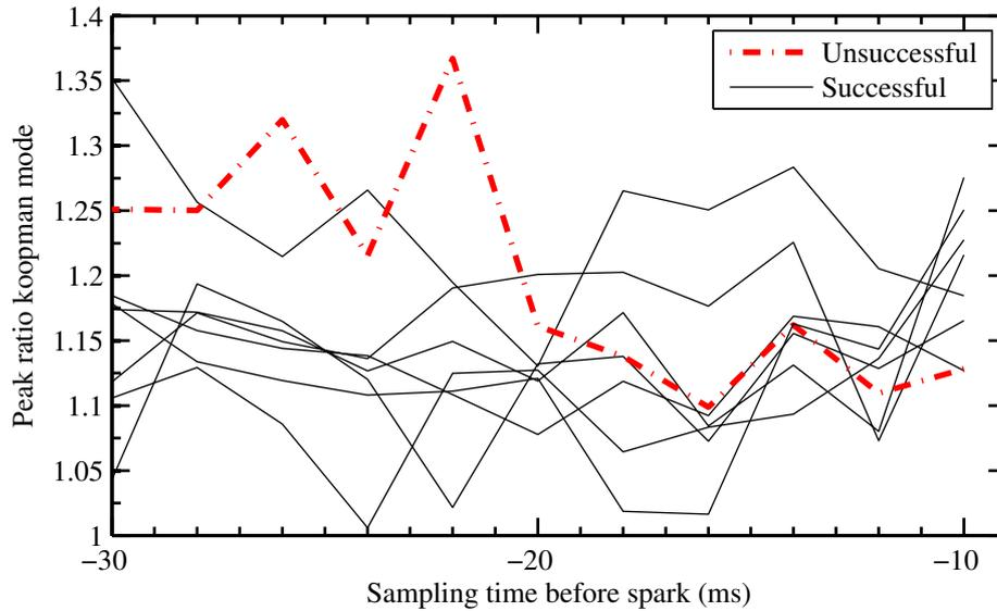
**Figure 9.13:** Variation of PVC strength before sparks for 7 igniting and 1 failed sparks.
