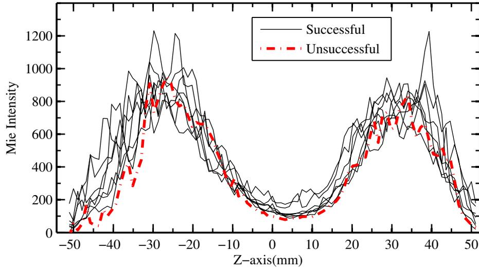
**Figure 9.9:** Radial profiles of mean Mie-scattering intensity (over 10 ms, before sparks) at axial location of the sparks created at location 'b'; Seven successful and one unsuccessful sparks compared.
