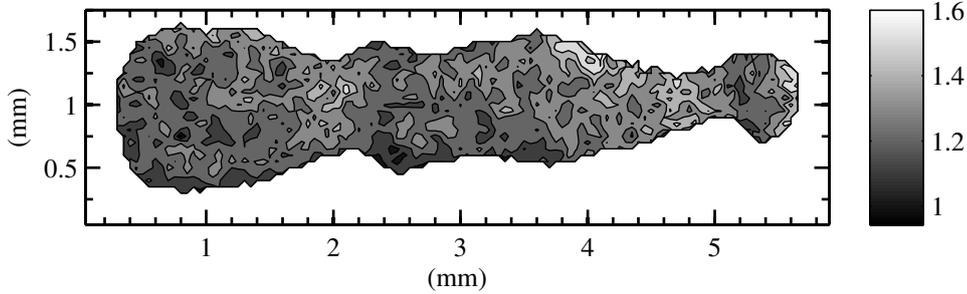
**Figure 7.14:** Typical intensity ratio ( $O/N$ ) obtained using image correlation through a grid image and image processing with Flow Manager; Images acquired with oxygen and nitrogen filters on ICCD cameras, laser-induced spark of energy 117 mJ created in a constant flow of air.
