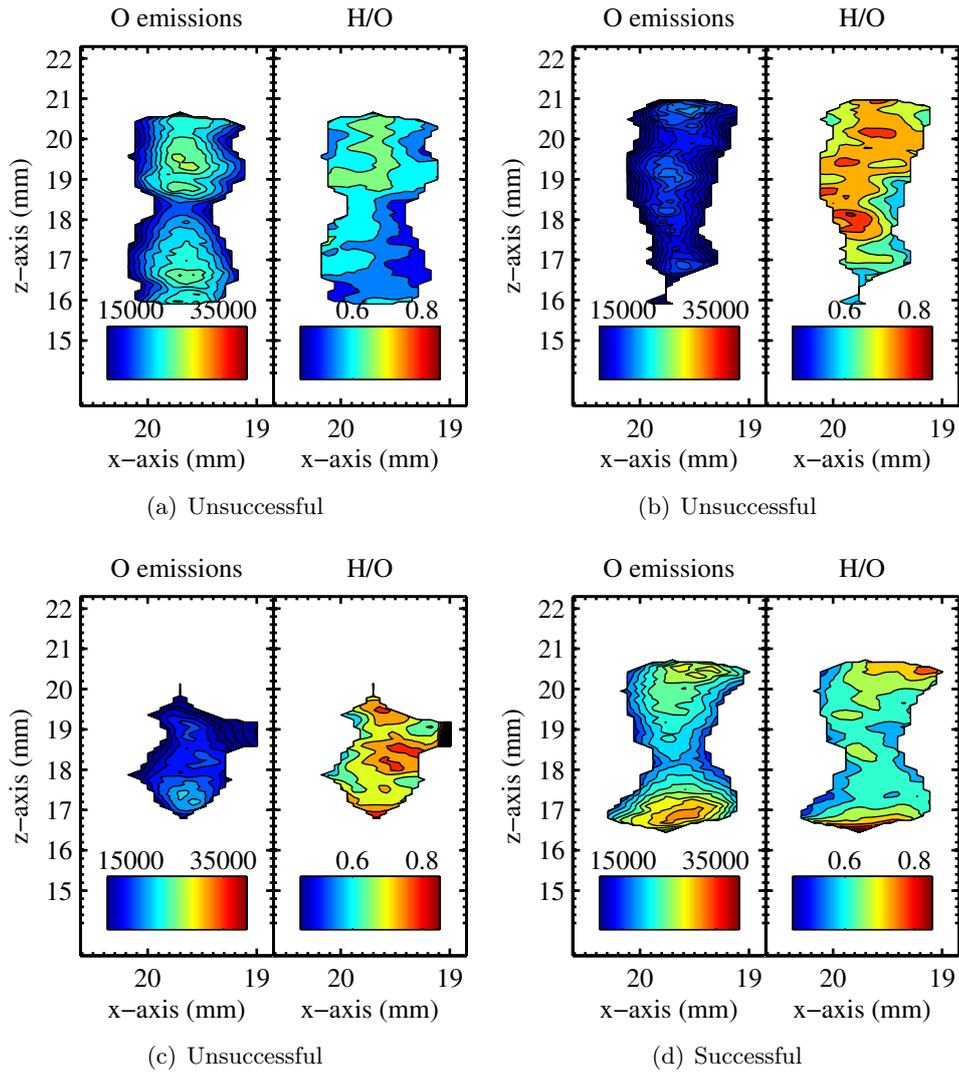
**Figure D.33:** Location *g*; Test#5, Analysis of 2D-LIPS experiments for (a) Spark#1, (b) Spark#2, and (c) Spark#3 which failed to ignite, and (d) Spark#4 which successfully ignited.
