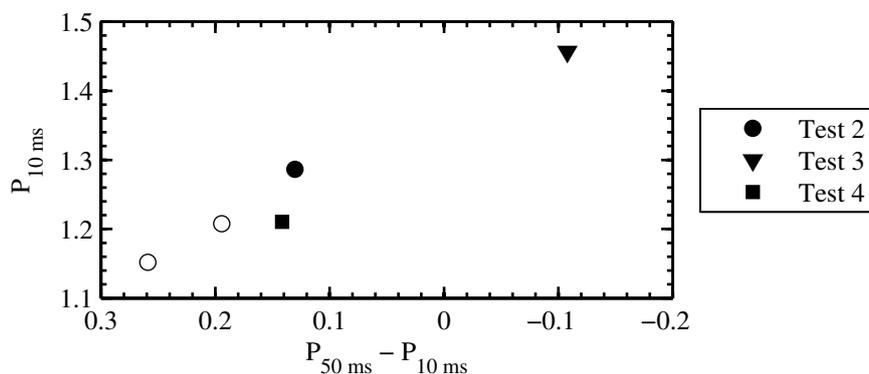
**Figure 9.24:** Strength of the PVC 10 ms before the spark as a function of decrease in the strength of PVC, for sparks created at location 'd'
