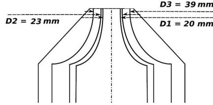
**Figure 3.1:** Schematic view of the co-flow nozzle used for calibration and validation of the 2D-LIPS technique.
