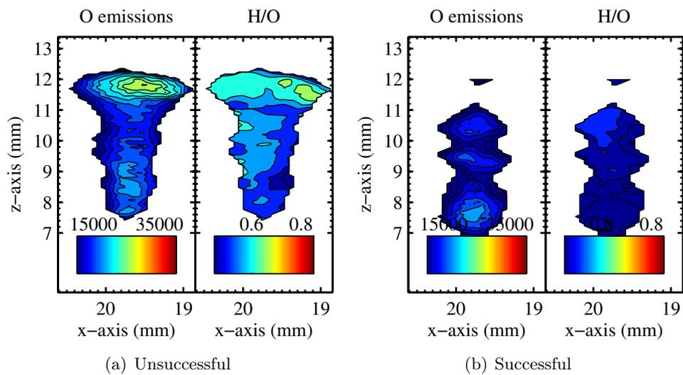
Figure D.3: Location a; Test#3, Analysis of 2D-LIPS experiments for (a) Spark#1 which failed to ignite, and (b) Spark#2 which successfully ignited.
