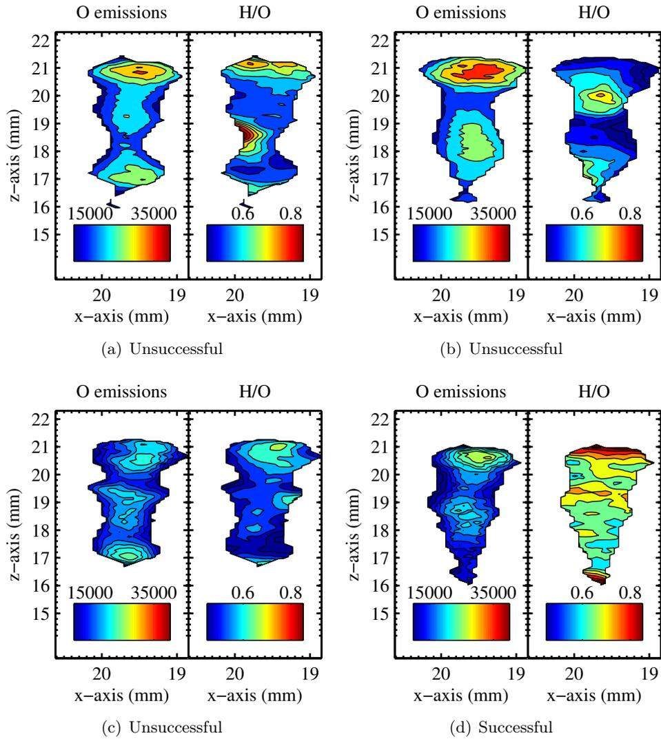
**Figure D.31:** Location *g*; Test#3, Analysis of 2D-LIPS experiments for (a) Spark#1, (b) Spark#2, and (c) Spark#3 which failed to ignite, and (d) Spark#4 which successfully ignited.
