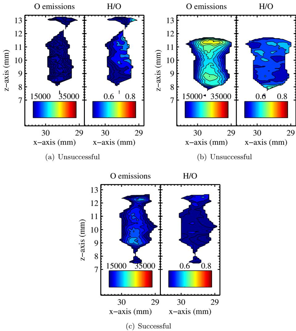
**Figure D.11:** Location c; Test#3, Analysis of 2D-LIPS experiments for (a) Spark#1, and (b) Spark#2 which failed to ignite, and (c) Spark#3 which successfully ignited.
