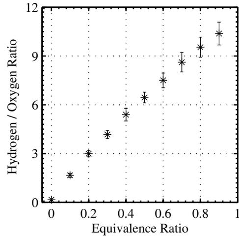
**Figure 8.10:** Variation of Hydrogen-Oxygen ratio obtained by LIPS as a function of equivalence ratio.
