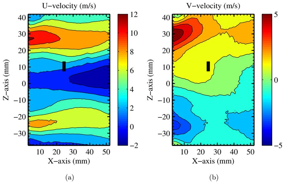
**Figure 9.2:** Location of laser-induced spark for location *b* (small black rectangle) shown in mean velocity fields.
