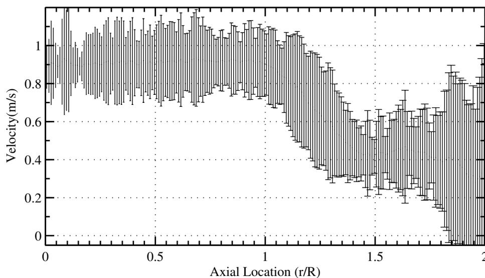
**Figure 8.8:** *Velocity Measurements and fluctuations at vertical location of the plasma as a function of horizontal location.*
