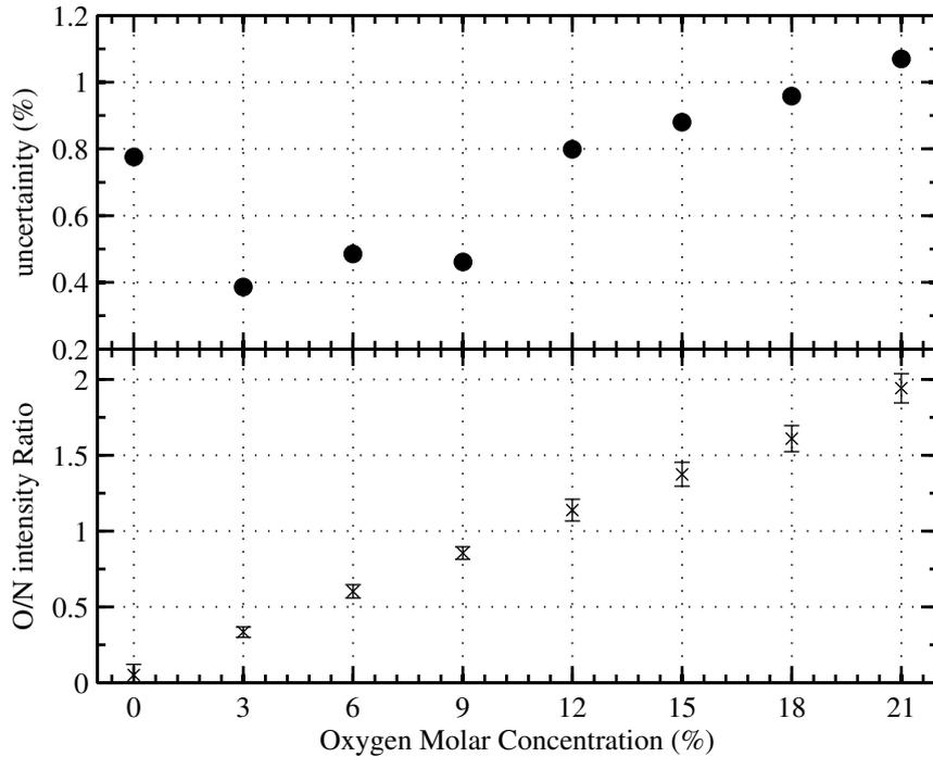
**Figure 8.5:** Analysis of the spectral data in premixed conditions. From bottom to top: (a) Oxygen/Nitrogen ratio as calculated from spectral measurements as a function of input oxygen concentration (b) uncertainty in the measurements of oxygen concentration for given input oxygen concentration.
