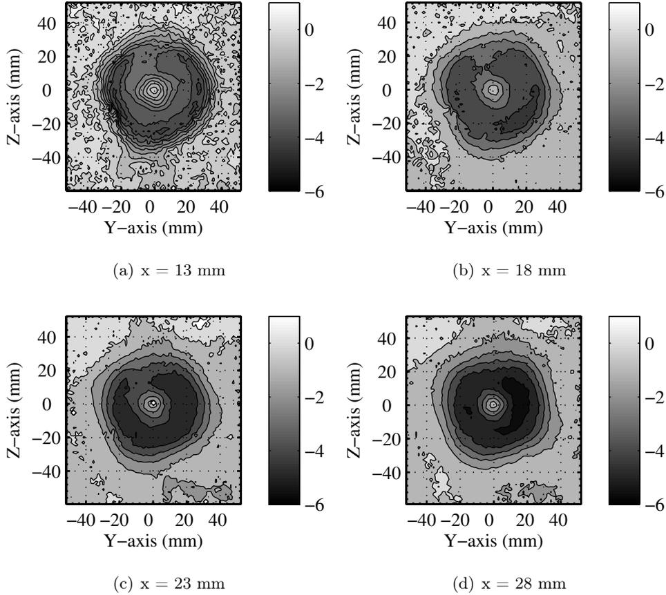
**Figure 5.17:** Azimuthal velocity fields for droplet flow at different axial locations inside the burner.
