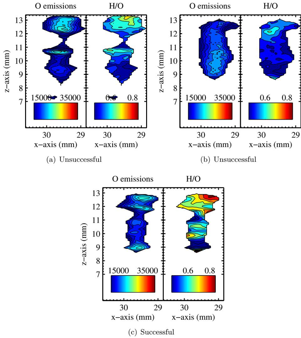
**Figure D.12:** Location *c*; Test#4, Analysis of 2D-LIPS experiments for (a) Spark#1, and (b) Spark#2 which failed to ignite, and (c) Spark#3 which successfully ignited.
