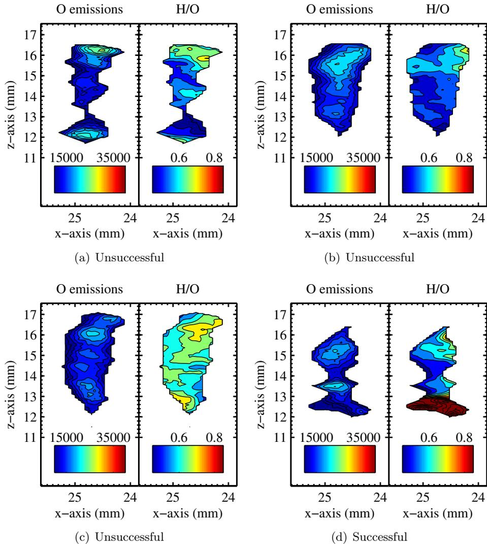
**Figure D.20:** Location e; Test#3, Analysis of 2D-LIPS experiments for (a) Spark#1, (b) Spark#2, and (c) Spark#3 which failed to ignite, and (d) Spark#4 which successfully ignited.
