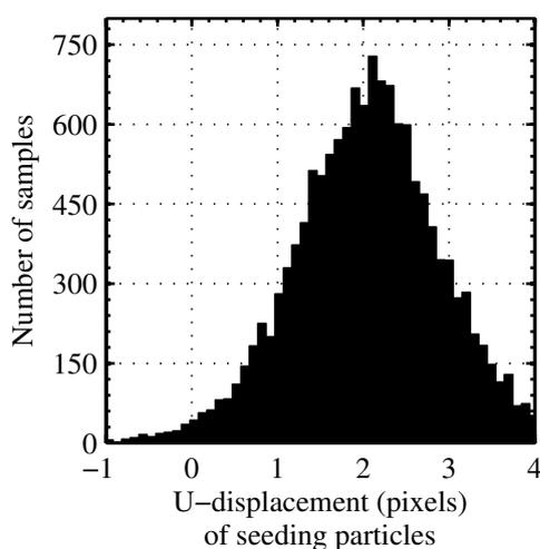
**Figure 5.10:** Histogram of horizontal velocity component at  $y = 0$  mm and  $z = 12$  mm for a transverse plane at an axial distance of 25 mm.
