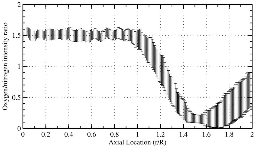
**Figure 8.4:** Variation of oxygen-by-nitrogen intensity ratio as a function of axial distance from the center of the burner.
