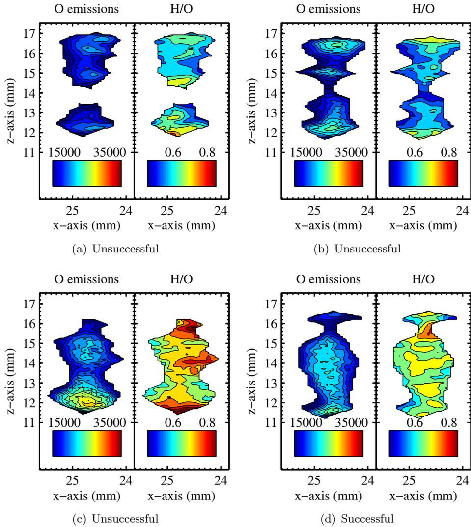
**Figure D.22:** Location e; Test#5, Analysis of 2D-LIPS experiments for (a) Spark#1, (b) Spark#2, and (c) Spark#3 which failed to ignite, and (d) Spark#4 which successfully ignited.
