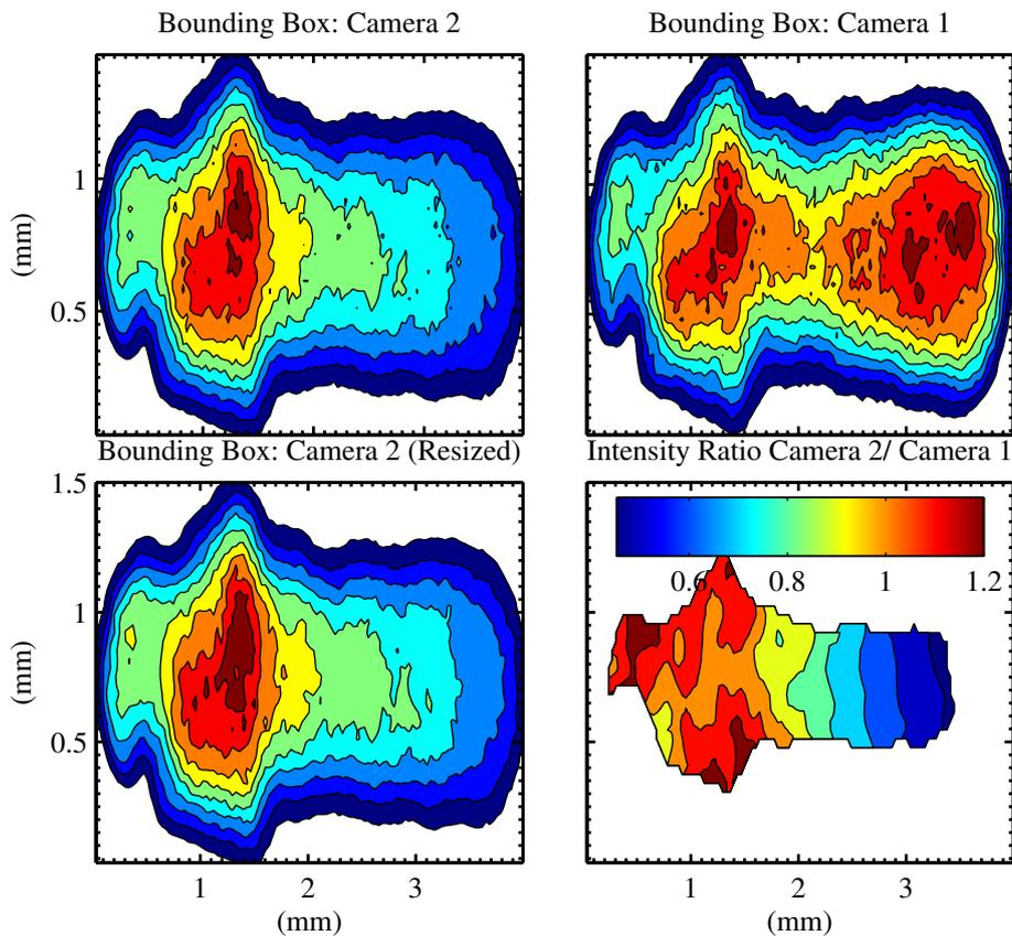
**Figure 8.1:** Typical intensity ratio calculations using the bounding box approach in the region of concentration gradient.
