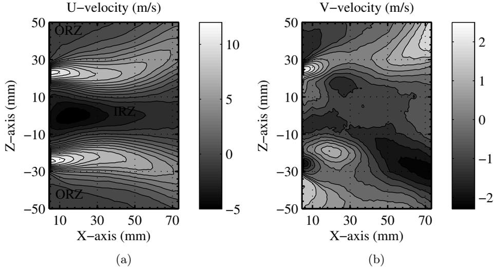
**Figure 5.2:** Mean axial (a) and vertical (b) components of aerodynamic velocity fields, mean calculated over 10000 velocity fields (1 s).
