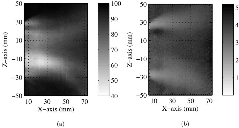
**Figure 5.4:** (a) Percentage of validated vectors for velocity field measurements in axial plane.; (b) Mean of peak ratios during velocity field calculations.
