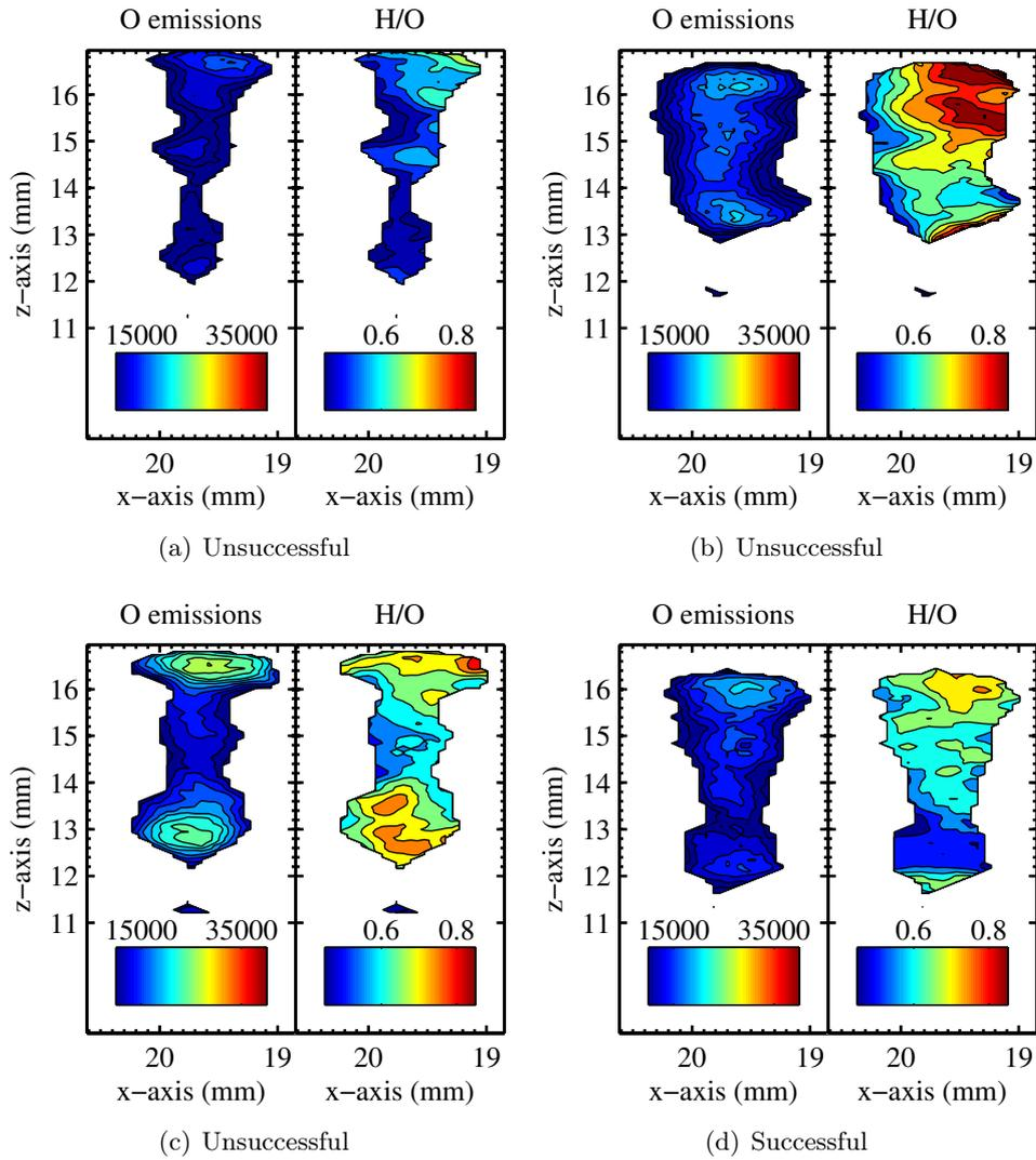
**Figure D.15:** Location d; Test#2, Analysis of 2D-LIPS experiments for (a) Spark#1, (b) Spark#2, and (c) Spark#3 which failed to ignite, and (d) Spark#4 which successfully ignited.
