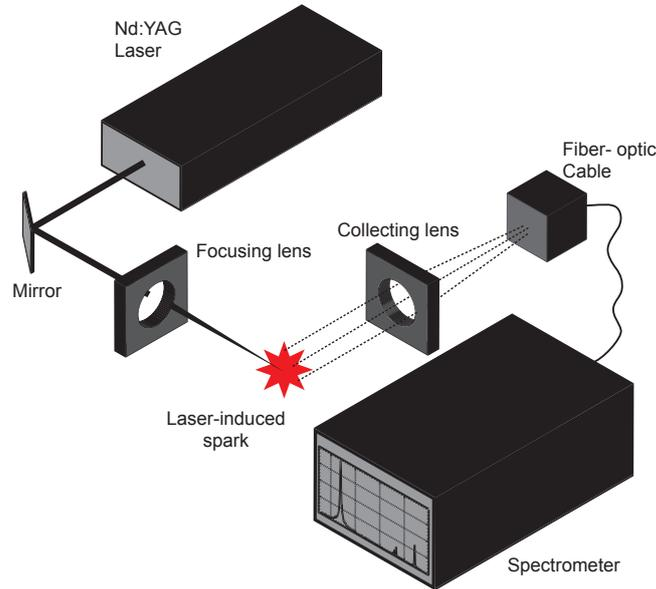
**Figure 2.4:** *Typical setup and principle of LIBS/LIPS measurements.*
