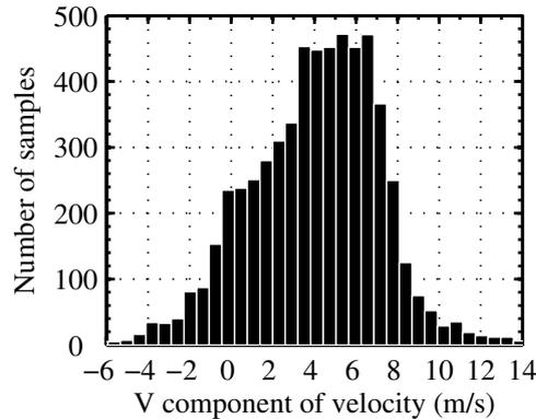
**Figure 5.19:** Histogram of vertical velocity component (m/s) at  $y = -20$  mm and  $z = 20$  mm for a transverse plane at an axial distance of 13 mm.
