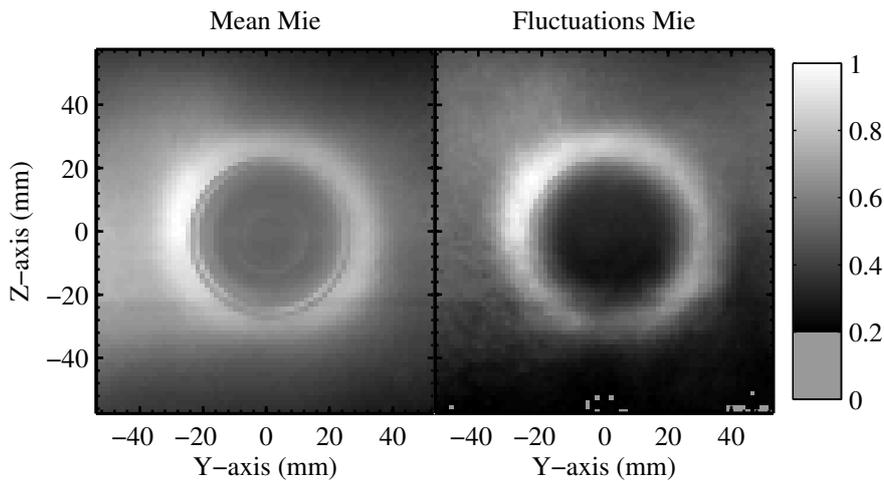
**Figure 5.5:** Mean and fluctuations (over 0.5 s) of Mie-scattering intensity in a transverse plane at an axial distance of 25 mm.
