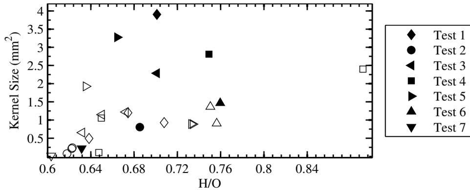
**Figure 9.30:** Size of the initial flame kernel as a function of mean H/O inside the kernel for sparks created at location 'g'. Filled markers represent successful sparks and blank markers represent unsuccessful sparks.
