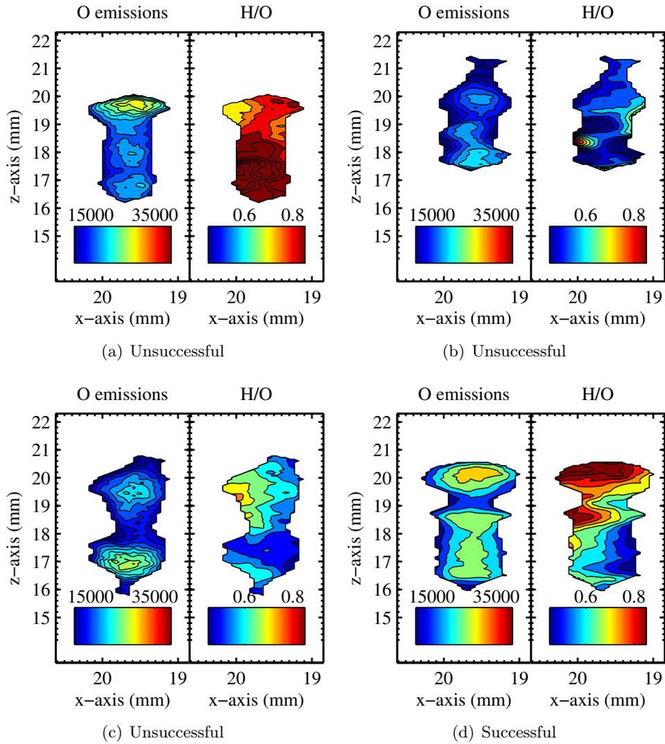
**Figure D.32:** Location *g*; Test#4, Analysis of 2D-LIPS experiments for (a) Spark#1, (b) Spark#2, and (c) Spark#3 which failed to ignite, and (d) Spark#4 which successfully ignited.
