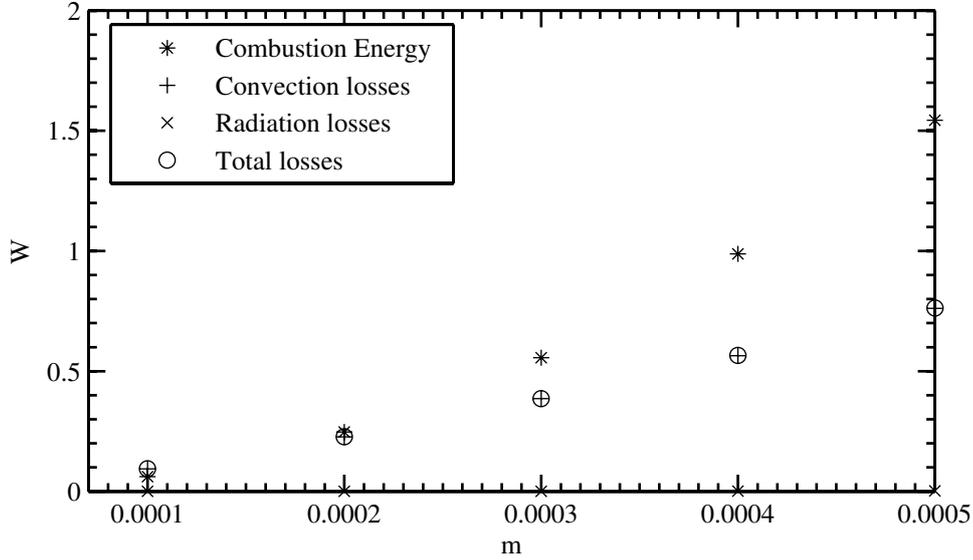
**Figure C.2:** Rate of generation of combustion energy and rate of convection and radiation losses as a function of initial spherical kernel diameter, for sparks created in premixed methane-air mixture with an equivalence ratio of 0.7.
