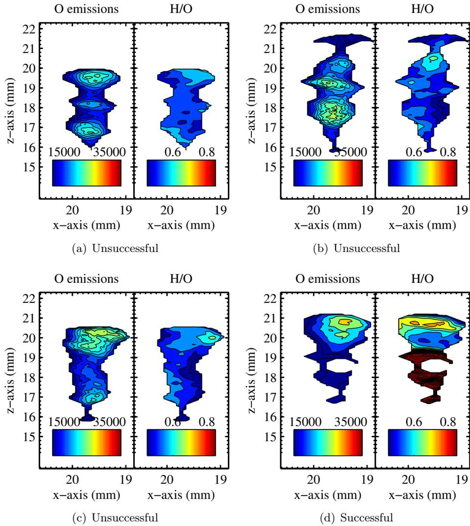
**Figure D.30:** Location *g*; Test#2, Analysis of 2D-LIPS experiments for (a) Spark#1, (b) Spark#2, and (c) Spark#3 which failed to ignite, and (d) Spark#4 which successfully ignited.
