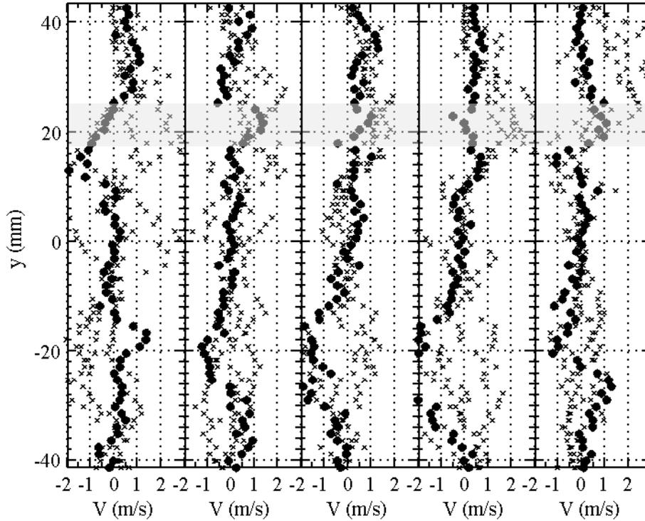
**Figure 6.13:** Mean (over 40 velocity fields  $\bar{1}$  PVC cycle) of vertical velocity components at the axial location of the spark after spark energy deposition;  $\times$  corresponds to non-igniting sparks and  $\bullet$  corresponds to successfully igniting spark; from left to right: test 1-5.
