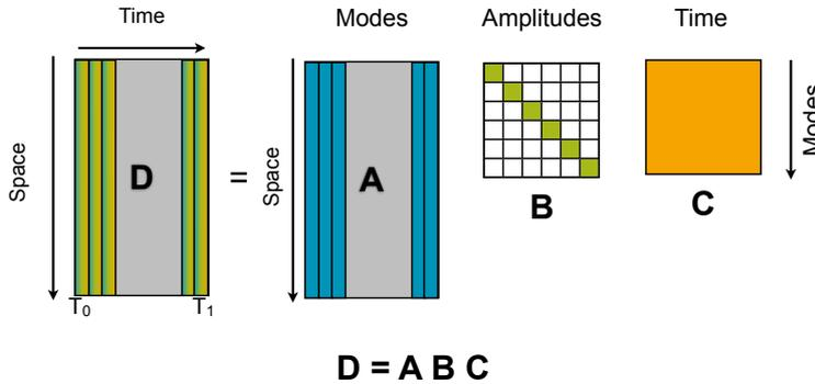
**Figure 4.4:** *Decomposing a matrix  $D$  containing all data into three matrices representing respectively the modes, the amplitudes and temporal evolution.*
