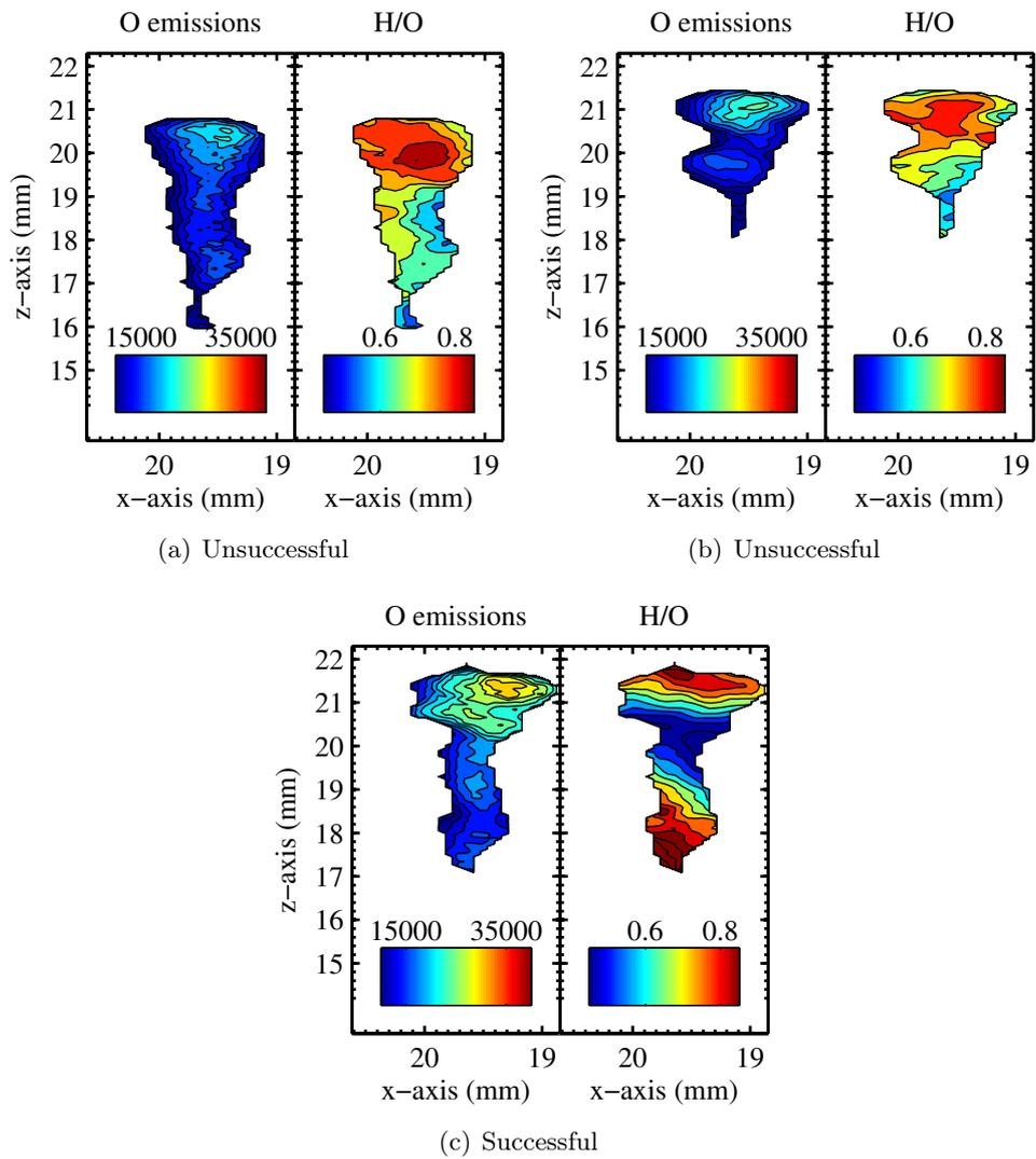
**Figure D.34:** Location *g*; Test#6, Analysis of 2D-LIPS experiments for (a) Spark#1, and (b) Spark#2 which failed to ignite, and (c) Spark#3 which successfully ignited.
