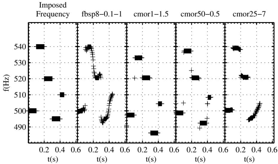
**Figure 4.3:** Results of Continuous Wavelet Transform (CWT) analysis of a synthetic signal.
