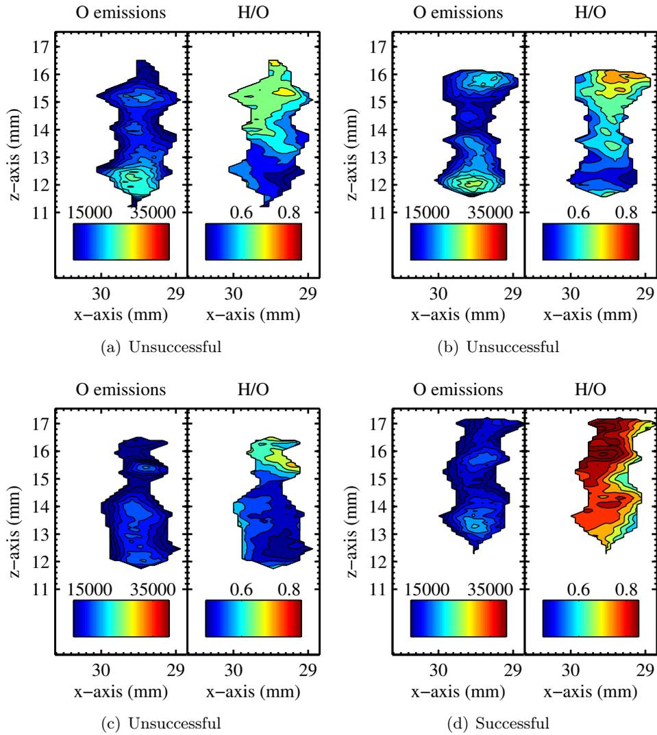
**Figure D.27:** Location *f*; Test#1, Analysis of 2D-LIPS experiments for (a) Spark#1, (b) Spark#2, and (c) Spark#3 which failed to ignite, and (d) Spark#4 which successfully ignited.
