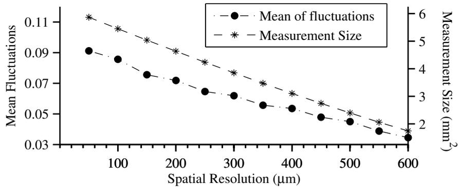
**Figure 7.18:** Variation of standard deviation in calculations of intensity ratio and the number of points/pixels where information is available with size of digital FIR filters or resulting resolution of measurements.
