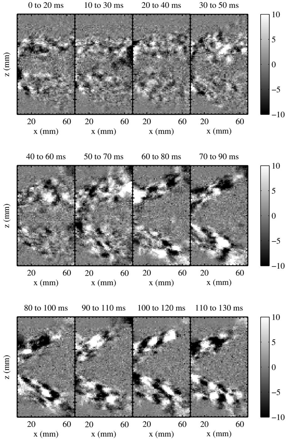
**Figure 6.16:** Time-resolved DMD after igniting spark, Test 1: images 1-12 show results using velocity fields, respectively, over (0-to-20 ms), (10-to-30 ms), ....., (30-10 ms), (20-0 ms) after the igniting spark
