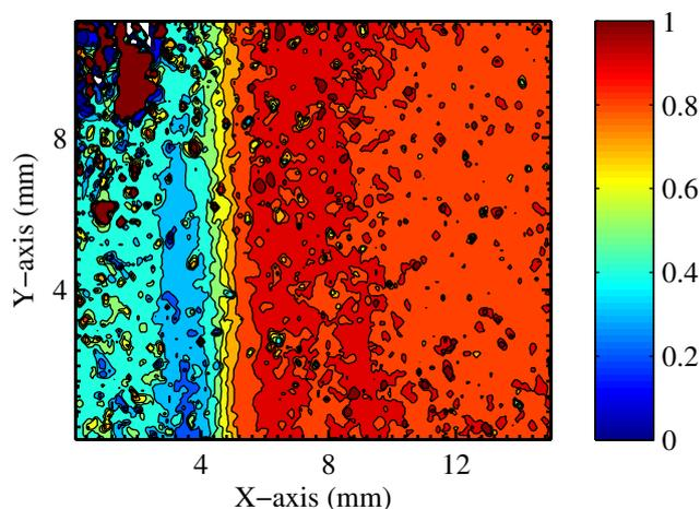
**Figure 8.7:** *Velocity field measurement above the burner using PIV.*
