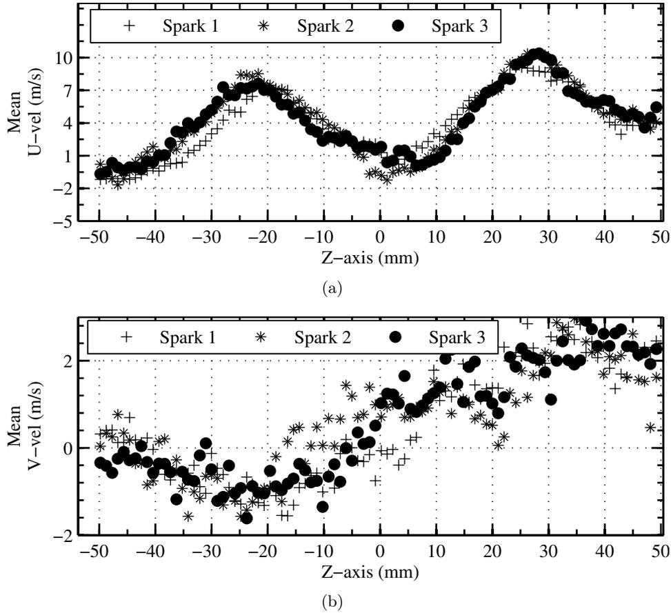
**Figure 9.12:** Location *b*; Test#2, Analysis of PIV measurements for 3 consecutive sparks. Spark#1 and #2 failed to ignited while Spark#3 successfully ignited. Velocity profiles at the location of spark have been plotted as a function of radial distance; spark located at 8-13 mm. Profiles plotted using mean velocity fields (over 100 instantaneous fields equivalent to 10 ms) before the deposition of spark energy.
