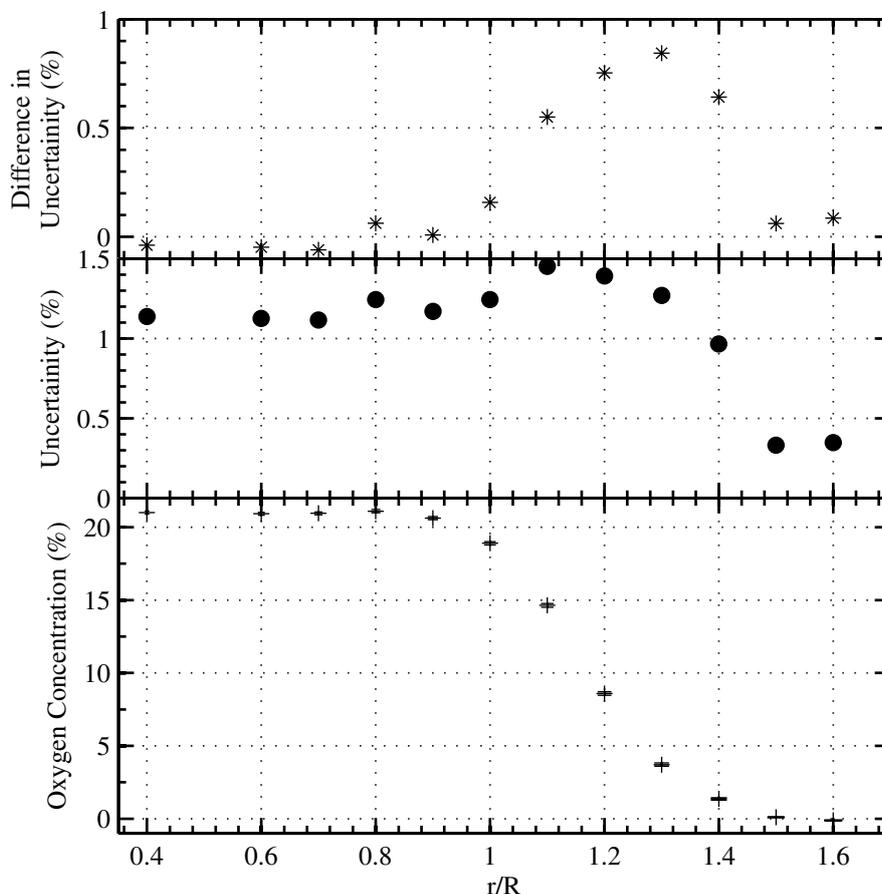
**Figure 8.6:** Analysis of the spectral data across the mixing layer. From bottom to top: (a) error bar showing calculated Oxygen concentration and corresponding fluctuations. (b) Uncertainty in the calculation of oxygen concentration. (c) Difference in the uncertainty in oxygen concentration as compared to the uncertainty corresponding to the same mean oxygen concentration in the premixed measurements.
