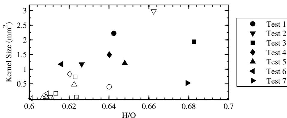
**Figure 9.8:** Size of the initial flame kernel as a function of mean H/O inside the kernel. Filled markers represent successful sparks and blank markers represent unsuccessful sparks.
