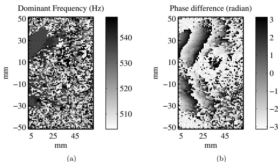
**Figure 5.22:** (a) Dominant frequencies in an axial plane inside the burner.; (b) Cross power spectral density analysis of Mie-scattering images in an axial plane.
