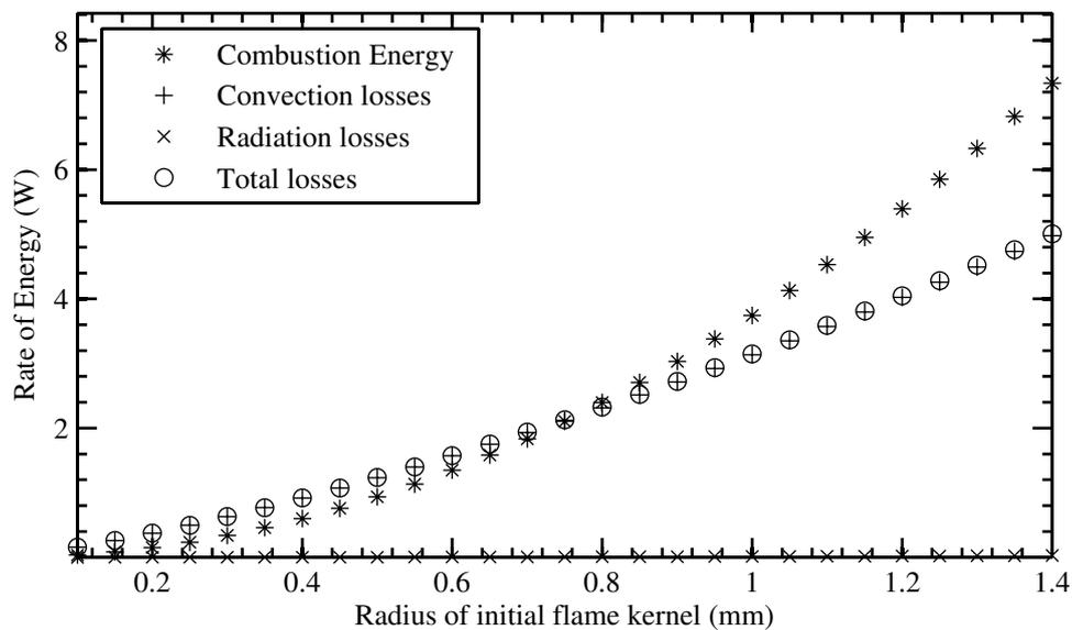
**Figure C.3:** Rate of generation of combustion energy and rate of convection and radiation losses as a function of initial spherical kernel diameter for dodecane.
