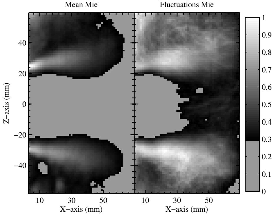
**Figure 5.1:** Mean and fluctuations of Mie-scattering intensity in an axial plane, averaged over 1 s, i.e. 10000 image frames.
