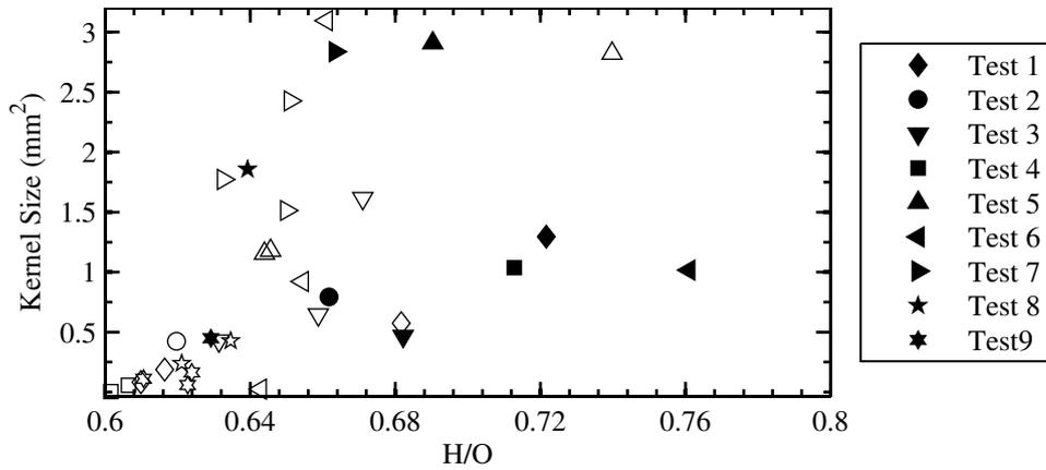
**Figure 9.25:** Size of the initial flame kernel as a function of mean  $H/O$  inside the kernel for sparks created at location 'e'. Filled markers represent successful sparks and blank markers represent unsuccessful sparks.
