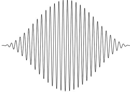
**Figure 2.2:** *Typical signal of a Doppler burst.*
