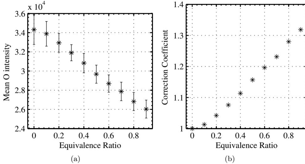
**Figure 8.13:** (a) Mean intensity of oxygen images as a function of equivalence ratio; and, (b) Correction factor for oxygen image intensity as a function of local equivalence ratio in order to obtain local spark energy.
