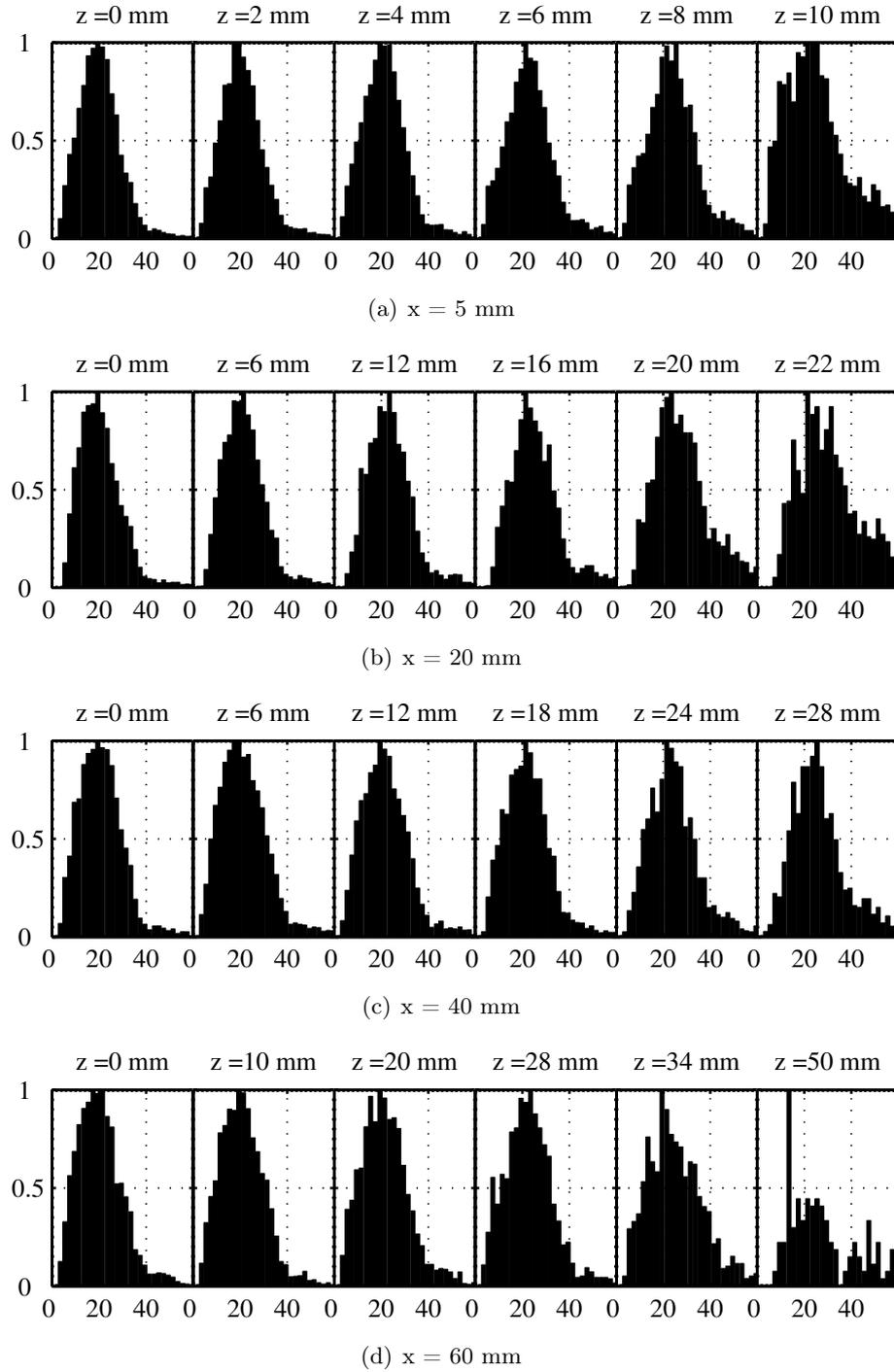
**Figure 5.11:** Histogram of droplet diameters ( $\mu\text{m}$ ), at axial locations of (a) 5 mm, (b) 20 mm, (c) 40 mm, and (d) 60 mm. At each axial location, histograms are plotted at few vertical locations  $z$ .
