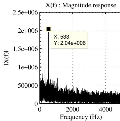
**Figure 6.7:** Fast fourier transform of the Mie scattering intensity at the exit of the injector.
