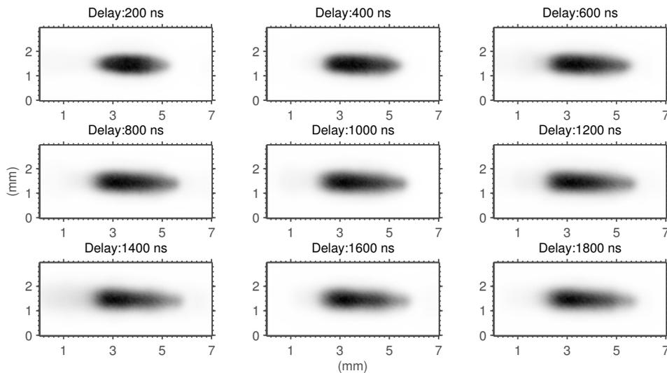
**Figure 7.10:** Mean Images of laser-induced plasmas in air, acquired with oxygen filter for different delays with respect to the initial occurrence of plasma; Spark energy = 30 mJ
