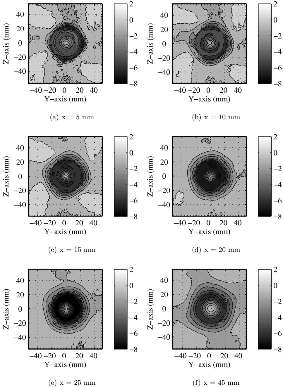
**Figure 5.8:** Azimuthal velocity fields for different axial locations inside the burner.
