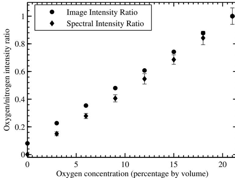
**Figure 8.3:** Comparison of 0D-LIPS and 2D-LIPS technique: Mean and fluctuations of 2D-LIPS and 0D-LIPS measurements as a function of oxygen concentration.
