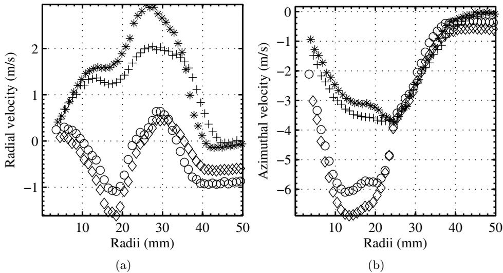
**Figure 5.24:** Comparison between aerodynamic and droplets' velocity fields: (a) Comparison of radial components and (b) comparison between azimuthal components; (\*)  $x = 13$  mm, droplets, (+)  $x = 18$  mm, droplets, (o)  $x = 15$  mm, aerodynamic, (◇)  $x = 20$  mm, aerodynamic.
