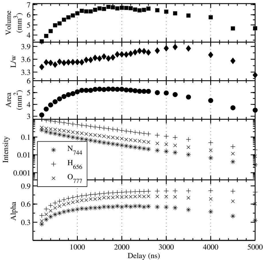
**Figure 7.9:** Effects of delay after plasma formation on, from top to bottom: (1) volume of the plasma, (2) aspect ratio of the plasma, (3) area of the plasma image, (3) normalized intensity for different atomic emission and (4)  $\alpha$  for the same atomic emissions, as a function of time after the initial occurrence of plasma; plasma created in premixed air-methane mixture with an equivalence ratio of 0.6.
