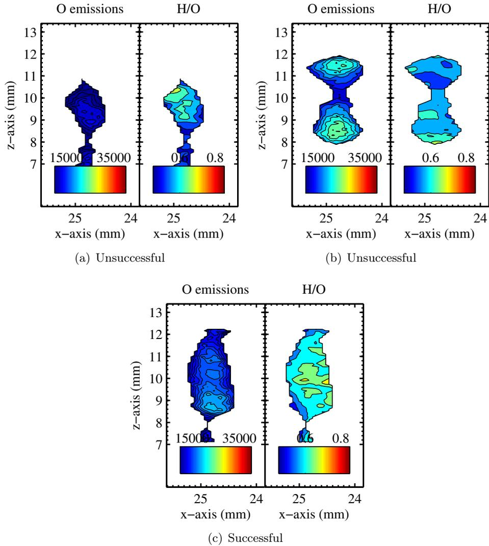
**Figure D.6:** Location b; Test#4, Analysis of 2D-LIPS experiments for (a) Spark#1, and (b) Spark#2 which failed to ignite, and (c) Spark#3 which successfully ignited.
