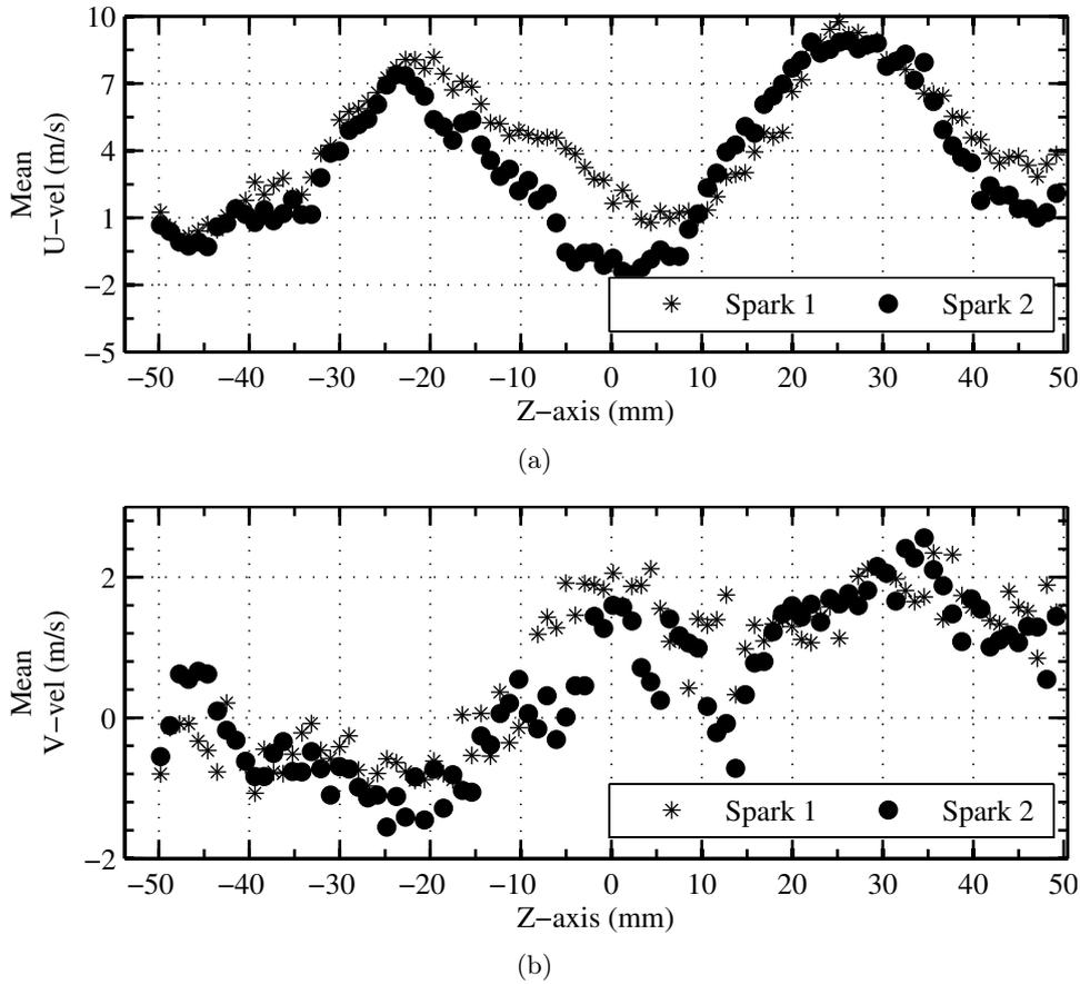
**Figure 9.10:** Location *b*; Test#1, Analysis of PIV measurements for 2 consecutive sparks. Spark#1 failed to ignited while Spark#2 successfully ignited. Velocity profiles at the location of spark have been plotted as a function of radial distance (*Z*-axis); spark located at 8-13 mm. Profiles plotted using mean velocity fields (over 100 instantaneous fields equivalent to 10 ms) before the deposition of spark energy.
