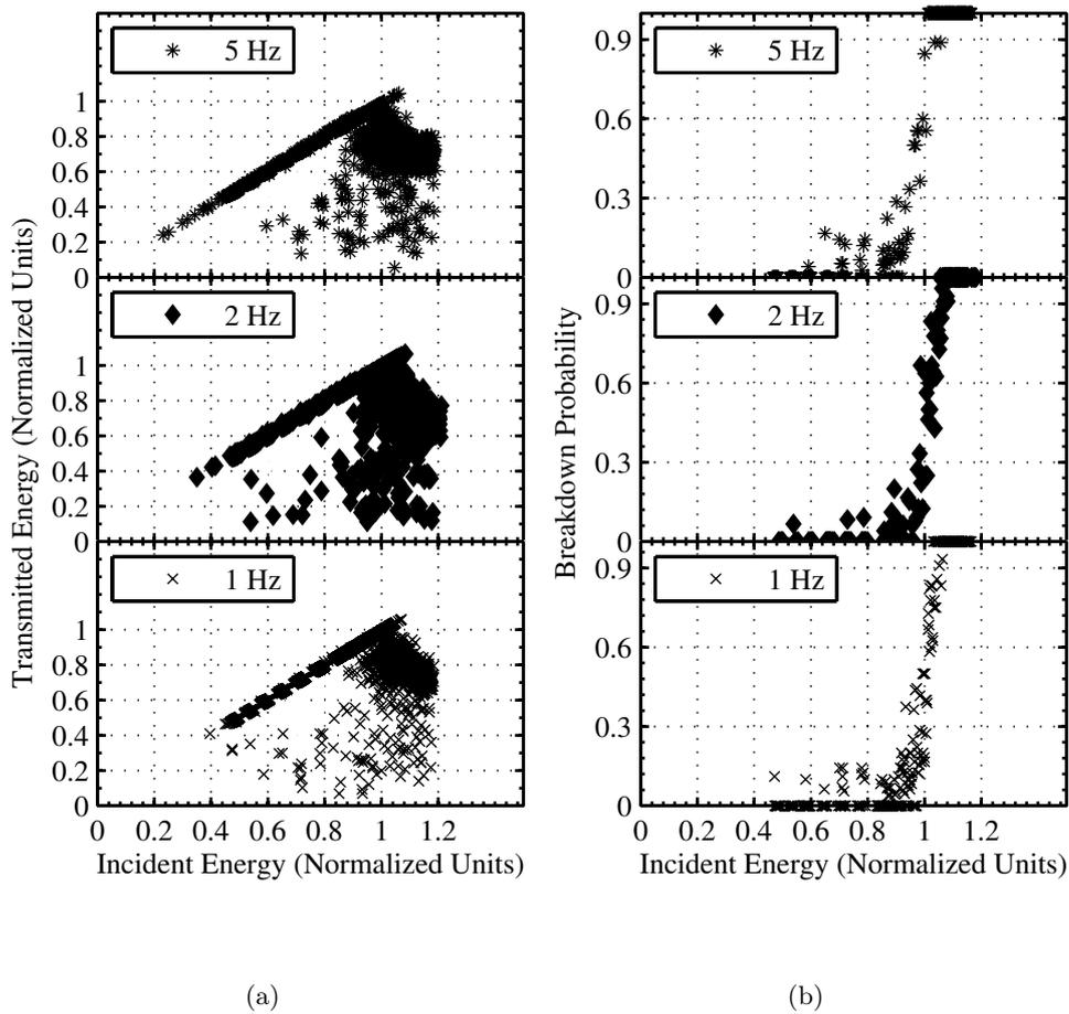
**Figure 7.4:** Effect of laser pulse frequency on breakdown: (a) Incident vs Transmitted Energy for different laser pulse frequency; and, (b) Breakdown probability as a function of incident laser energy.
