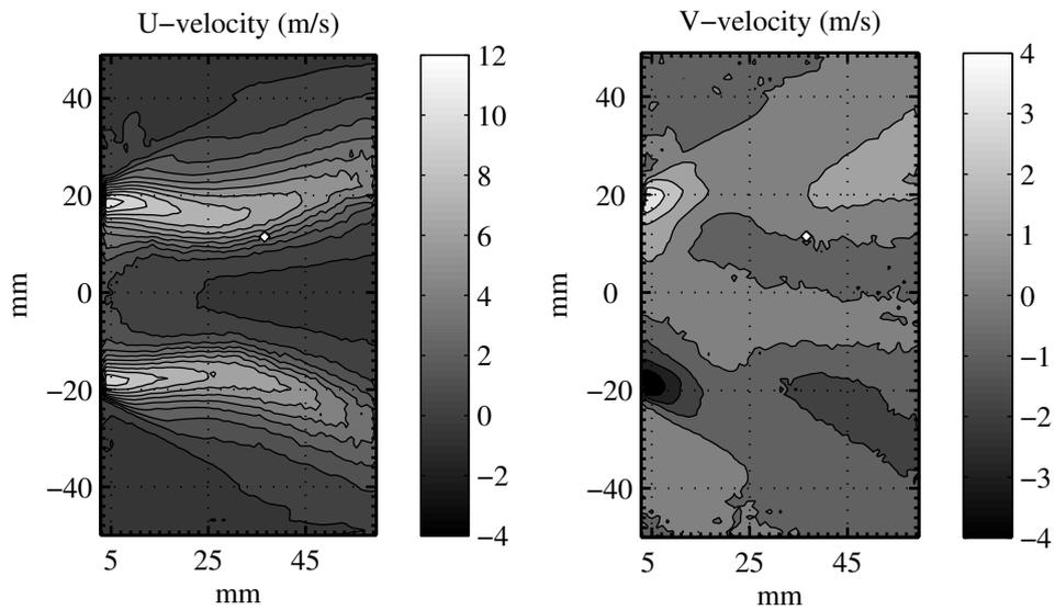
**Figure 5.14:** Mean axial ( $U$ ) and vertical ( $V$ ) components of droplets velocity fields, calculated over 1 s
