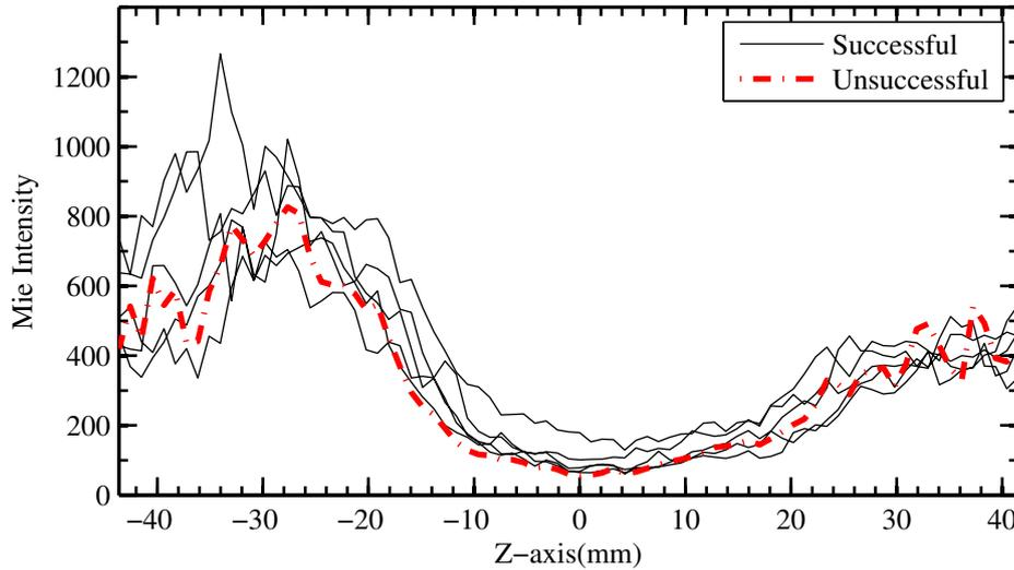
**Figure 9.20:** Radial profiles of mean Mie-scattering intensity (over 10 ms, before sparks) at axial location of the sparks created at location 'c'; Five successful and one unsuccessful sparks compared.
