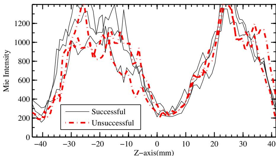
**Figure 9.23:** Radial profiles of mean Mie-scattering intensity (over 10 ms, before sparks) at axial location of the sparks created at location 'd'; Three successful and two unsuccessful sparks compared.
