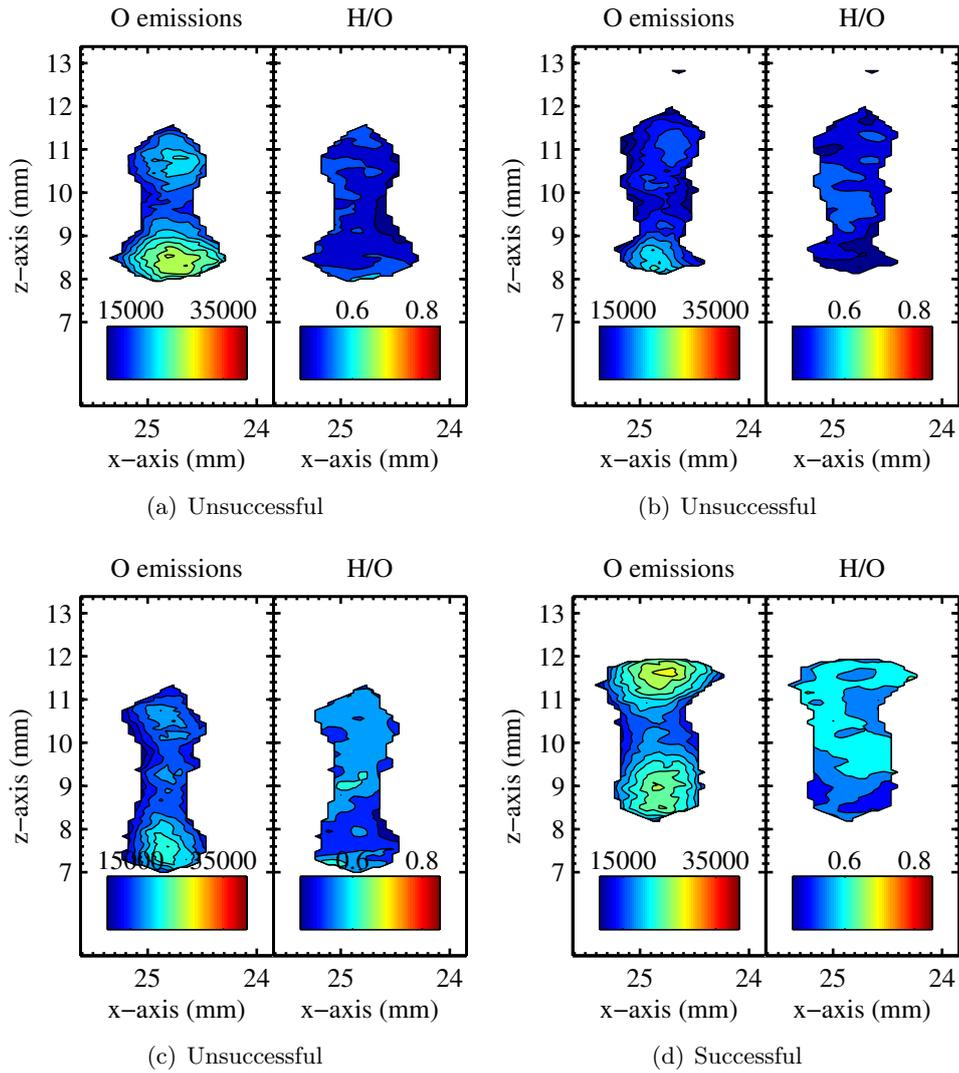
**Figure D.8:** Location *b*; Test#6, Analysis of 2D-LIPS experiments for (a) Spark#1, (b) Spark#2, and (c) Spark#3 which failed to ignite, and (d) Spark#4 which successfully ignited.
