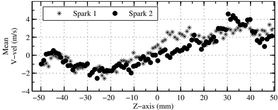
**Figure 9.16:** Location *a*; Test#3, Analysis of PIV measurements for 2 sparks. Spark#1 failed to ignite while Spark#2 successfully ignited. Velocity profiles at the location of spark have been plotted as a function of radial distance; spark located at 8-13 mm. Profiles plotted using mean velocity fields (over 100 instantaneous fields equivalent to 10 ms) before the deposition of spark energy.
