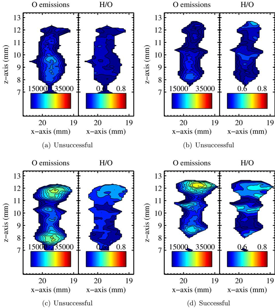
**Figure D.1:** Location a; Test#1, Analysis of 2D-LIPS experiments for (a) Spark#1, (b) Spark#2, and (c) Spark#3 which failed to ignite, and (d) Spark#4 which successfully ignited.
