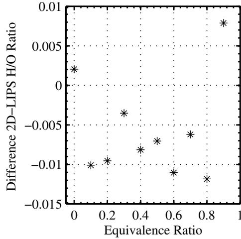
**Figure 8.12:** Difference between the mean H/O ratio calculated by 2D-LIPS for two different spark energies of 73 mJ and 113 mJ.
