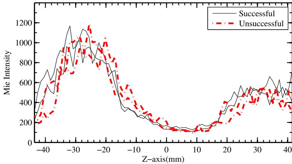
**Figure 9.28:** Radial profiles of mean Mie-scattering intensity (over 10 ms, before sparks) at axial location of the sparks created at location 'f'; Two successful and two unsuccessful sparks compared.
