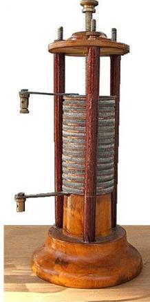
Figure I.4: Pile Voltaïque [14]
