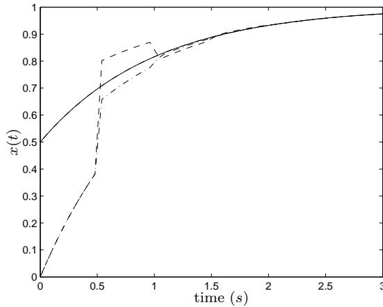
FIGURE 4.15: observer simulation with the state  $x(t)$  (continuous) and the estimation of  $\hat{x}(t)$  (dashed  $k = 0.8$ , dashed-dot  $k = 0.5$ ),  $h = 0.5$  and the initial condition is  $x_0 = 0.5$ , (Example 4.10).
