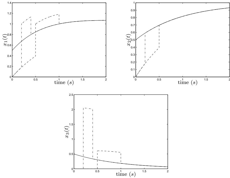
FIGURE 4.16: observer simulation with the state  $x(t)$  (continuous) and the estimation of  $\hat{x}(t)$  (dashed  $h = 0.5$ , dashed-dot  $h = 0.2$ ), the initial condition is  $x_0 = [0.5 \ 0.5 \ 0.5]^T$ , (Example 4.11).
