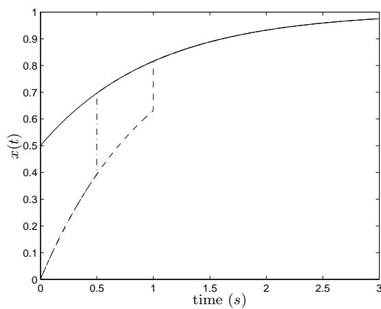
FIGURE 4.14: observer simulation with the state  $x(t)$  (continuous) and the estimation of  $\hat{x}(t)$  (dashed  $h = 1$ , dashed-dot  $h = 0.5$ ),  $k = e^{-h}$  and the initial condition is  $x_0 = 0.5$ , (Example 4.10).
