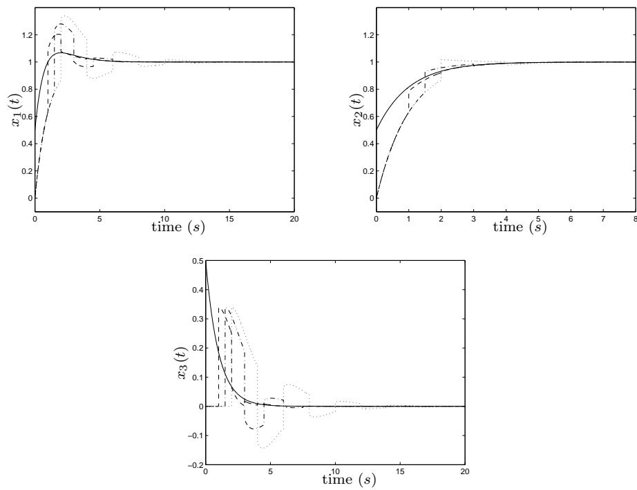
FIGURE 4.18: observer simulation with the state  $x(t)$  (continuous) and the estimation of  $\hat{x}(t)$  ( $\Delta h = 0.5$  (dash),  $\Delta h = 1$  (dash-dot),  $\Delta h = 1.5$  (dot) ), the initial condition is  $x_0 = [0.5 \ 0.5 \ 0.5]^T$ , (Example 4.12).
