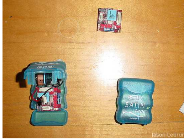
Figure 2.1: iMotes: these devices were used in most of the real-life based measurements. They embed a Bluetooth chip alternatively collecting and sending probes in their vicinity. When an iMote detects a probe, it collects the sender's ID.
