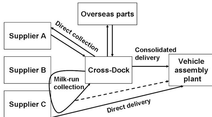
**Fig. 1.3** Inbound supply chain process Source [Miemczyk and Holweg, 2004]. Cross-docking is a well-known practice in logistics, consisting in unloading materials from ingoing trucks and loading them in outgoing trucks with little or no storage in between.
