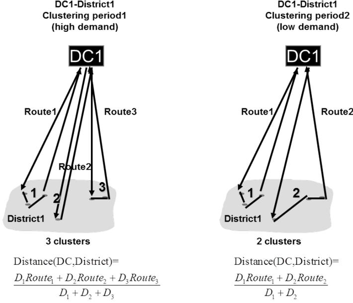
**Fig. 5.4** Clustering per district/DC/period. Example of 2 time-periods for a given DC and a given district.  $D_i$  denotes the total demand of cluster  $i$ .  $Route_i$  is the optimal route visiting the customers of cluster  $i$
