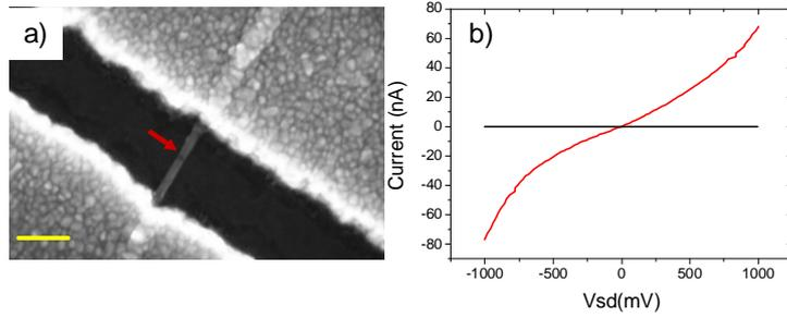
**Figure 3.12:** a) SEM micrograph of the nanowire after the Joule heating annealing on both contacts. The unreacted silicon channel (red arrow) is 8nm long. Scale bar 100nm. b) IV characteristics of the nanowire taken before (black) and after (red) the annealing.
