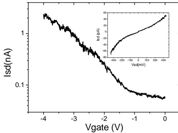
**Figure 3.14:** Transfer characteristic ( $V_{sd}=500\text{mV}$ ) of a top gated Schottky barrier transistor with a channel length of 78nm and 5nm  $\text{HfO}_2$  gate oxide deposited by ALD. Inset: IV characteristic
