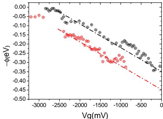
**Figure 2.14:** *Extracted effective barrier heights from the Arrhenius plots for the two Schottky contacts as a function of the corresponding gate. The intercepts to the zero gate voltage axis are the SBH for the source and drain contacts and they differ by  $\approx 100\text{meV}$ . Dashed lines are guide to the eye.*
