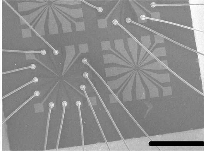
**Figure 3.19:** SEM micrograph of a typical sample. The bonded pads left floating develop an important static charge when exposed to the electron beam and they appear darker than the other bonding pads. Scale bar 1mm.
