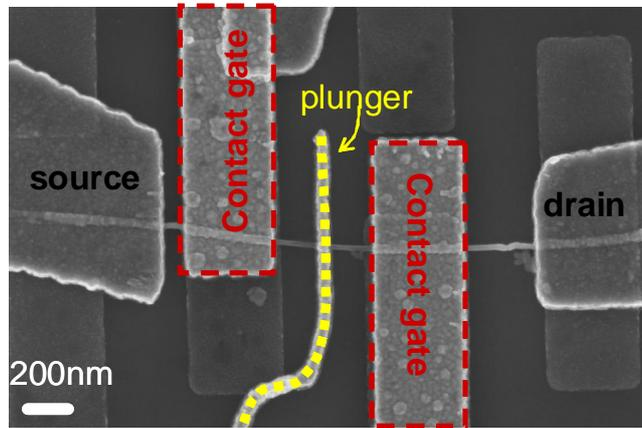
**Figure 2.7:** SEM micrograph of a Silicon nanowire (diameter  $d \approx 35\text{nm}$ ) device with three independent addressable gates at the contacts (dashed red boxes) and in the middle portion of the nanowire (dashed yellow line). The injection of carriers at the source and drain Schottky contacts is controlled by two surround gates while a thin ( $\approx 70\text{nm}$ ) plunger gate controls the channel potential
