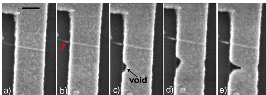
**Figure 3.21:** Real time observation of the Joule assisted silicidation by varying the heating current  $I_h$ . Starting with a value of 16mA a), the current was stepped to 20mA b) leading to a formation of the silicide (red arrow). Formation of a void was observed at 22nA c) and progressed in the next two image scans d)e). Scale bar 300nm
