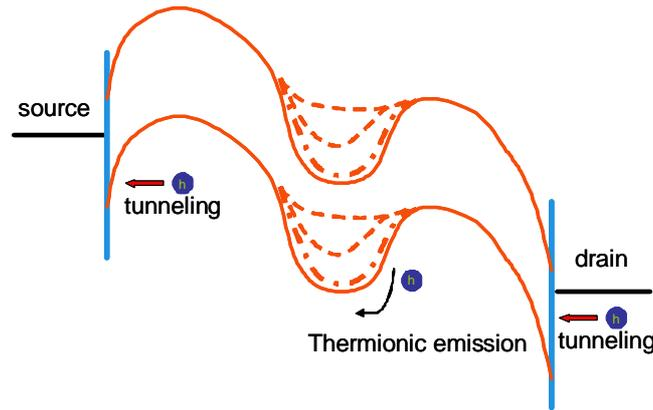
**Figure 2.9:** Schematic diagram of the band bending for  $V_{SD} < 0$  at the contacts and in the channel due to the combined action of both contact and plunger gates. The contact gates control the band bending at the source and drain while the plunger gate controls the bulk. If the source potential is sufficiently large and negative the current saturates as a consequence of a thermally activated transport across the bulk potential barrier controlled by the plunger.
