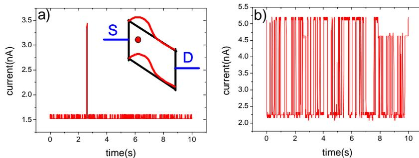
**Figure 3.17:** Time domain  $I(t)$  traces taken at 4.2K over a time period of 10 seconds for the device in fig.3.16 taken with a source-drain polarization of a) 400mV and b) 500mV. The current switches between different levels with a time dynamics strongly dependent on the bias applied. Inset: simplified schematics illustrating the effect of a single trap site which modifies the potential barrier experienced by the carriers between the source and drain terminals.
