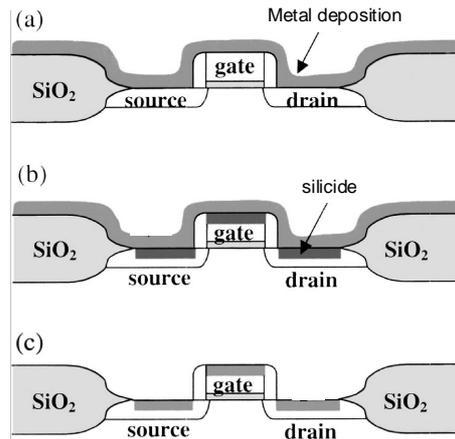
**Figure 1.6:** Flow chart for the SALICIDE process. a) The metal layer is deposited over the MOSFET structure. b) A thermal annealing promotes the formation of the silicide on the source, drain and gate terminals, no reaction takes place on the oxide spacers if the metal atoms are the dominant diffusing species like in the case of Nickel. c) After a selective wet chemical etch the excess metal is removed.
