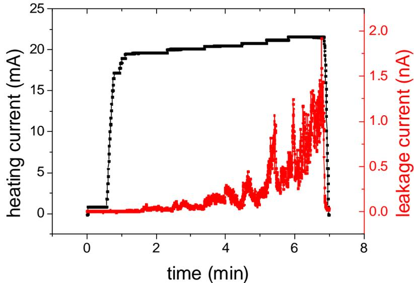
**Figure 3.10:** (red curve). Leakage current flowing in the nanowire as a function of time and the heating current on the first contact. The nanowire is polarized with a fixed bias voltage while the heating current is ramped up to 20.5mA. When the leakage current reaches a value around 1nA the heating current is brought to zero.
