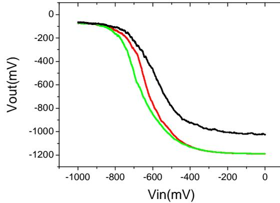
**Figure 2.19:** Output characteristic of the logic gate as a function of the logic address level input. Black curve:  $V_{in} = V_1$ ,  $V_2 = -1V$  corresponding to the transition from the address level inputs  $(1, 1) \leftrightarrow (0, 1)$ ; red curve:  $V_{in} = V_2$ ,  $V_1 = -1V$  corresponding to the transition  $(1, 1) \leftrightarrow (1, 0)$ ; green curve:  $V_{in} = V_1 = V_2$ ; corresponding to the transition  $(1, 1) \leftrightarrow (0, 0)$ .
