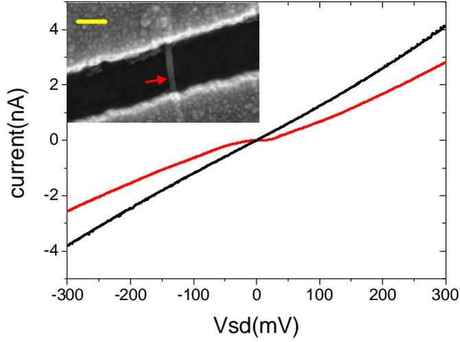
**Figure 3.15:** *I-V characteristic of a device with a channel length of 10nm between room temperature (black curve) and 230mK (red curve). Inset: SEM micrograph of the device before top gate patterning. Scale bar 100nm. The silicon channel is highlighted by the red arrow. Transport in the device is governed by direct tunneling through the channel. The device after deposition of 5nm  $\text{HfO}_2$  oxide and top gate patterning doesn't show any gate induced modulation of the channel current.*
