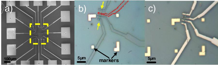
**Figure 1.3:** a) SEM picture of one of the four subcells. The active part of the device, highlighted by the yellow dashed box, is enclosed in macroscopic sized contact pads already predefined on the sample along with alignment markers. b) Optical micrograph showing the contacts patterned in the resist right after the developing step described in 1.2 and c) the finished device after metal evaporation and lift-off.
