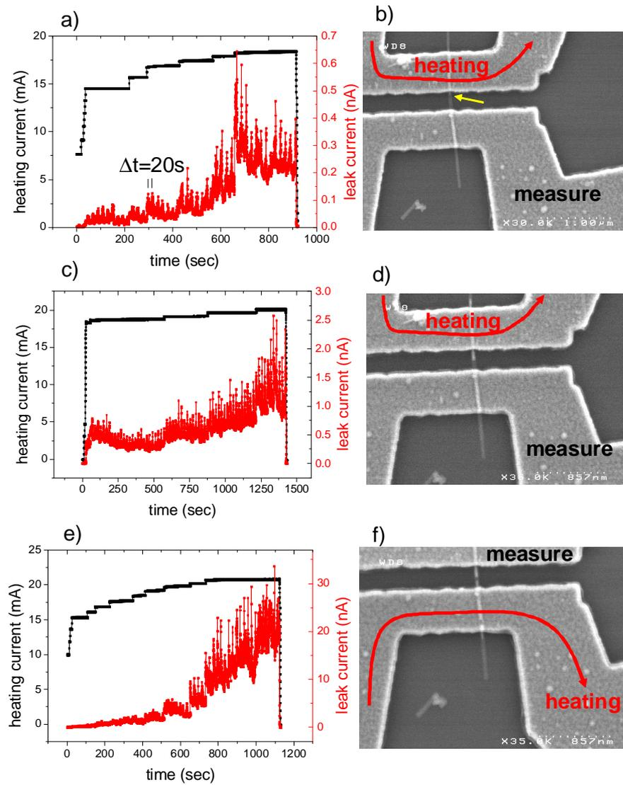
**Figure 3.22:** a)-d) Leakage current and corresponding images of the nanowire taken at the end of each time series for the first heated contact. e) Same time trace when inverting the role of the two contacts and f) final device.
