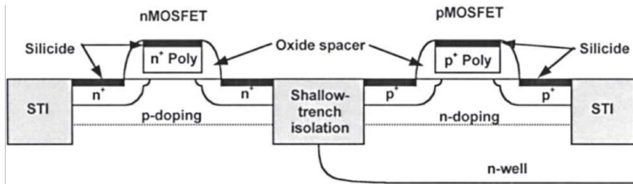
**Figure 1.4:** Cross section of modern CMOS transistors where the source, drain and gate terminals are contacted with metal silicides.
