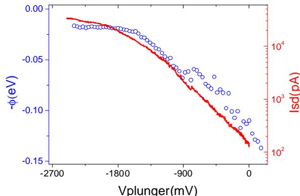
**Figure 2.12:** Extracted barrier heights as a function of the plunger gate (blue curve) and the transfer characteristic of the transistor (red curve) taken with  $V_{SD} = 100\text{mV}$  and  $V_{GS} = V_{GD} = -3.2\text{V}$  at room temperature and in a vacuum tube at a pressure of  $10^{-6}\text{mbar}$ .
