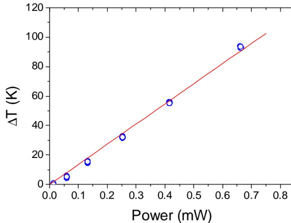
**Figure 3.9:** *Temperature difference between the heater and the thermometer as a function of the power dissipated in the heater. From the slope of the curve we can extract the thermal conductivity  $\kappa$  of the substrate which amounts to  $0.3\text{W/mK}$ .*
