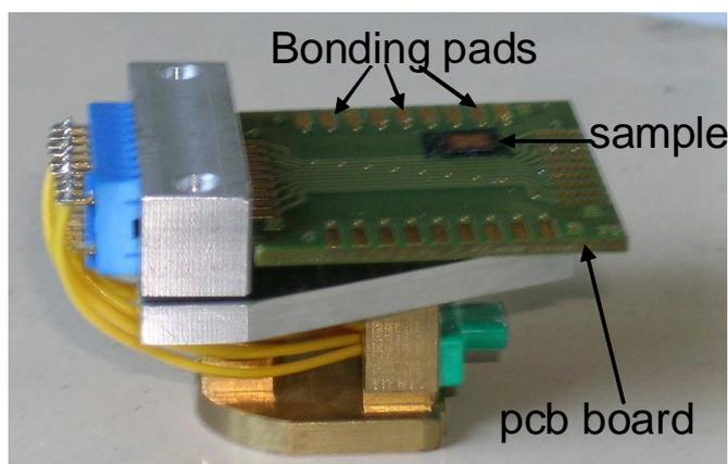
**Figure 3.20:** Sample holder for the Hitachi 4110S.
