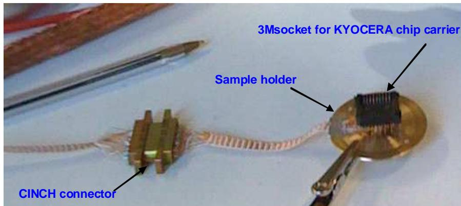
**Figure 3.18:** Sample holder for the JEOL 840A
