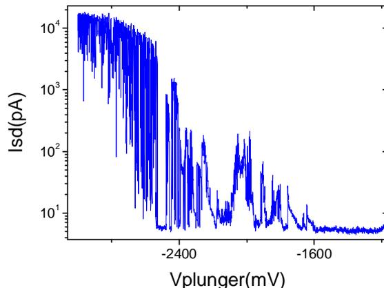
**Figure 2.15:**  $I_{SD} - V_{Plunger}$  characteristic at  $T = 4K$ . Transport is activated for a plunger gate voltage  $V_{Plunger} < -1600mV$  where the residual barrier can be made negligibly small.  $V_{SD} = 100mV$
