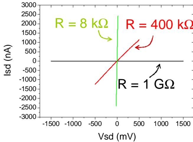
**Figure 2.3:** *IV comparison between nanowires with degenerate uniform  $n$ -type doping (green curve), heavily doped sections with an intrinsic channel (red curve) and undoped (black curve). In all the three cases the contacting material is Nickel and the channel length is  $1\mu\text{m}$ .*
