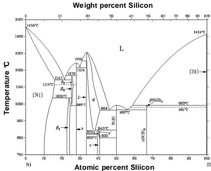
Figure 1.7: Phase diagram for the Ni-Si binary system.
