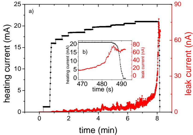
**Figure 3.11:** a) Leakage current measured on the first contact while the second one is been heated by the current flowing in the second stripline. b) Close up view of the region with steepest slope for the leakage current in a).
