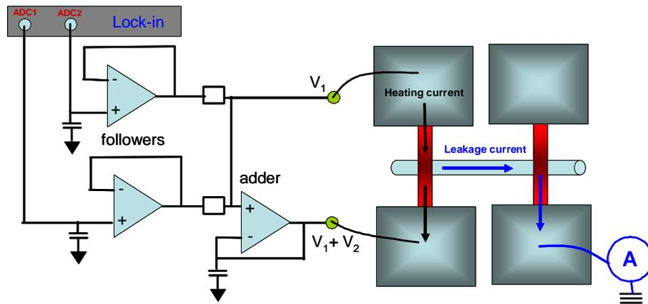
**Figure 3.5:** Schematics of the experimental set-up used to decouple the heating voltage used to drive the heating current through the stripline from the biasing voltage falling on the nanowire. The heating current and the biasing voltage can be varied independently allowing a simultaneous measurement of the leakage current flowing into the nanowire as a function of the heating current and the bias potential.
