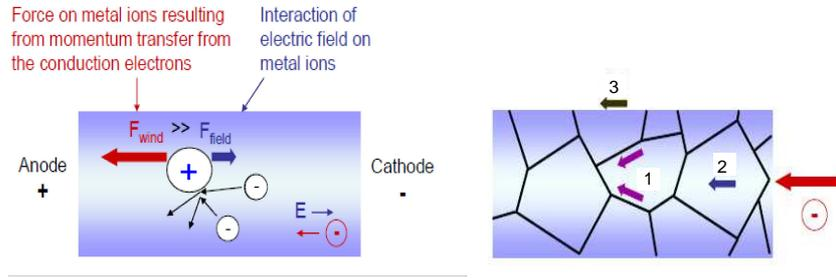
**Figure 3.3:** a) Schematic representation for the phenomenon of electromigration. The metal ions become mobile under the action of an intense current density which increases locally the temperature. On the ions two forces are exerted one due to the external field applied and one due to scattering with electrons. b) Schematic view of a polycrystalline metal. The mobile ions can follow paths along 1) the grain boundaries, 2) single grains 3) the surface.
