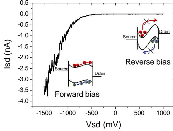
**Figure 2.17:** *IV characteristic showing the rectifying behaviour of the device working as a p-n diode and schematics of the band bending in forward and reverse bias. The measurement is taken with  $V_{GS} = 2V$  and  $V_{GD} = -2V$ .*
