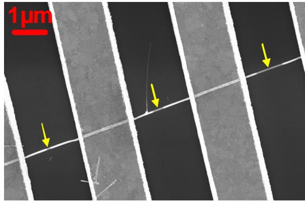
**Figure 1.9:** SEM micrograph of a  $10\mu\text{m}$  long nanowire contacted with three equidistant contacts. The silicides extending from the contacts grew at different rates and as a consequence the three unreacted silicon portions highlighted by the yellow arrows have different dimensions.
