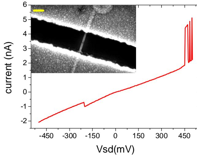
**Figure 3.16:**  $I$ - $V$  characteristic of a device with a channel length of 9nm (inset, scale bar 100nm) taken at 4.2K. Current switches due to electrostatically coupled charge traps are seen for both  $V_{sd}$  polarities.
