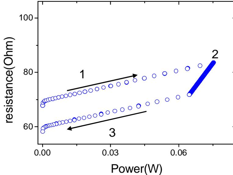
**Figure 3.4:** Resistance of a typical stripline defined by optical lithography as a function of the power dissipated. 1. The current is ramped up by a current generator and the resistance increases due to Joule heating 2. For a fixed driven current of 30mA the resistance shows a transient behaviour and starts to decrease as a function of time. 3. Once the new equilibrium value is reached the current is ramped down to zero.
