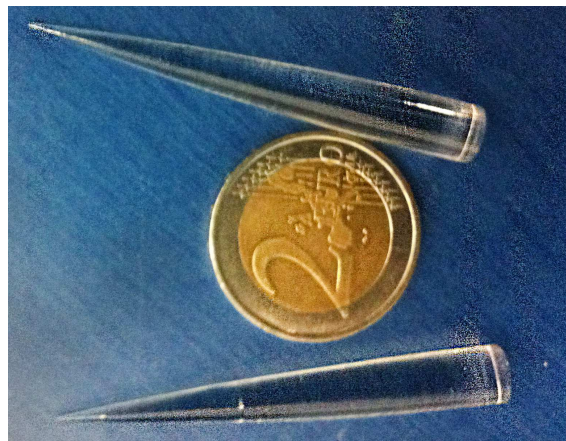
Figure 4.15: Fabricated concentrator prototypes (CPC types)
