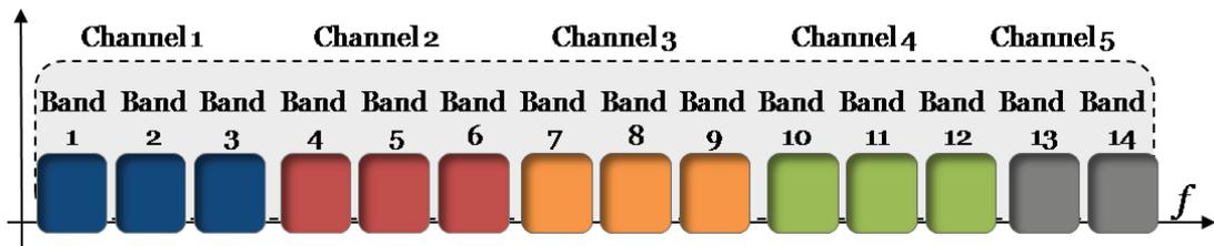
Figure 2.5: UWB spectrum bands in the MB-OFDM system
