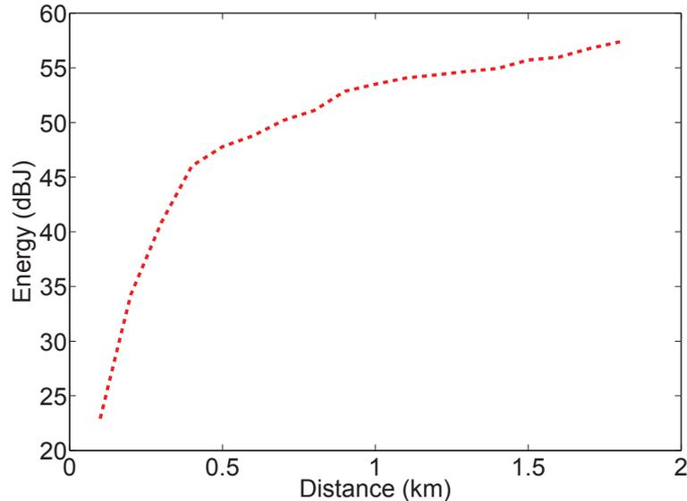
**Figure 2.6:** Energy consumption of conventional WiMAX systems
