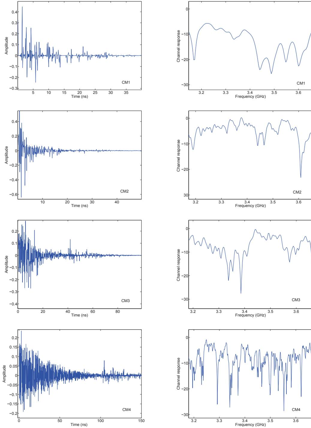
**Figure 2.10:** Example of UWB channel realizations for models CM1, CM2, CM3, CM4, in time and frequency domains
