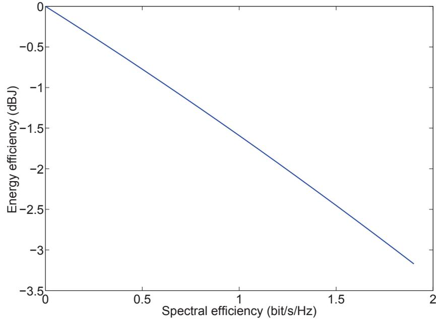
**Figure 3.2:** Relationship between spectral efficiency and energy efficiency.
