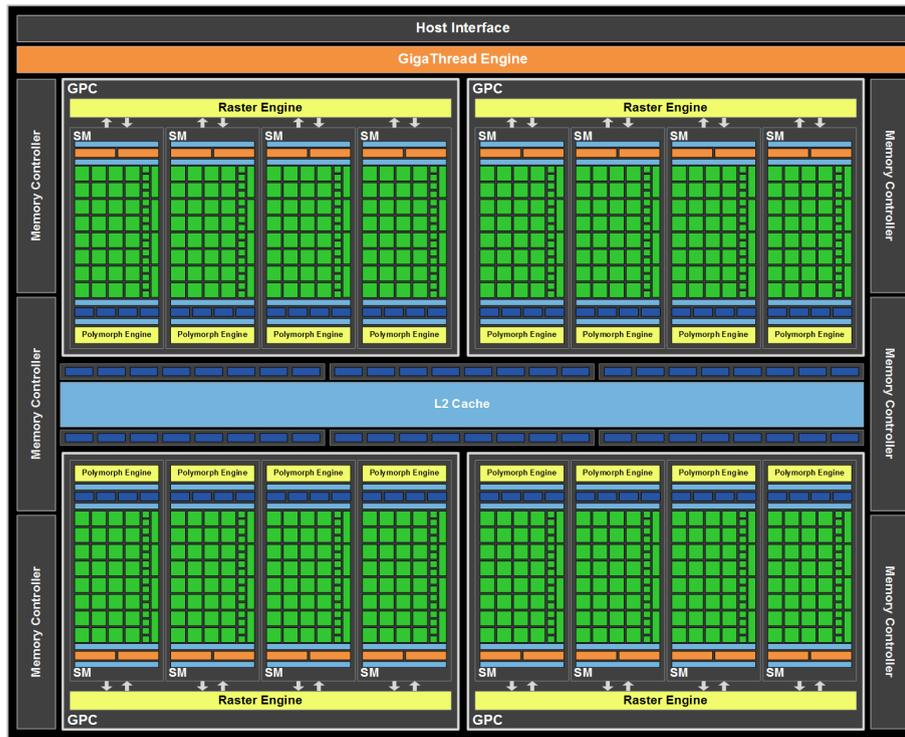
FIGURE 2.15 – Architecture *Nvidia Fermi* du *GF100*
