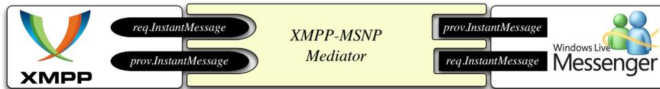
**Figure 6.3.** Making XMPP and MSNP components interoperable
