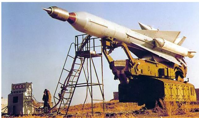
**FIGURE 7.7** – *Kholod mounted on the nose of a modified SA-5*
