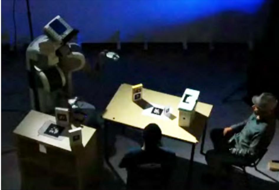
Figure 4.13: Example scenario with two humans, and the PR2 robot. There are different objects, reachable and visible by different agents with different effort levels.
