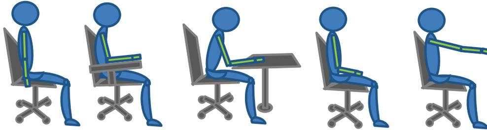
(a) Categorization of hand mode in different sitting postures of an agent. Left posture: hand in *rest mode*, rest mode type: *by posture*. Middle three postures: hand in *rest mode*, rest mode type: *by support*, because the hand is lying on a support, armrest, table, lap. Right most posture: hand in *manipulation mode*.
