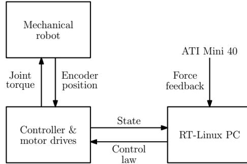
Figure 3.13: Conceptual representation of the real-time control architecture.
