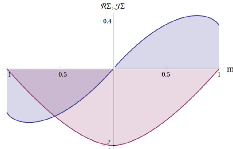
Figure 4.6: Energy dependence of the real (Blue curve) and imaginary part (Red curve) of the self energy. The variable used here is the normalized energy  $m = \frac{E}{4}$ . The imaginary part is always negative (True for the retarded self energy).
