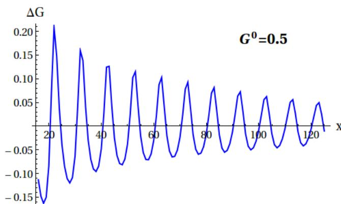
Figure 3.10: Change in the conductance (in units of  $\frac{2e^2}{h}$ ) as a function of the tip position. The tip is Lorentzian and the QPC realistic. The conductance of the systems without tip is  $G^0 = 0.5$ . The position  $x$  is in units of the the lattice step  $a$ . The effect has both signs: negative and positive.
