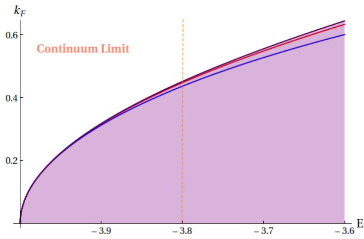
Figure E.1: different formulas of  $k_F$  near the bottom of the conduction band. Formula (b): Red curve, formula (c): Purple curve, formula (d): Blue curve. The continuum limit is the region of energies where the three curves are very close.
