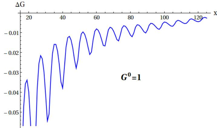
Figure 3.11: Change in the conductance (in units of  $\frac{2e^2}{h}$ ) as a function of the tip position. The tip is Lorentzian and the QPC realistic. The conductance of the systems without tip is  $G^0 = 1$  (First plateau of conduction). We notice that the effect is always negative.
