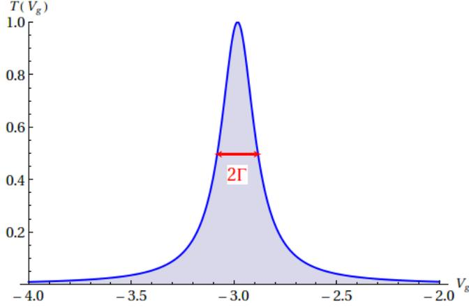
Figure 4.2: Transmission of the toy model as a function of the gate voltage  $V_g$ . The curve is a Lorentzian centered at  $E - 2\Re(\Sigma)$  and full width at half maximum  $2\Gamma$ . This curve is obtained for the Fermi energy  $E = -3.8$  and the coupling  $t_c = 1$ .
