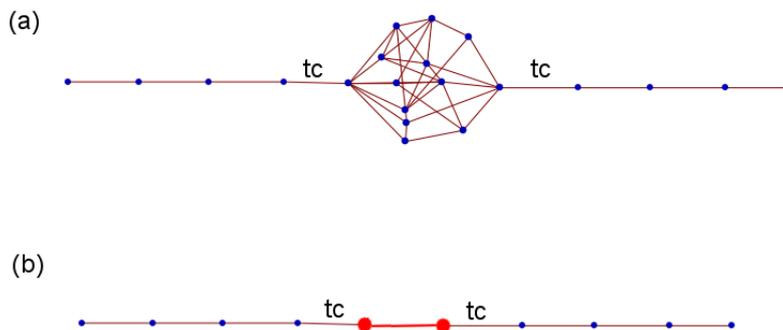
Figure 6.8: Decimation and renormalization procedure of the original model. We obtain a simpler model with only two random sites (red system).the coupling the two sites is also random.  $t_c$  is the coupling to the perfect 1D leads.
