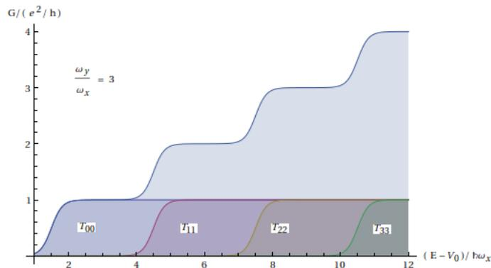
Figure 1.6: Transmission probabilities through a saddle point potential. The total transmission is obtained by summing over all the conducting channels.  $T = \sum_n T_{nn}$  (No channels mixing). Adapted from [11]
