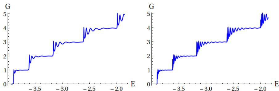
Figure 1.8: Transmission profile for a wide-narrow-wide model. In the right Fig, the length of the constriction is twice the length of the constriction which gave the left Fig. In both figures Fabry-Perot oscillations are visible. The bottom of the conduction band is taken at  $-4$  (units of  $t_h$ ). The conductance is expressed in units of the quantum  $2e^2/h$ .
