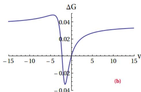
Figure 3.14: Numerical simulation for  $\Delta G$  vs the tip potential for Dirac delta model and half opened first mode. The tip is positioned at  $x = 40a$  far from the QPC. The resonance is a local extremum. ( $\Delta G$  in units of  $\frac{2e^2}{h}$  and 'a' is the step of the lattice).
