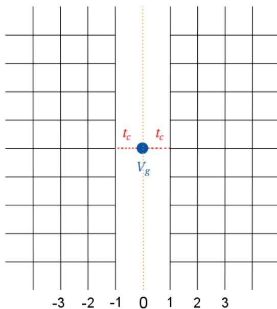
Figure 4.5: Left (from  $-1$  to  $-\infty$ ) and right (from  $1$  to infinite  $+\infty$  semi-infinite 2D leads. The point  $(0,0)$  is the place of the site biased to potential  $V_g$ . This picture helps to find the Green's function of a 2D semi-infinite lead from the Green's function of an infinite 2D lattice by the method of mirror images.
