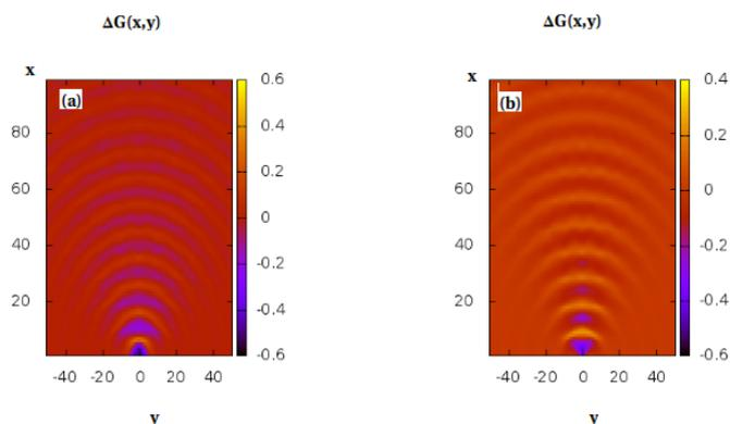
Figure 3.1: Spatial map of the zero temperature conductance change  $\Delta G(x, y)$  in units of the quantum conductance  $\frac{2e^2}{h}$  for two different models of the QPC. (a) a Wide-narrow-wide model shown in Fig (1.7). (b) Potential  $V(x, y)$  defined with Eq. (3.1). The effect of the tip on the 2DEG is modeled with an on-site potential at position  $(x, y)$ .
