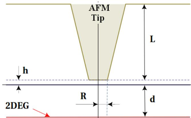
Figure 3.8: Geometry used in Poisson-3D simulation. adapted from [37]
