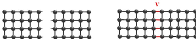
Figure 2.5: The whole system is constructed by gluing disconnected parts. The calculation of the Green's function is easily obtained using the Dyson equation in a recursive algorithm
