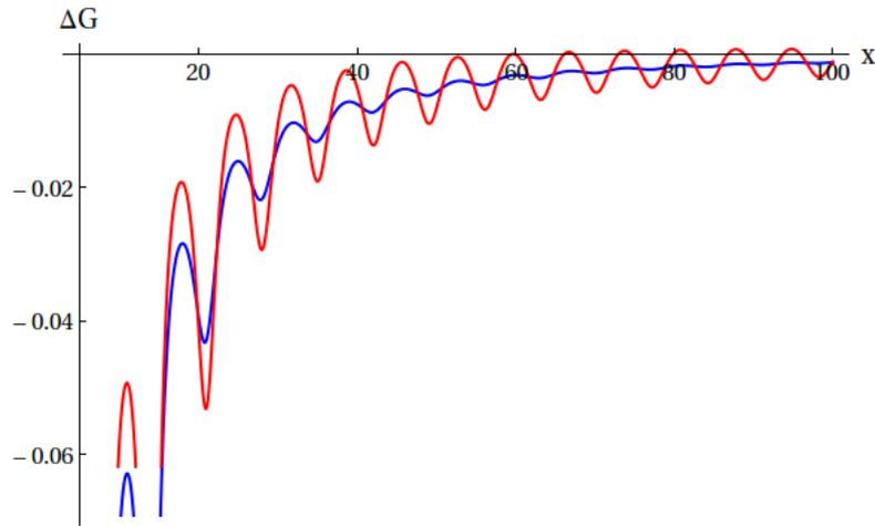
Figure 4.8: Thermal enhancement of interference fringes: The blue curve represents the conductance change  $\Delta G$  as a function of the tip position  $x$  at zero temperature for the RLM. red curve represents  $\Delta G$  at higher temperature  $\mathcal{T} = 682mk$ . The system is fully open ( $T^\circ = 1$ ) and the Fermi energy is  $E_F = -3.8$ . The lattice step is  $a = 2nm$  and  $\mathcal{A} = -5$ . The coupling to the leads is weak,  $t_c = 0.2$
