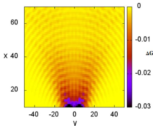
Figure 3.5: The map of the zero-temperature conductance change for the second plateau of conduction ( $G^{\circ} \simeq 2$ ). The effect of the tip is mostly visible in the directions  $\pm 45^{\circ}$ . The tip model is a delta function potential.
