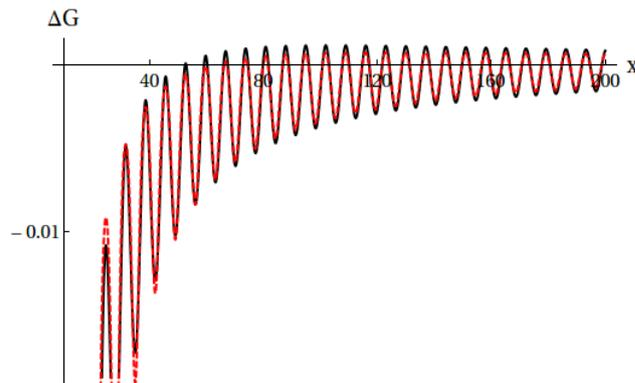
Figure 4.9: Temperature effect on the conductance change  $\Delta G$ : Comparison between the Sommerfeld expansion (black curve) and the result of the numerical integration of the exact formula which gives  $\Delta G$ . the comparison is good and becomes nicer far from the center of the system. The result is obtained for RLM with  $t_c = 0.2$ ,  $E_F = -3.8$  and  $\mathcal{T} = 682mK$ . The transmission of the system is  $T^\circ = 1$ .
