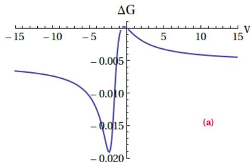
Figure 3.13: Numerical simulation for  $\Delta G$  vs the tip potential for Dirac delta model and completely open first mode. The tip is positioned at  $x = 40a$  far from the QPC. The effect is always negative and show a resonance at some negative potential value. ( $\Delta G$  in units of  $\frac{2e^2}{h}$  and 'a' is the step of the lattice).
