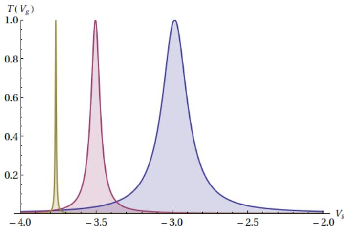
Figure 4.3: Resonant level model (RLM) transmission profiles for different coupling constant  $t_c$ .  $t_c = 1$  blue curve,  $t_c = 0.6$  purple curve,  $t_c = 0.2$  green curve. the Fermi energy is the same for all the curves ( $E_F = -3.8$ ).
