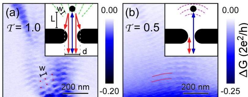
Figure 1.11: Imaging conductance changes by SGM technique for different opening of the QPC. In the case of  $\mathcal{T} = 1$  a checkerboard pattern of interference is visible whereas for less transmissions ( $\mathcal{T} = 0.5$ ) the picture shows ring pattern. From [18]
