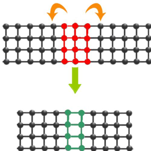
Figure 6.7: Decimation and renormalization procedure: We can remove one part (Red color) from a system and replace it by its effect on the remaining part to which it was attached. The potential on the neighboring sites are renormalized and so is the coupling between the remaining two parts
