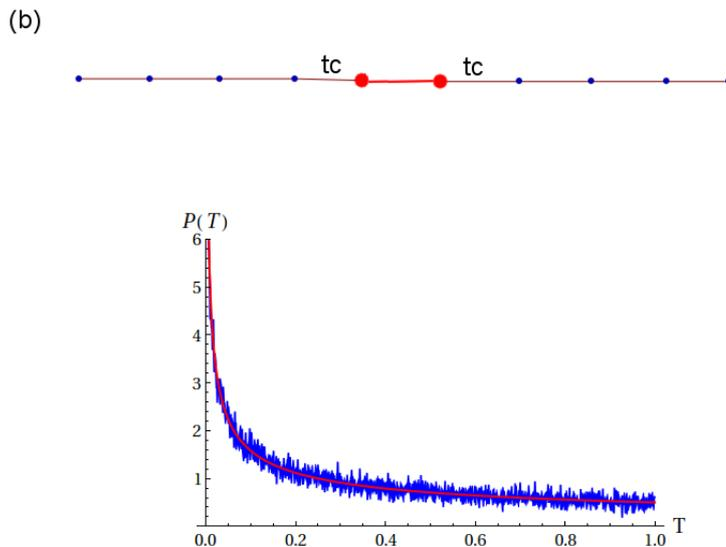
Figure 6.9: Transmission probability distribution: The transmission is distributed according to the law  $\frac{1}{2\sqrt{T}}$  (red color). The system considered in simulation is shown in top figure. The Hamiltonian is taken from Lorentzian orthogonal ensembles with mean  $(E - \Delta(E))$  and width  $\Gamma/2$ .
