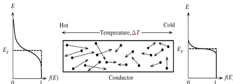
Figure 5.1: A conductor sketched between a hot and a cold electron reservoir. The Seebeck coefficient is given by the ratio between the difference of the two reservoirs temperatures and the voltage  $\Delta V$  induced by the difference  $\Delta\mathcal{T}$ . Taken from [63]
