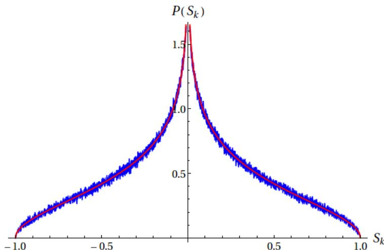
Figure 6.10: The distribution of the Seebeck coefficient  $S_k$  at half filling limit ( $E=0$ ).  $S_k$  is bounded and the distribution is singular at the origin. The numerical simulation is well fitted with the function obtained analytically. This Seebeck is for a chaotic cavity connected to two 1D leads (one conducting mode in each one).
