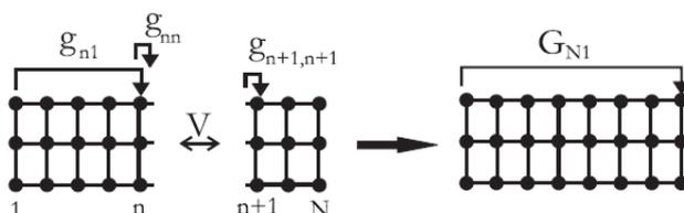
Figure 2.6: The different Green's function submatrices before and after connection. The Green's function is obtained recursively while the system is constructed slice by slice using the Dyson equation [24]
