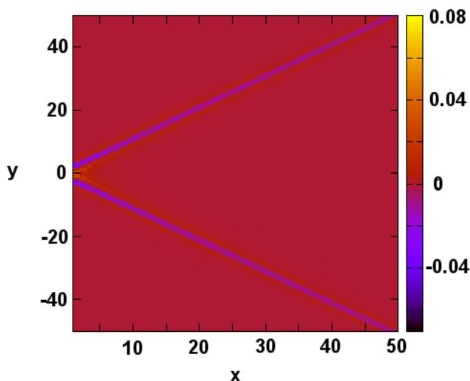
Figure 5.3: The change  $\Delta\Re\Sigma(x, y)$  in the real part of the self energy of a 2D lead as a function of the tip position. This result is given at the half filling limit. The effect of the tip is significant only in two directions  $\pm 45^\circ$ .
