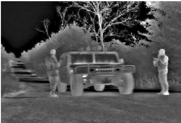
(b) Reconstruction OMP,  $SNR_{rec} = 16.2$  dB
