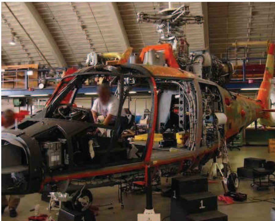
Figure 1.3: The backbone and circuitry of a eurocopter HH-65.
