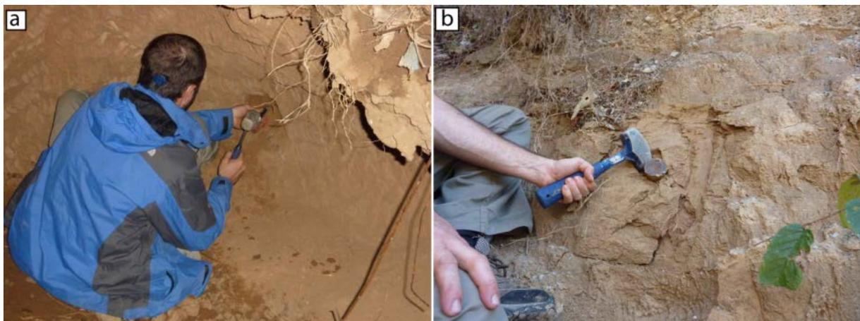
*Figure 17: Pictures of sampling for OSL dating. (a) in Czero deposits, (b) at the base of N1 at the footwall of scorpion fault*
