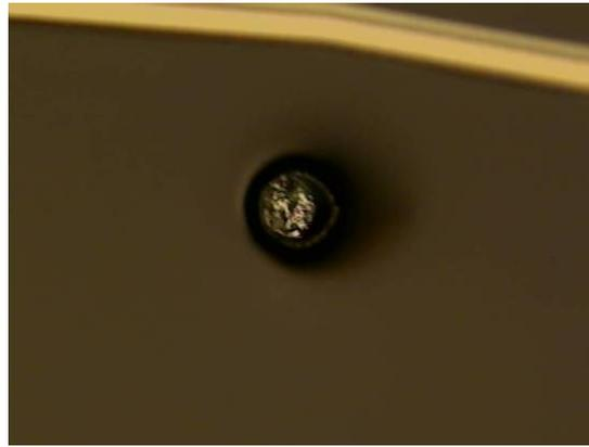
FIGURE 1.25 – Picture of a micropipe taken on-wafer during the fabrication process of SiC diodes at CNM of barcelona
