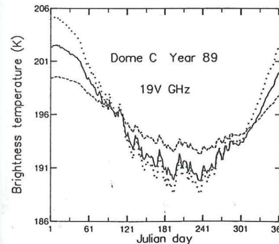
Fig. 7. Calculated brightness temperatures for different extinction coefficients and with a constant conductivity:  $K_e$  computed previously and equal to  $1.35 \text{ m}^{-1}$  (solid line),  $K_e + 50\%$  (dotted line) and  $K_e - 50\%$  (dashed line).
