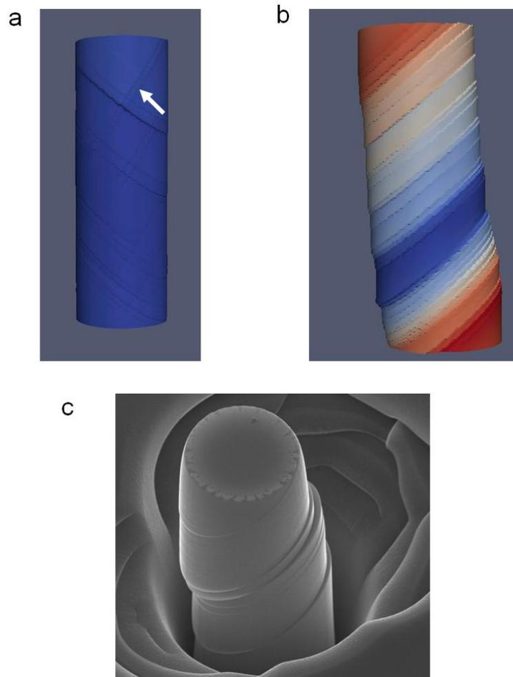
**Figure 7.16:** Shape of the deformed [2-1-12] pillar. DD simulation obtained with a CRSS of basal, prismatic, pyramidal  $\pi_1$  and pyramidal  $\pi_2$  of (a) 0.5, **5**, 100, 100 MPa, respectively and (b) 0.5, **30**, 100, 100 MPa, respectively. The white arrow in (a) indicates a slip mark from the prismatic slip. The actual deformed pillar is given in (c) for comparison.
