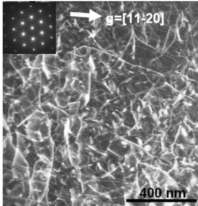
**Figure 4.13:** The dislocation structure on the basal plane resultant from compression of a [10-11] oriented column. Each of dislocation has the Burgers vector of  $\langle a \rangle$  or  $\langle c+a \rangle$ .
