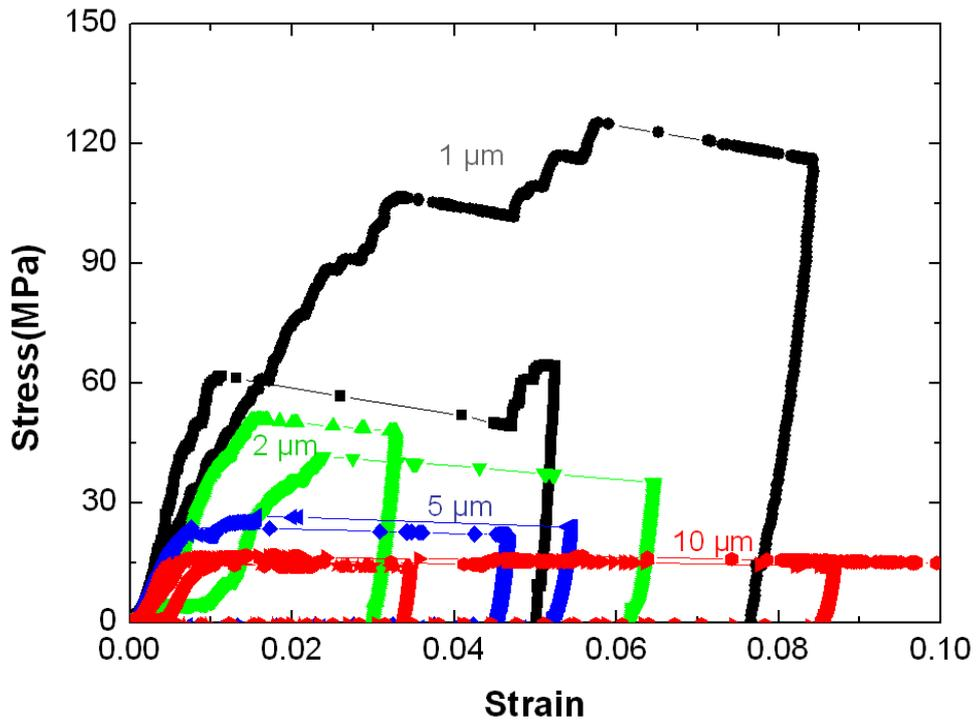
**Figure 5.4:** Size dependent stress-strain behavior of the [2-1-12] orientation.
