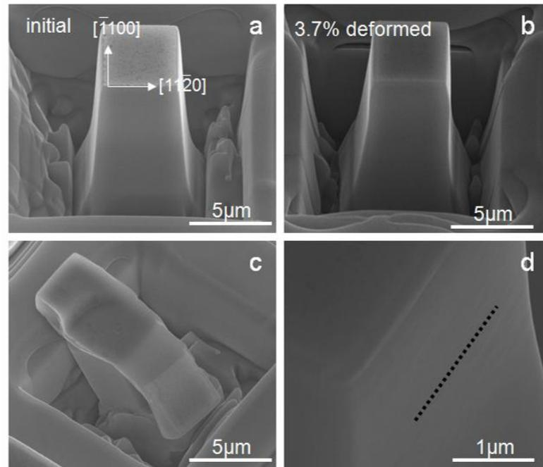
**Figure 8.2:** SEM images of a typical square type column. (a) initial (b) 3.7% deformed (c) strain burst occurred (d) slip traces. The slip trace in (d) indicated by black dot-line may likely correspond to the basal slip trace. However, more investigations are needed to confirm this hypothesis since it could also correspond geometrically to pyramidal slip system.
