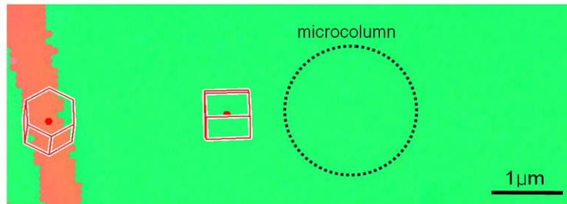
**Figure 3.3:** EBSD micrograph of the [11-20] sample surface. The [11-20] out of plane orientation is designated in green. Due to spark erosion, deformation twins (shown in orange) were not avoidable. Microcolumns were fabricated in twin-free regions.
