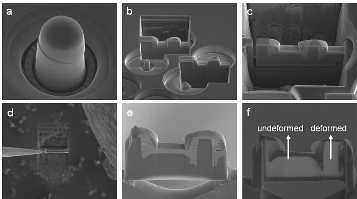
**Figure 3.6:** Typical working procedure of TEM sample by cross-sectioning. Figure shows (a) the initial deformed column, (b) regular and cleaning cross sections conducted on two columns, (c) through-cutting to partially free the lamella from the bulk material, (d) lift out of the lamella using an Omniprobe micromanipulator, (e) mounting of the lamella on a copper TEM grid, and (f) thinning to electron transparent thickness.
