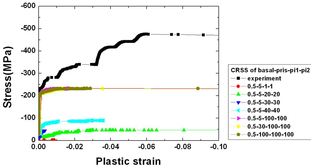
**Figure 7.1** Stress-plastic strain curve with different CRSS on the hcp slip systems.
