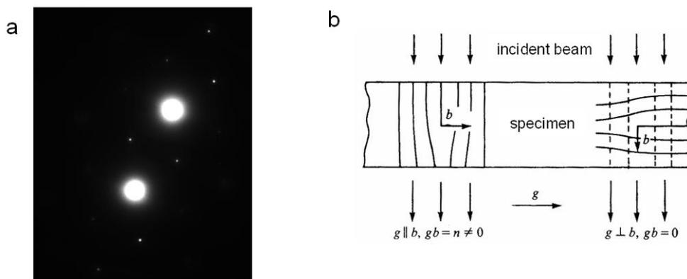
**Figure 3.11:** (a) Typical two beam condition used in dislocation imaging. (b) The dislocation can be visible or invisible depending on the reflected beam. The dislocations are analyzed by comparing the images of different reflection conditions.
