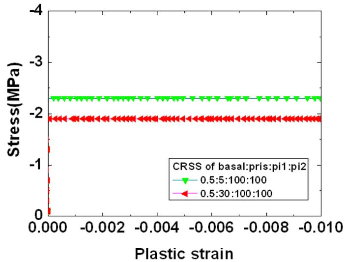
**Figure 7.12** The DD simulation results of [2-1-12] orientation. In both cases, the stress saturates in the early stage of the deformation and no hardening is observed
