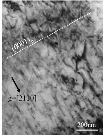
**Figure 4.21:**  $\langle a \rangle$  type dislocations on the prismatic plane within the untwinned region of a compressed  $[11\bar{2}0]$  oriented column. The zone axis is  $[0\bar{1}10]$ .
