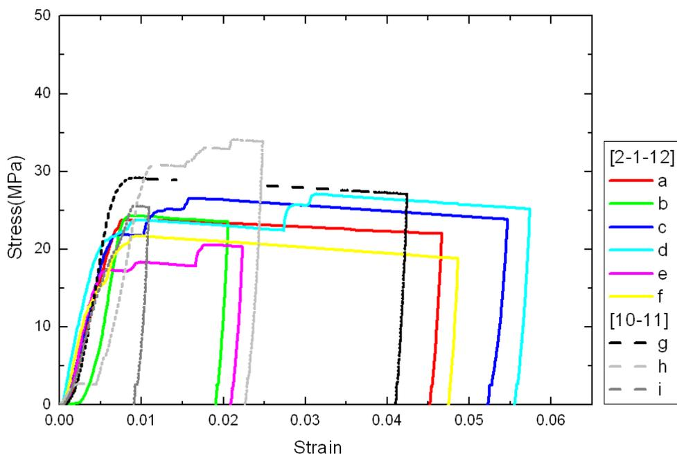
**Figure 4.8:** Stress-strain curve of [2-1-12] and [10-11] orientation.
