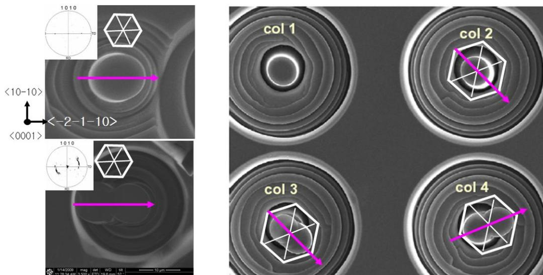
**Figure 5.3:** Massive shearing occurred along one of the three of  $\langle 11-20 \rangle$  directions. The apparent buckling or bending observed is not due to the misalignment of the flat punch tip or an inclination of the sample surface, since the direction of buckling is evenly distributed radially.
