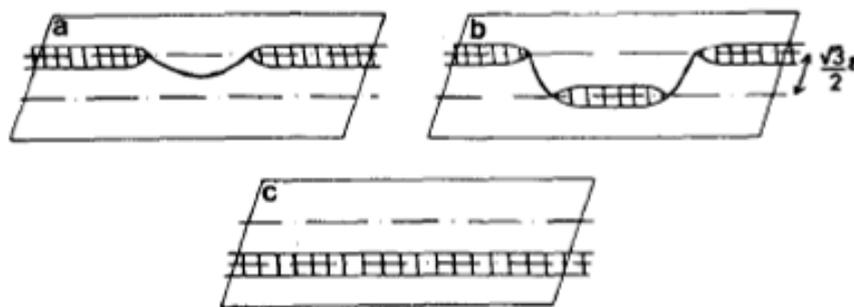
**Figure 2.6:** Kink-pair mechanism. ([Couret *et al.* 85]).
