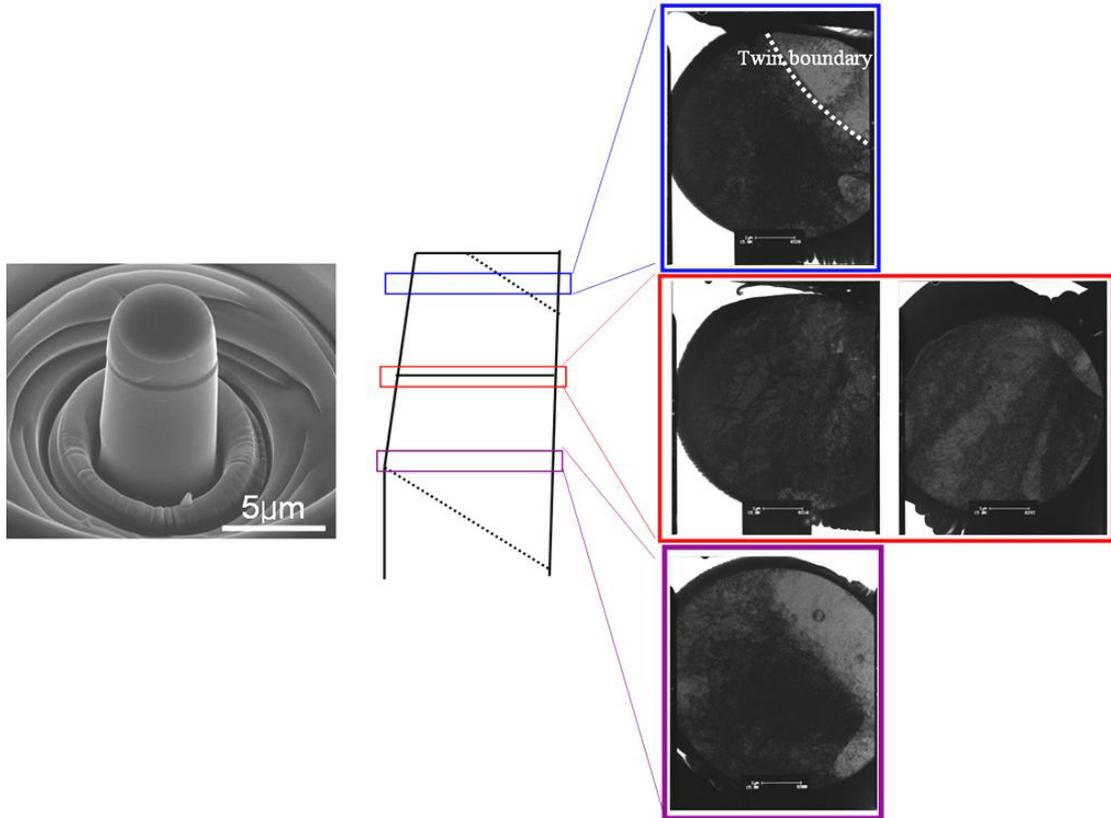
**Figure 4.25:** A compressed column which has been sectioned for TEM analysis in three positions along its compression axis, along with a schematic identifying the TEM foil positions relative to the twinned region, and TEM images from the three foils.
