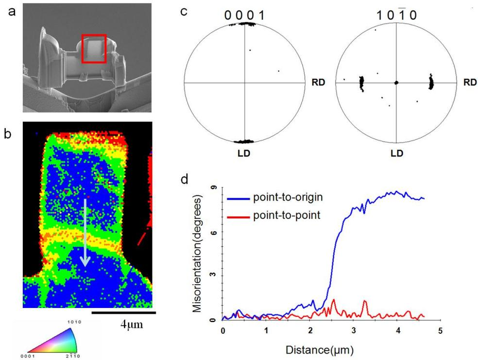
**Figure 4.4:** EBSD observations of a 10% deformed column. (a) The thinned section of the microcolumn and surrounding material attached to a TEM grid. (b) The EBSD orientation map of the column, along with (c) the corresponding pole figure and (d) point-to-point (red) and accumulated (blue) misorientation profile along a white arrow of (c). RD and LD in orientation map are radial direction and loading direction, respectively.
