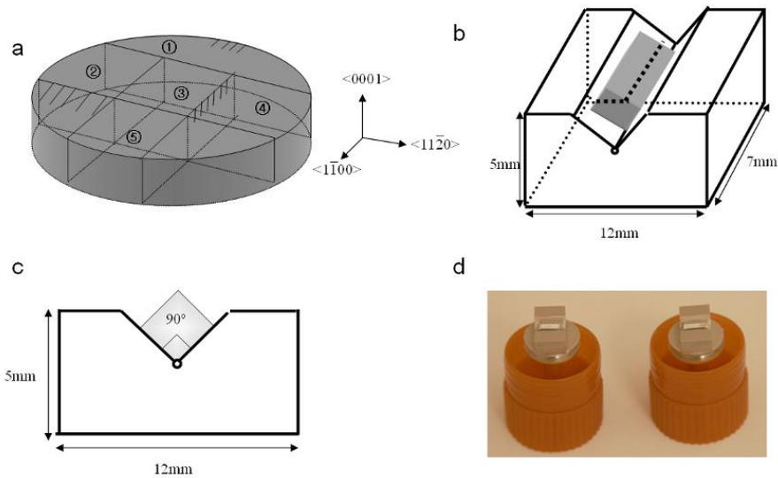
**Figure 3.1:** (a) Schematic image of the orientation and cutting direction of [0001] disk. (b) The specimen ④ and ⑤ were mounted to sample holder. (c) Front-view image of mounted sample and its holder. (d) Polished sample surface of the specimen ④ and ⑤.
