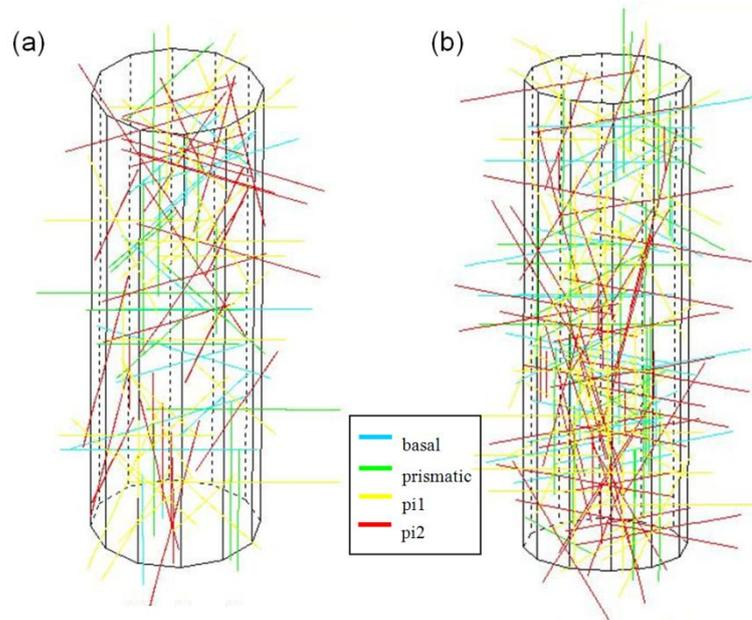
**Figure 7.3:** Initial dislocation configurations used in the simulations (a)  $1.2 \times 10^{13} \text{m}^{-2}$  (b)  $2.4 \times 10^{13} \text{m}^{-2}$ . Each of pillars has  $2 \mu\text{m}$  of diameter.
