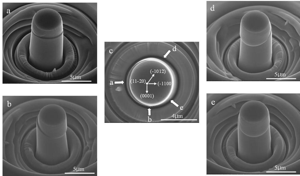
**Figure 4.17:** SEM images of a deformed column from different points of view, as indicated.
