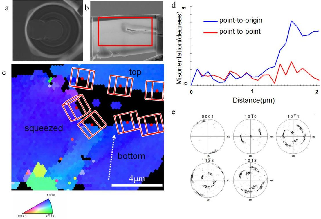
**Figure 4.5:** EBSD observations of a column having undergone massive, unstable slip. (a) A plan-view SEM image of the deformed column and (b) an SEM of the thinned out cross section through the column. (c) The EBSD orientation map showing the lattice rotations along with the associated (d) misorientation profile and (e) pole figures. RD and LD in orientation map are radial direction and loading direction, respectively.
