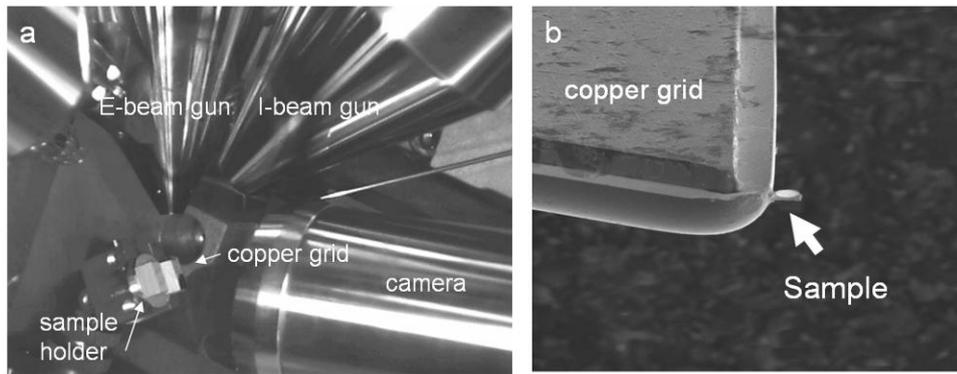
**Figure 3.9:** EBSD measurement inside the FIB Nanolab 200. A CCD camera image inside the microscope chamber is shown in (a) and an example of a sample used for EBSD measurement is shown in (b). The bright ring in the middle is the sample.
