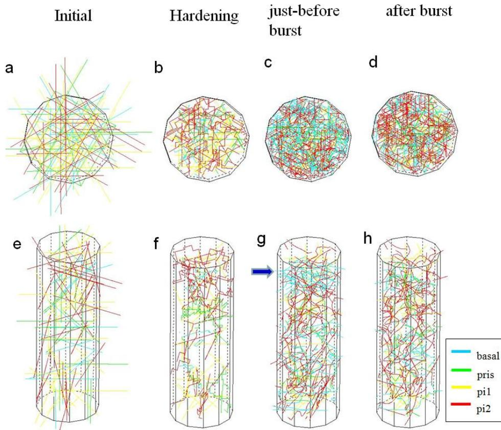
**Figure 7.8:** Dislocation organization inside the column with the deformation. (a), (e) initial configuration, (b),(f) hardening stage (c),(g) just before strain burst, (d),(h) just after burst. Strain burst is initiated by the basal dislocations pointed out by the blue arrow in (g).
