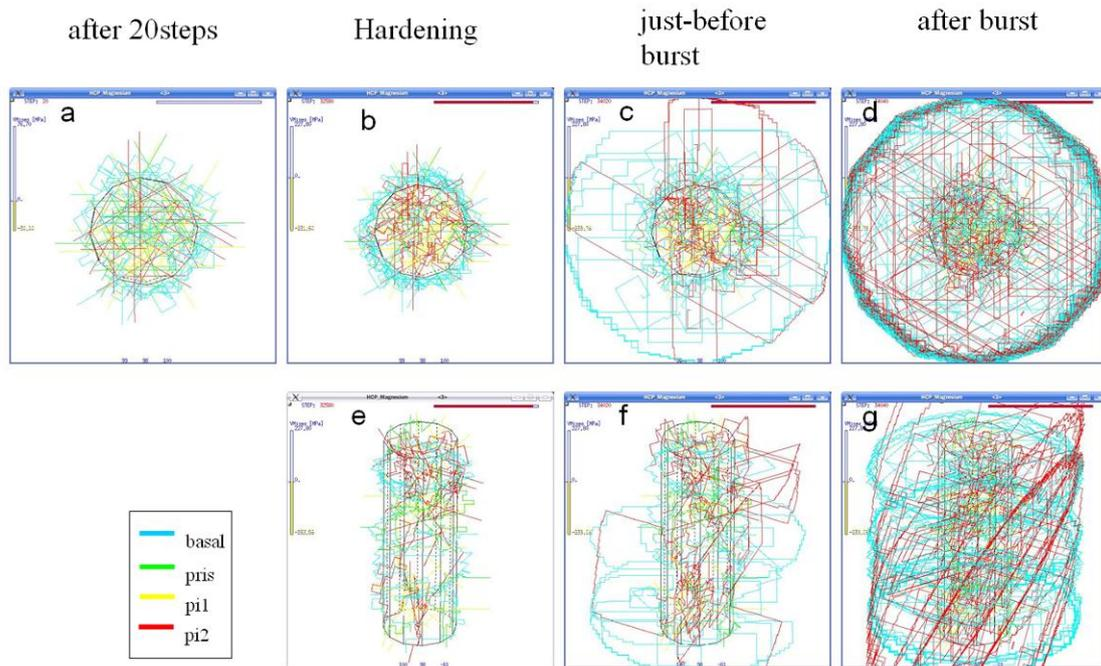
**Figure 7.9:** The dislocation features both outside and inside the column with the deformation. Snapshots taken at different time steps (a) after 20 steps of the simulation, (b), (e) during the hardening stage, (c), (f) just before the strain burst (d),(g) just after the strain burst
