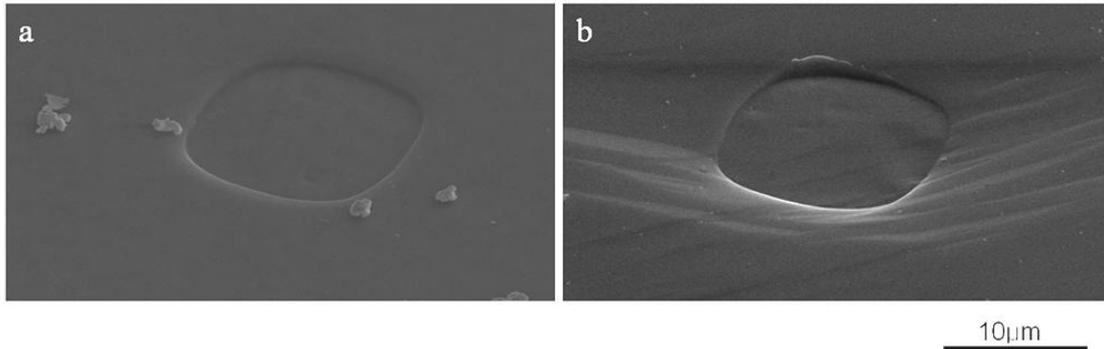
**Figure 3.14:** The imprint of a flat punch indent on (a) the [0001] surface and (b) the [2-1-12] surface. Microcompression test has been performed with a 15µm diameter circular punch. We also can see the plastic anisotropy of magnesium single crystal from the punch imprint.
