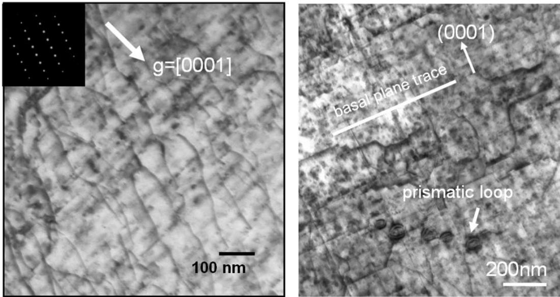
**Figure 4.7:** TEM shows  $\langle c \rangle$  component dislocation. The zone axis is  $[2-110]$ . Prismatic loops were only observed when  $g=[0001]$ .
