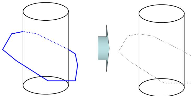
**Figure 6.3.** Elimination of dislocation loops when totally located outside the pillar.
