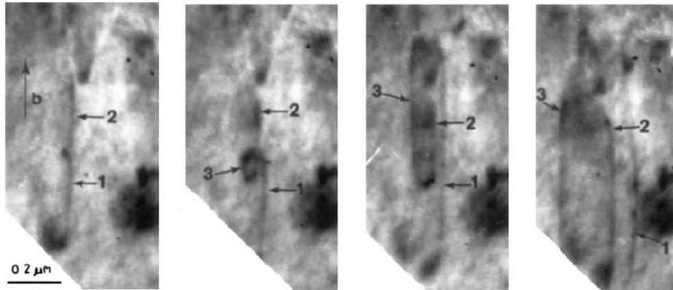
**Figure 2.5:** Prismatic slip in magnesium at 300 K The movement of screw dislocations is controlled by the kink-pair mechanism. A dislocation loop formed at a pinning point expands by the rapid movement of its edge parts ([Couret *et al.* 85]).
