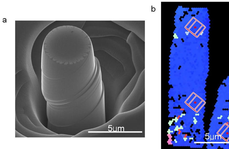
**Figure 4.11:** An SEM image of a typical deformed [2-1-12] column is shown in (a). EBSD shows no twin in the deformed region, and confirms that the sample is loaded in a direction 45 degrees to the basal plane normal.
