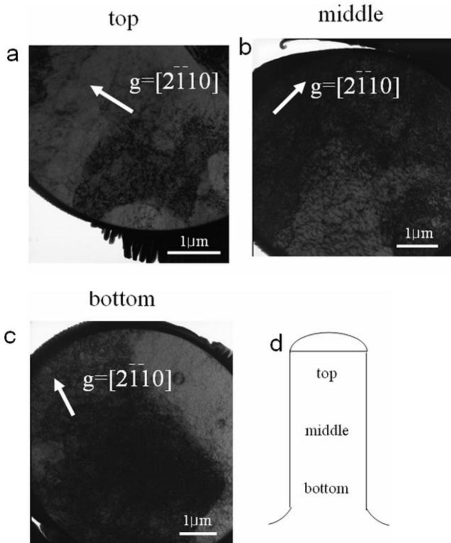
**Figure 4.27:** Size dependence of subgrain on the distance from the top of the column. With increasing distance from the top part of the column, the number of subgrains decreases and the size of the subgrains increases. The zone axis is  $[0001]$ .
