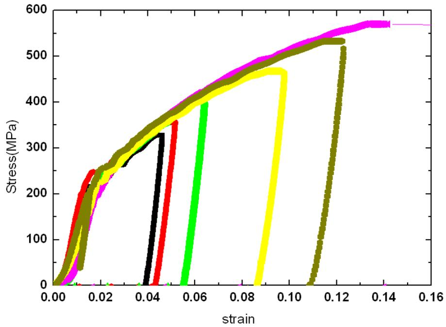
**Figure 4.1:** Stress-strain behavior of 6 microcolumns with nominal mid-height diameter of  $5\mu\text{m}$ .
