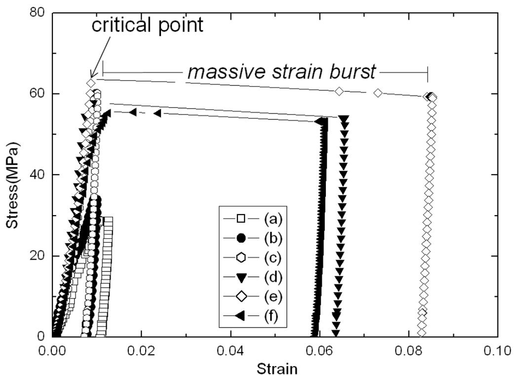
Figure 4.15: Stress-strain responses of [11-20] orientated columns
