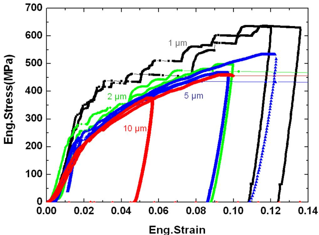
Figure 5.1: Size dependent stress-strain behavior of the [0001] orientation.
