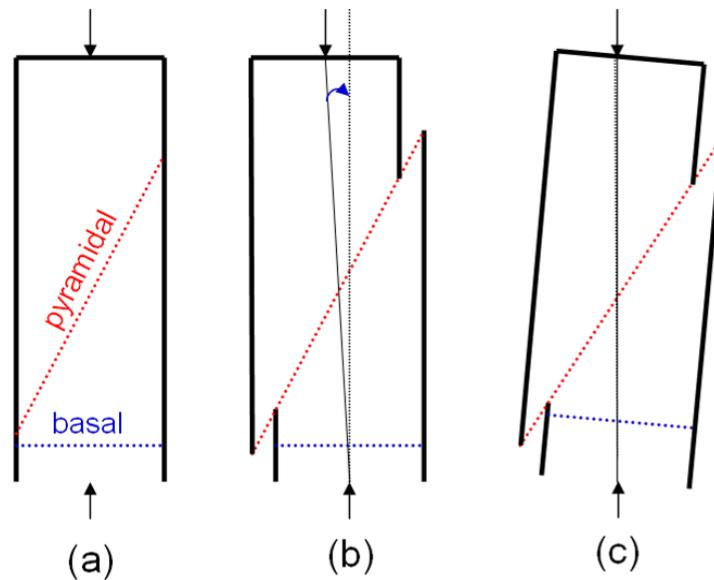
**Figure 7.10:** Schematic description of the deformation process in the case of [0001] orientation of the compression axis. (a) initial (b) activation and gliding of pyramidal slip systems. The pillar axis is tilted from the initial loading axis due to the local misorientation induced by pyramidal slip. (c) massive basal slip occurs.
