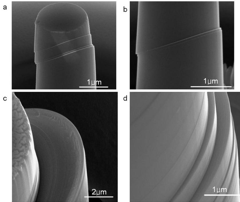
**Figure 4.10:** SEM images of slip steps occurring from compression in the 45 degree orientation columns. Images are taking from a tilted angle such that the slip lines do not show a 45 degree angle in-plane.
