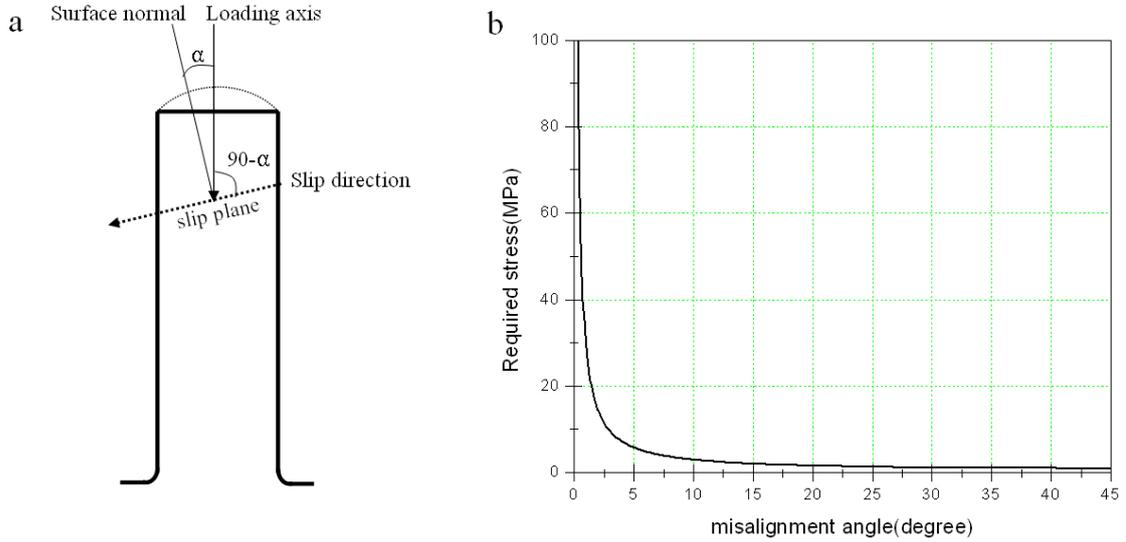
**Figure 4.6:** (a) Schematic showing a column and basal slip plane with plane normal at an angle of  $\alpha$  from the loading axis. (b) Required applied stress for the activation of basal slip as a function of misalignment angle, assuming a CRSS of 0.5 MPa.
