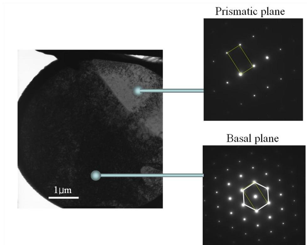
**Figure 4.26:** TEM micrograph and the two corresponding diffraction patterns showing subgrains in the twinned region. Subgrains were not observed in the untwinned region.
