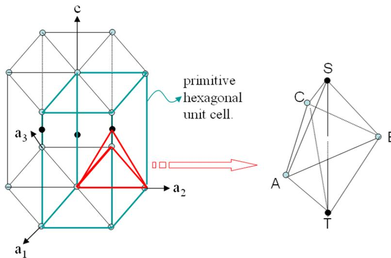
**Figure 2.1:** Hexagonal close-packed structure. The hexagonal primitive unit cell contains 2 atoms and Thomson-tetrahedron which is used in fcc can be applied to explain the slip system
