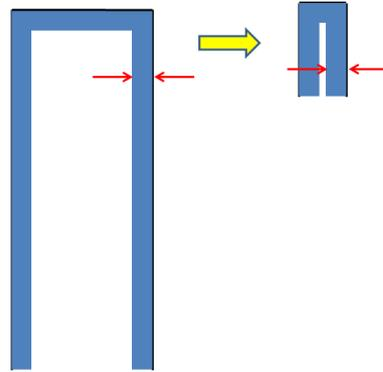
**Figure 8.3:** Schematic explanation of the Ga damage layer both for large and small pillars.
