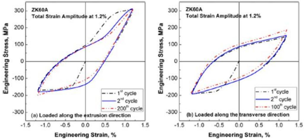
**Figure 2.9:** Strain hysteresis due to twinning during cyclic loading is shown with two loading direction ([Wu *et al.* 08]).
