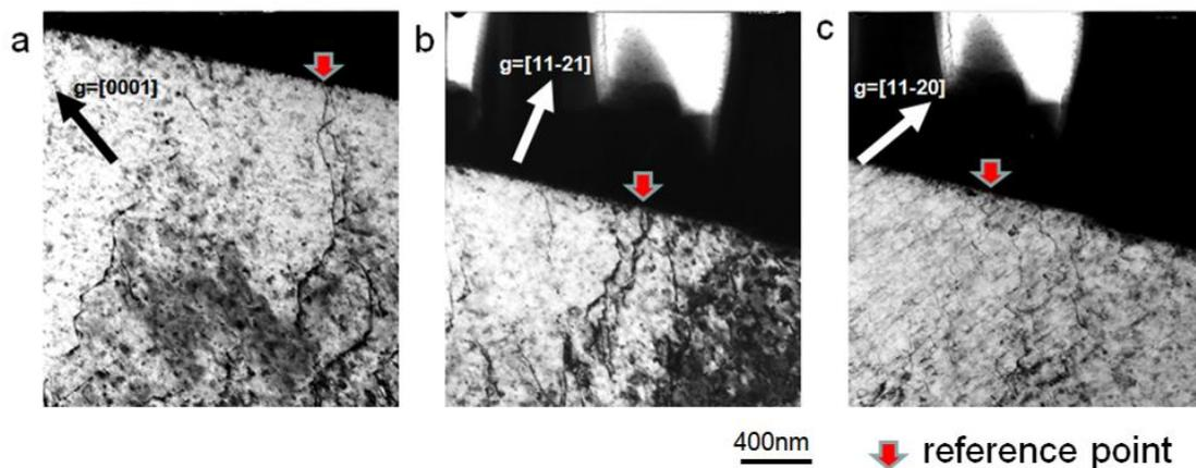
**Figure 4.12:** The dislocation extinction condition analysis by different diffraction conditions identifies the observed dislocation in (a) and (b) as  $\langle a \rangle$  dislocations. The zone axis is  $[1-100]$ .
