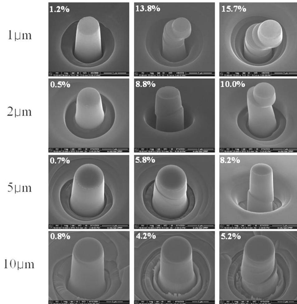
**Figure 5.7:** SEM images of deformed [11-20] oriented pillars with varying size and plastic strain. As the size decreases, multiple massive slip bands on the basal plane were observed after the strain burst.
