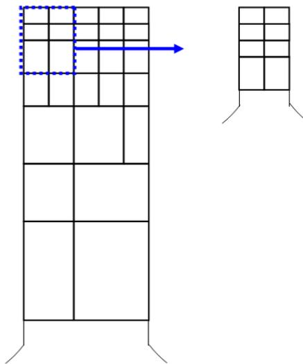
**Figure 5.10:** Schematic image showing the gradient in the size of the subgrain structure for a relatively large and relatively small pillar. It can be seen that the absolute size of the subgrain structure at the mid-height position in the small pillar is smaller than that for the large pillar.
