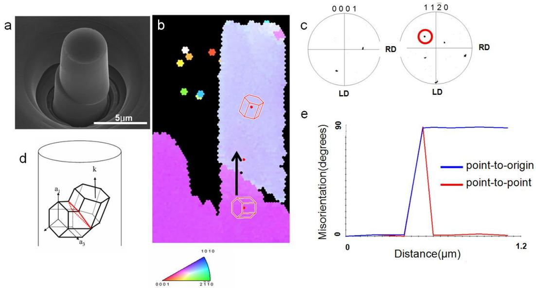
**Figure 4.20:** (a) SEM image of a deformed column initially oriented along the [11-20] loading axis showing massive basal slip. The associated (b) EBSD map, (c) corresponding pole figure, (d) relationship of the twin and parent orientations, and (e) misorientation profile showing the resultant twinned structure. RD and LD in orientation map are radial direction and loading direction, respectively.
