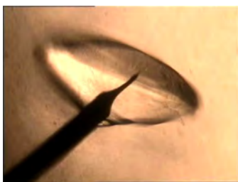
Figure 4 BPTI (20 mg/mL – NaCl 1.6 M) nucleation in the vicinity of the tip in 0.5% agarose gel (0.8 V–0.74 \mu A), length of experiment 12 h. As reference, the W-electrode wire diameter is 125 \mu m. After [7] with permission of ACS (see online version for colours)
