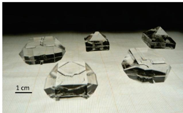
**Figure 4.** Examples of high purity KDP crystals grown at 10 mm/day (on millimeter paper). Three crystals are grown with horizontal  $c$ -axis (parallel to the image); two (in the back, on the right) are grown with vertical  $c$ -axis.
