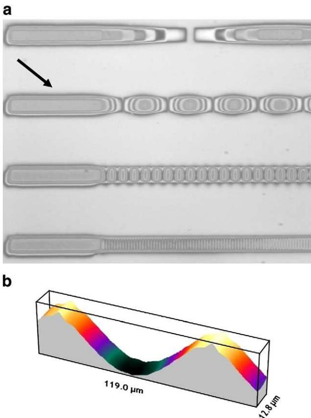
Fig. 9. Long period Bragg grating structures. (a) Picture of 4 long period Bragg gratings with pitches varying from 6 to 40  $\mu\text{m}$  in 3  $\mu\text{m}$  wide waveguides. (b) 3D interferometric microscope view of the structure indicated by an arrow on the top picture.
