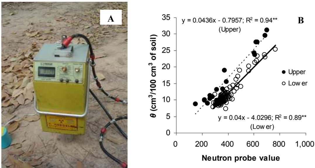
**Figure 13** A) A neutron probe (3322, Troxler, Research Triangle Park, North Carolina, USA).
