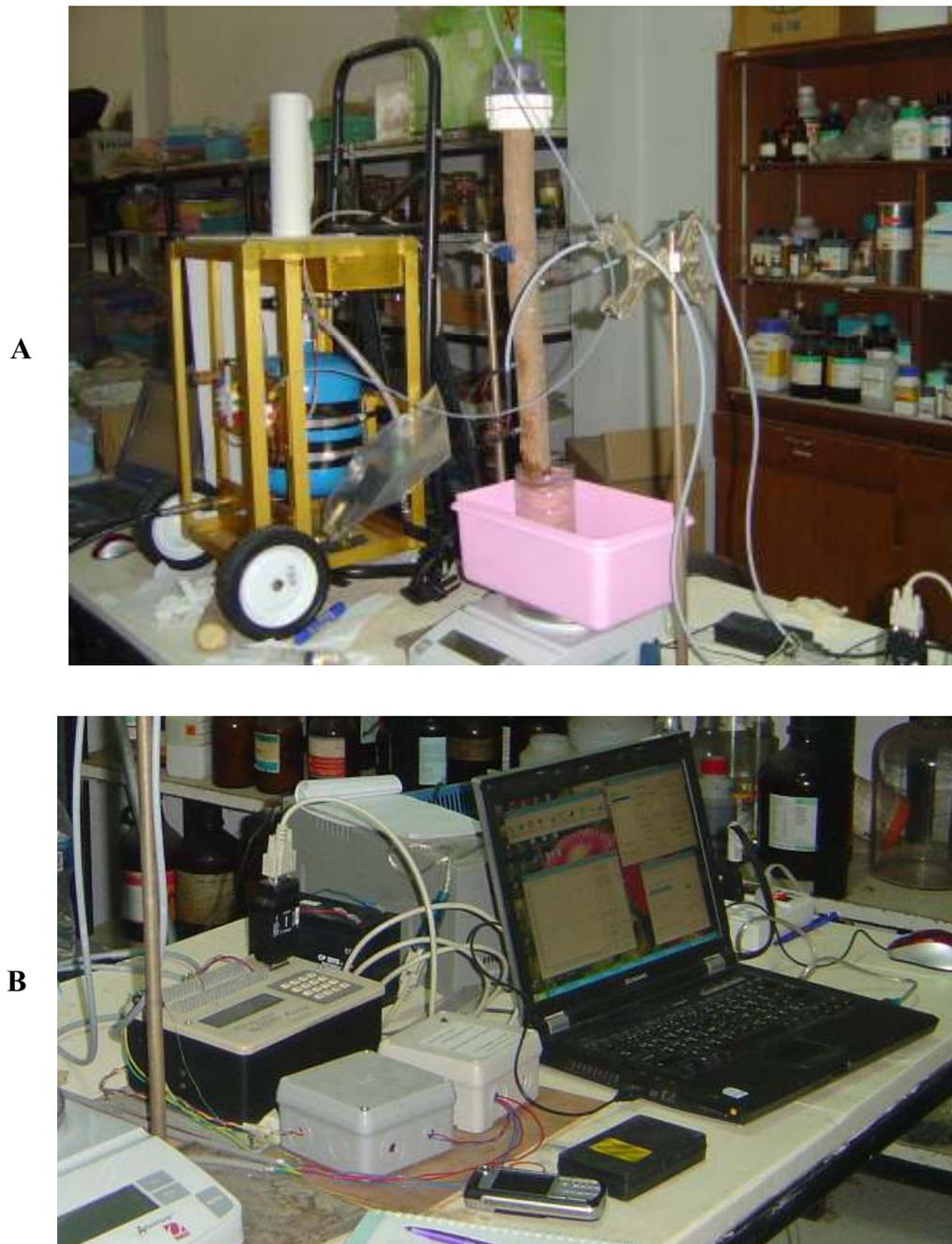
**Figure 9** A) Installation of cut stem with a high pressure flow meter (HPFM) and weighing water flowing out of cut segments by 0.01 g accuracy balance. Also, the two sets of Granier's type probe were inserted to the cut stem, which the distance between two set of probe was 10 cm.
