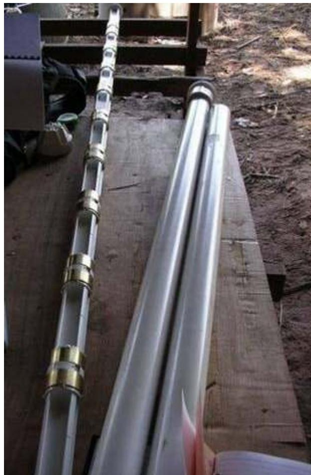
**Figure 14** A capacitive probe (EnvironSCAN System, Sentek Sensor Technologies, South Australia, Australia).
