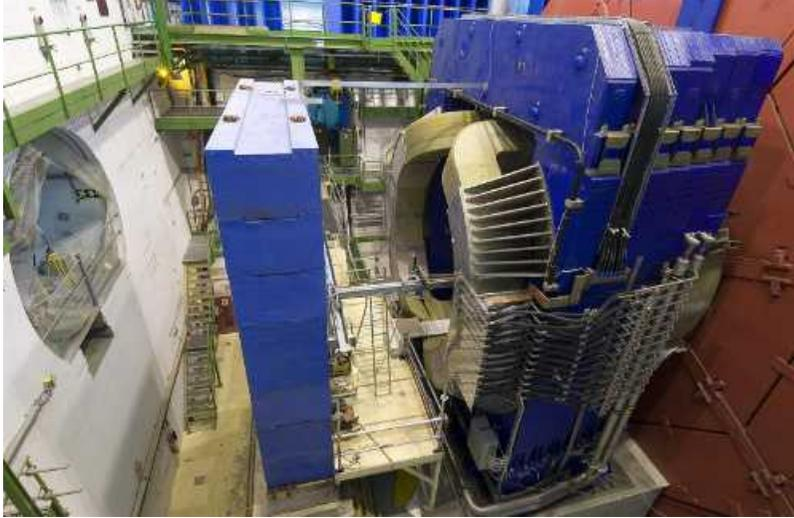
Figure 2.19: View of the muon filter (left) and dipole magnet (right).
