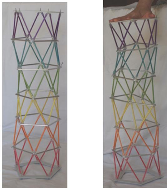
**Fig. 5.4:** Non-stiffened pentagonal structure — locking during packing
