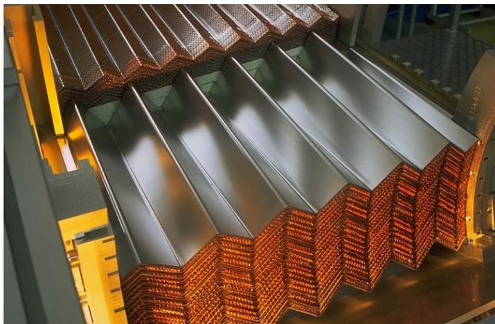
Figure 3.2: Photograph of barrel accordion-shaped electrodes and absorbers [83].
