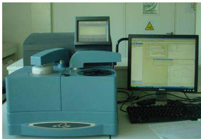
**Figure 5** Appareil DSC Q2000
